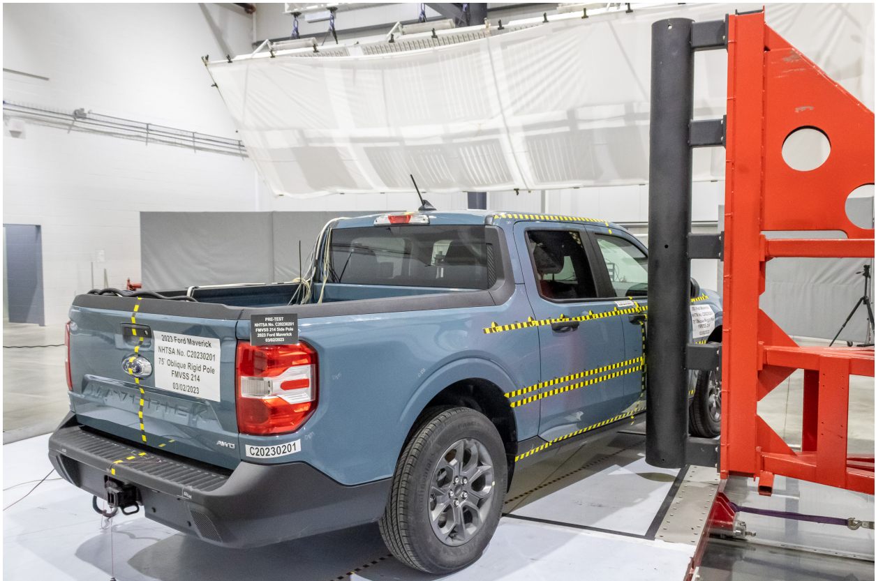
Figure A-8: Pre-Test Impacted Side \frac{3}{4} Rear View of Vehicle and Pole
