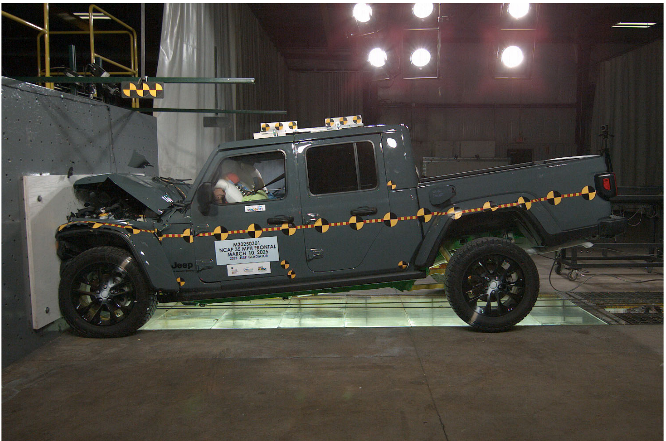
Photo No. 082 - 2025 Jeep Gladiator Sport 4x4 4-Door Pickup Frontal Impact Event
