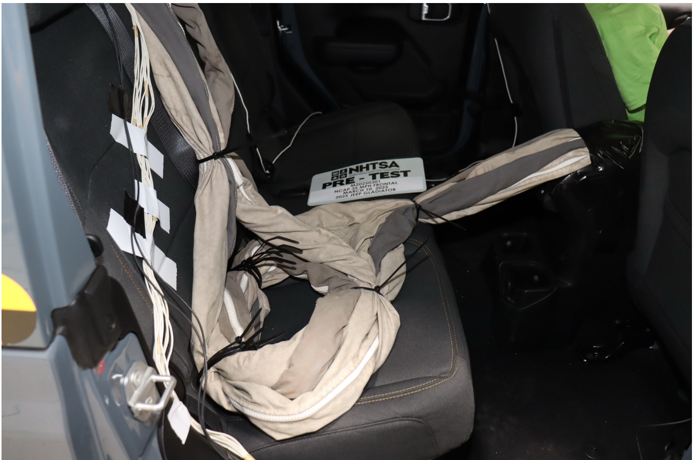
Photo No. 028 - Pre-Test Dummy Cable Routing
