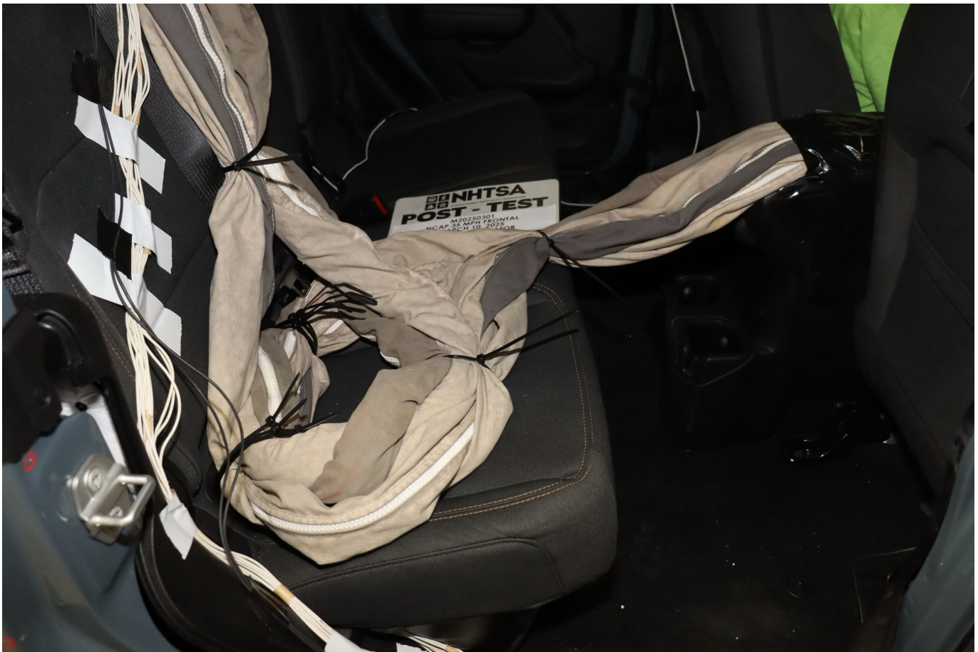
Photo No. 029 - Post-Test Dummy Cable Routing
