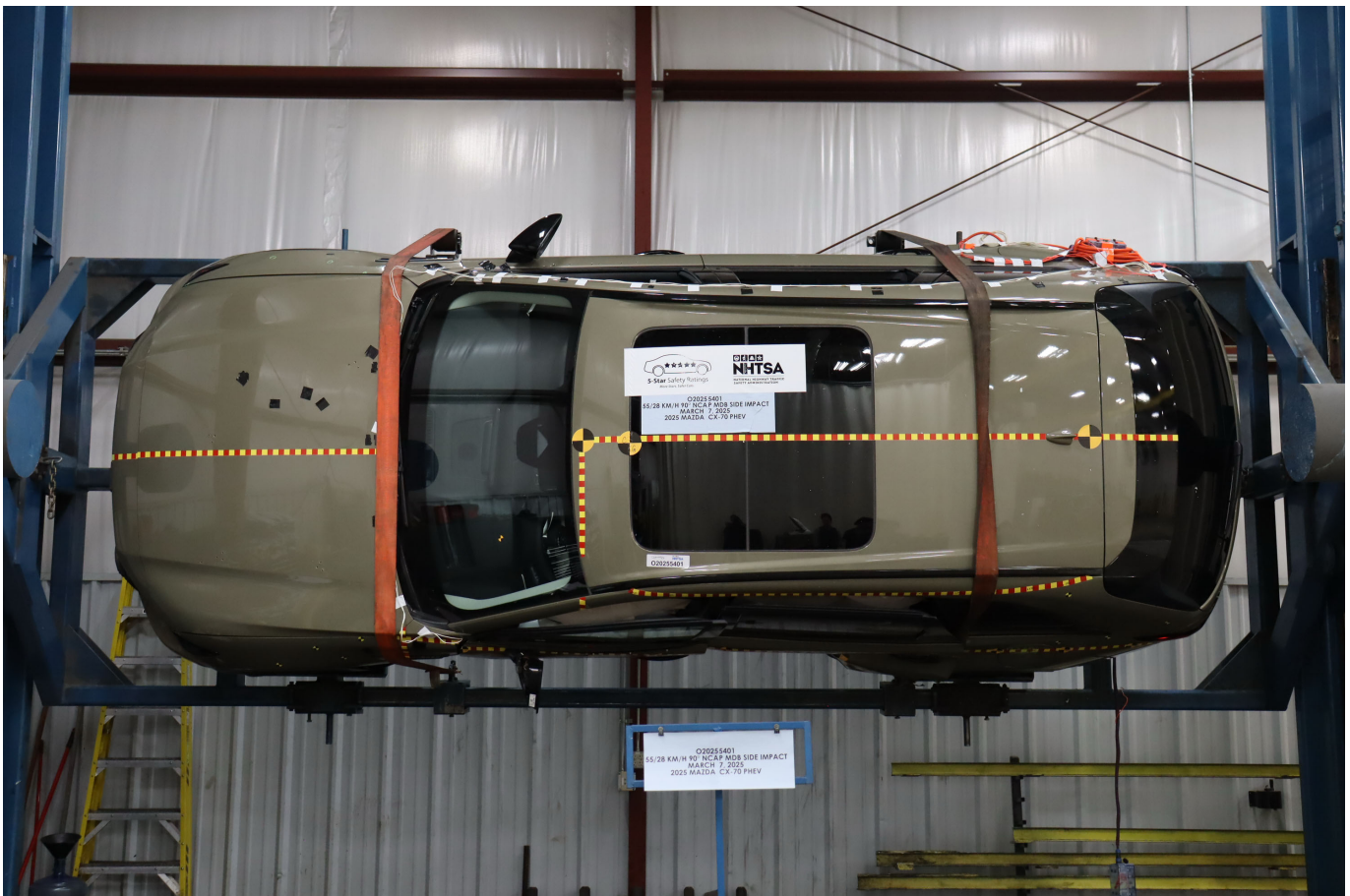
Photo No. 305-28 - FMVSS No. 305 Static Rollover at 90 Degrees
