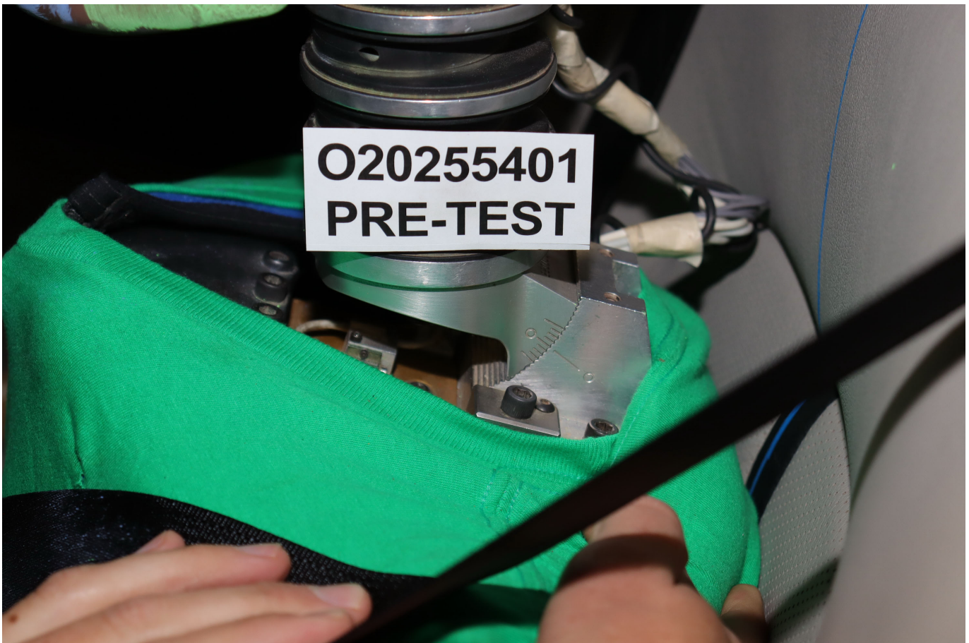
Photo No. 062 - Pre-Test View of Rear Passenger Dummy's Neck Showing Position of Adjustable Neck Bracket
