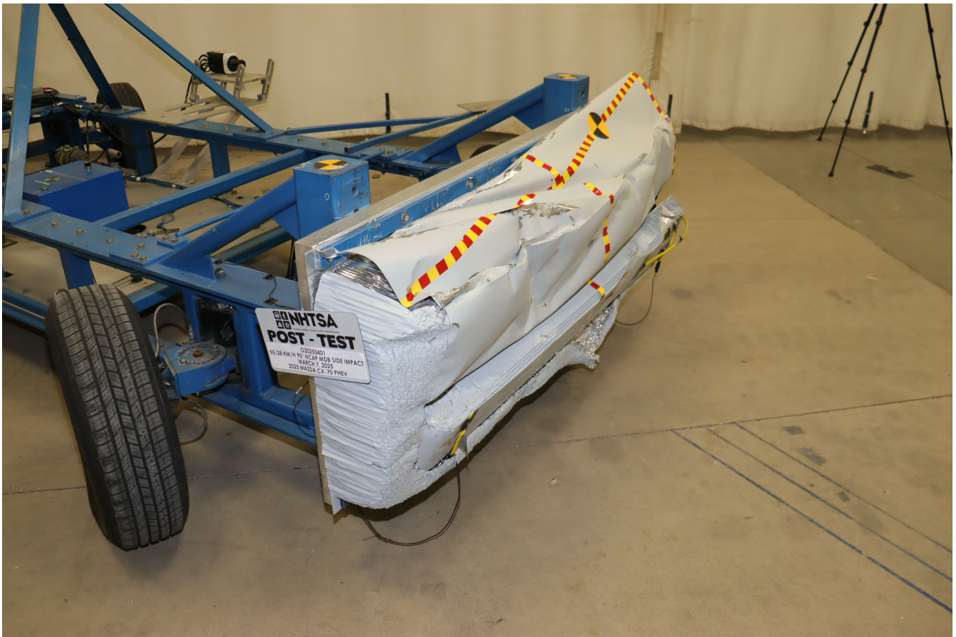
Photo No. 091 - Post-Test Right Side View of MDB Impactor Face
