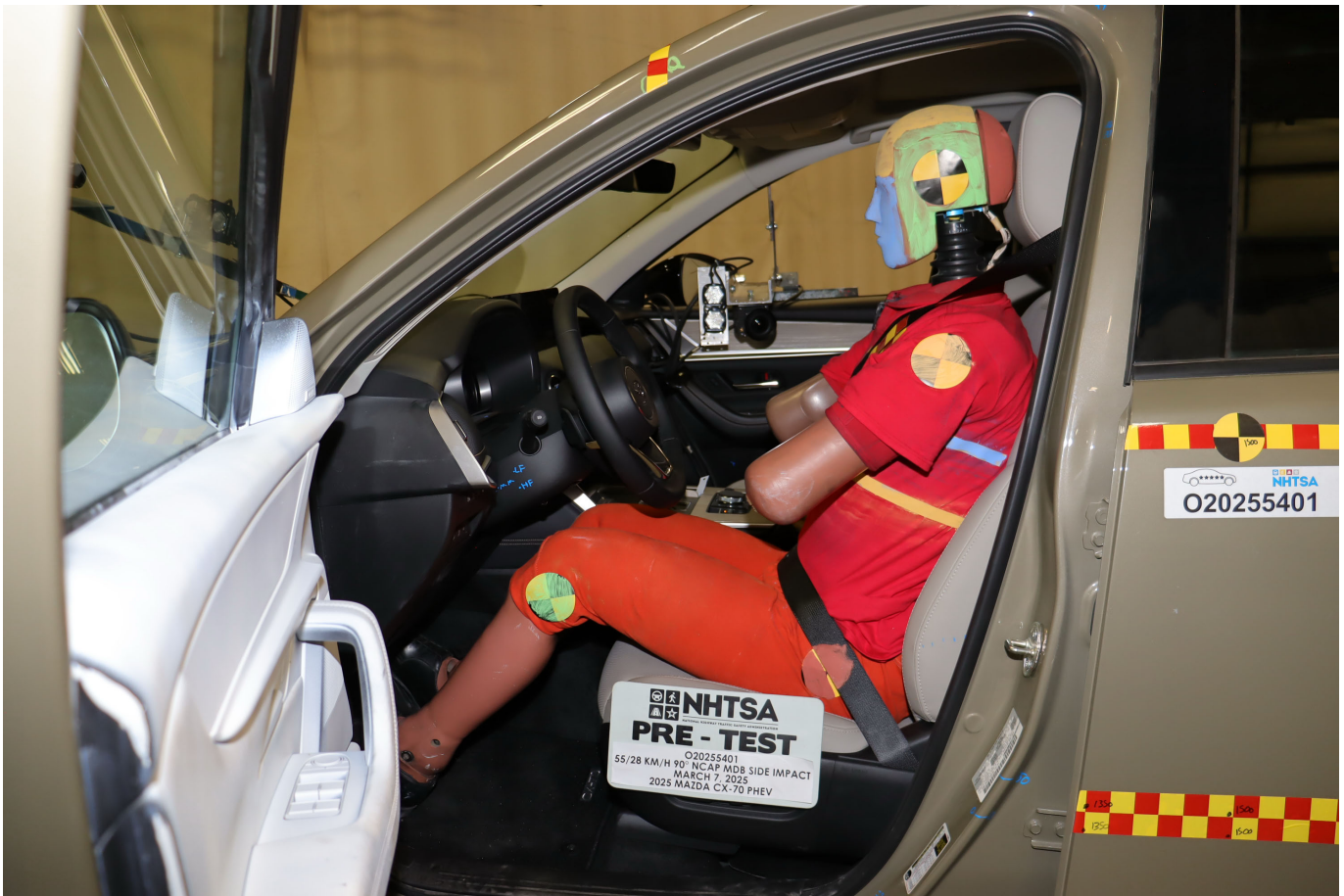
Photo No. 027 - Pre-Test Left Side View of Driver Dummy Showing Belt and Chalking
