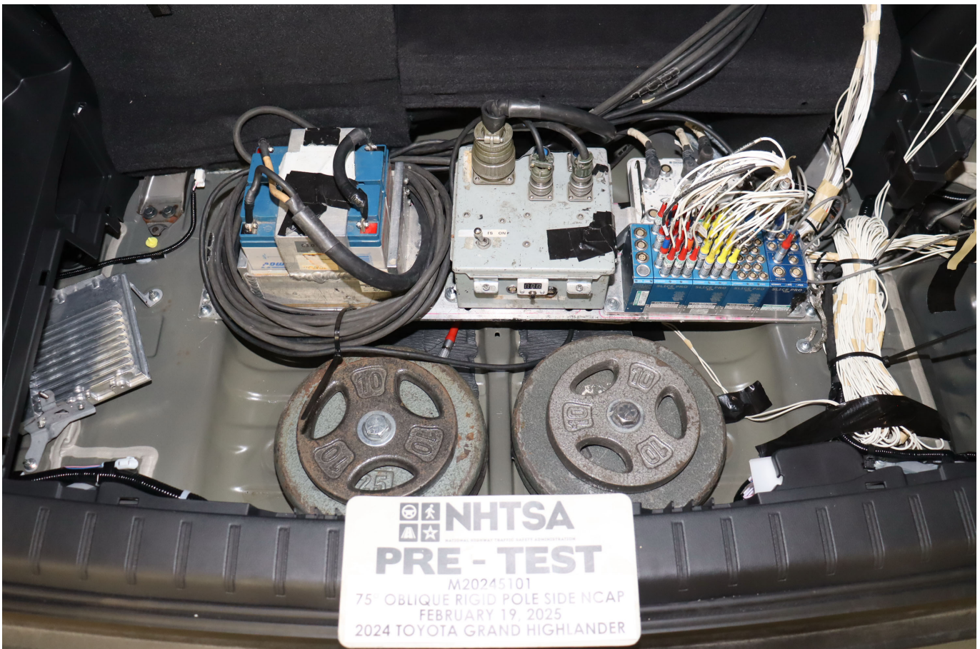
Photo No. 063 - Pre-Test Ballast View
