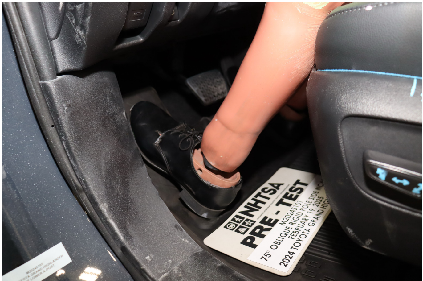
Photo No. 032 - Pre-Test Placement of Dummy's Feet
