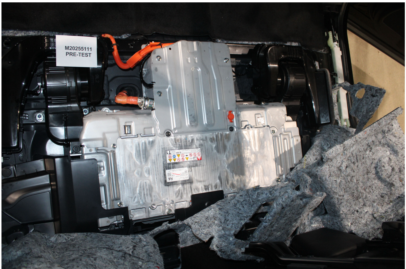
Photo No. 305-09 - Pre-Impact View of Propulsion Battery
