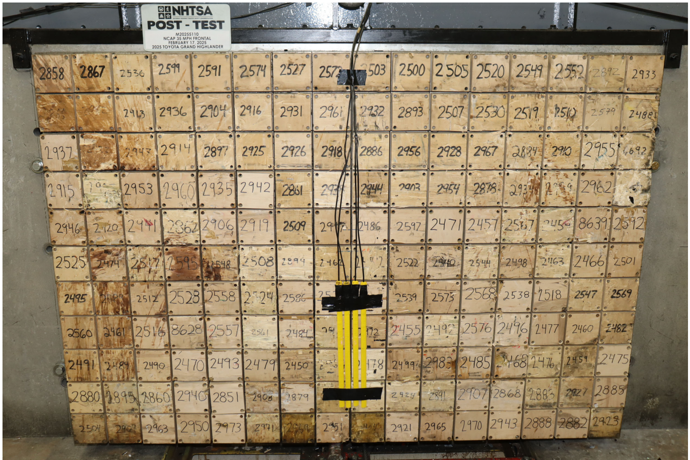
Photo No. 003 - Post-Test Load Cell Wall
