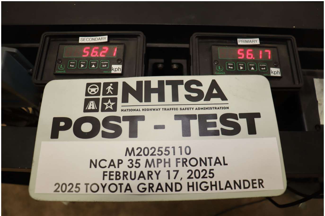
Photo No. 076 - Post-Test Speed Trap Read-Out
