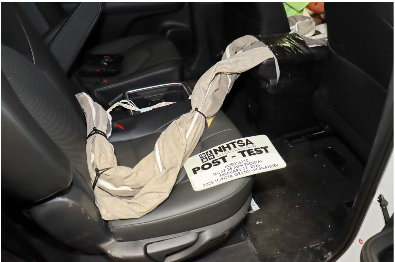
Photo No. 029 - Post-Test Dummy Cable Routing
