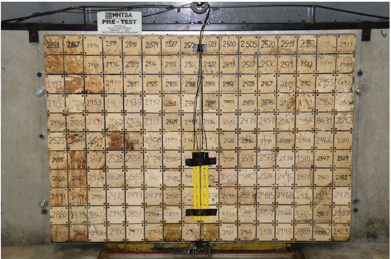
Photo No. 002 - Pre-Test Load Cell Wall
