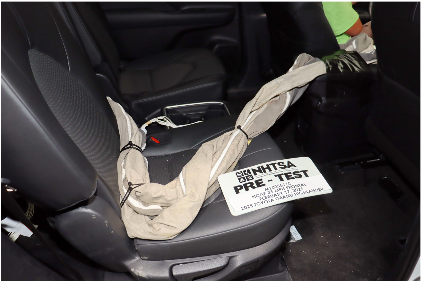
Photo No. 028 - Pre-Test Dummy Cable Routing
