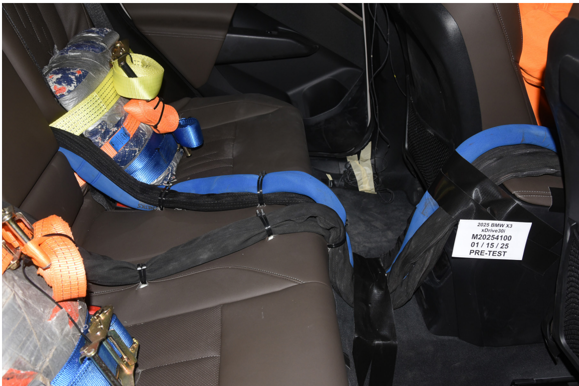
FIGURE 28. Pre-Test Dummy Cable Routing
