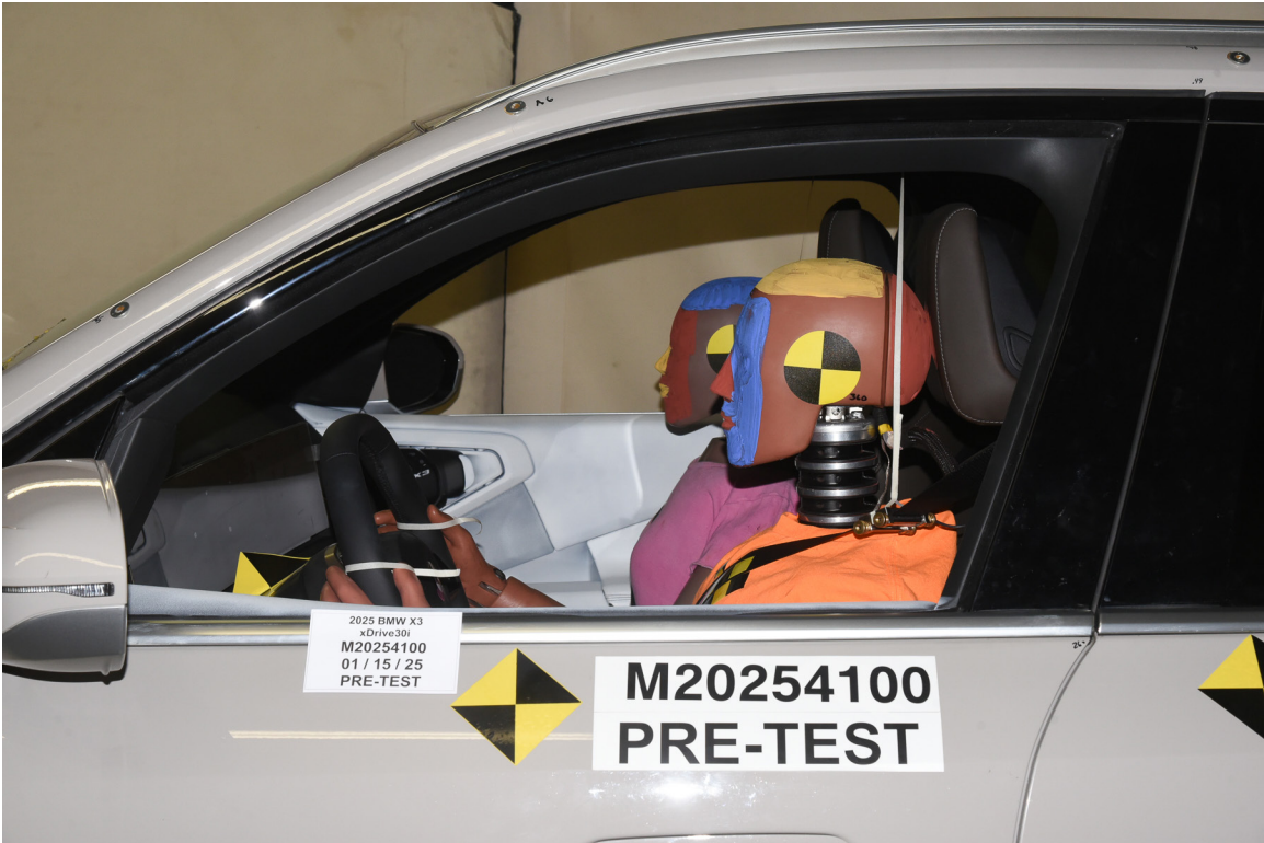
FIGURE 32. Pre-Test Driver Dummy Window View
