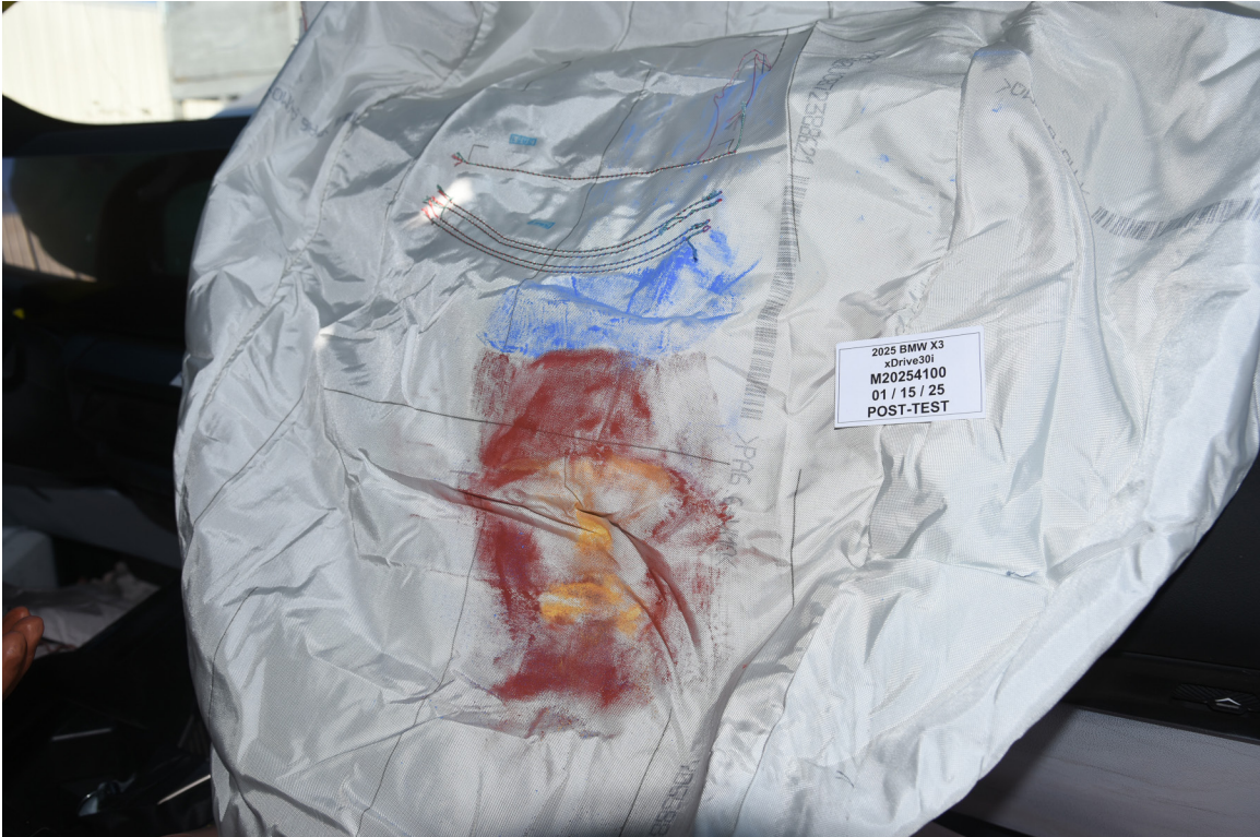
FIGURE 72. Post-Test Passenger Dummy Contact with Air Bag
