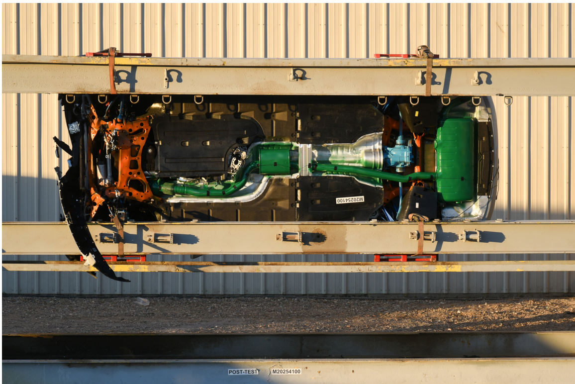
FIGURE 78. Vehicle at 90° on Static Rollover Device
