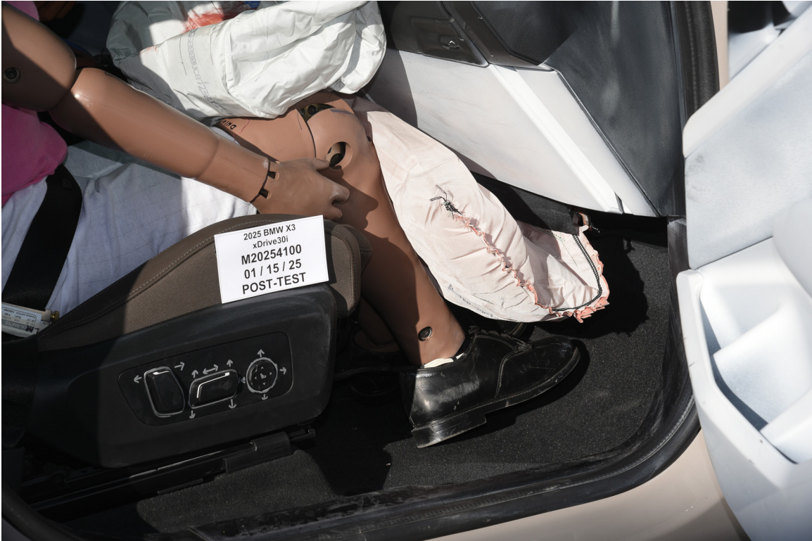
FIGURE 66. Post-Test Passenger Dummy Feet
