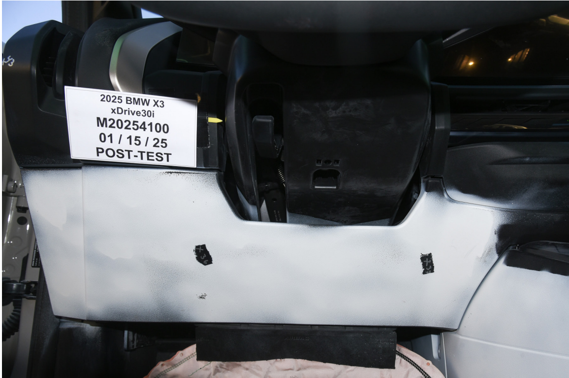
FIGURE 45. Post-Test Driver's Side Knee Bolster
