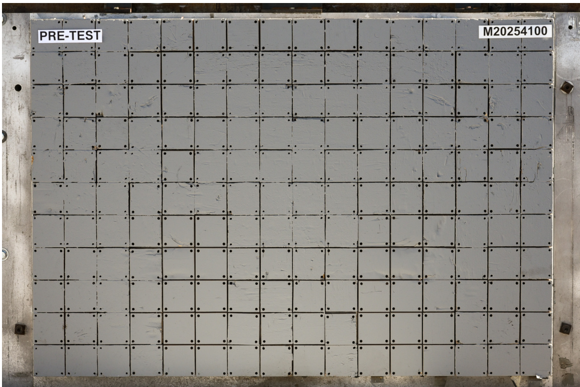
FIGURE 2. Pre-Test Load Cell Wall
