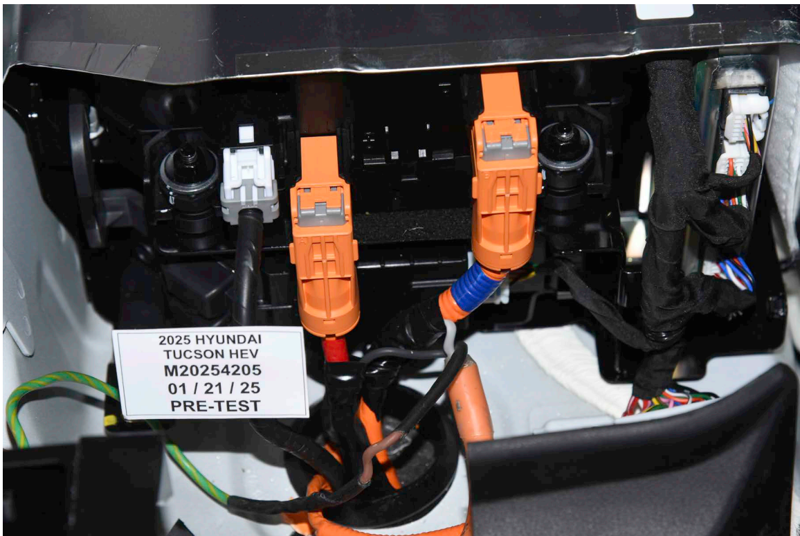
FIGURE 305-06 Manual High Voltage Service Disconnect in Place
