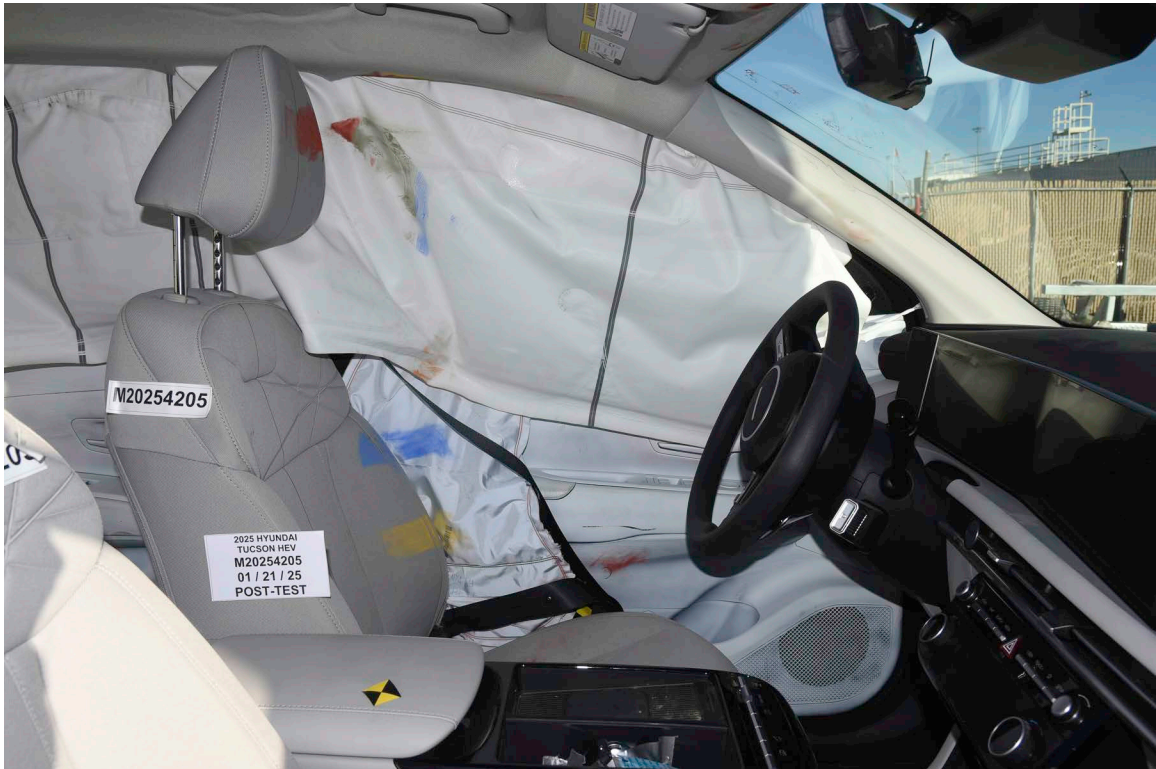
FIGURE 47. Post-Test Driver Inner Door Panel View
