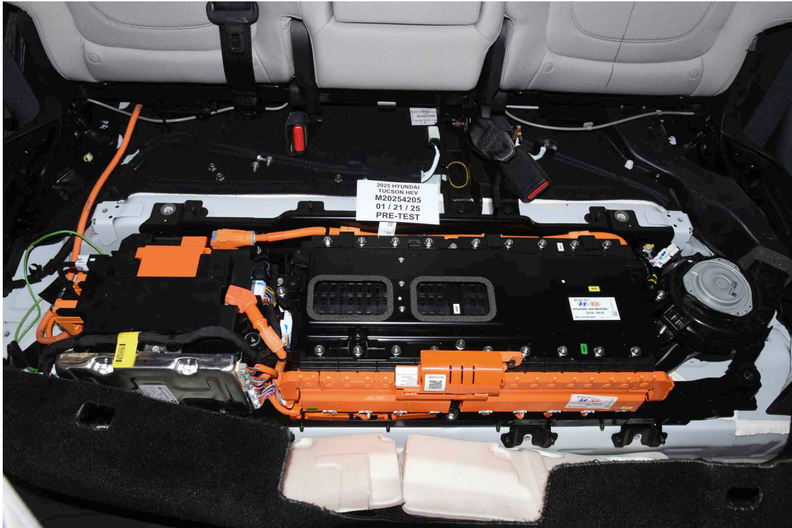
FIGURE 305-09 Pre-Impact View of Propulsion Battery
