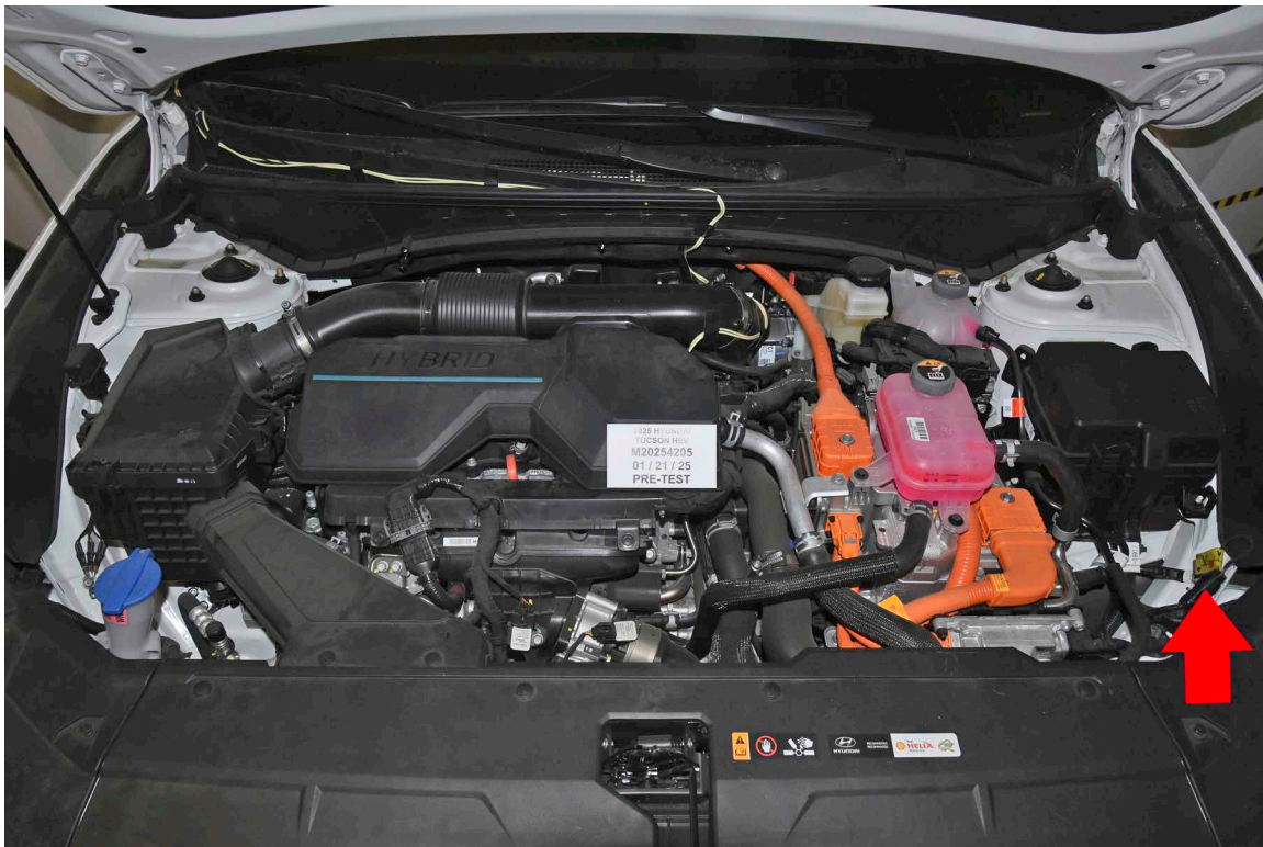
FIGURE 305-04 First Responder Warning Location
