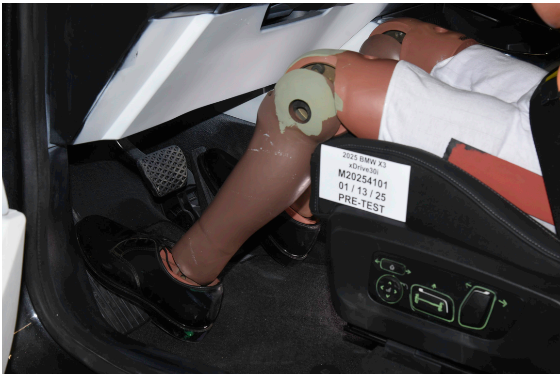
FIGURE 32. Pre-Test Placement of Dummy's Feet
