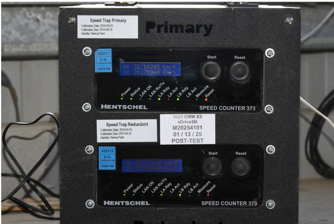
FIGURE 64. Post-Test Primary and Redundant Speed Trap Read-Out
