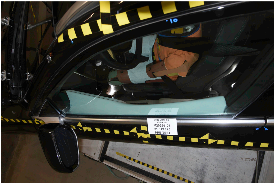
FIGURE 40. Pre-Test Dummy and Door Clearance View
