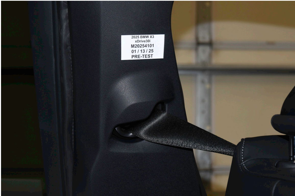
FIGURE 33. Pre-Test View of Belt Anchorage for Dummy
