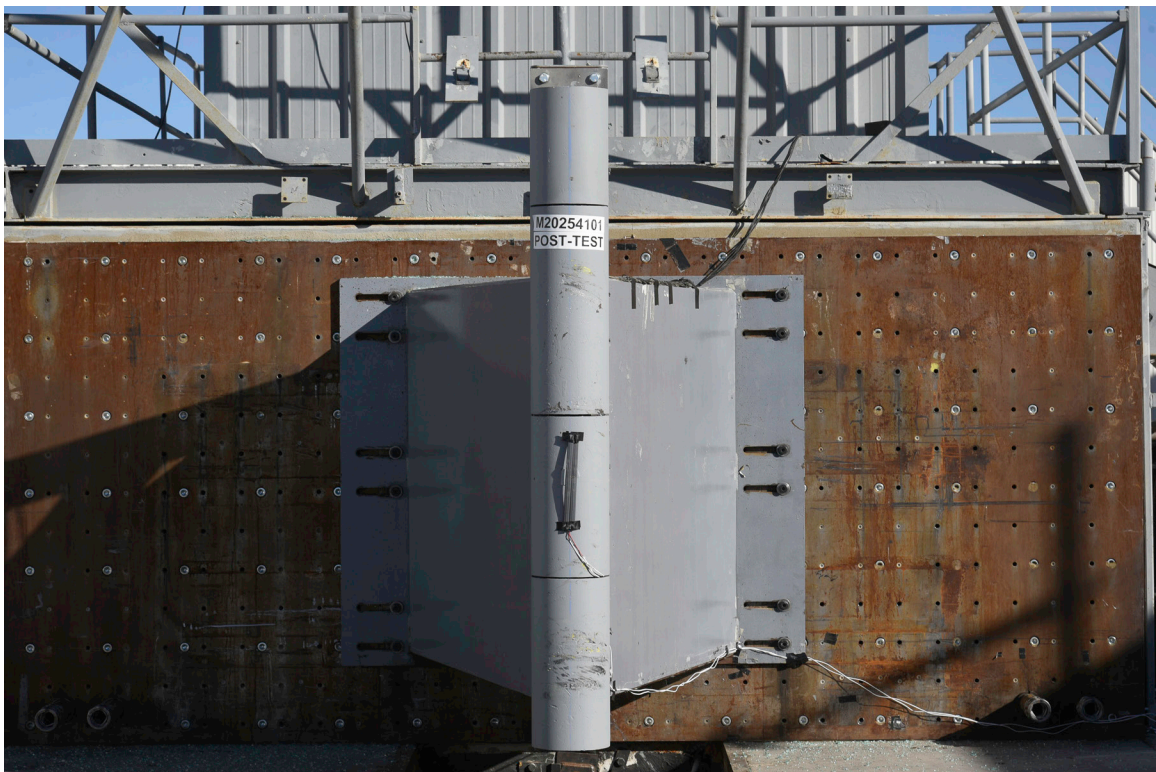
FIGURE 60. Post-Test Pole Barrier Front View
