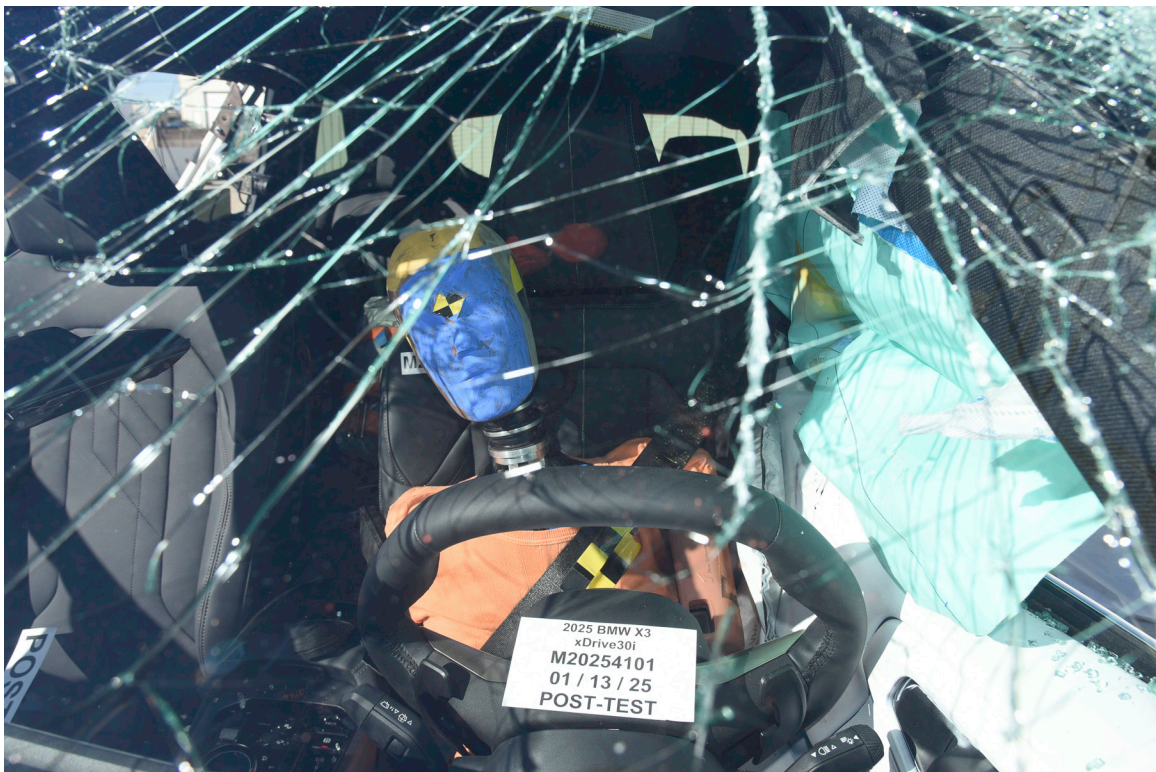
FIGURE 22. Post-Test Front Close-Up View of Dummy
