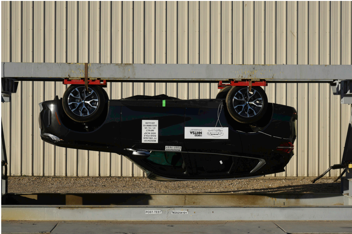
FIGURE 67. FMVSS No. 301 Static Rollover 180 Degrees
