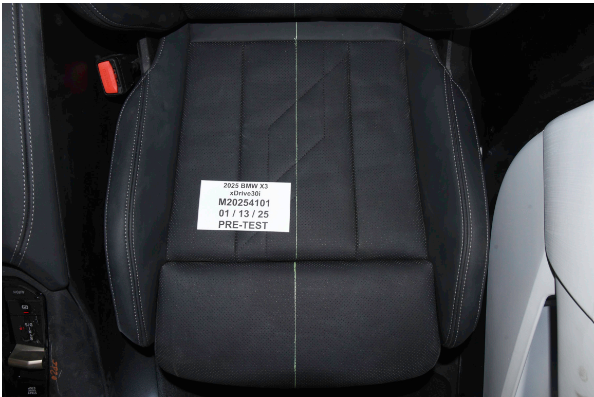
FIGURE 28. Pre-Test Front View of Seat Pan Prior to Dummy Positioning
