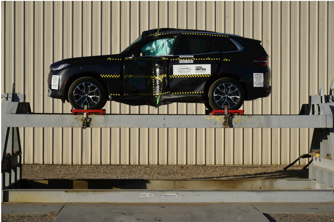
FIGURE 69. FMVSS No. 301 Static Rollover 360 Degrees
