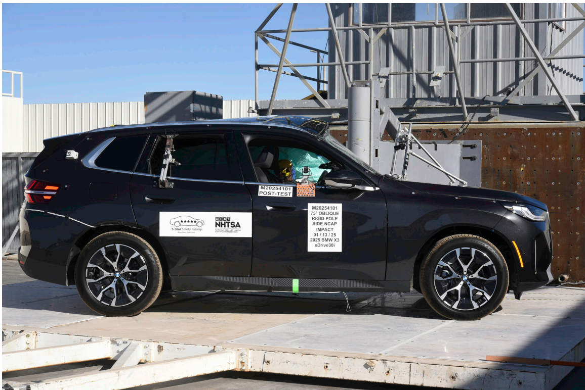
FIGURE 14. Post-Test Right Side View of Test Vehicle
