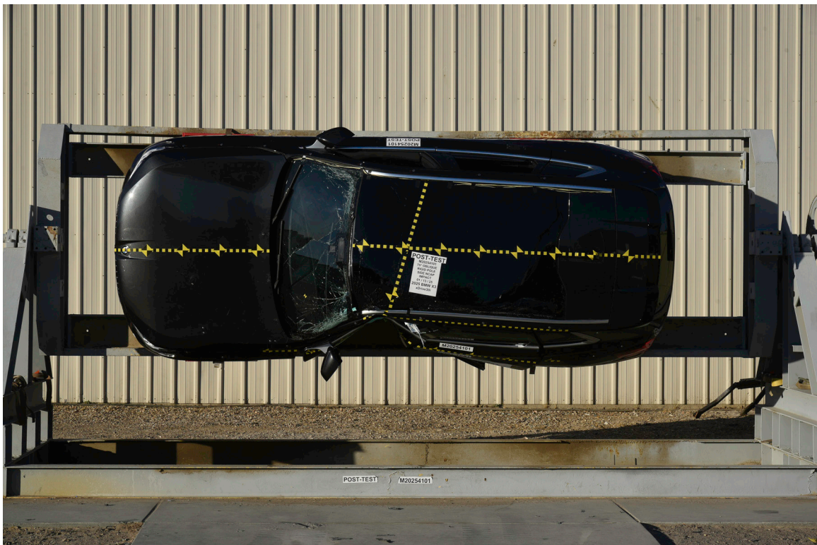
FIGURE 68. FMVSS No. 301 Static Rollover 270 Degrees
