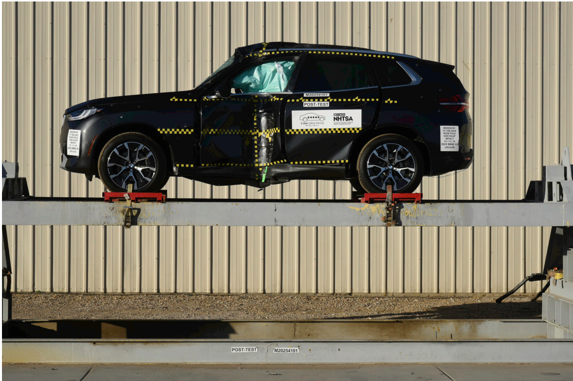
FIGURE 65. FMVSS No. 301 Static Rollover 0 Degrees
