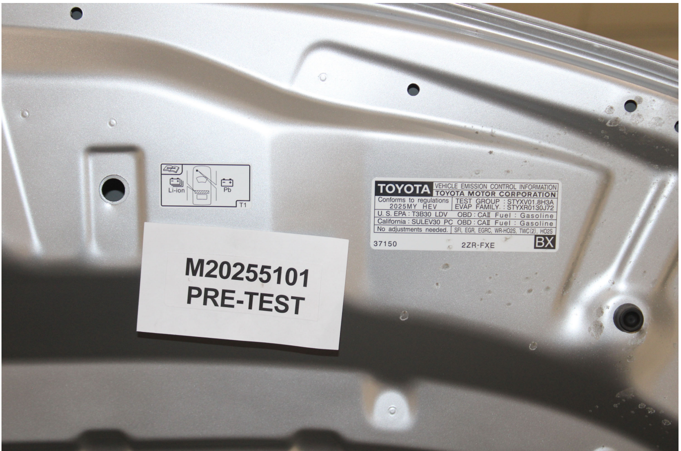
Photo No. 305-03 - First Responder Warning Label
