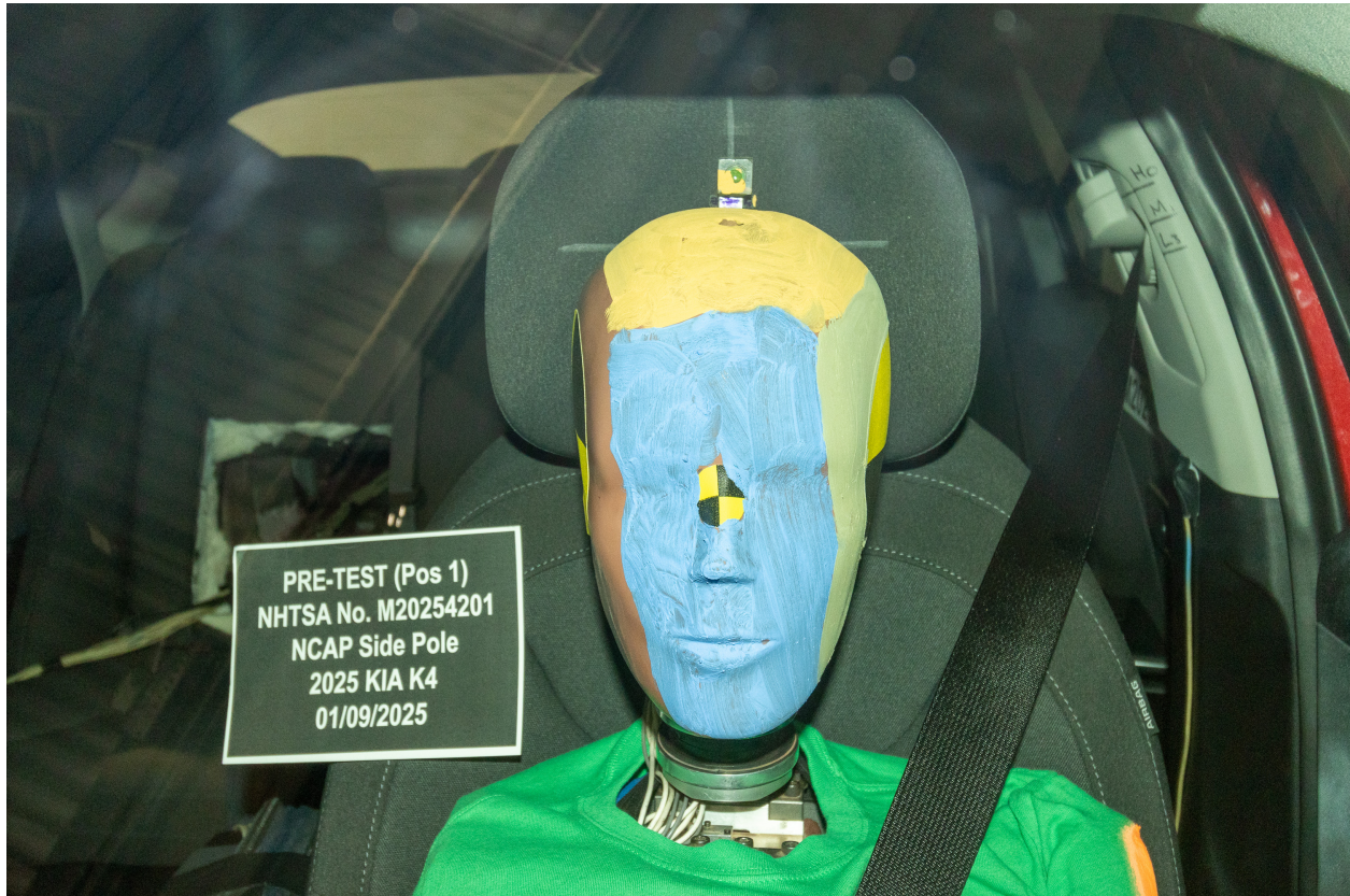
Figure A-27: Pre-Test Frontal Close-Up View of Dummy Head / Shoulders in Relation to Head Restraint
