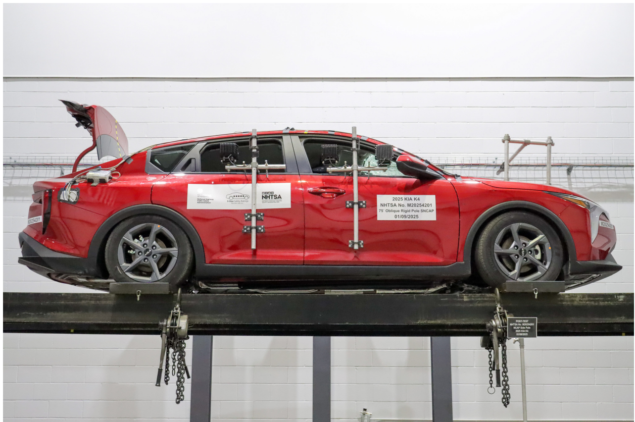
Figure A-65: FMVSS No. 301 Static Rollover 0 Degrees
