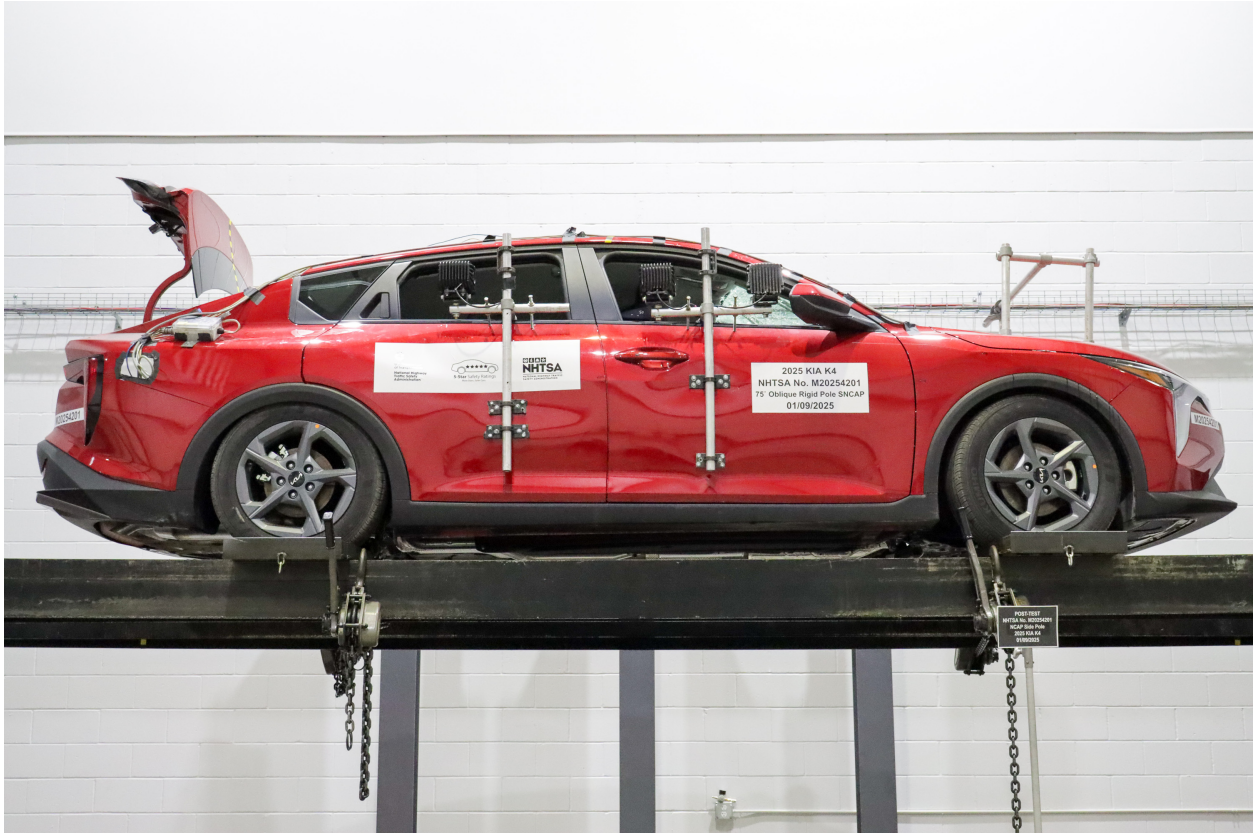
Figure A-69: FMVSS No. 301 Static Rollover 360 Degrees
