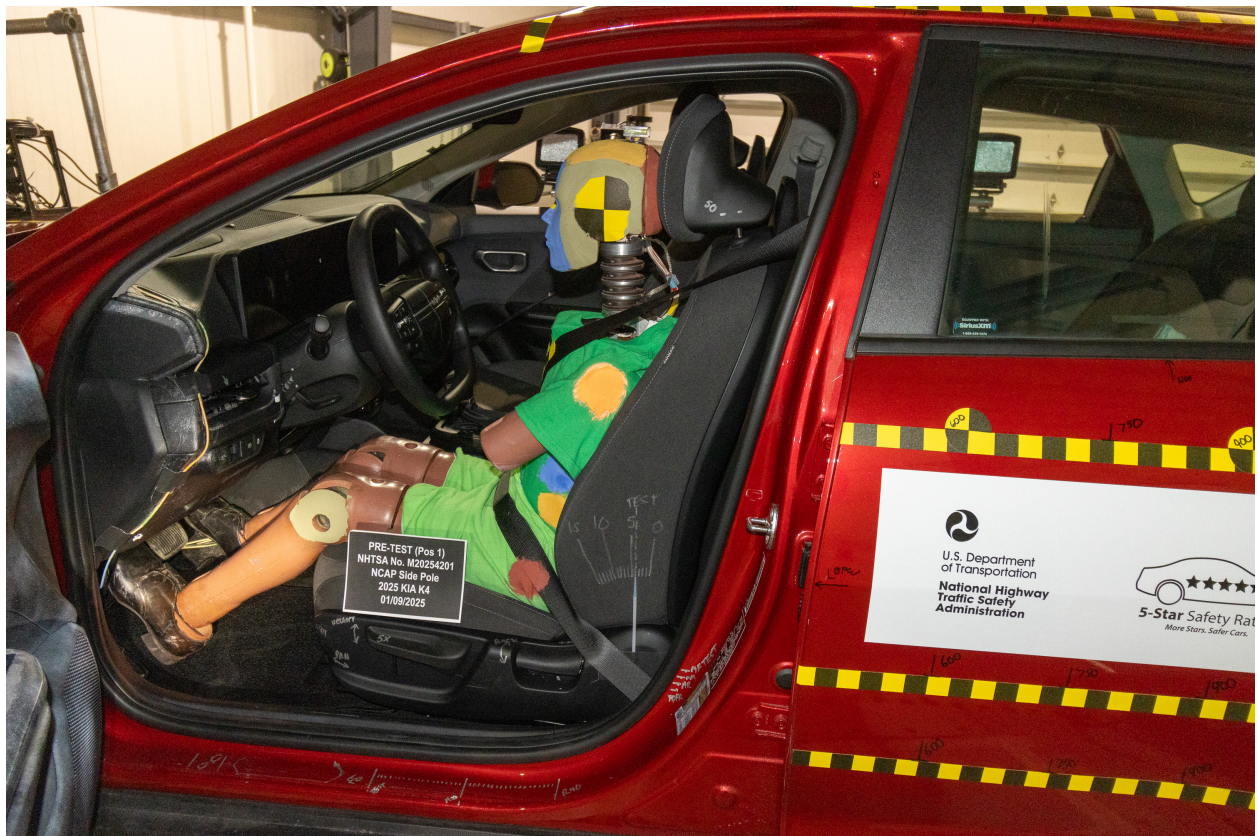
Figure A-23: Pre-Test Left Side View of Dummy Showing Belt and Chalking
