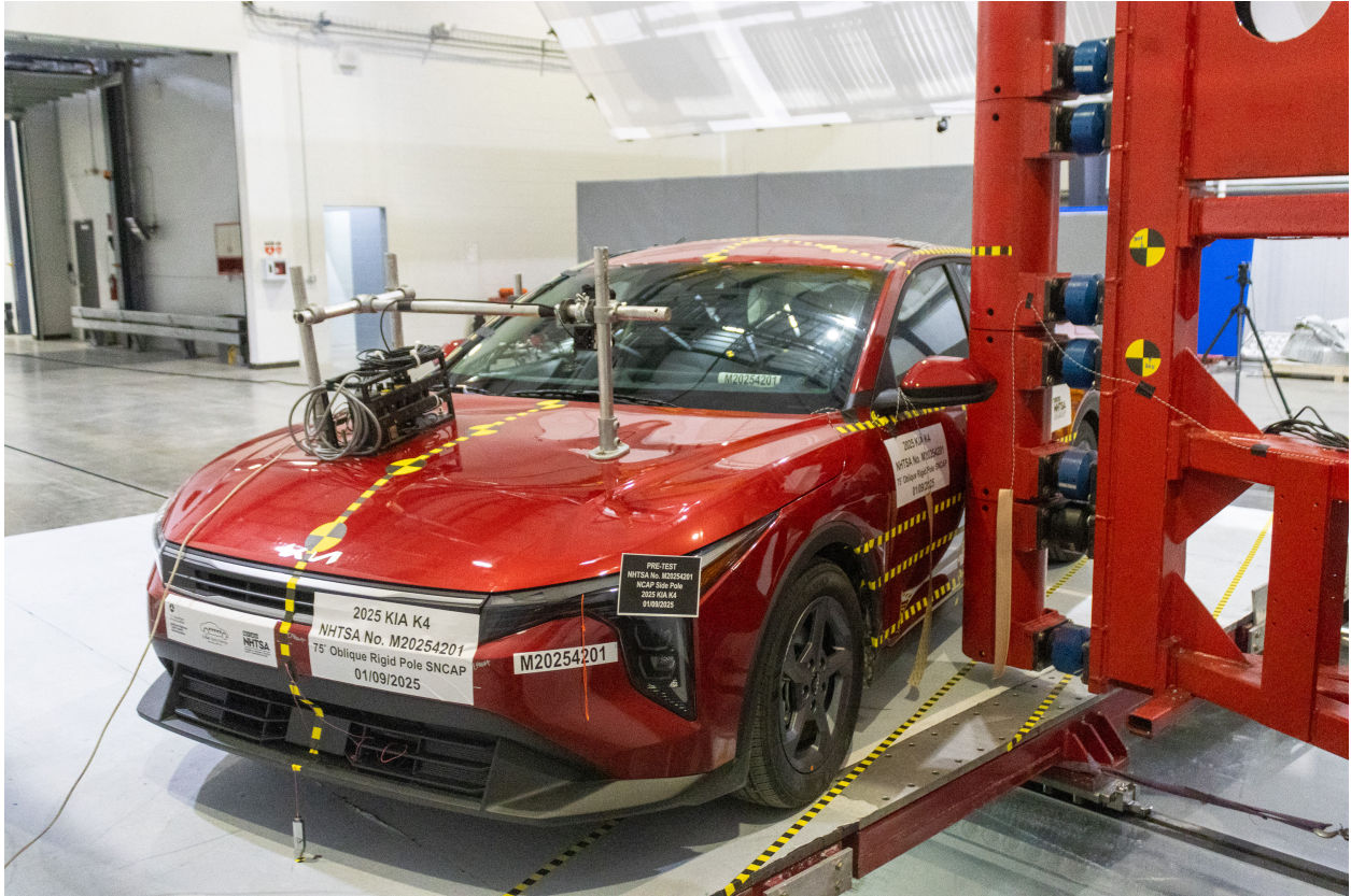
Figure A-17: Pre-Test Left Side View of Pole Positioned Against Side of Vehicle
