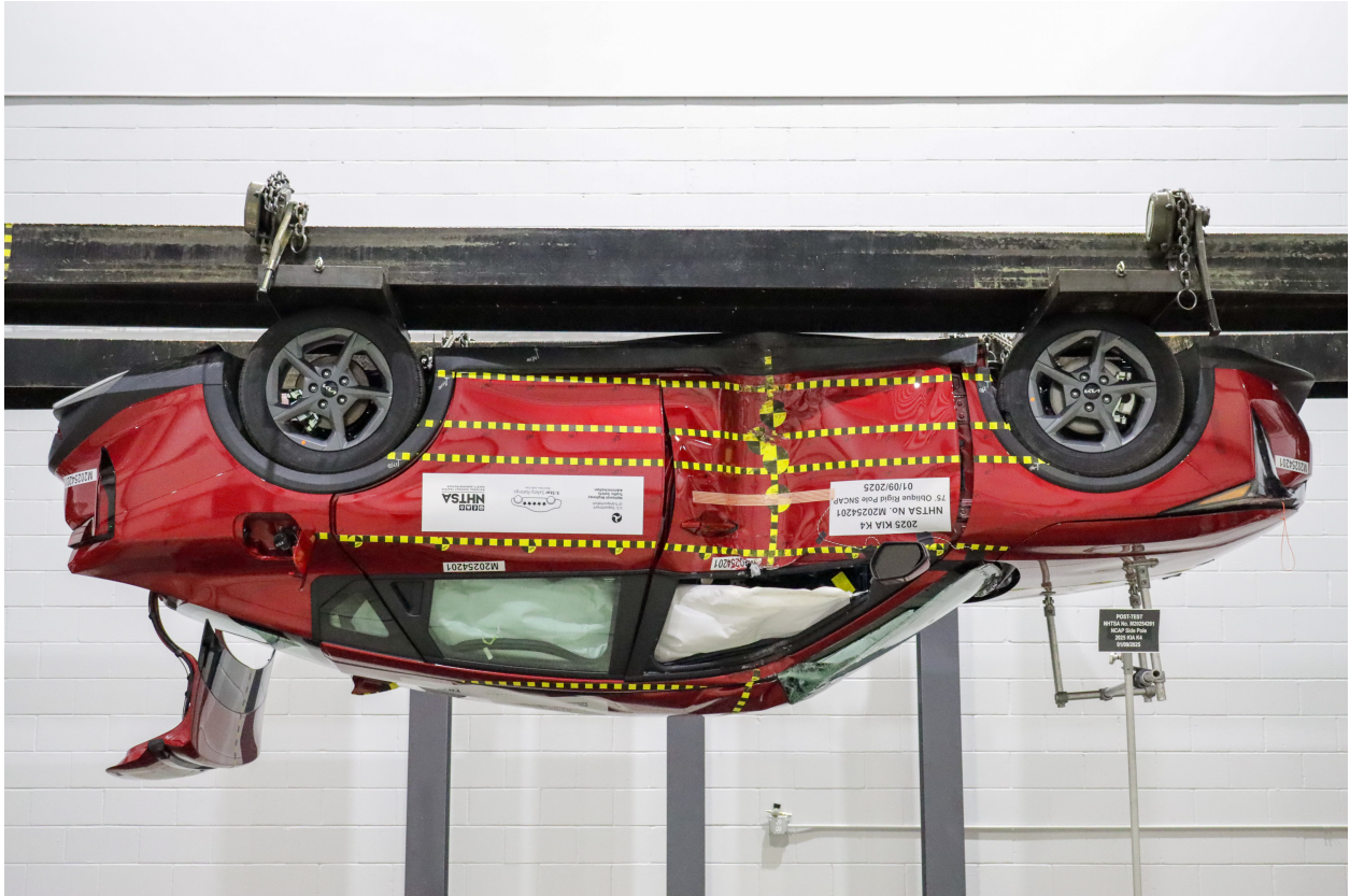
Figure A-67: FMVSS No. 301 Static Rollover 180 Degrees
