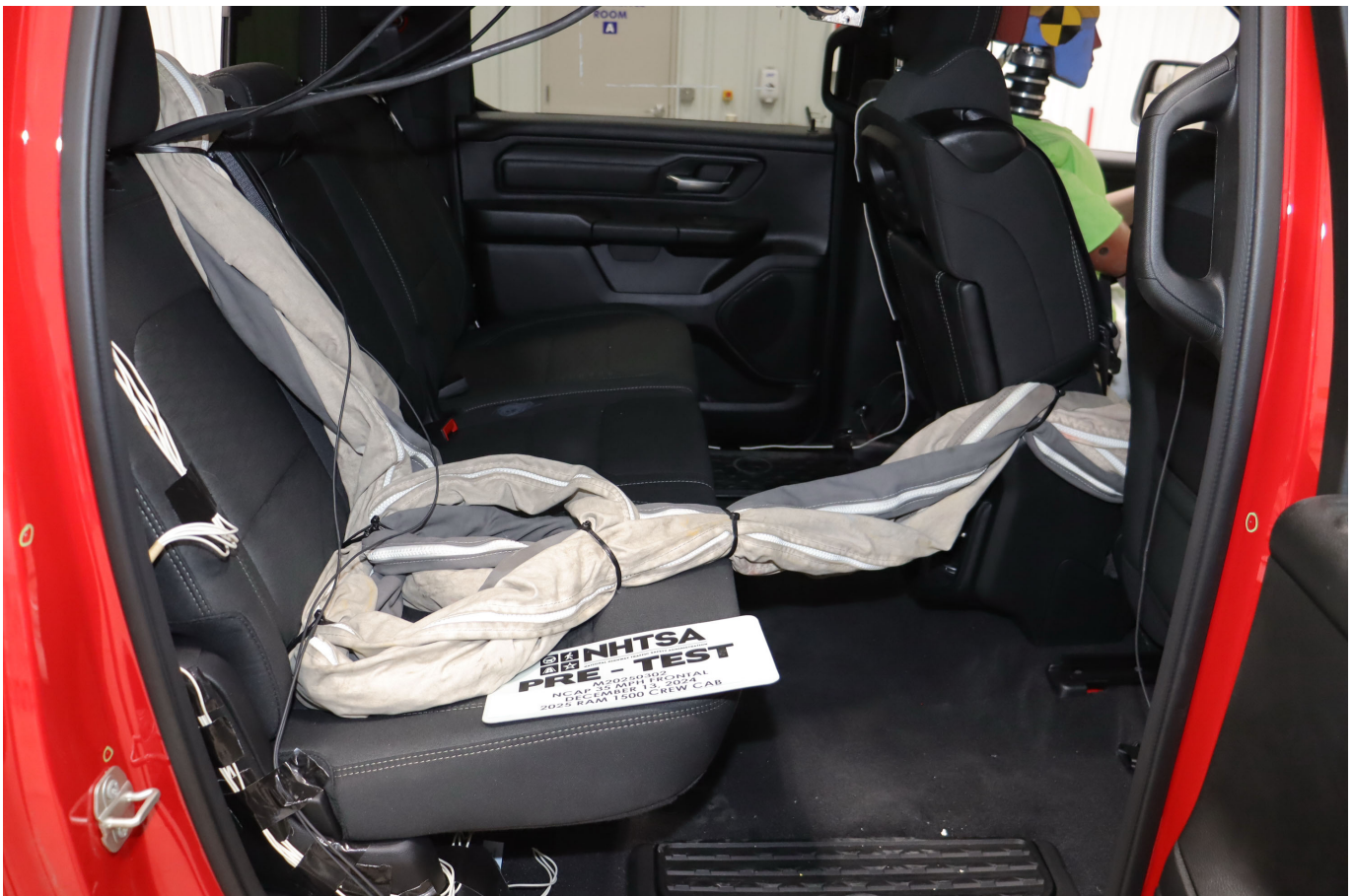
Photo No. 028 - Pre-Test Dummy Cable Routing
