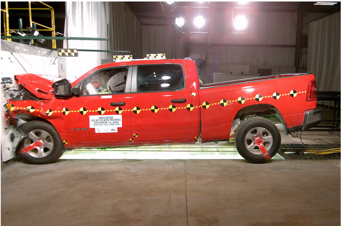
Photo No. 082 - 2025 RAM 1500 Crew Cab 4x4 Truck Frontal Impact Event
