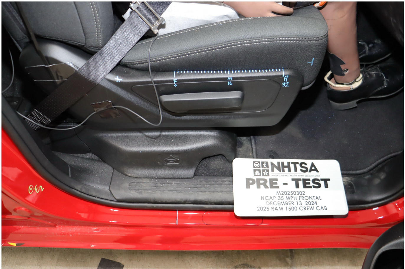
Photo No. 059 - Pre-Test Passenger's Seat Fore-Aft Markings
