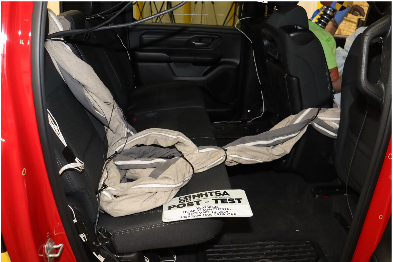
Photo No. 029 - Post-Test Dummy Cable Routing
