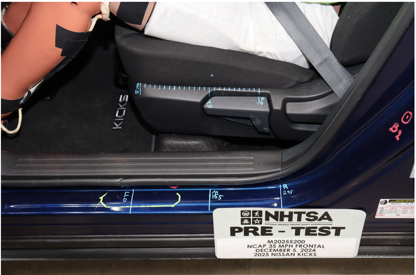
Photo No. 036 - Pre-Test Driver's Seat Fore-Aft Markings
