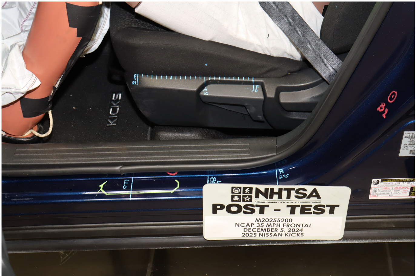
Photo No. 037 - Post-Test Driver's Seat Fore-Aft Markings
