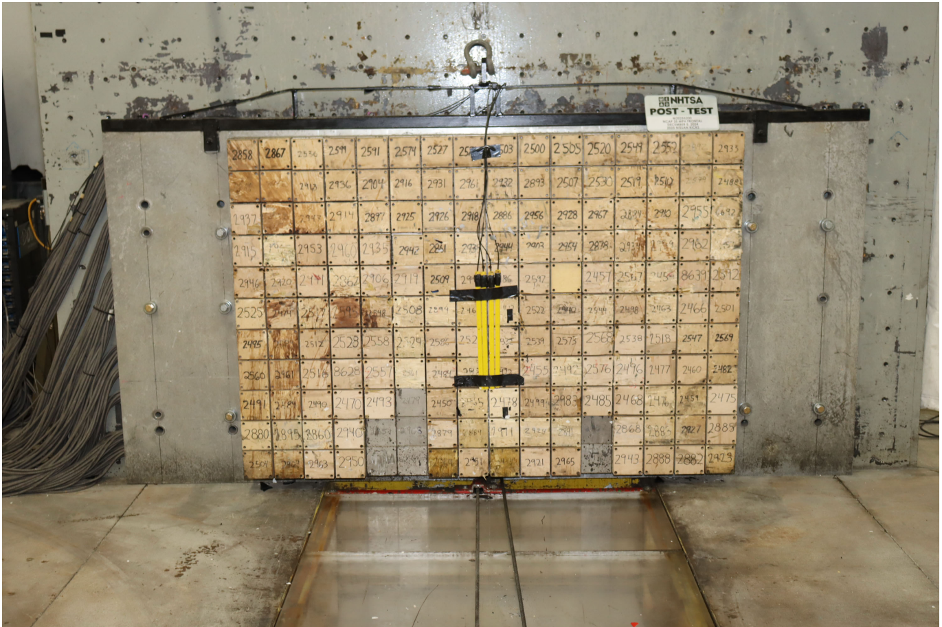
Photo No. 003 - Post-Test Load Cell Wall
