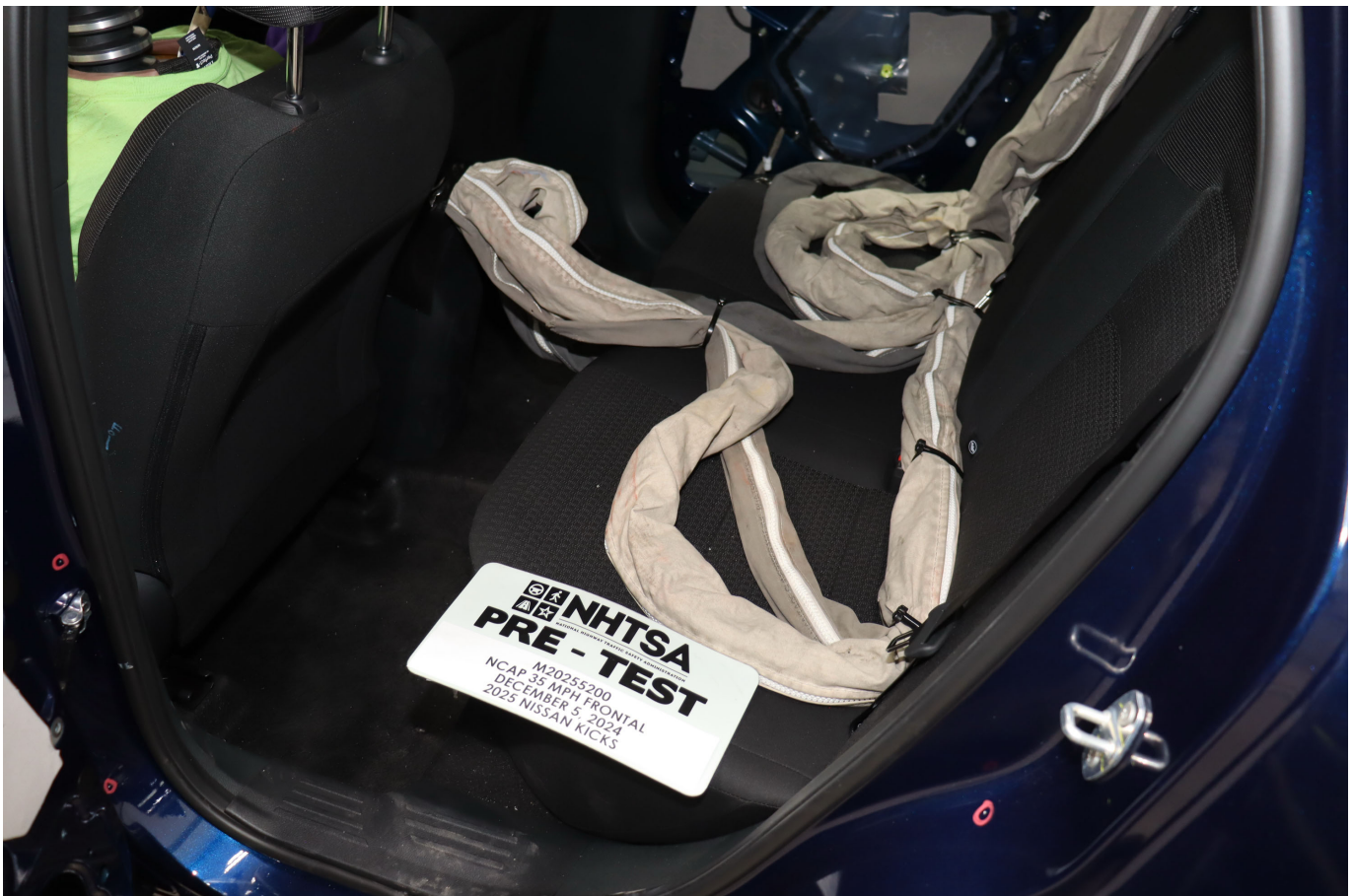
Photo No. 028 - Pre-Test Dummy Cable Routing
