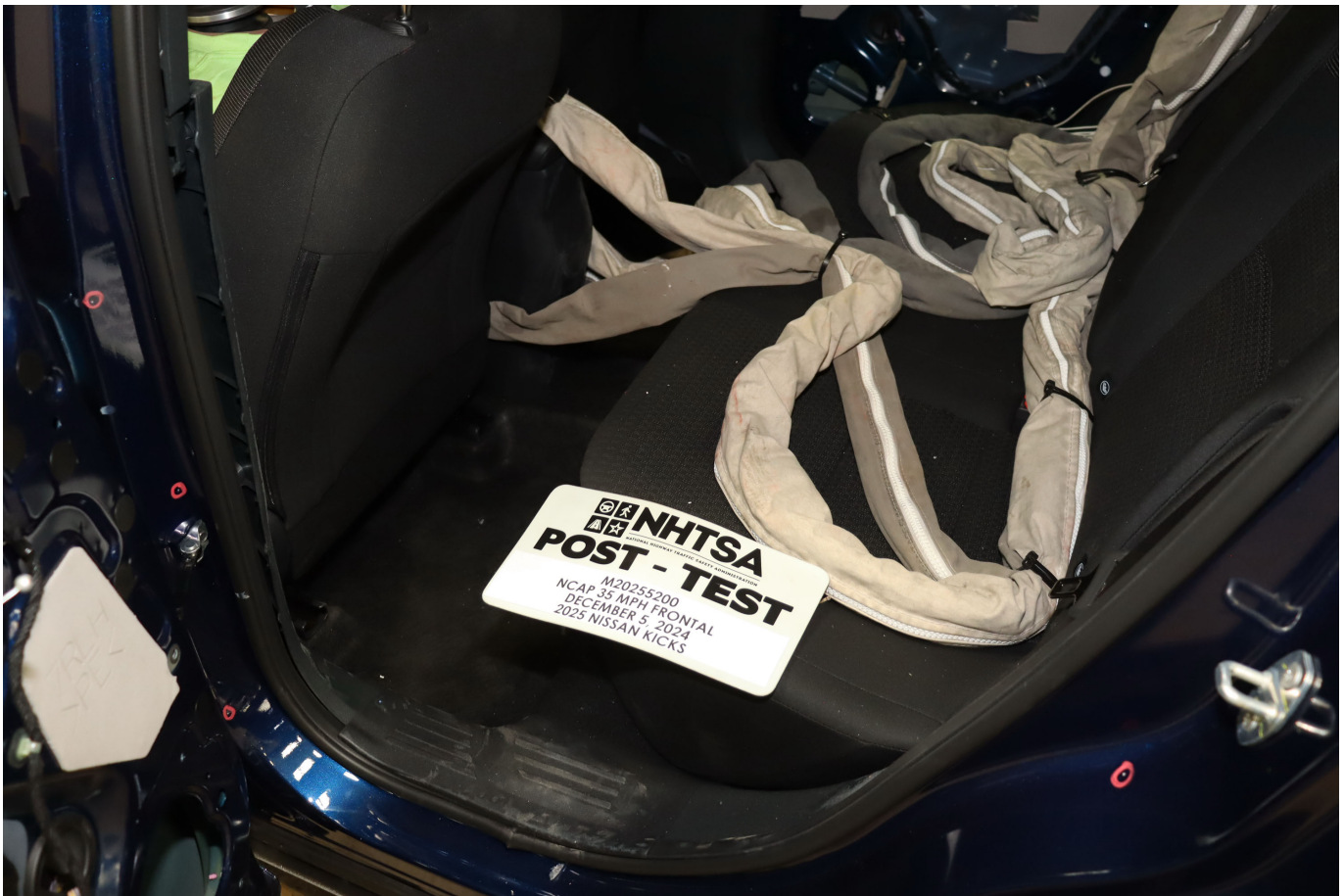
Photo No. 029 - Post-Test Dummy Cable Routing
