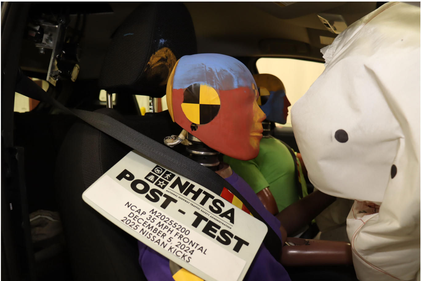
Photo No. 071 - Post-Test Passenger Dummy Face
