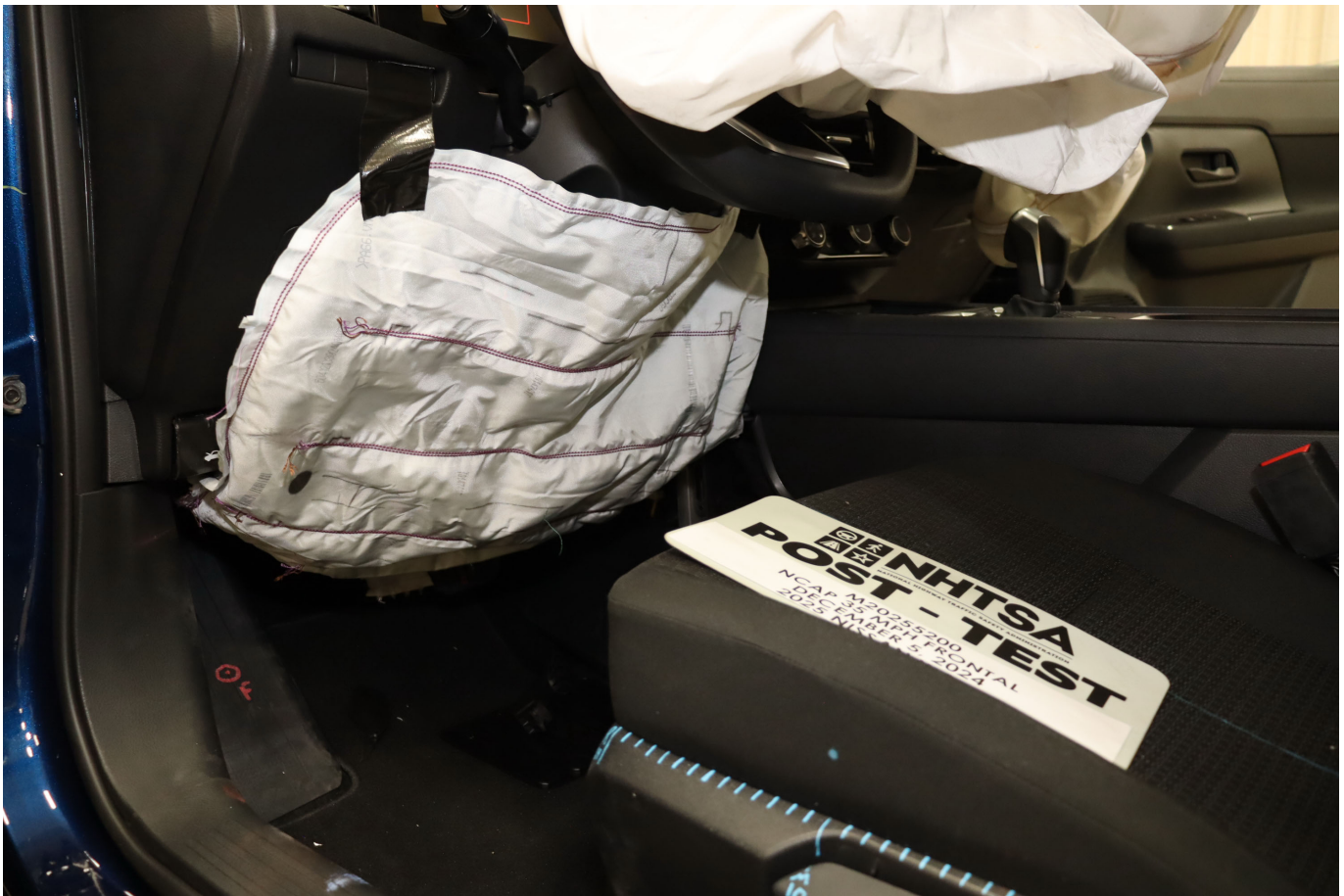
Photo No. 045 - Post-Test Driver's Side Knee Bolster
