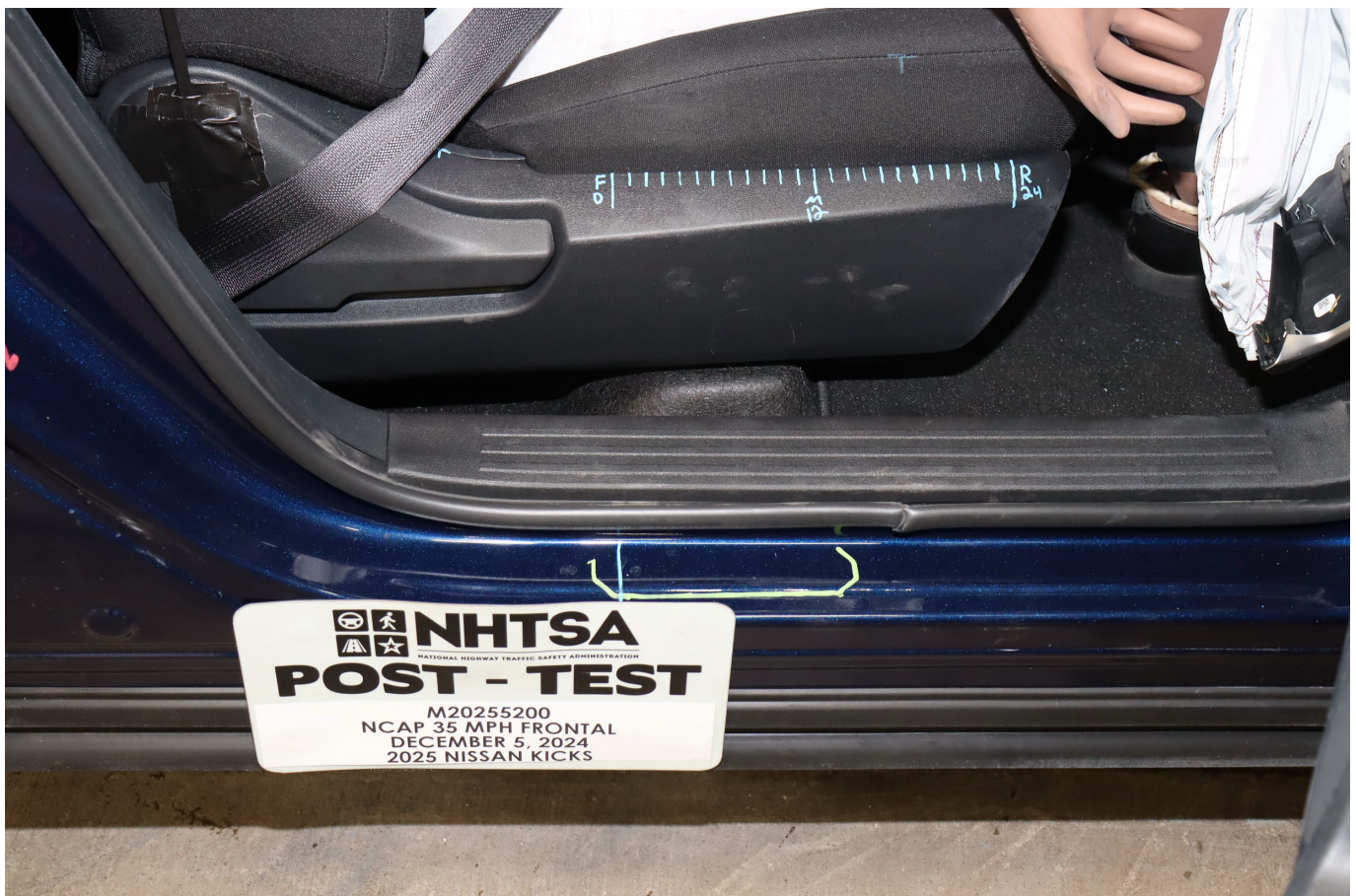
Photo No. 060 - Post-Test Passenger's Seat Fore-Aft Markings
