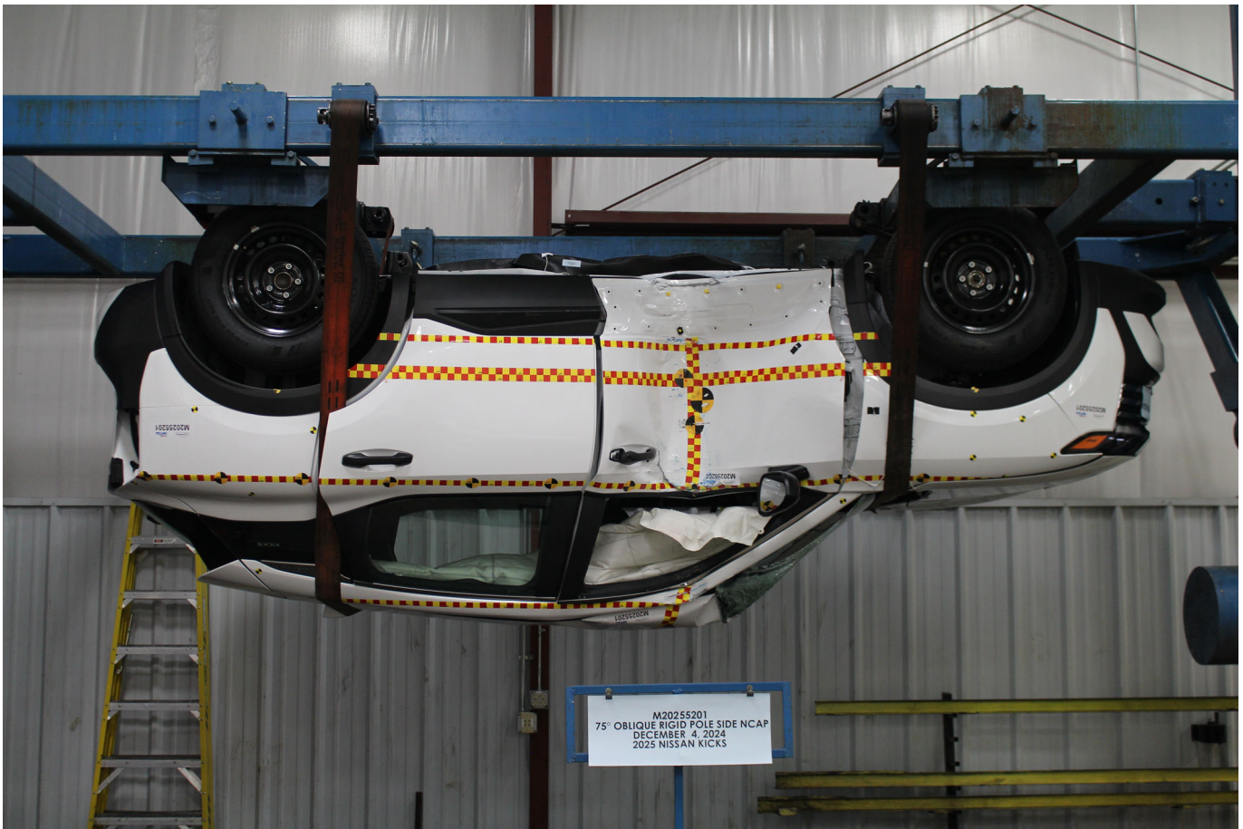
Photo No. 067 - FMVSS Photo No. 301 Static Rollover 180 Degrees
