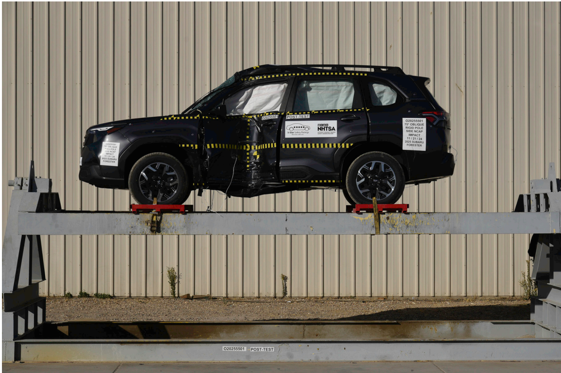
FIGURE 65. FMVSS No. 301 Static Rollover 0 Degrees
