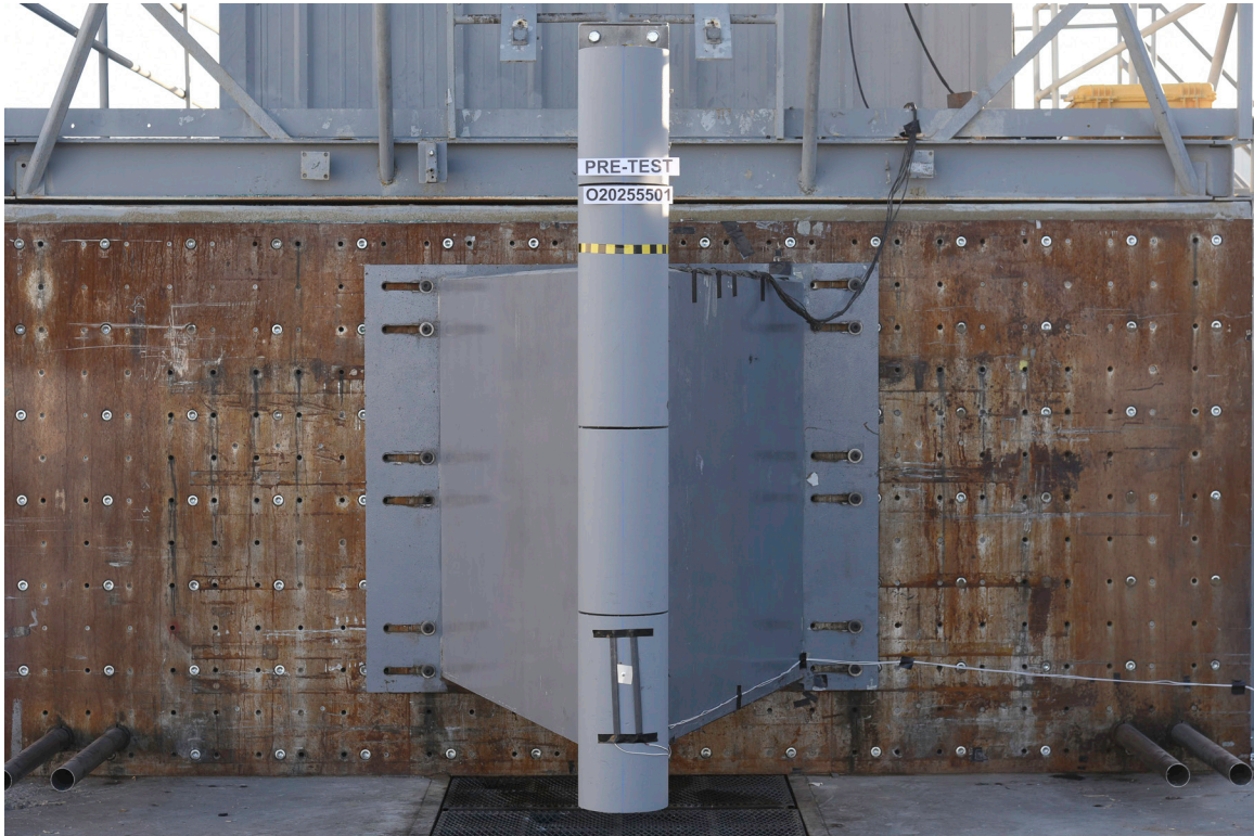
FIGURE 59. Pre-Test Pole Barrier Front View
