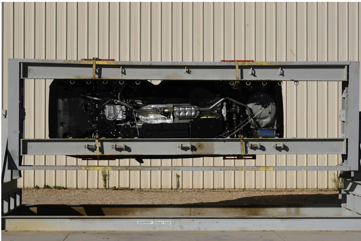
FIGURE 66. FMVSS No. 301 Static Rollover 90 Degrees
