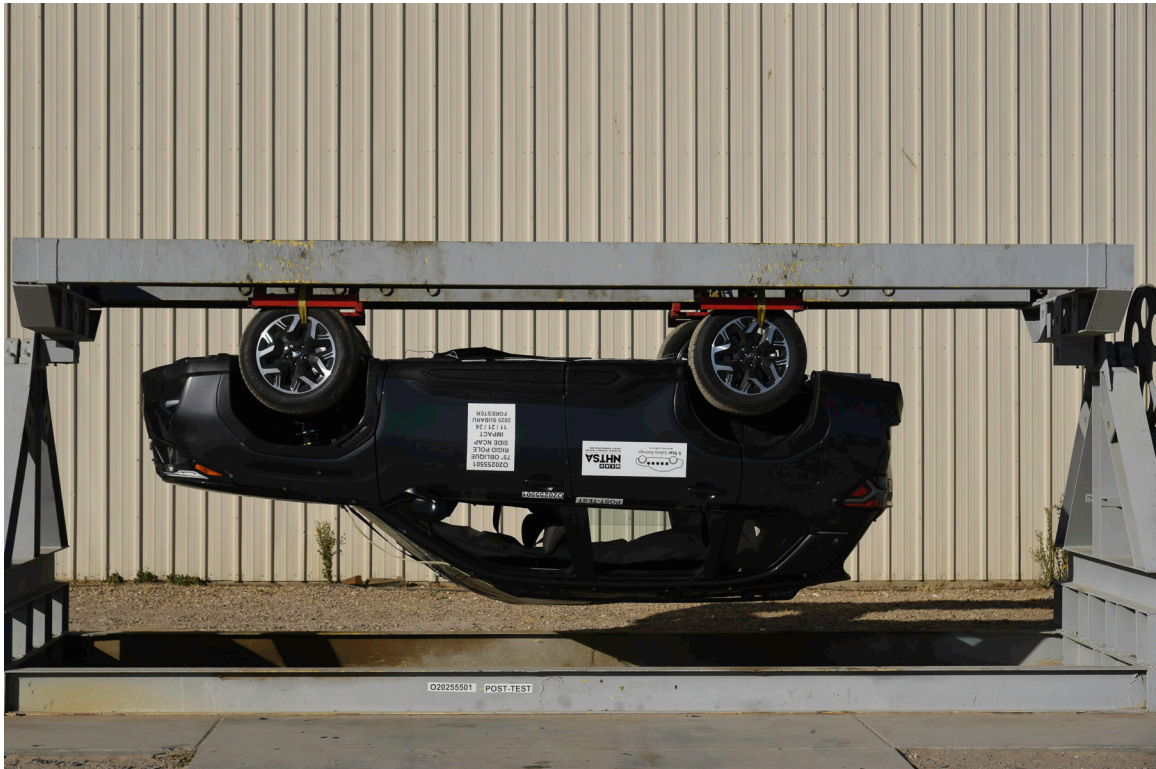
FIGURE 67. FMVSS No. 301 Static Rollover 180 Degrees
