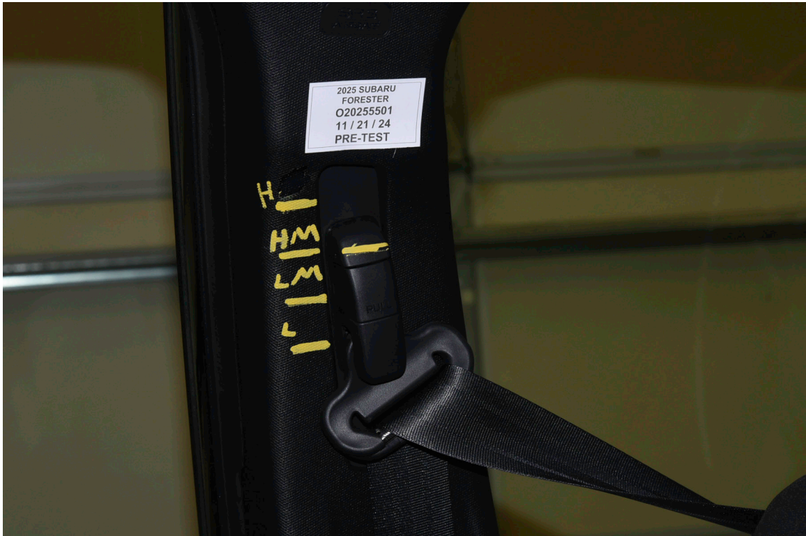
FIGURE 33. Pre-Test View of Belt Anchorage for Dummy
