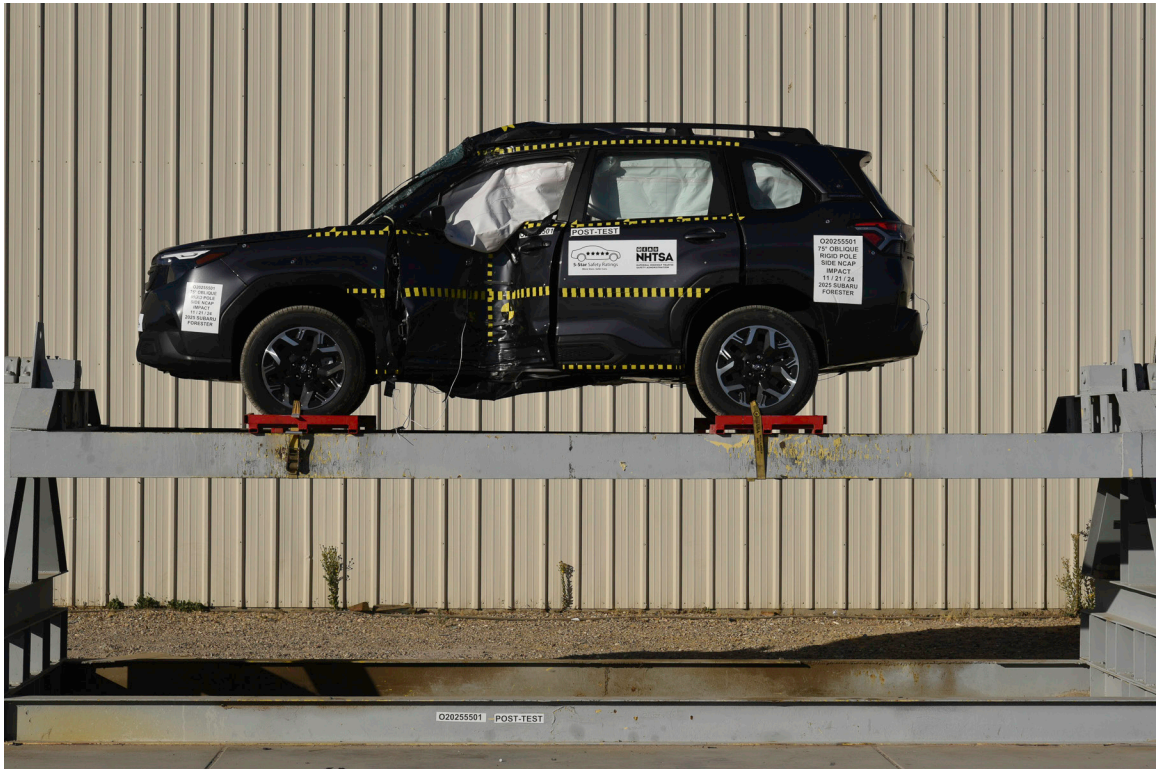
FIGURE 69. FMVSS No. 301 Static Rollover 360 Degrees
