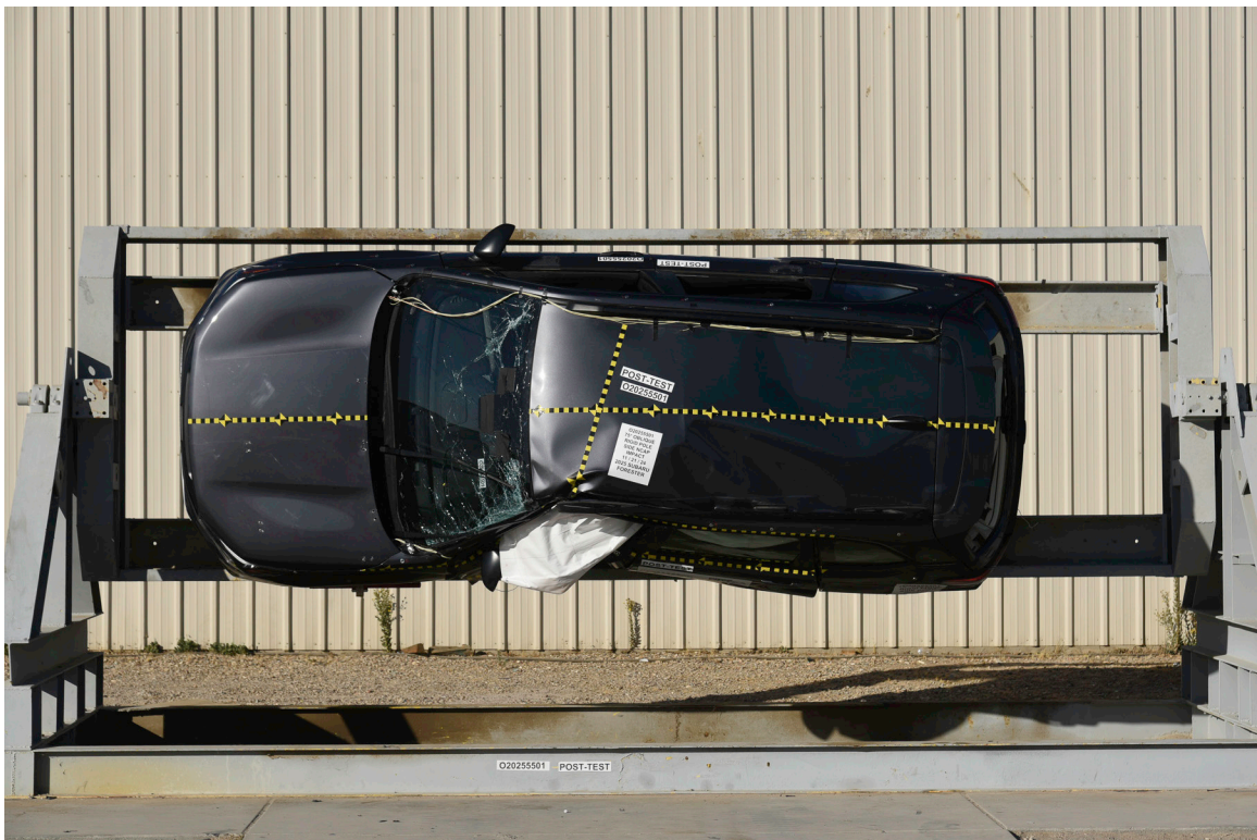
FIGURE 68. FMVSS No. 301 Static Rollover 270 Degrees
