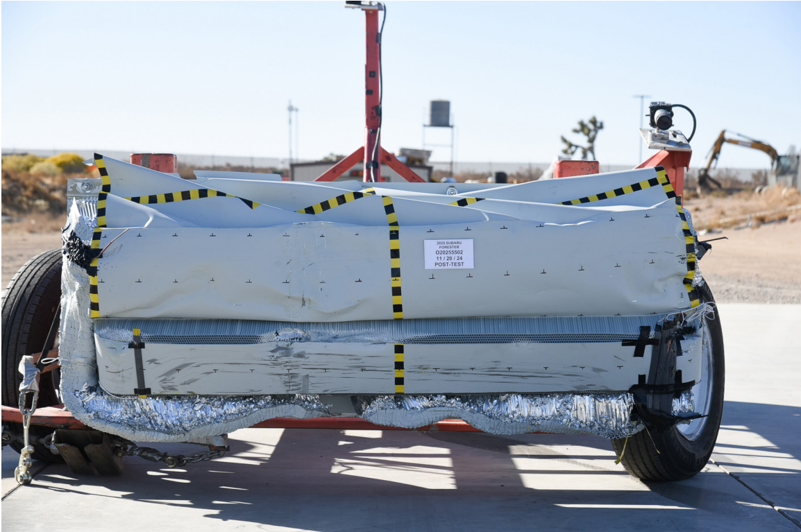
FIGURE 85. Post-Test Front View of MDB Impactor Face
