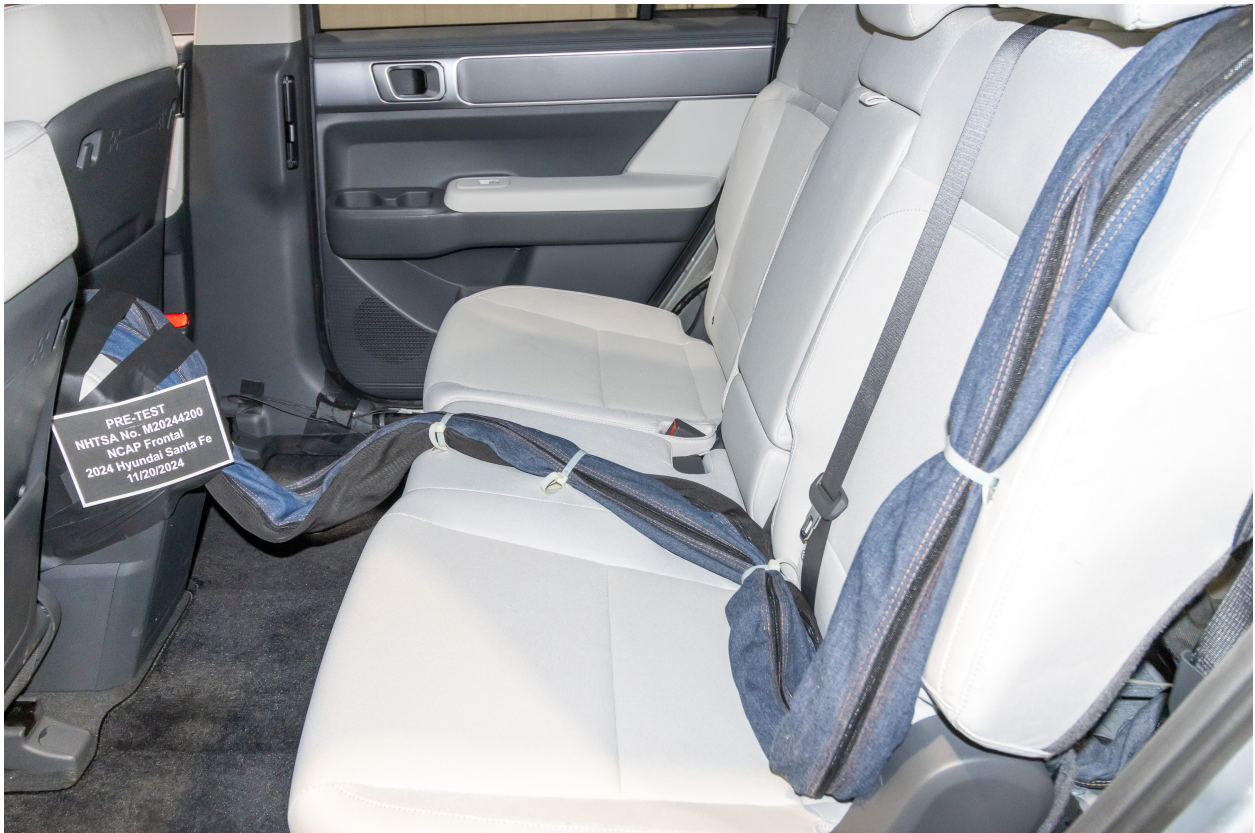
Figure A-28: Pre-Test Dummy Cable Routing
