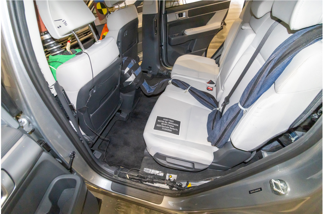
Figure A-29: Post-Test Dummy Cable Routing
