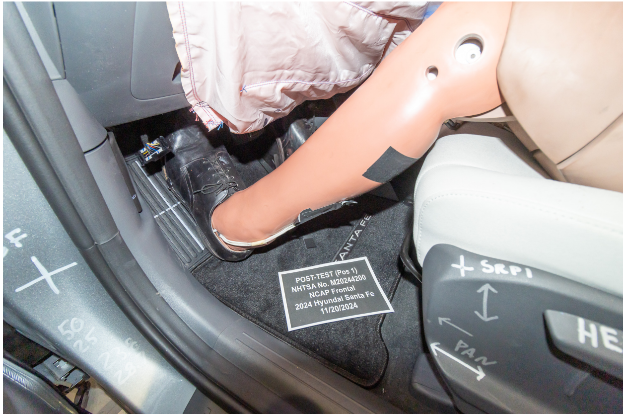
Figure A-43: Post-Test Driver Dummy Feet
