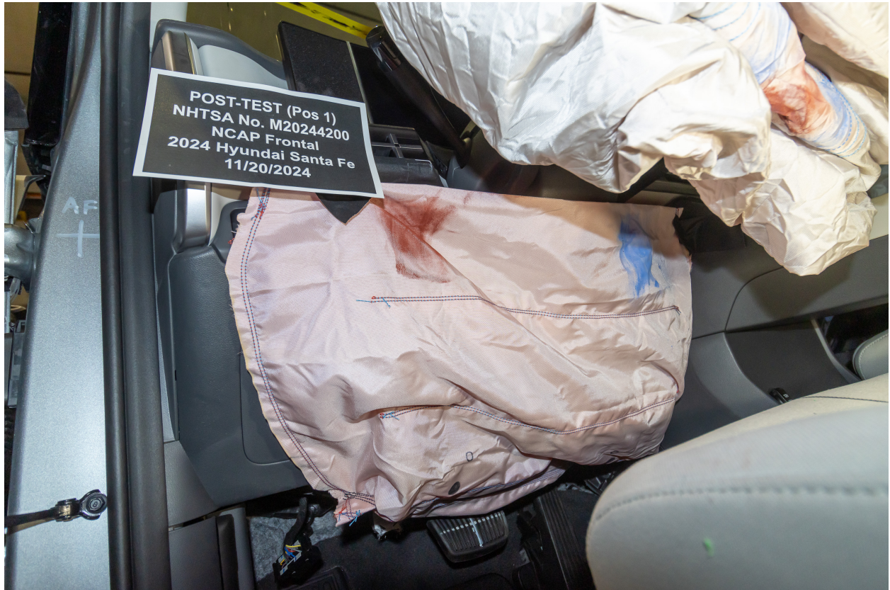
Figure A-45: Post-Test Driver's Side Knee Bolster
