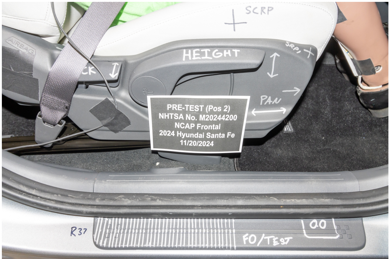
Figure A-59: Pre-Test Passenger's Seat Fore-Aft Markings
