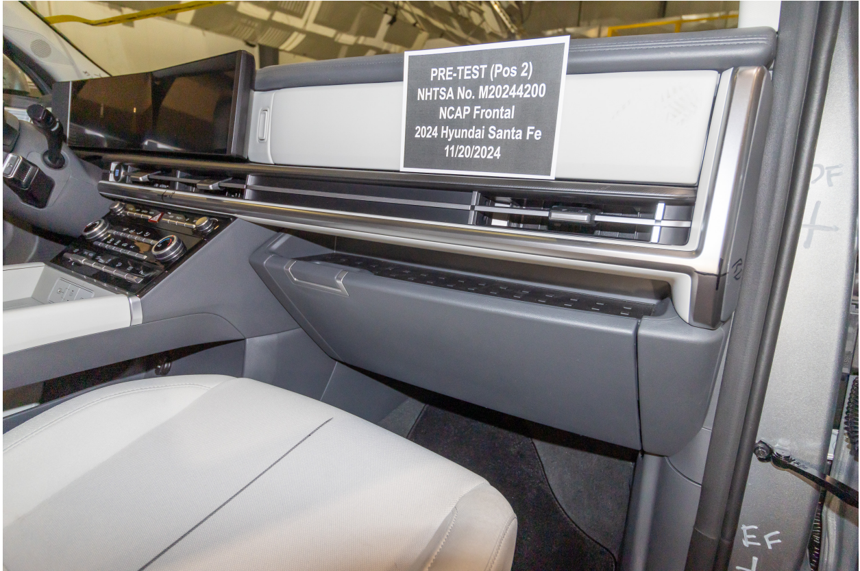
Figure A-67: Pre-Test Passenger's Side Knee Bolster
