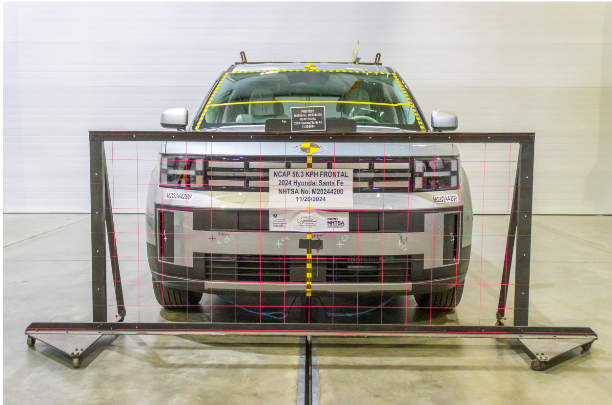
Figure A-1: Load Cell Location
