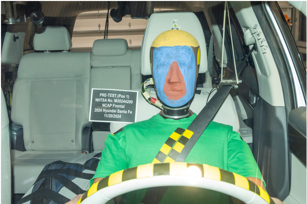
Figure A-30: Pre-Test Driver Dummy Front View
