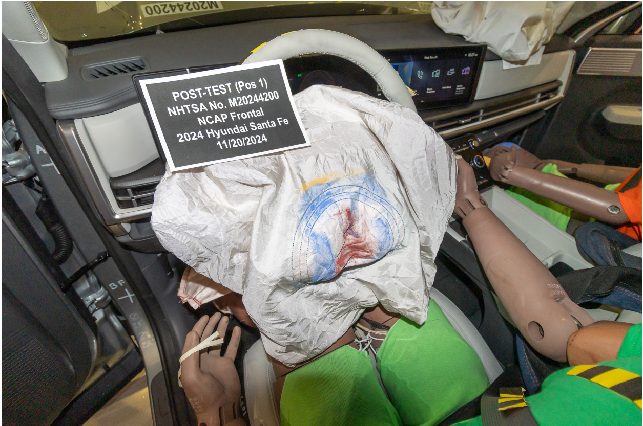
Figure A-49: Post-Test Driver Dummy Contact With Airbag
