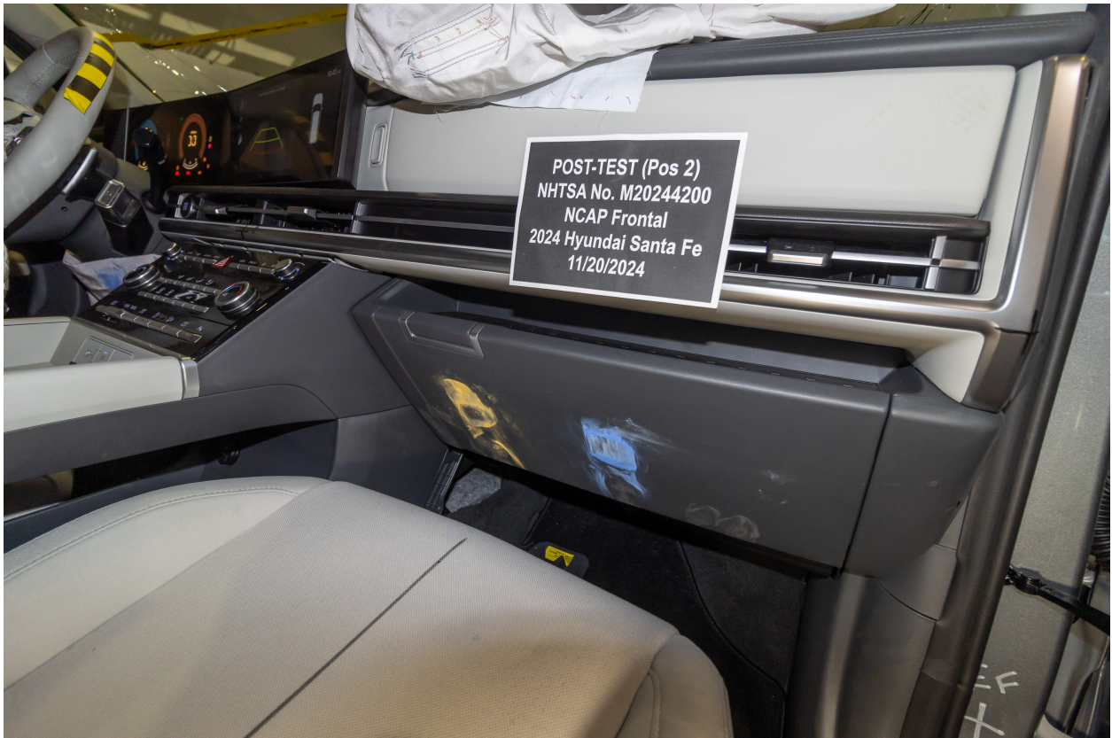
Figure A-68: Post-Test Passenger's Side Knee Bolster
