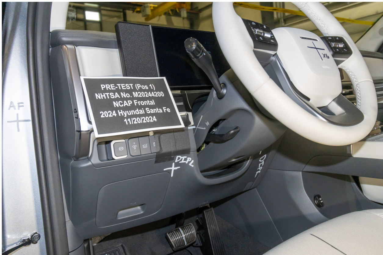
Figure A-44: Pre-Test Driver's Side Knee Bolster
