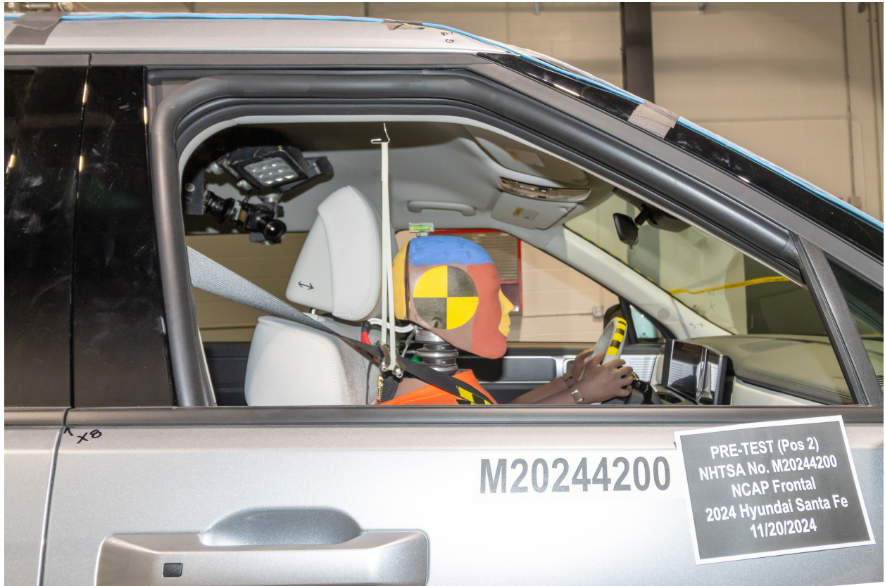
Figure A-55: Pre-Test Passenger Dummy Window View
