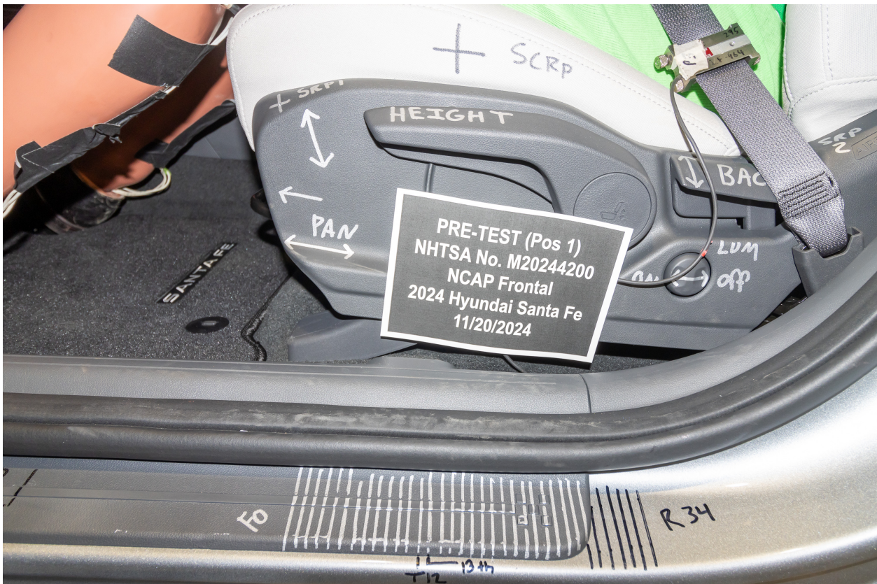
Figure A-36: Pre-Test Driver's Seat Fore-Aft Markings
