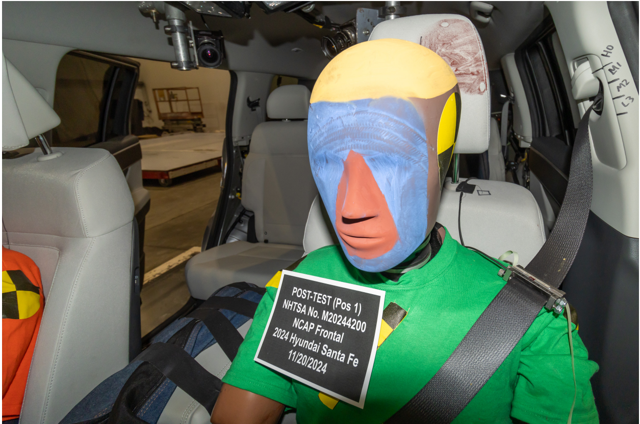
Figure A-48: Post-Test Driver Dummy Face
