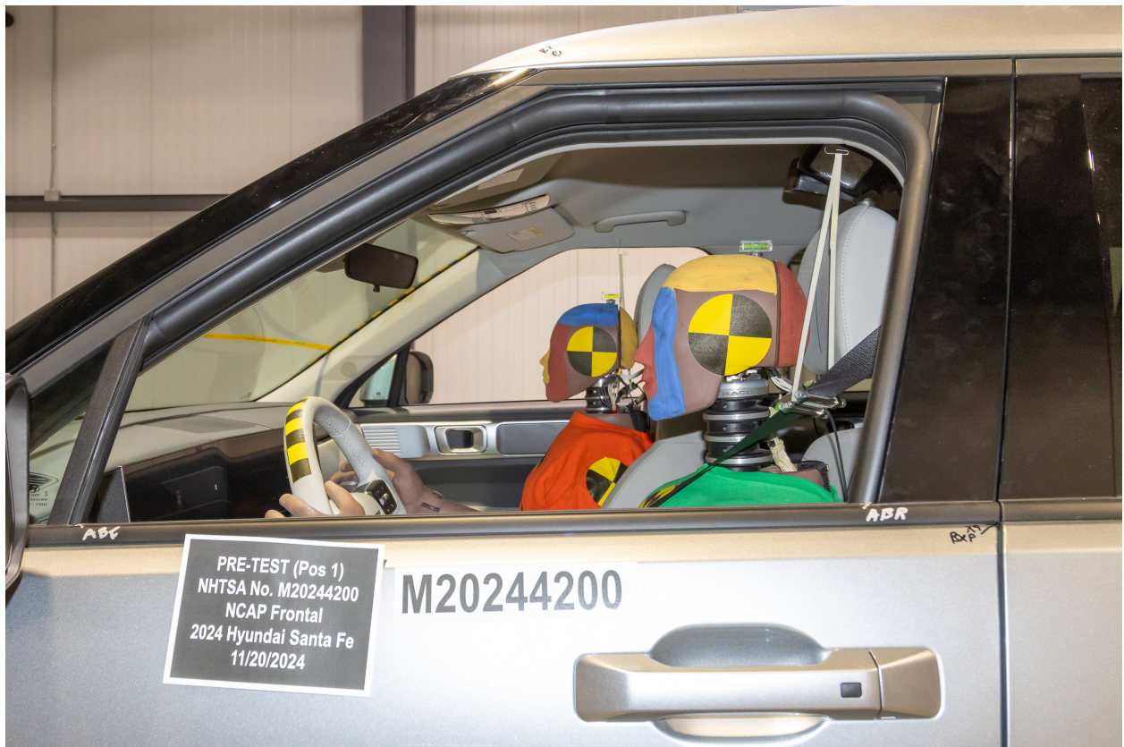
Figure A-32: Pre-Test Driver Dummy Window View
