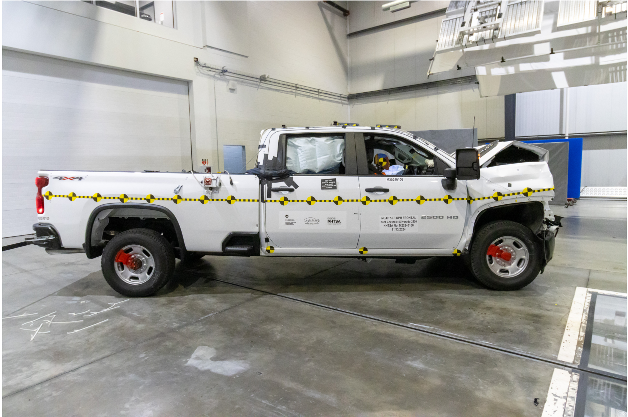
Figure A-13: Post-Test Right View of Test Vehicle
