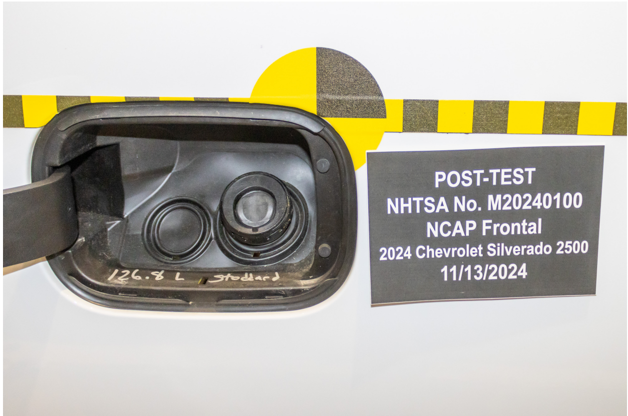
Figure A-23: Post-Test Fuel Filler Cap View
