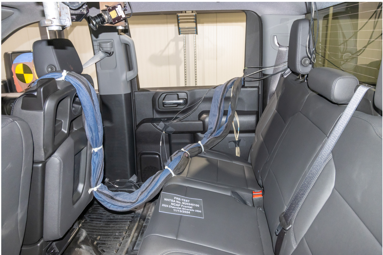
Figure A-28: Pre-Test Dummy Cable Routing
