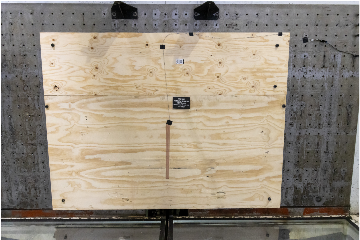
Figure A-2: Pre-Test Load Cell Wall
