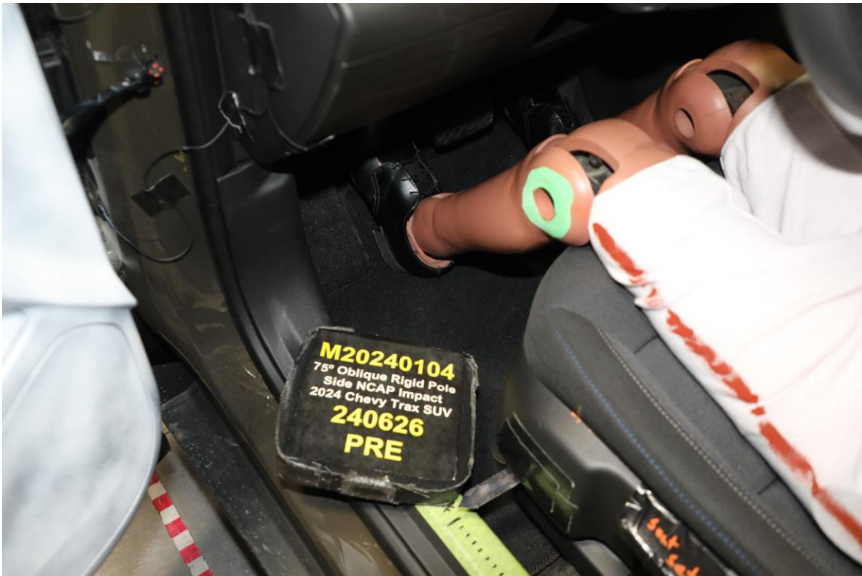
No. 032 Pre-Test Placement of Dummy Feet
