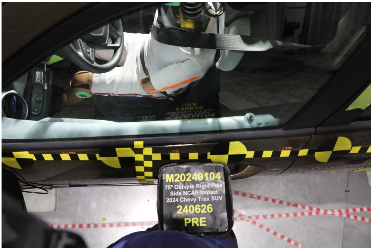
No. 040 Pre-Test Dummy and Door Clearance View
