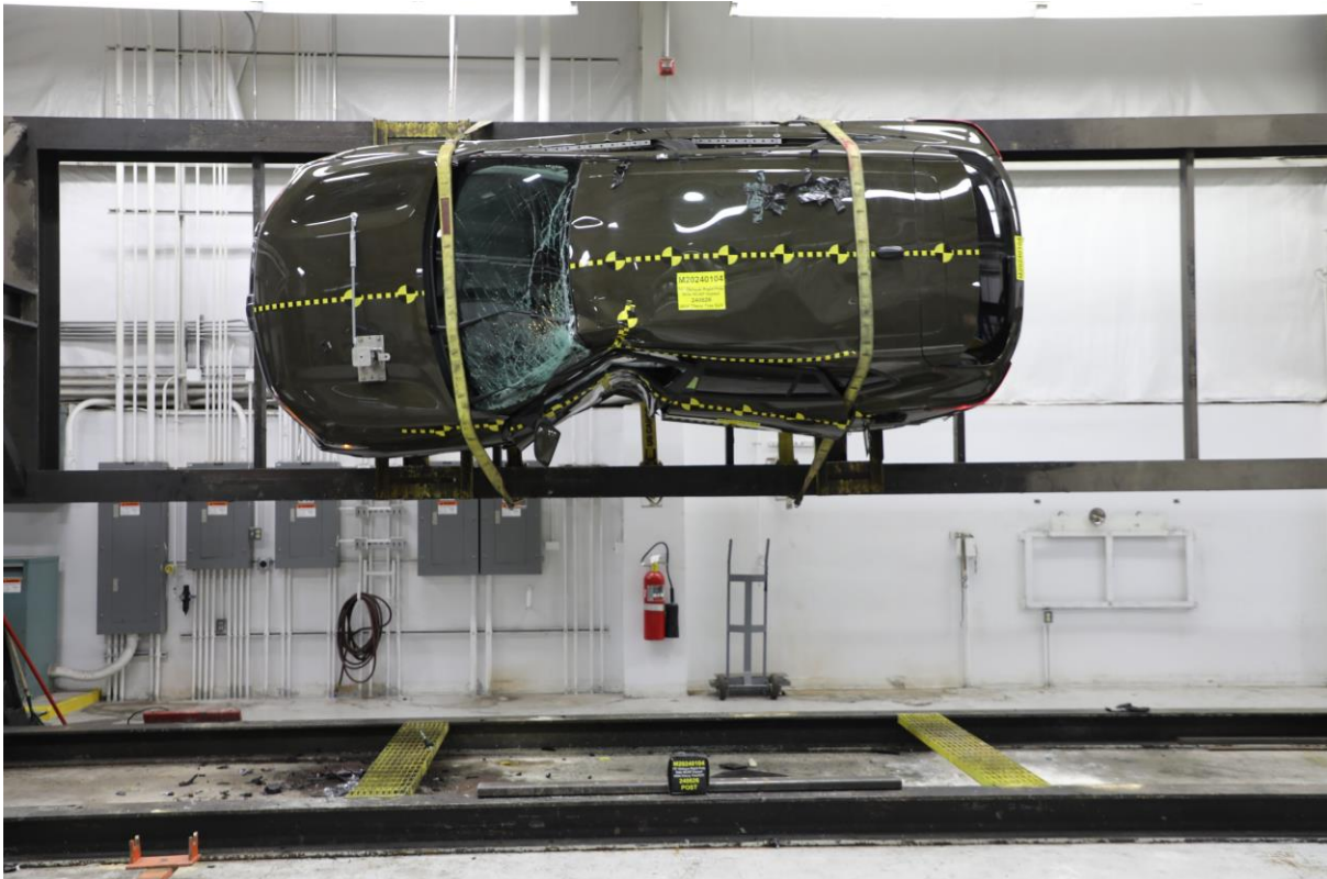
No. 066 FMVSS No. 301 Static Rollover 90 Degrees
