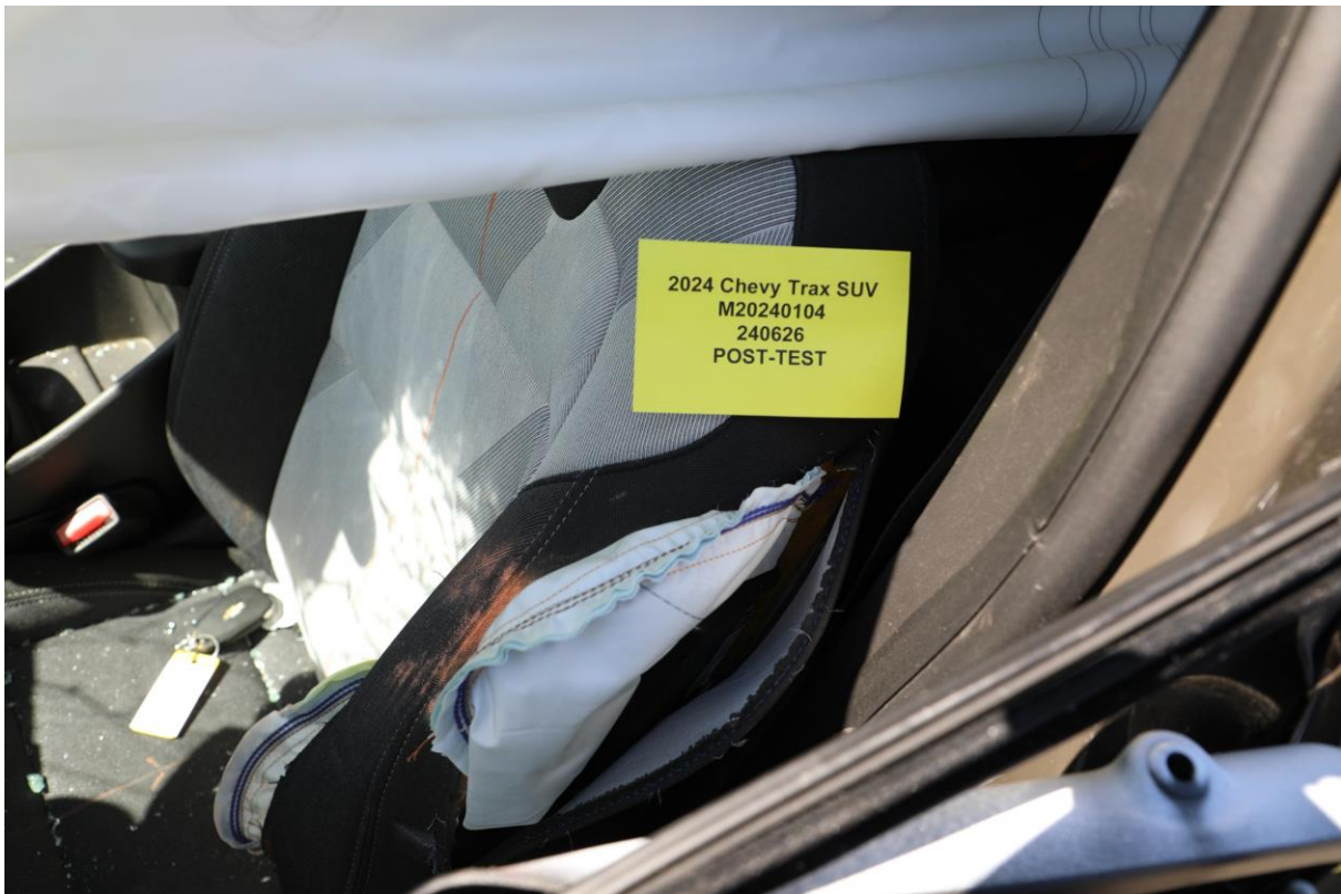
No. 074a Post-Test Close-up Driver Seat Airbag Deployment View
