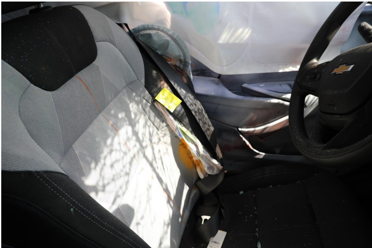
No. 074 Post-Test Close-up Driver Seat Airbag Deployment View
