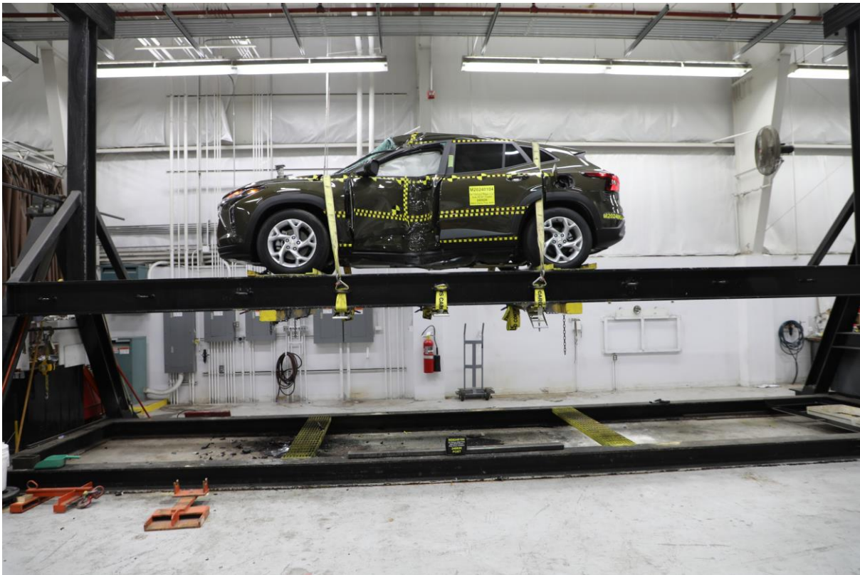
No. 069 FMVSS No. 301 Static Rollover 360 Degrees
