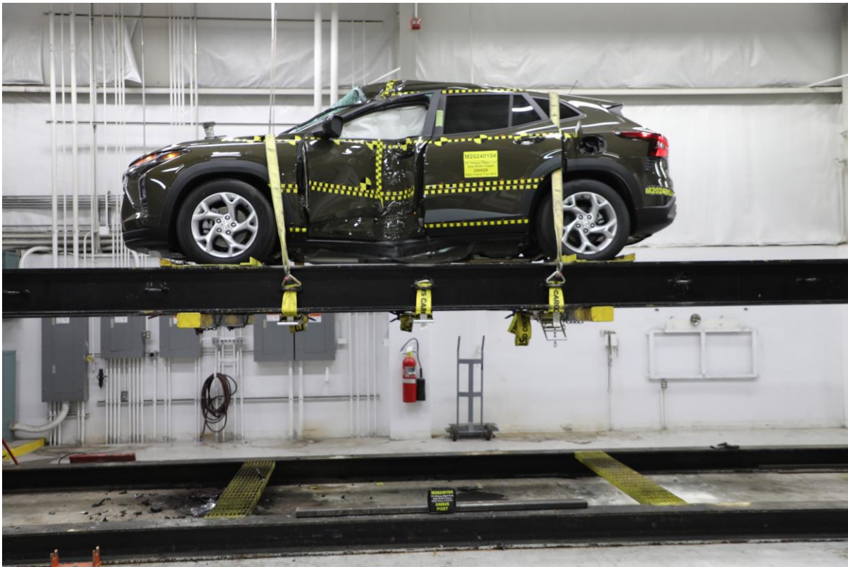
No. 065 FMVSS No. 301 Static Rollover 0 Degrees
