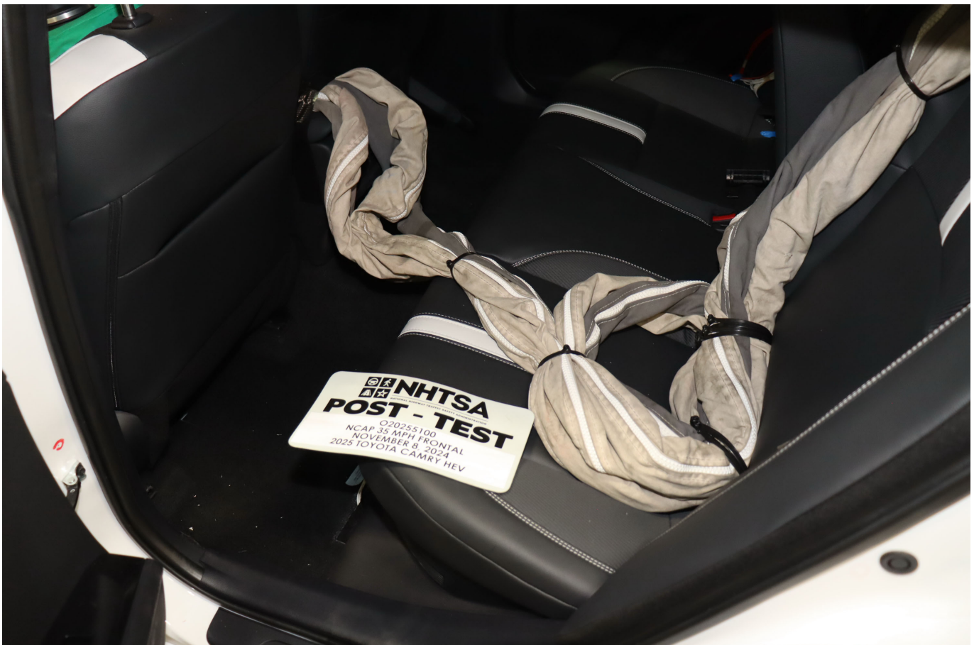
Photo No. 029 - Post-Test Dummy Cable Routing
