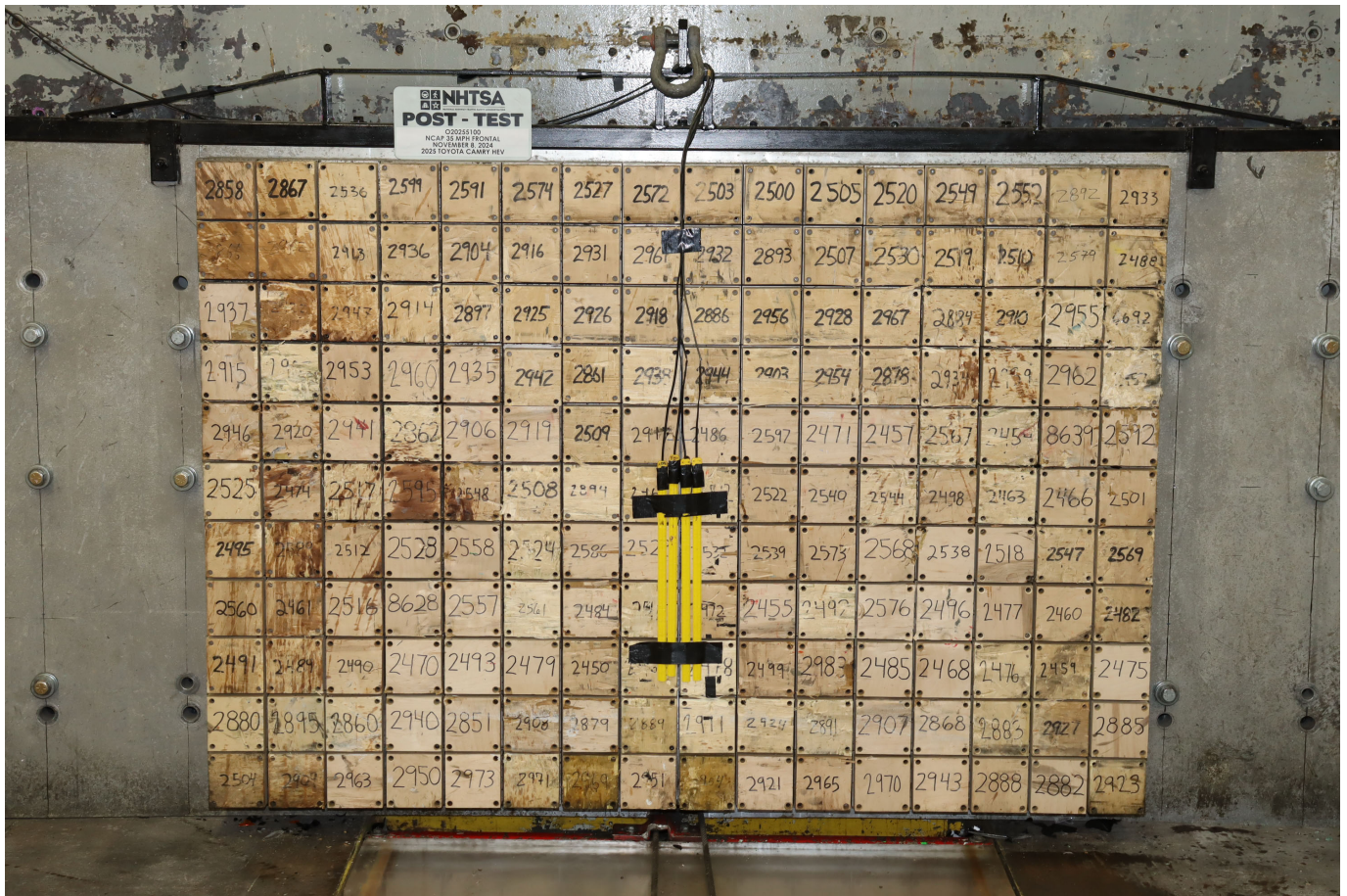
Photo No. 003 - Post-Test Load Cell Wall
