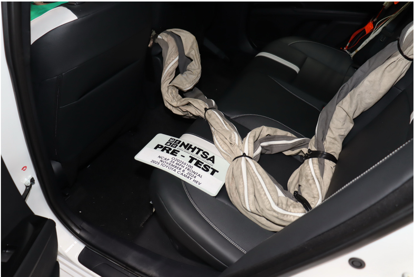
Photo No. 028 - Pre-Test Dummy Cable Routing
