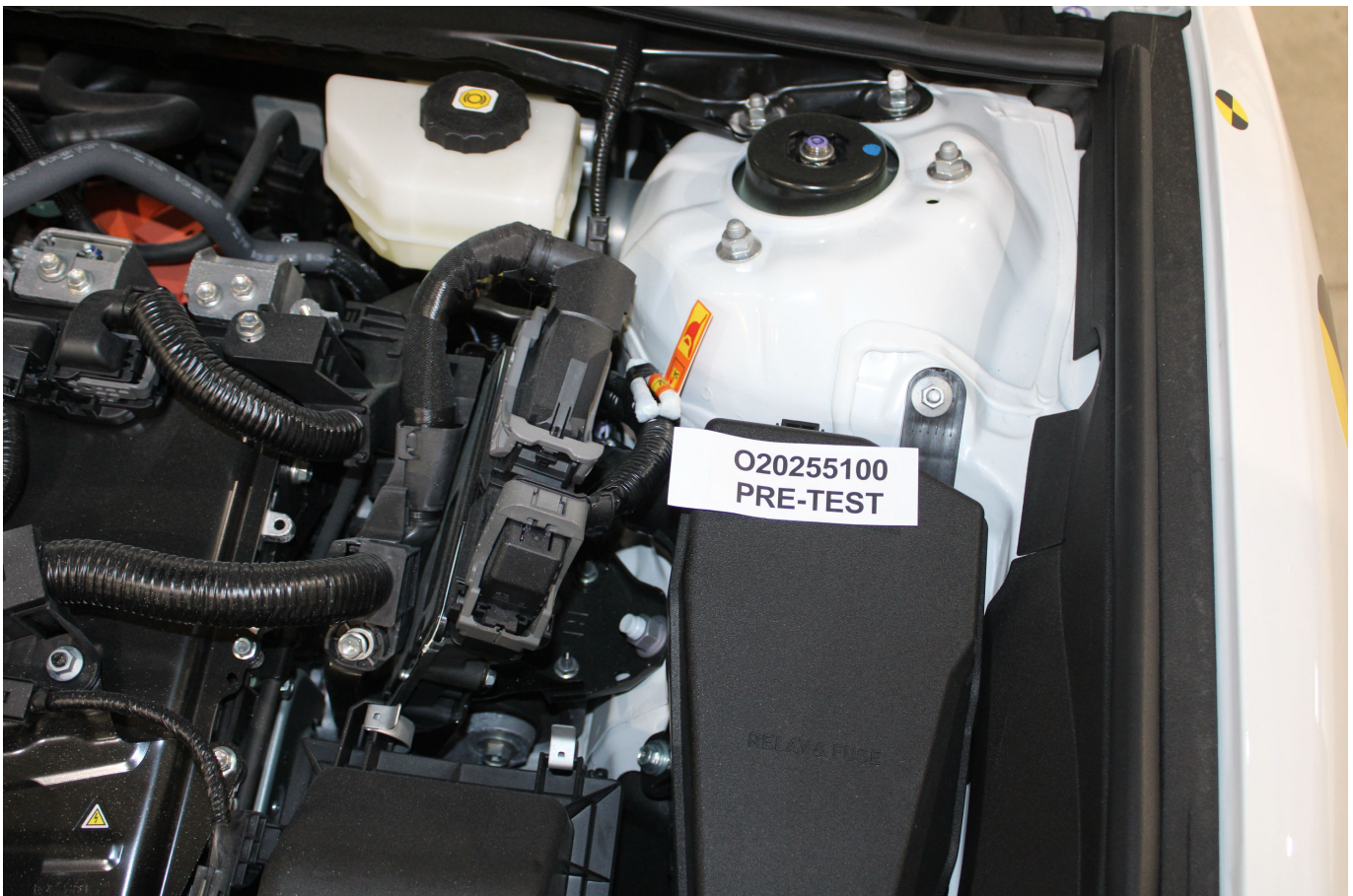
Photo No. 305-04 - First Responder Warning Location
