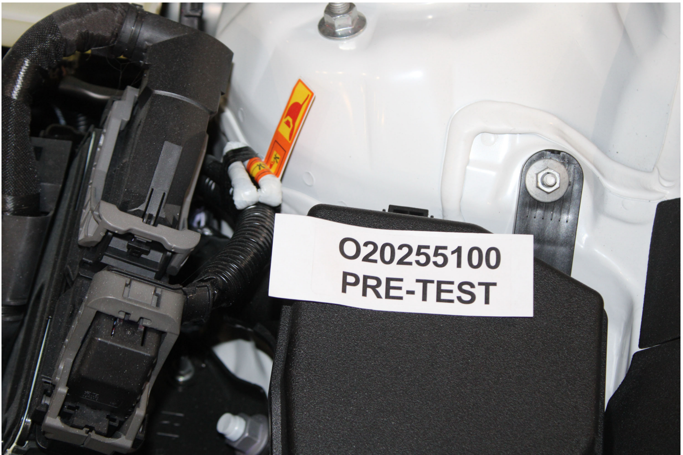
Photo No. 305-03 - First Responder Warning Label
