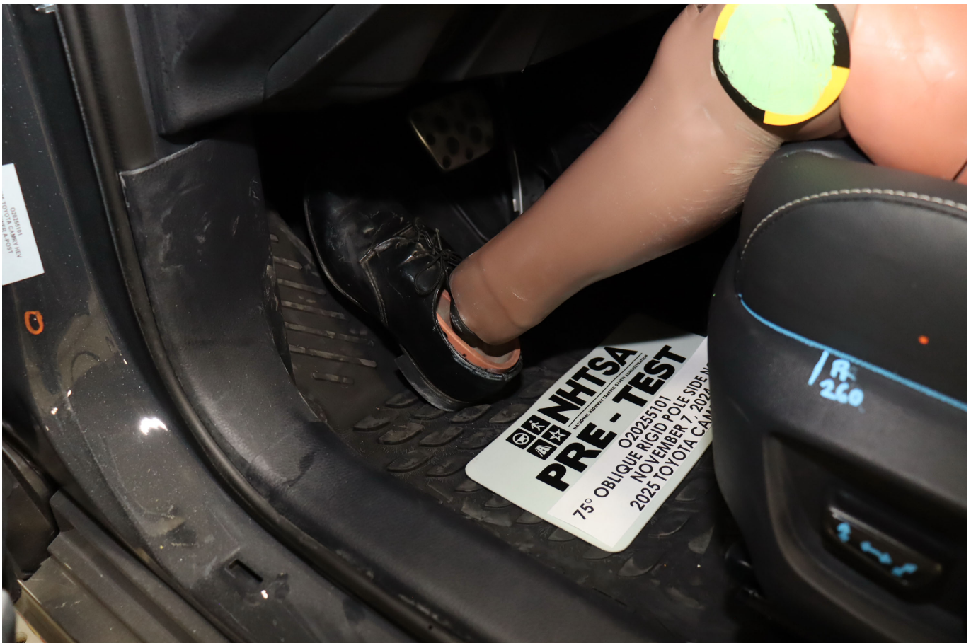
Photo No. 032 - Pre-Test Placement of Dummy's Feet
