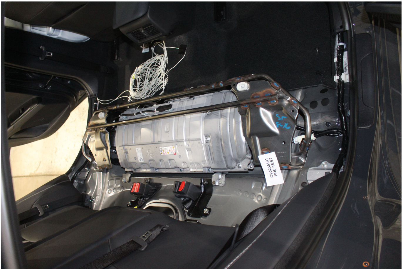
Photo No. 305-09 - Pre-Impact View of Propulsion Battery
