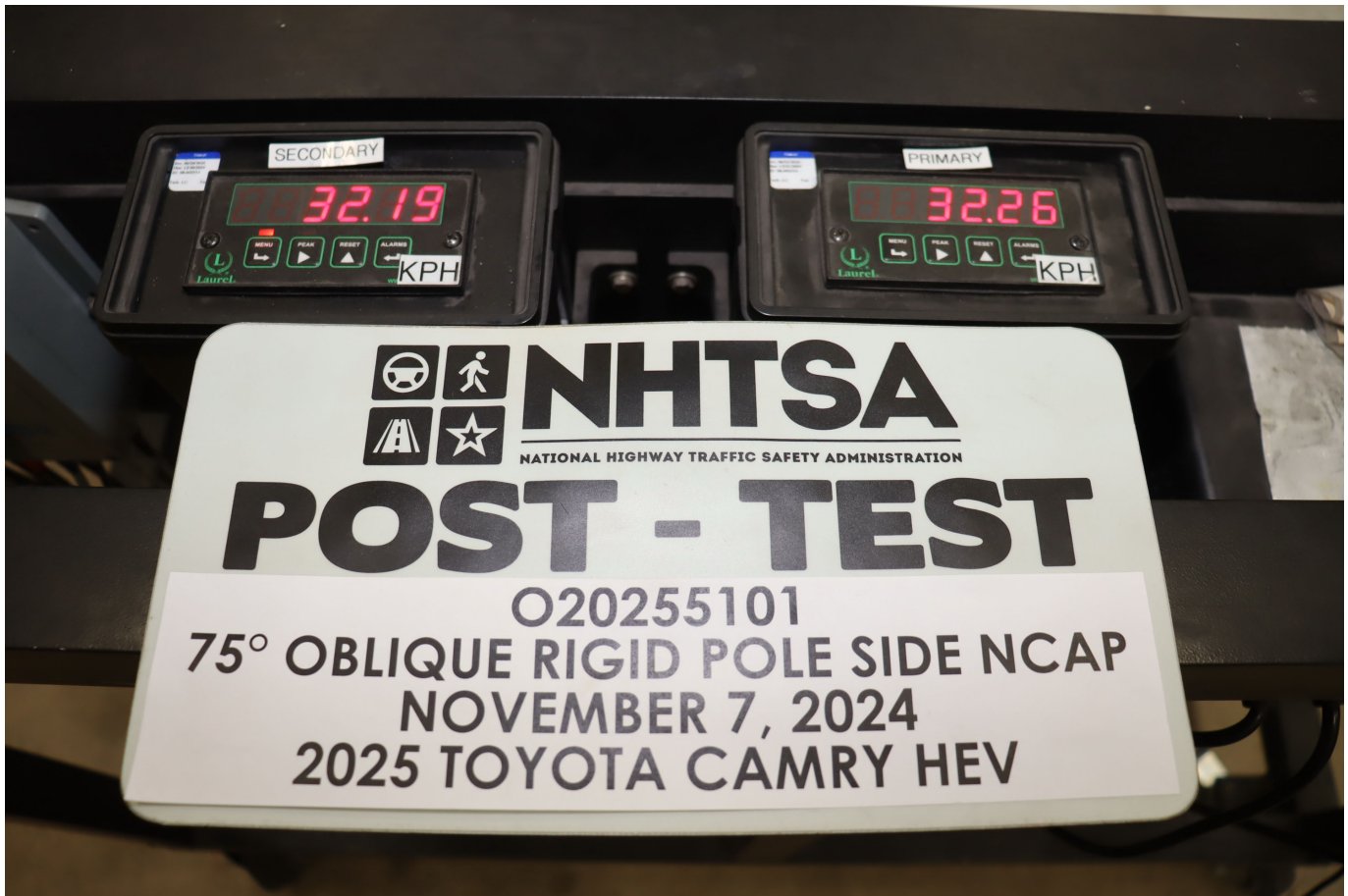
Photo No. 064 - Post-Test Primary and Redundant Speed Trap Read-Out
