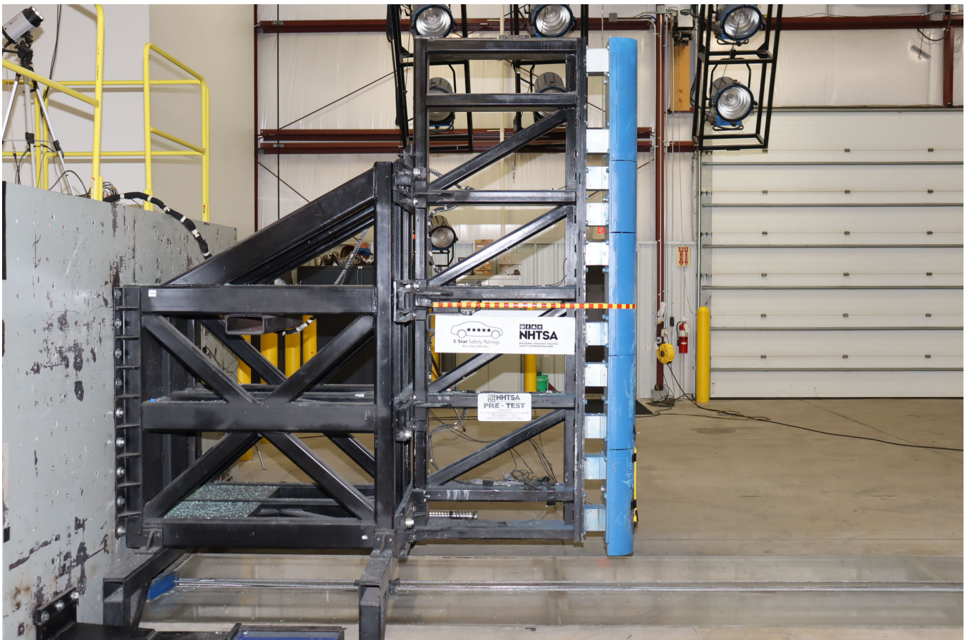
Photo No. 061 - Pre-Test Pole Barrier Side View
