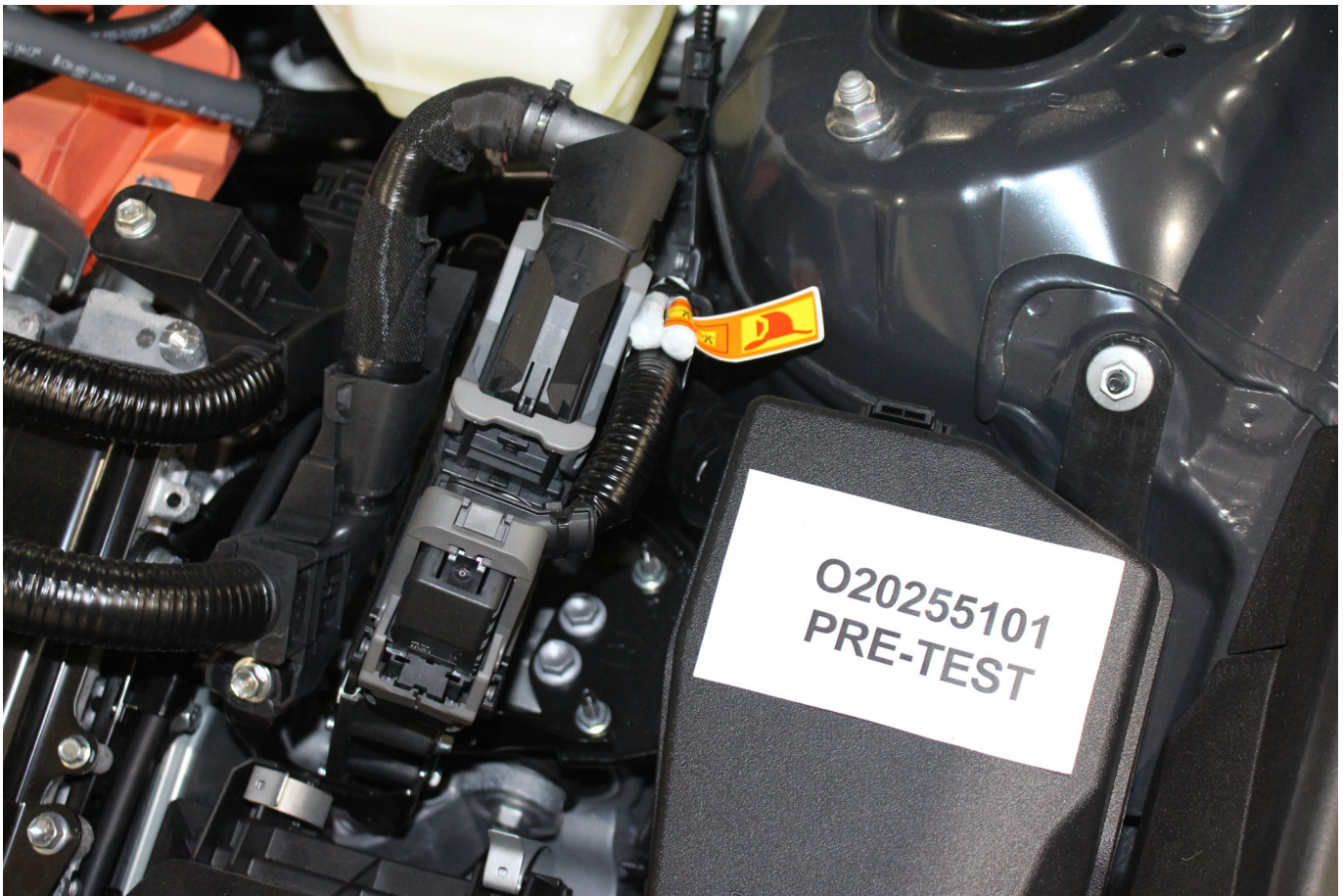
Photo No. 305-03 - First Responder Warning Label
