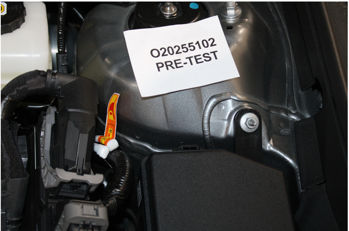
Photo No. 305-03 - First Responder Warning Label
