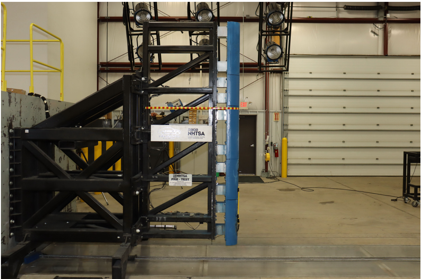
Photo No. 061 - Pre-Test Pole Barrier Side View
