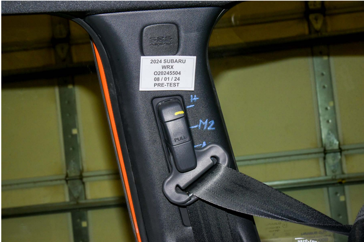
FIGURE 33. Pre-Test View of Belt Anchorage for Dummy
