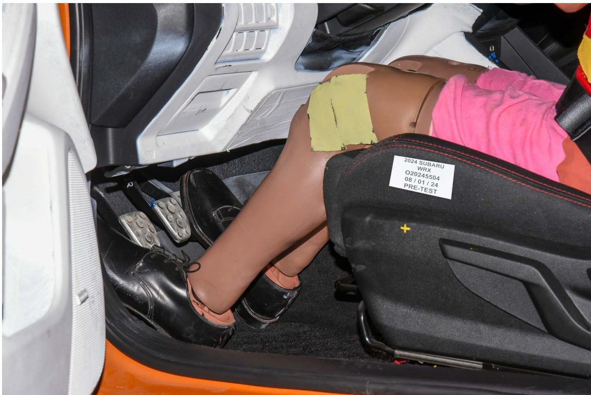
FIGURE 32. Pre-Test Placement of Dummy's Feet
