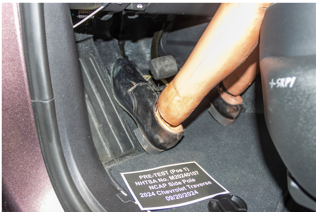
Figure A-32: Pre-Test Placement of Dummy's Feet
