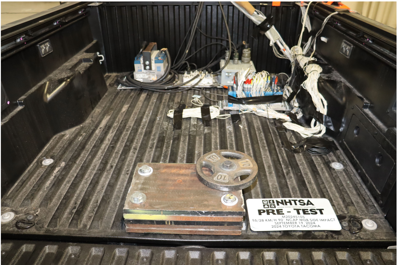
Photo No. 094 - Pre-Test Ballast View
