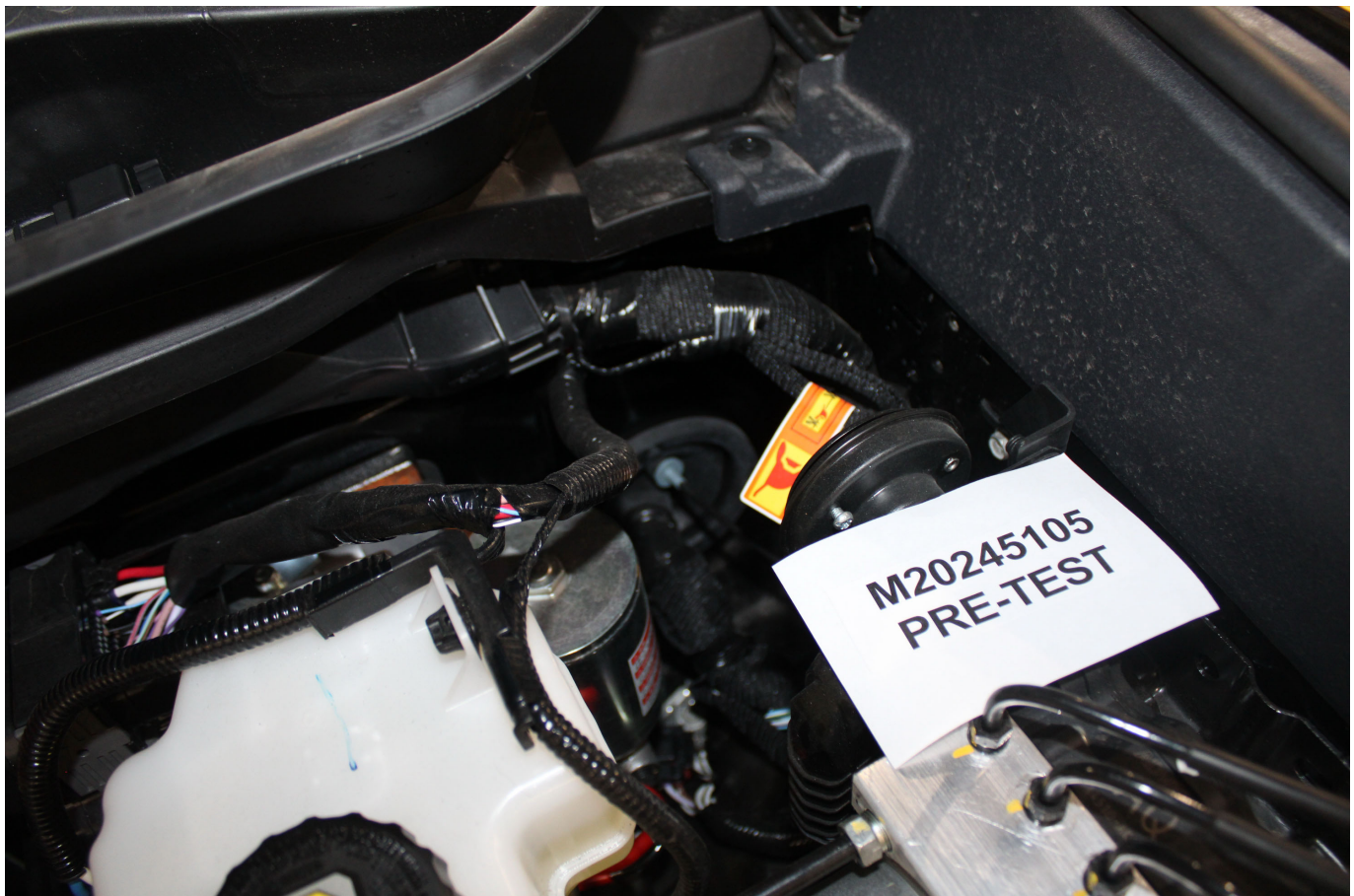
Photo No. 305-03 - First Responder Warning Label
