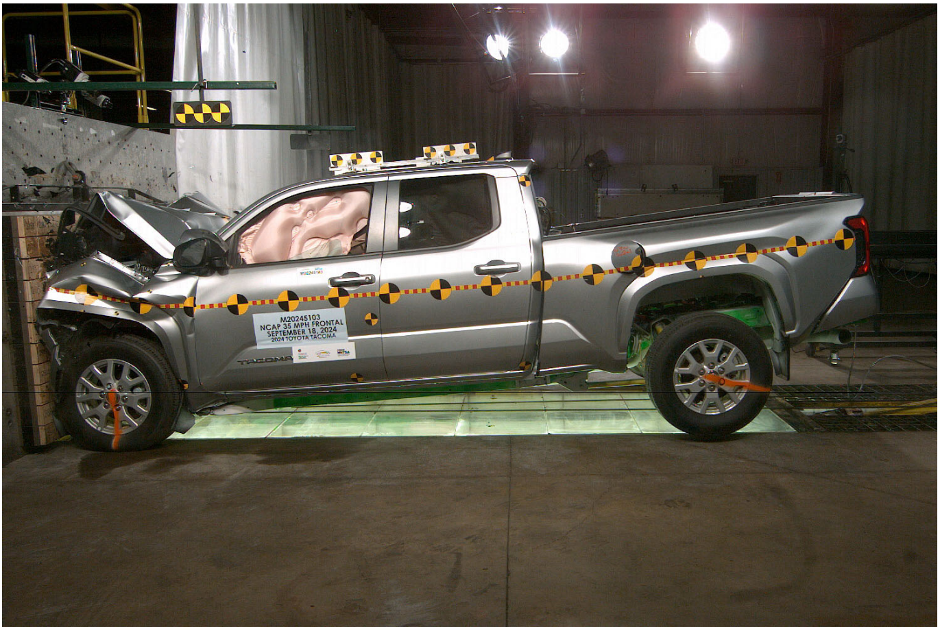
Photo No. 082 - 2024 Toyota Tacoma SR5 4x4 Double Cab Pickup Truck Frontal Impact Event
