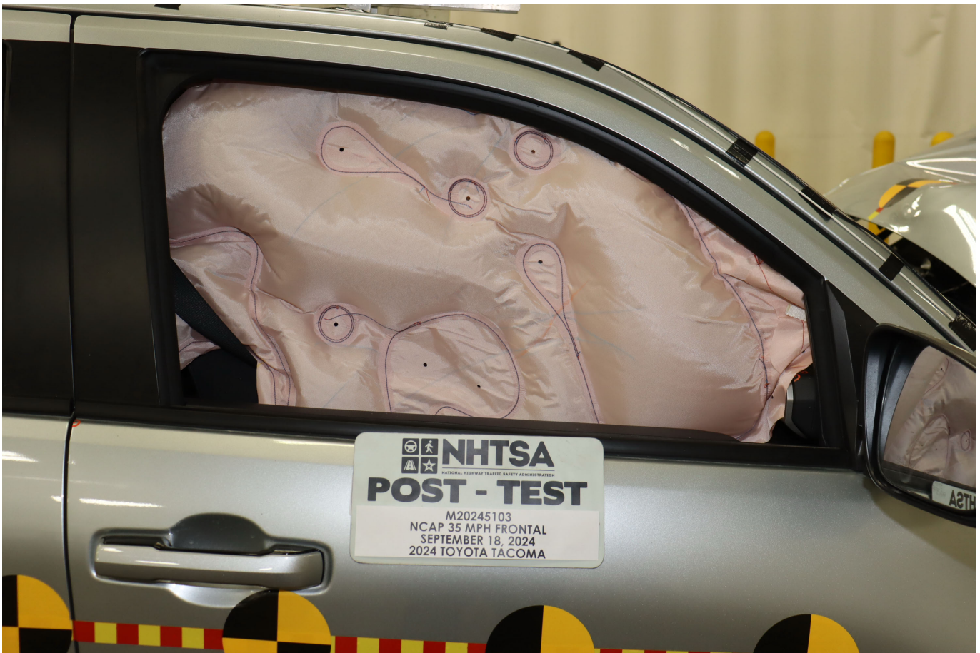
Photo No. 056 - Post-Test Passenger Dummy Window View
