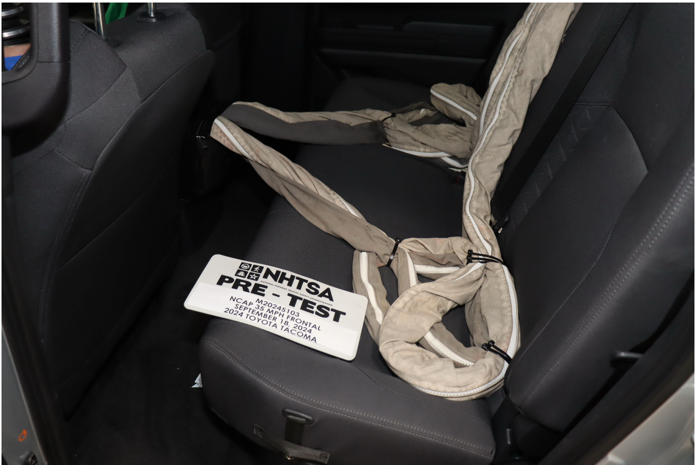
Photo No. 028 - Pre-Test Dummy Cable Routing
