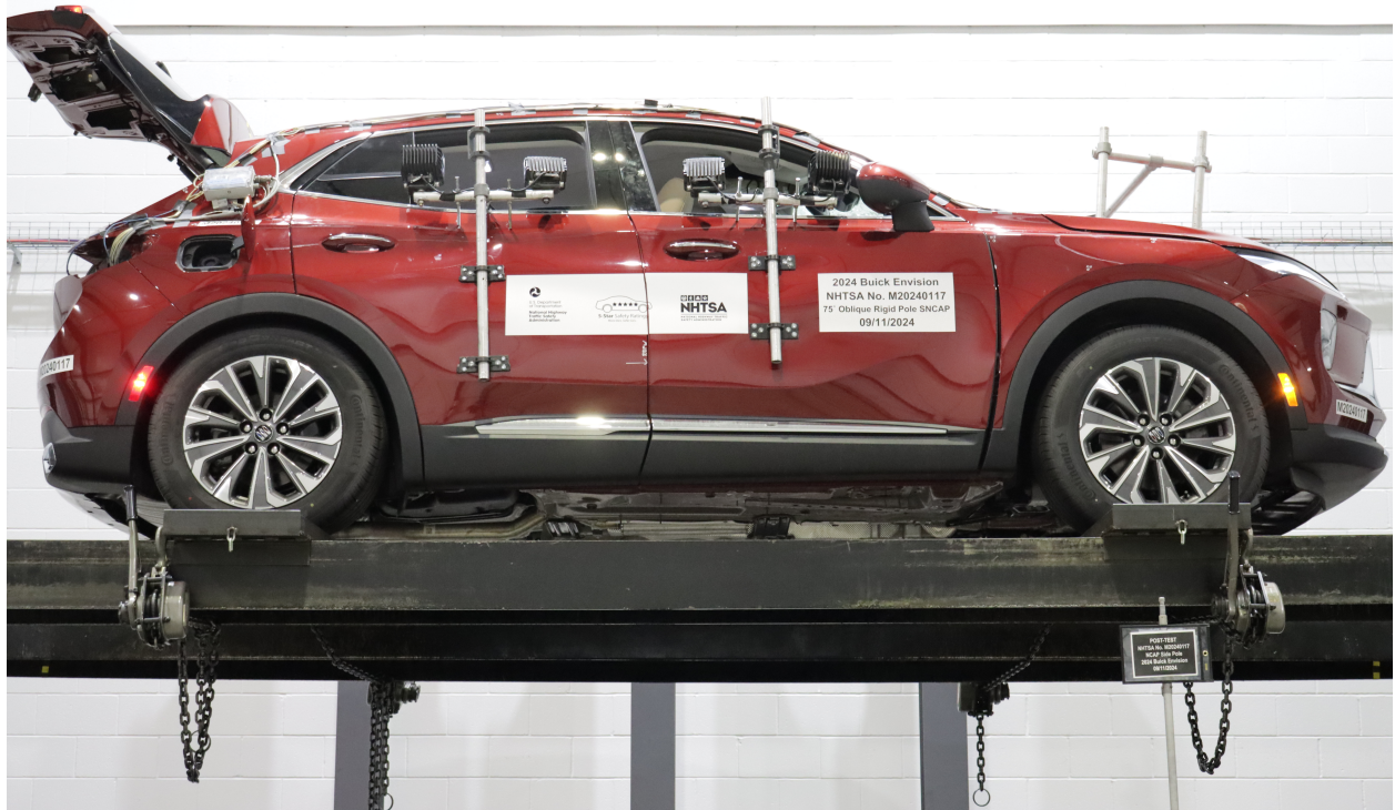
Figure A-69: FMVSS No. 301 Static Rollover 360 Degrees
