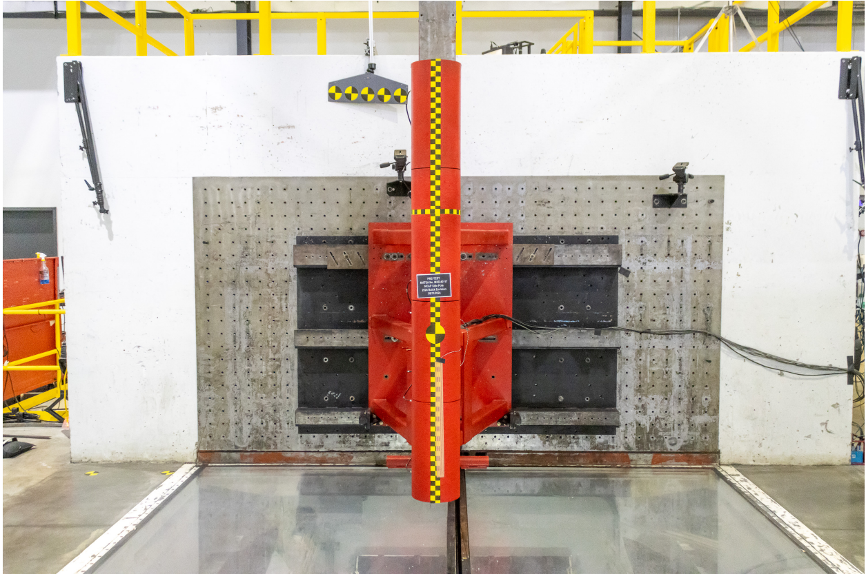
Figure A-59: Pre-Test Pole Barrier Front View
