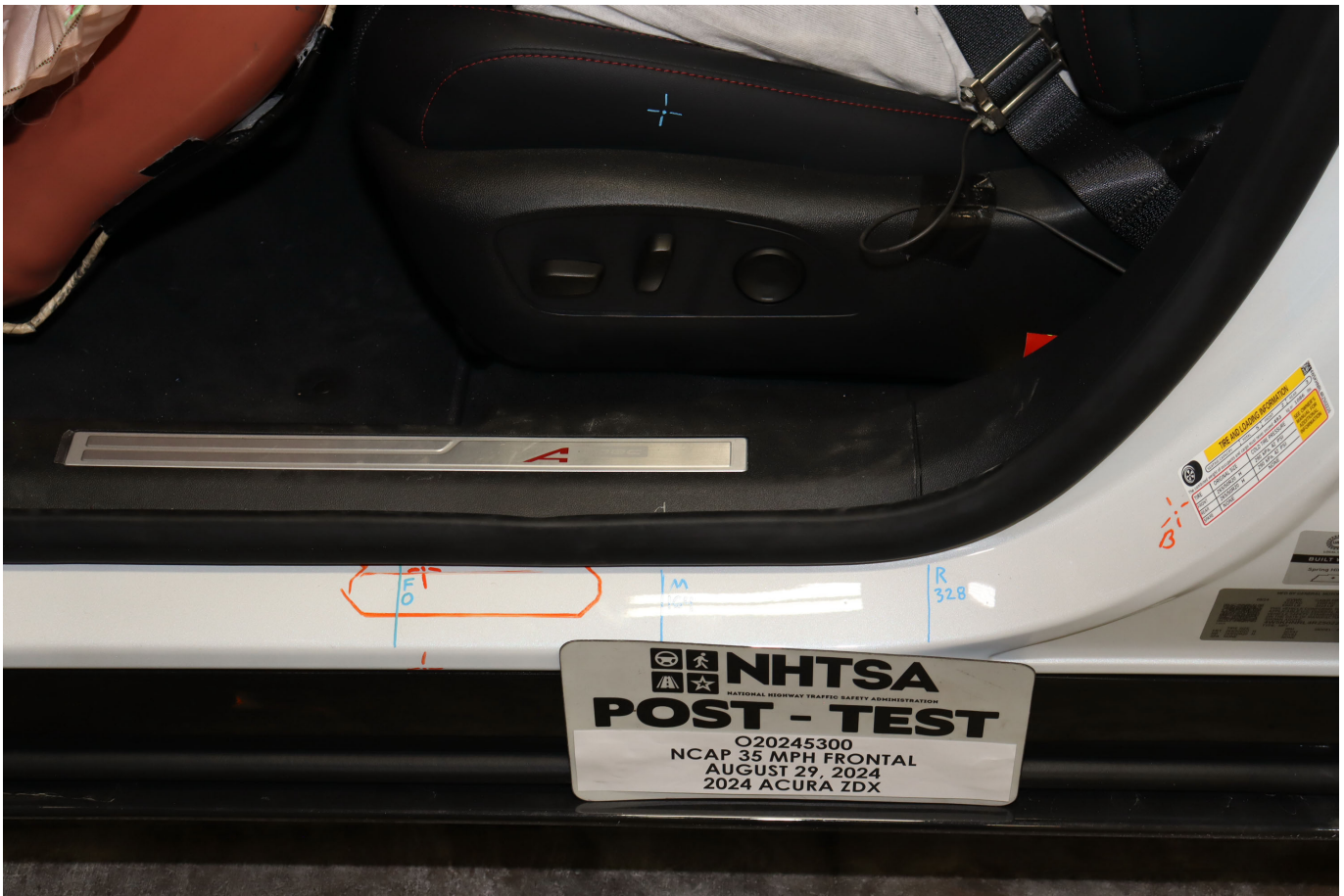
Photo No. 037 - Post-Test Driver's Seat Fore-Aft Markings
