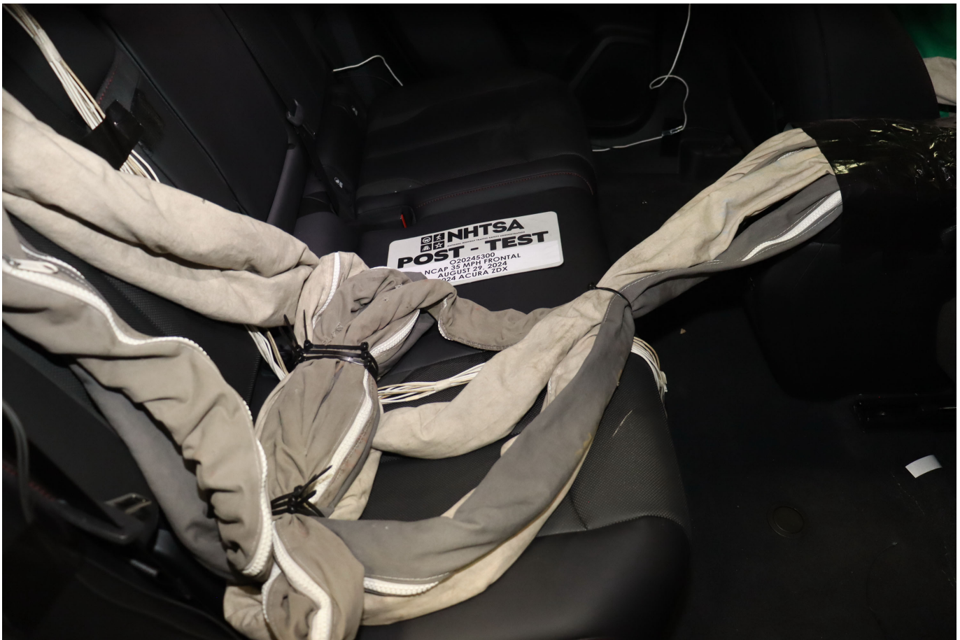
Photo No. 029 - Post-Test Dummy Cable Routing
