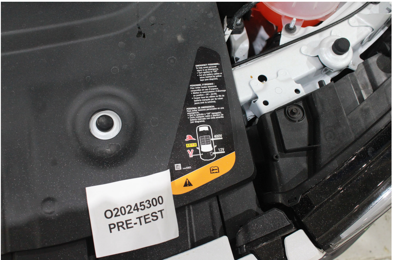
Photo No. 305-03 - First Responder Warning Label
