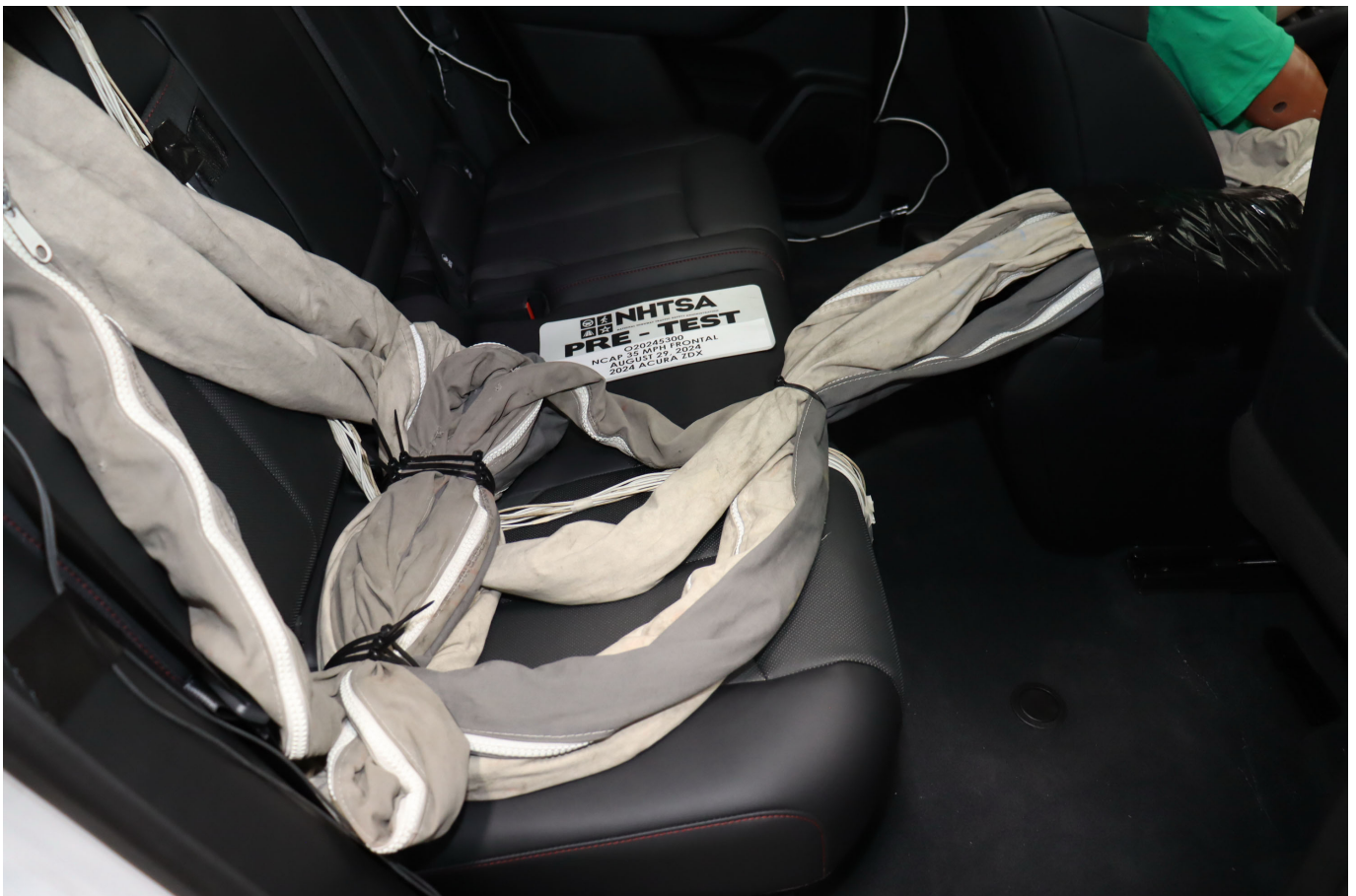
Photo No. 028 - Pre-Test Dummy Cable Routing
