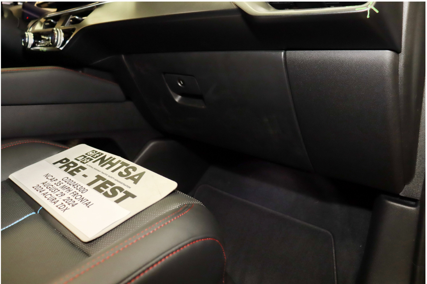
Photo No. 067 - Pre-Test Passenger's Side Knee Bolster
