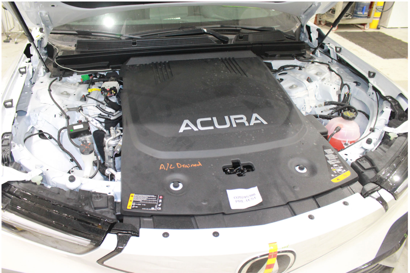
Photo No. 305-04 - First Responder Warning Location
