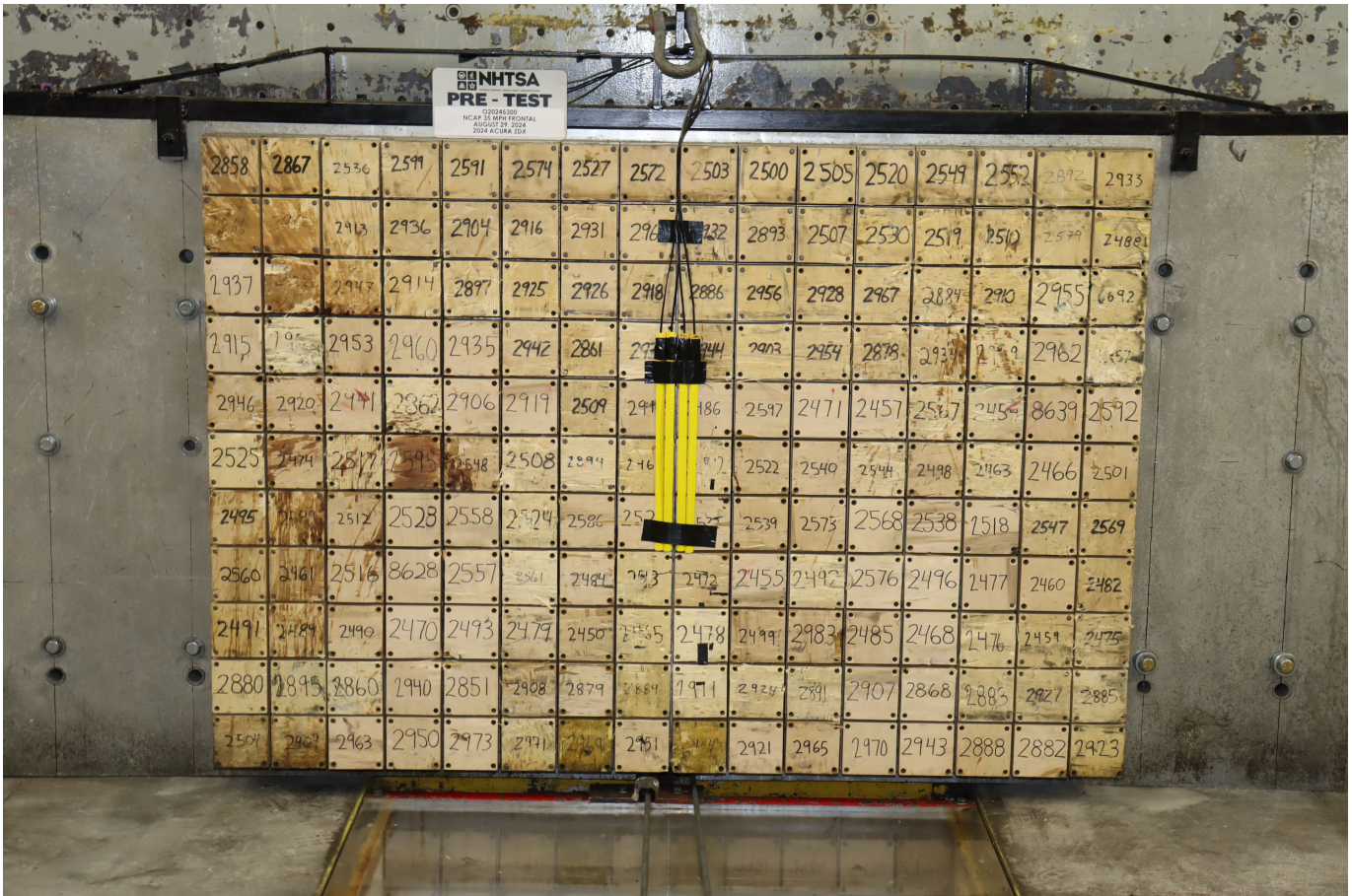
Photo No. 002 - Pre-Test Load Cell Wall
