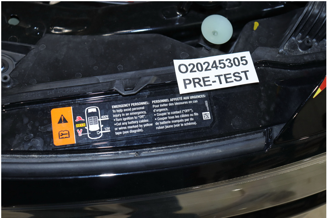
Photo No. 305-03 - First Responder Warning Label
