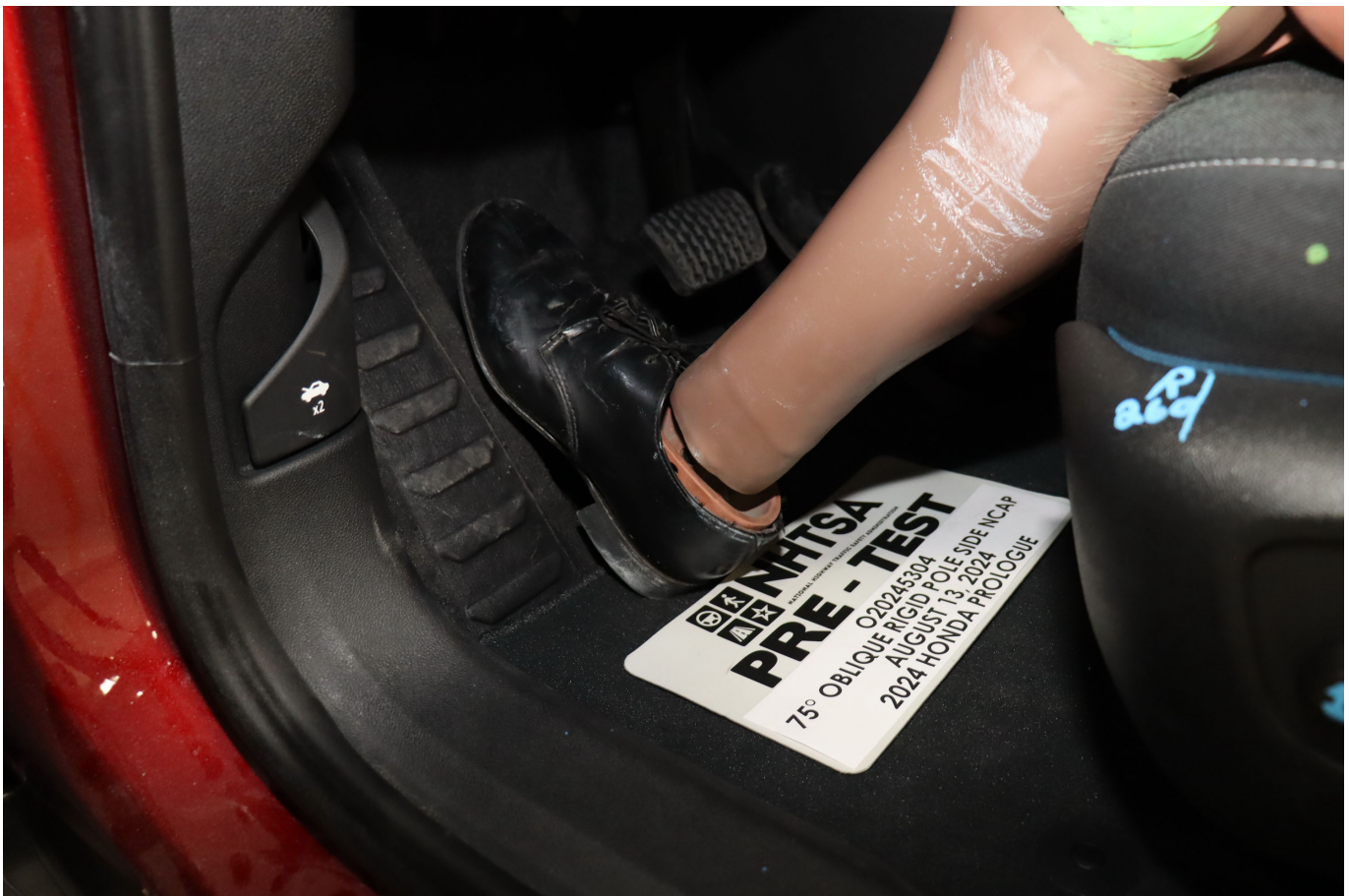
Photo No. 032 - Pre-Test Placement of Dummy's Feet
