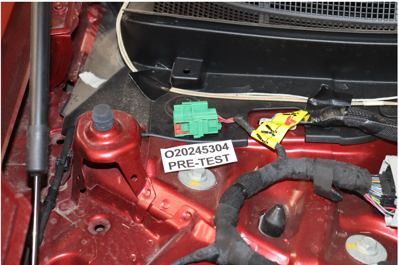
Photo No. 305-07 - Manual High Voltage Service Disconnect Removed
