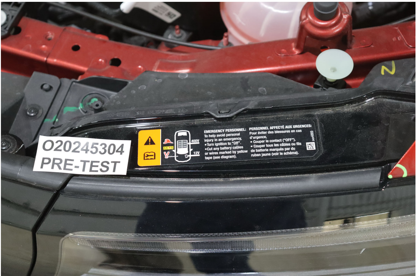
Photo No. 305-03 - First Responder Warning Label
