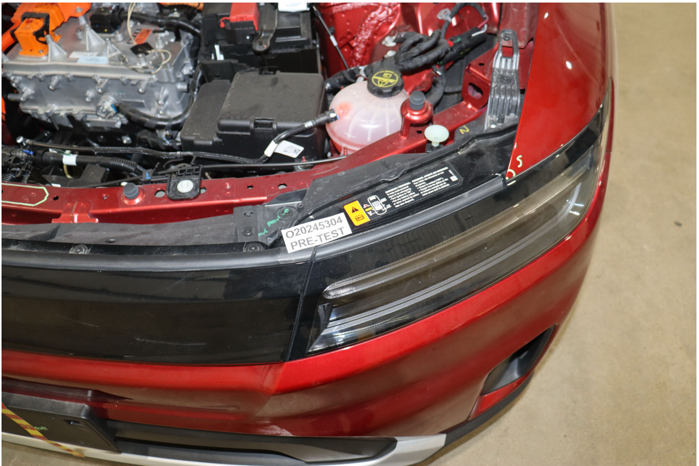
Photo No. 305-04 - First Responder Warning Location
