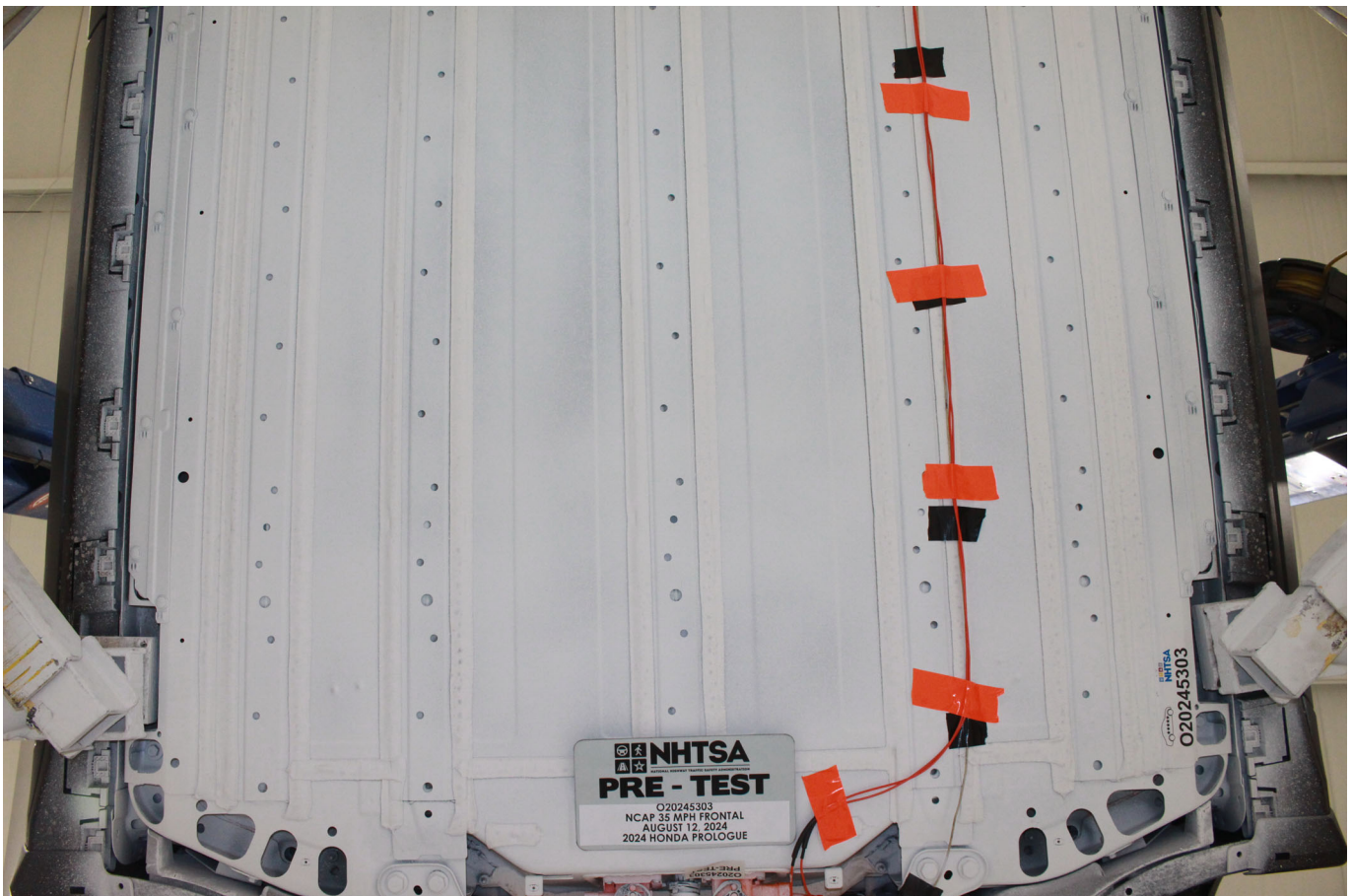
Photo No. 305-09 - Pre-Impact View of Propulsion Battery
