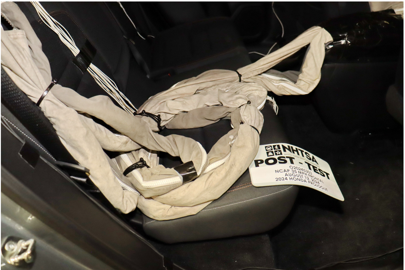
Photo No. 029 - Post-Test Dummy Cable Routing
