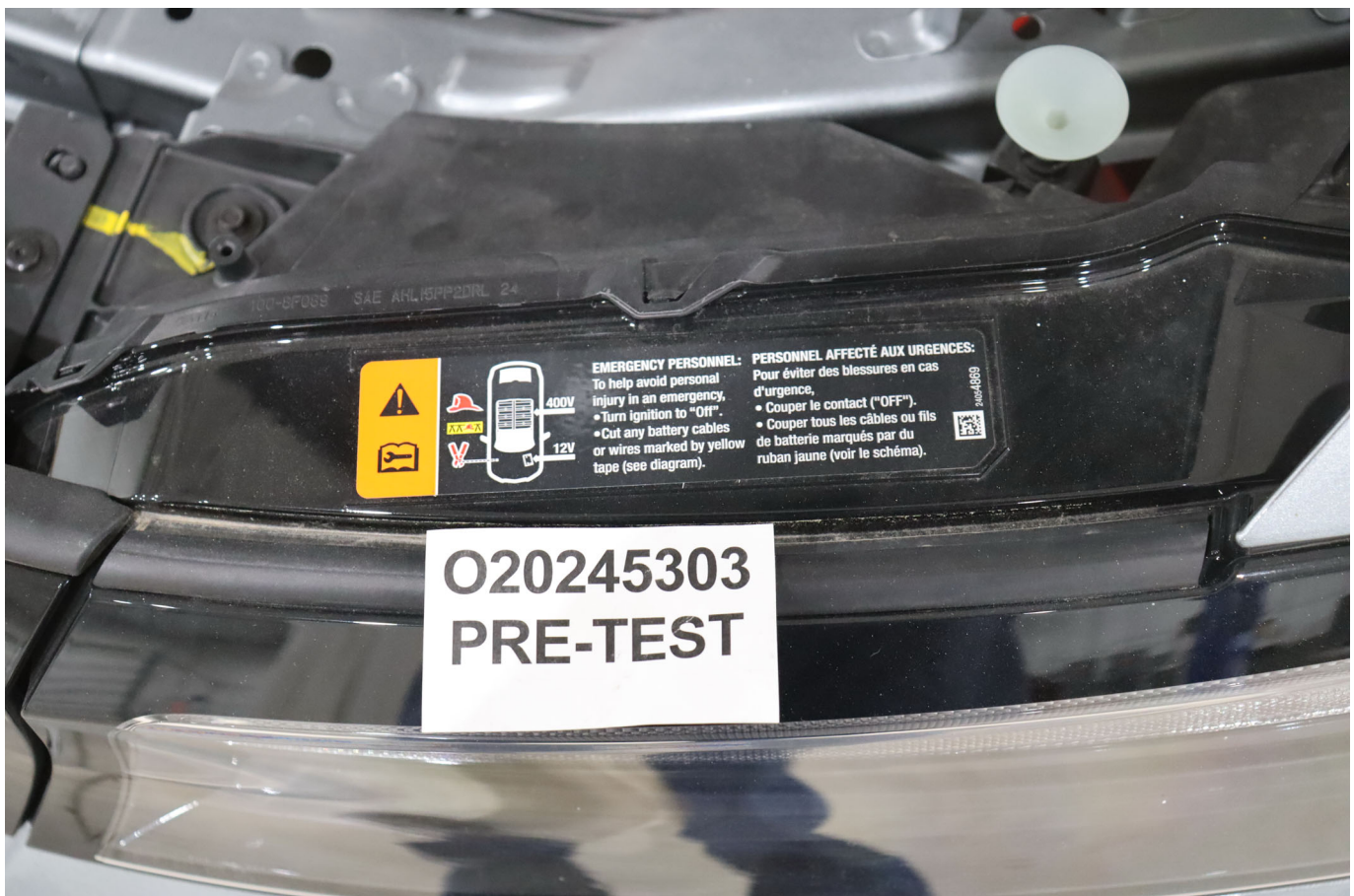
Photo No. 305-03 - First Responder Warning Label
