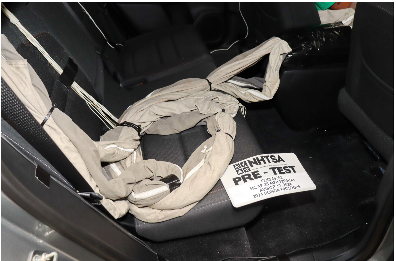
Photo No. 028 - Pre-Test Dummy Cable Routing
