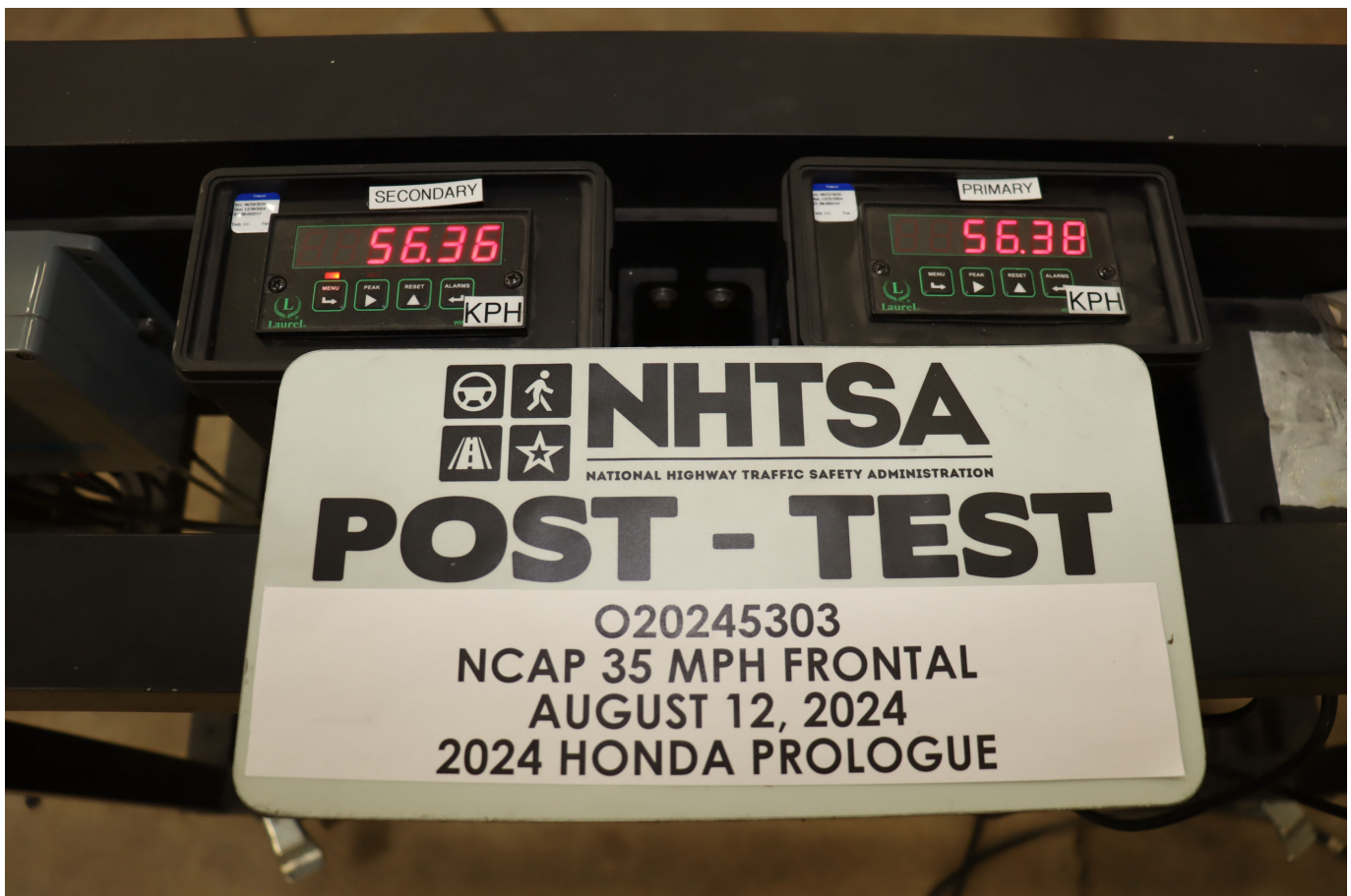
Photo No. 076 - Post-Test Speed Trap Read-Out
