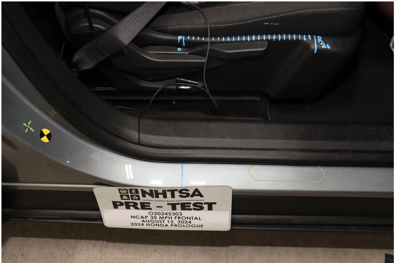
Photo No. 059 - Pre-Test Passenger's Seat Fore-Aft Markings
