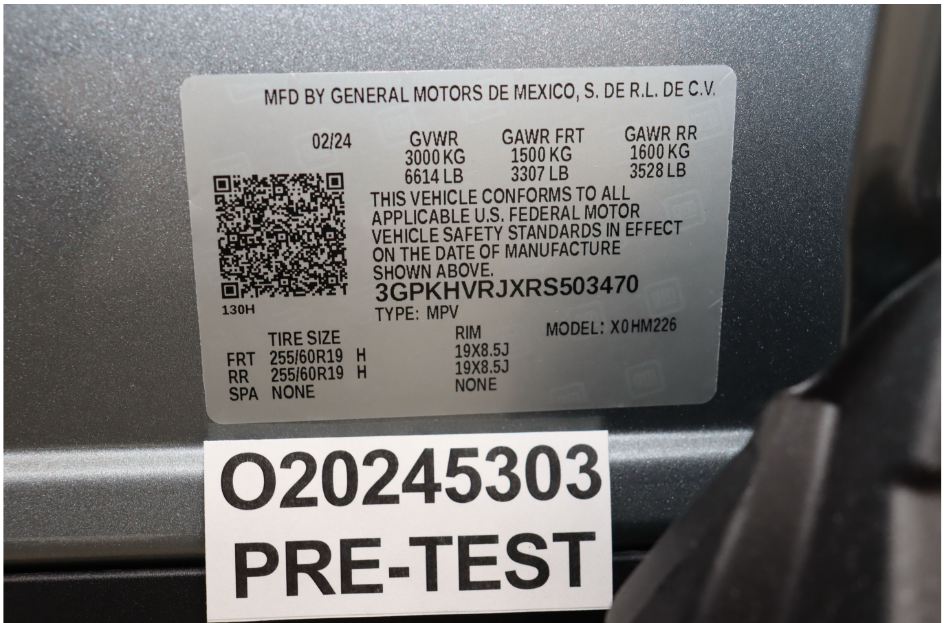
Photo No. 004 - Manufacturer's Label
