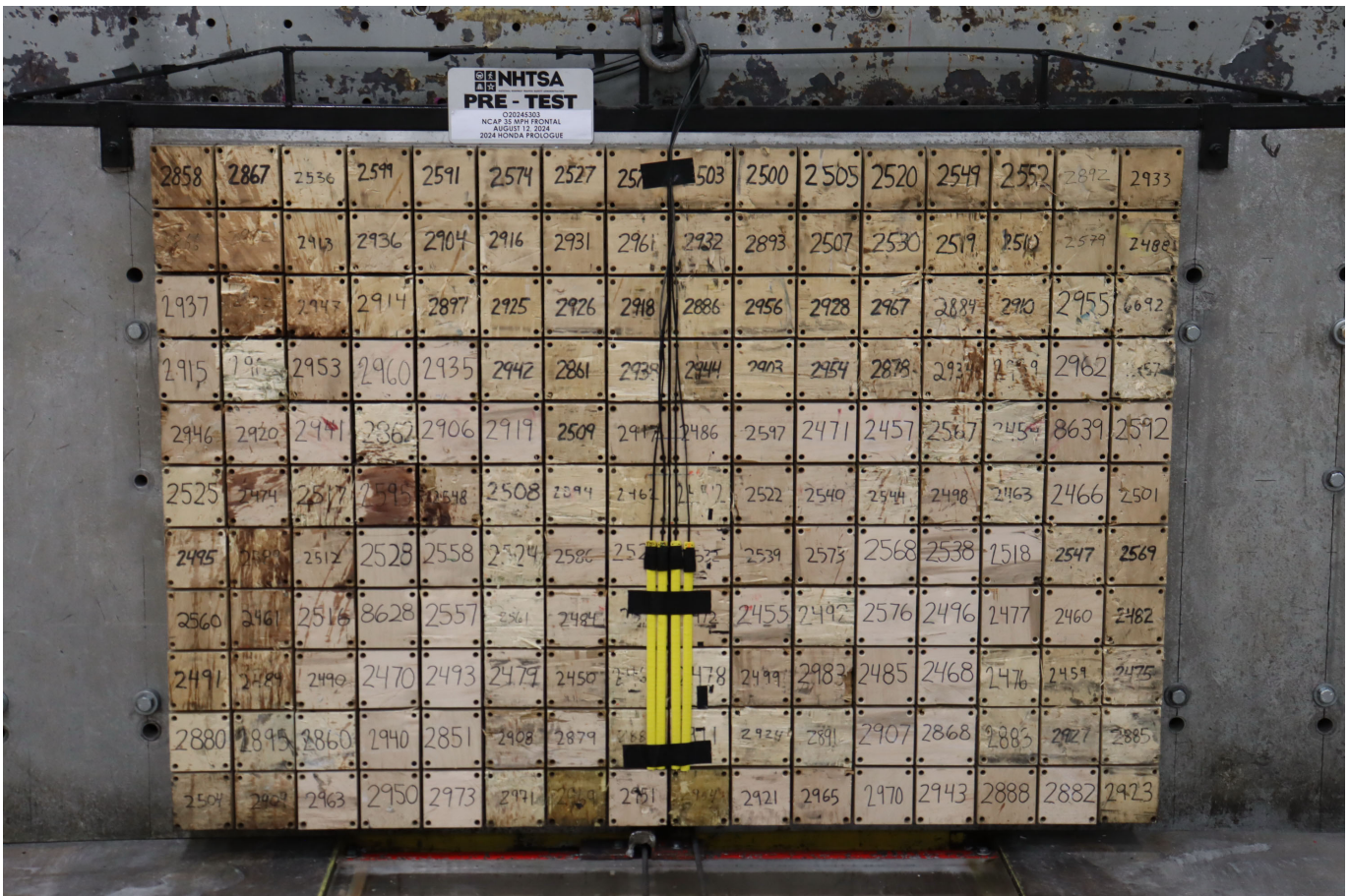
Photo No. 002 - Pre-Test Load Cell Wall
