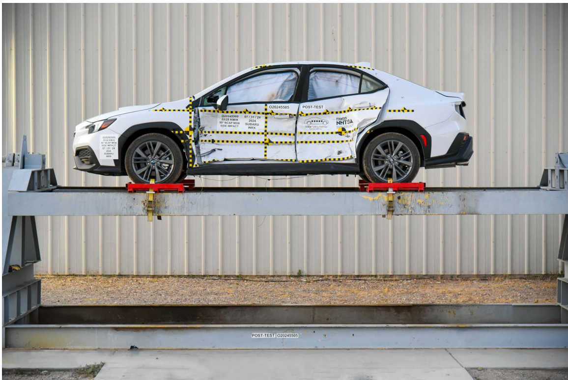
FIGURE 96. FMVSS No. 301 Static Rollover 0 Degrees
