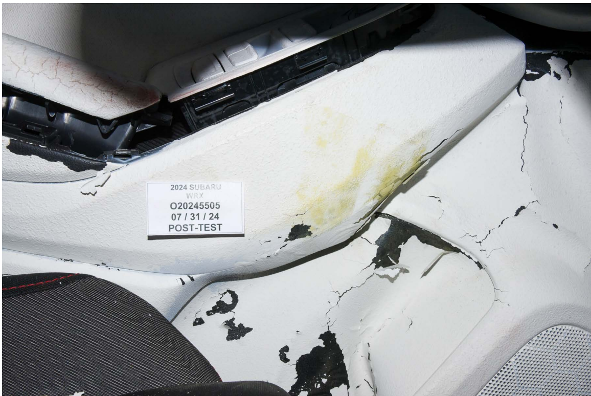
FIGURE 54. Post-Test Driver Dummy Close-Up Knee Contact View
