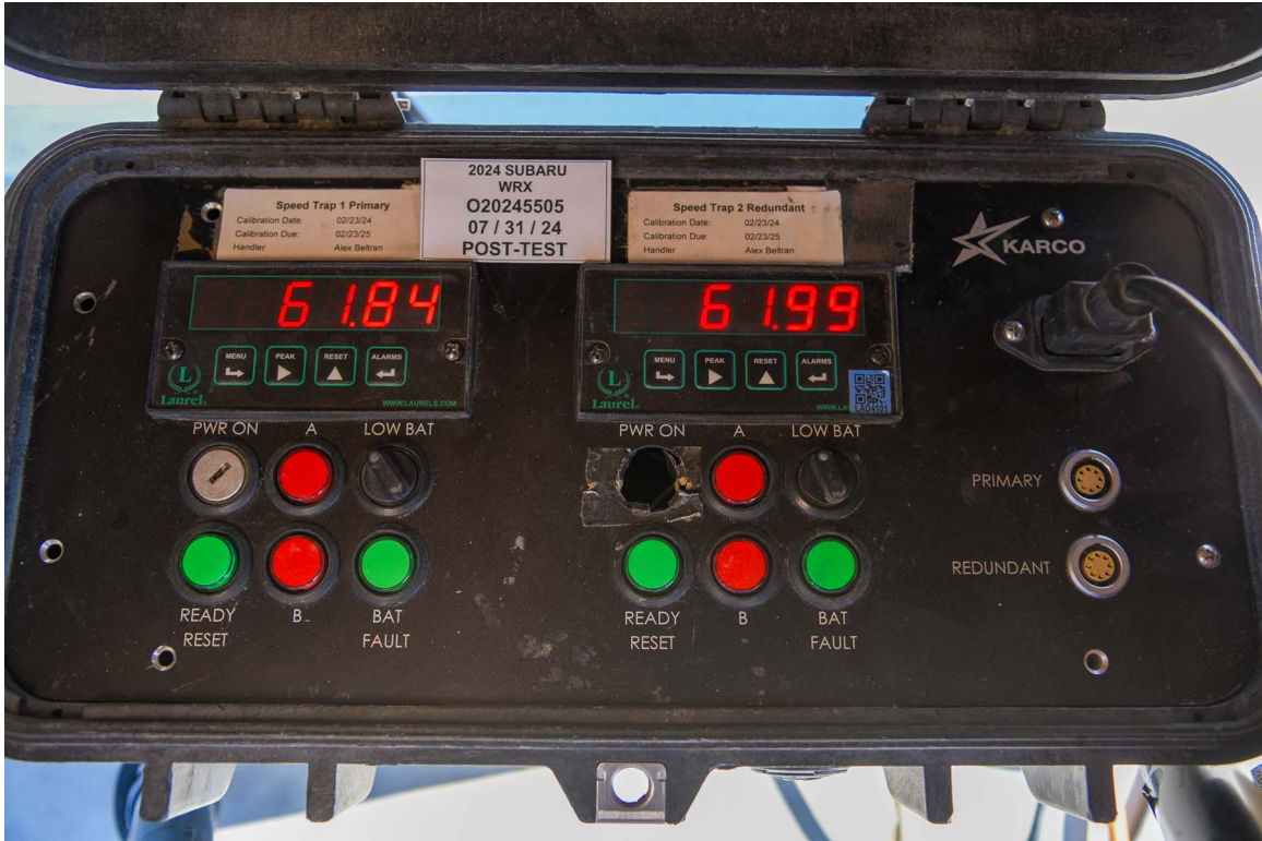
FIGURE 95. Post-Test Primary and Redundant Speed Trap Read-Out
