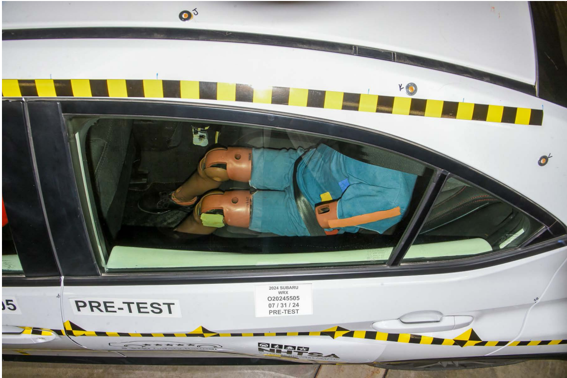
FIGURE 69. Pre-Test Rear Passenger Dummy and Door Clearance View
