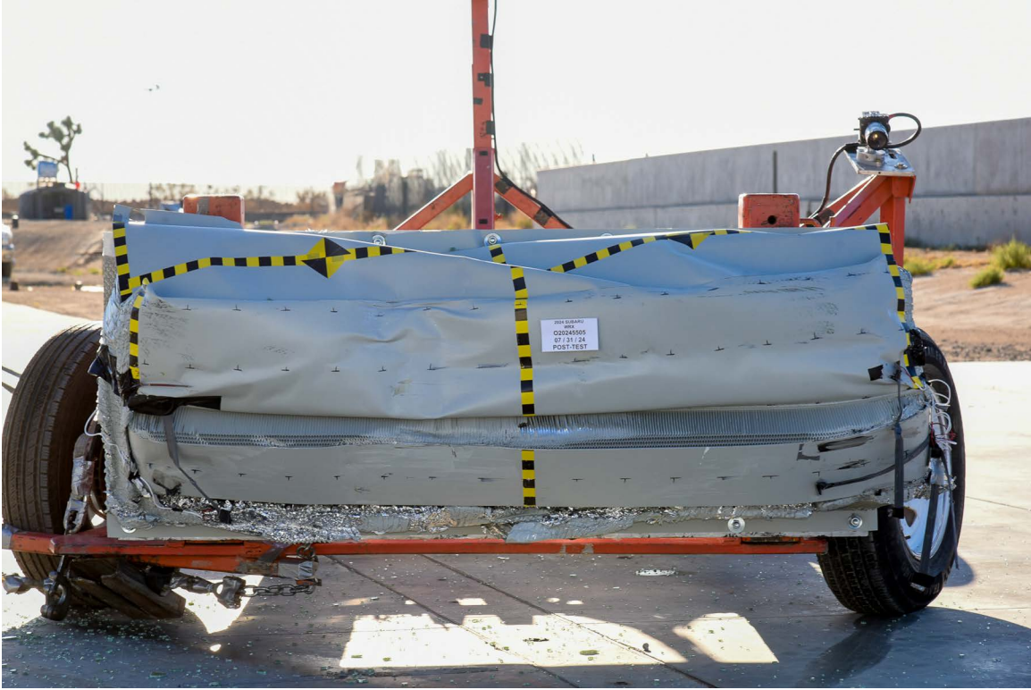
FIGURE 85. Post-Test Front View of MDB Impactor Face
