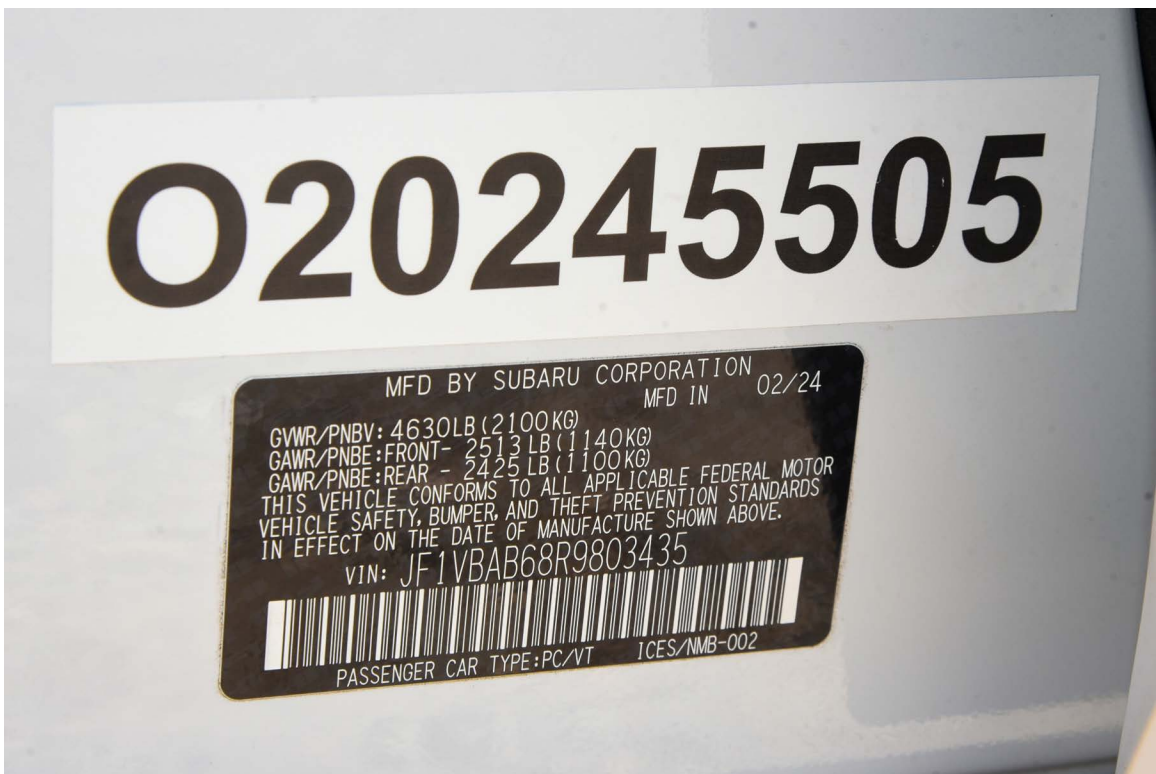
FIGURE 92. Close-Up View of Vehicle's Certification Label
