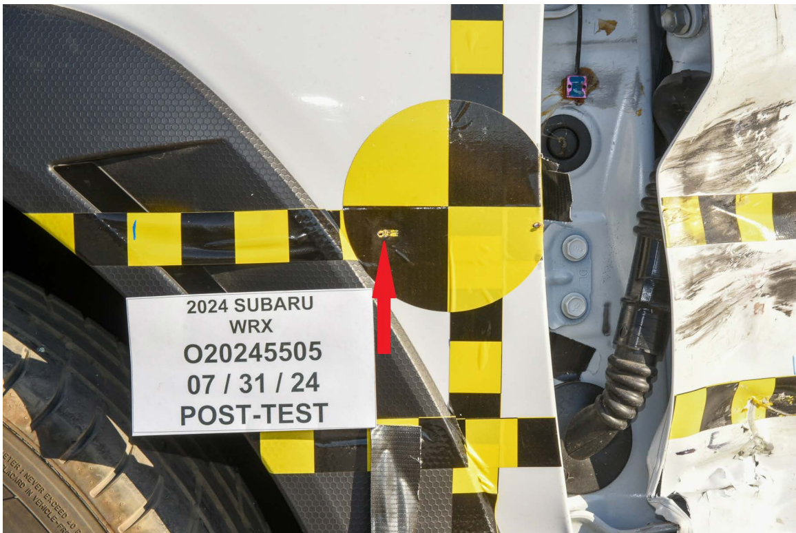
FIGURE 20. Post-Test Close-Up View of Impact Point Target
