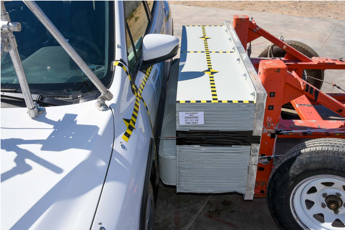
FIGURE 17. Pre-Test Left Side View of MDB Positioned Against Side of Test Vehicle
