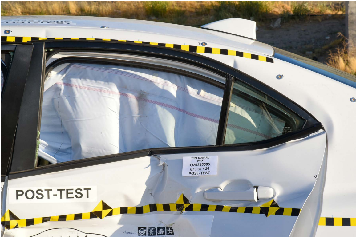
FIGURE 57. Post-Test Left Side View of Rear Passenger Dummy Shoulder and Door Top View
