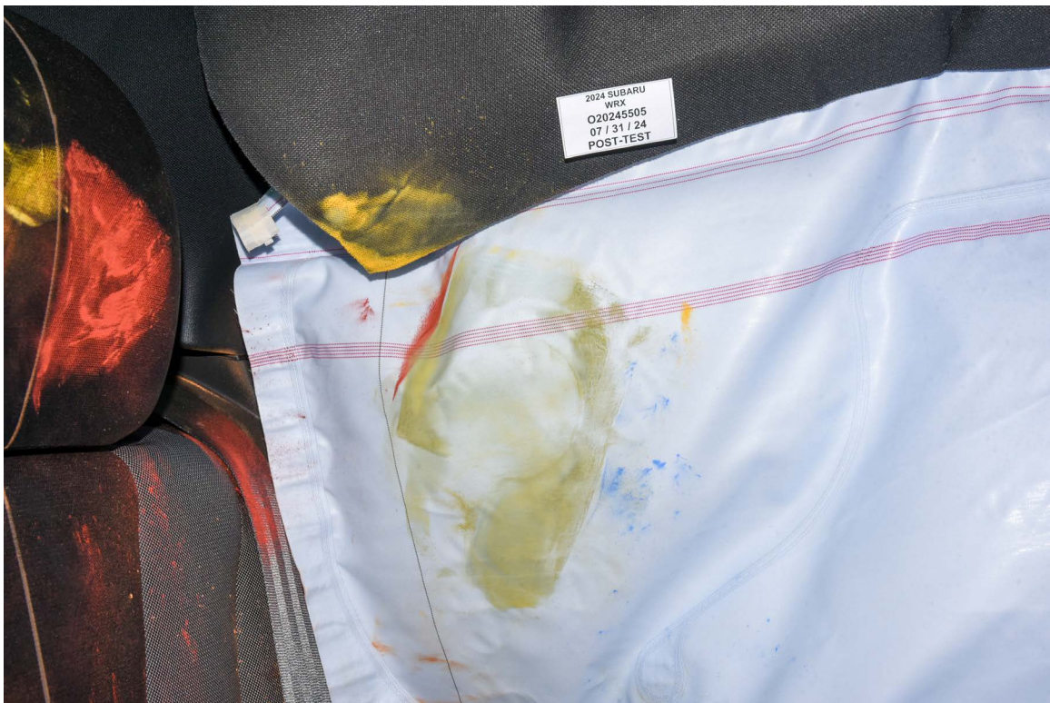
FIGURE 76. Post-Test Rear Passenger Dummy Close-Up Head Contact with Side Air Bag View
