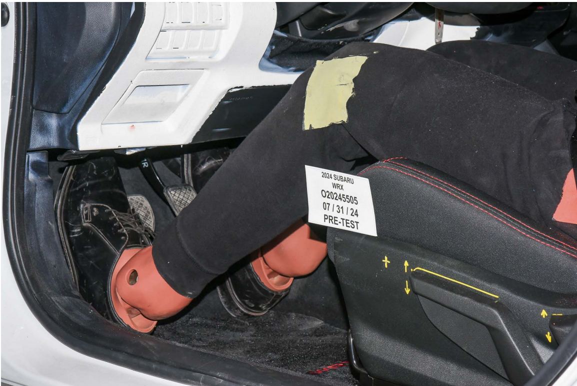
FIGURE 34. Pre-Test Placement of Driver Dummy's Feet
