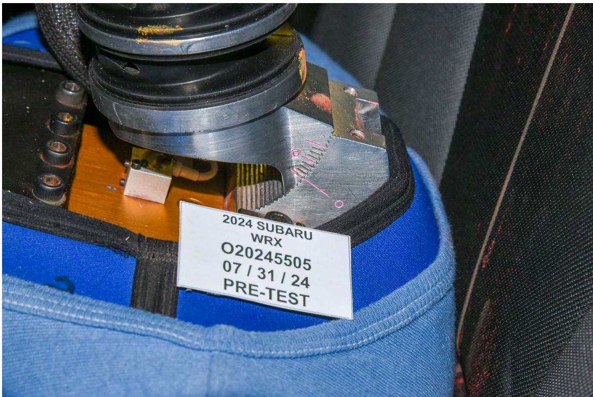
FIGURE 62. Pre-Test View of Rear Passenger Dummy's Neck Showing Position of Adjustable Neck Bracket
