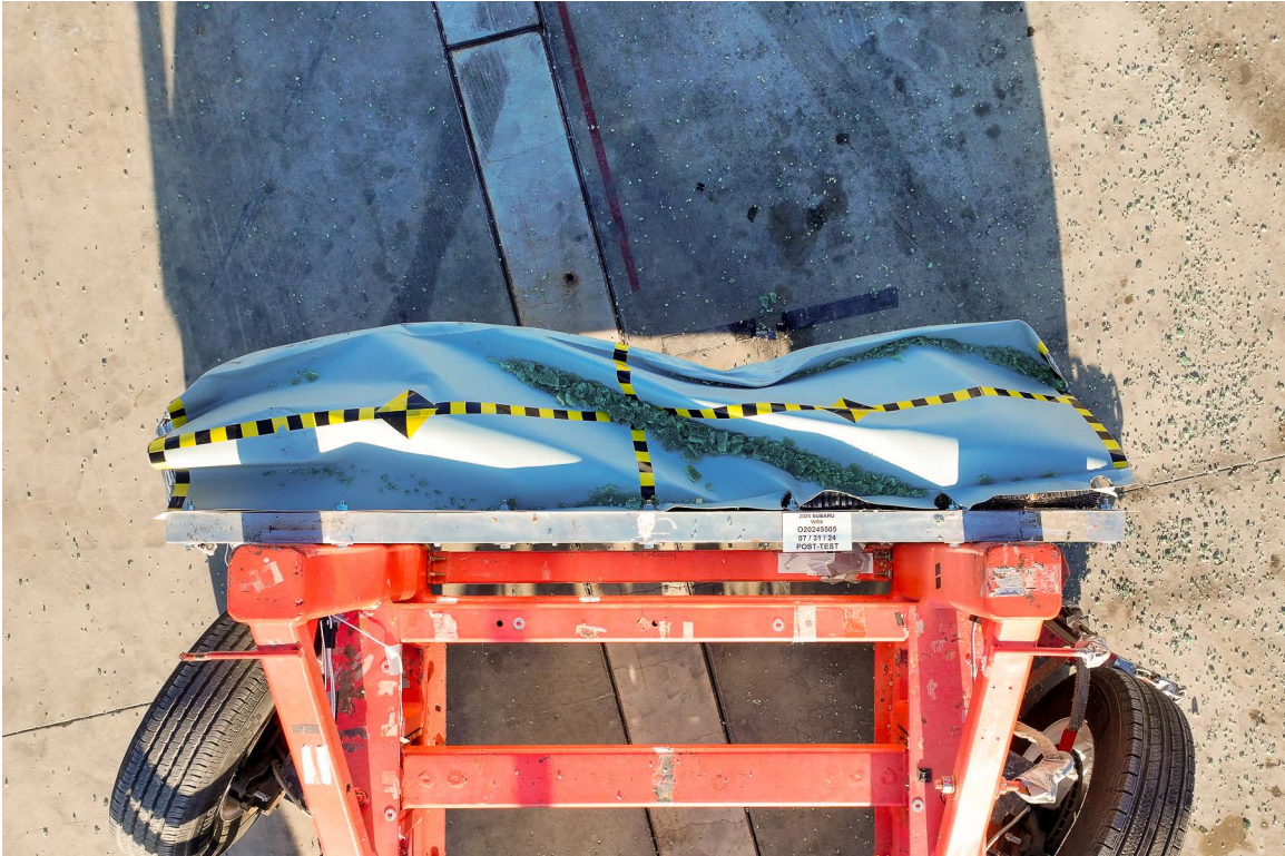
FIGURE 87. Post-Test Top View of MDB Impactor Face
