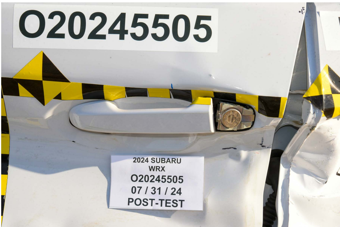
FIGURE 22. Post-Test Left Front Door Latch Close-Up
