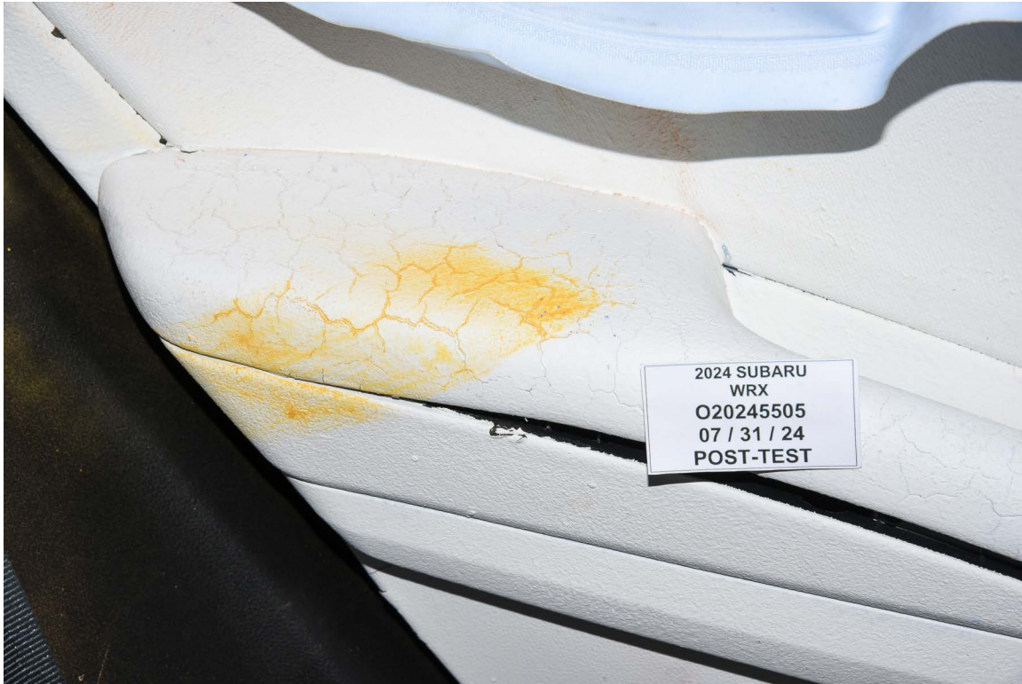
FIGURE 77. Post-Test Rear Passenger Dummy Close-Up Torso Contact with Vehicle Interior View
