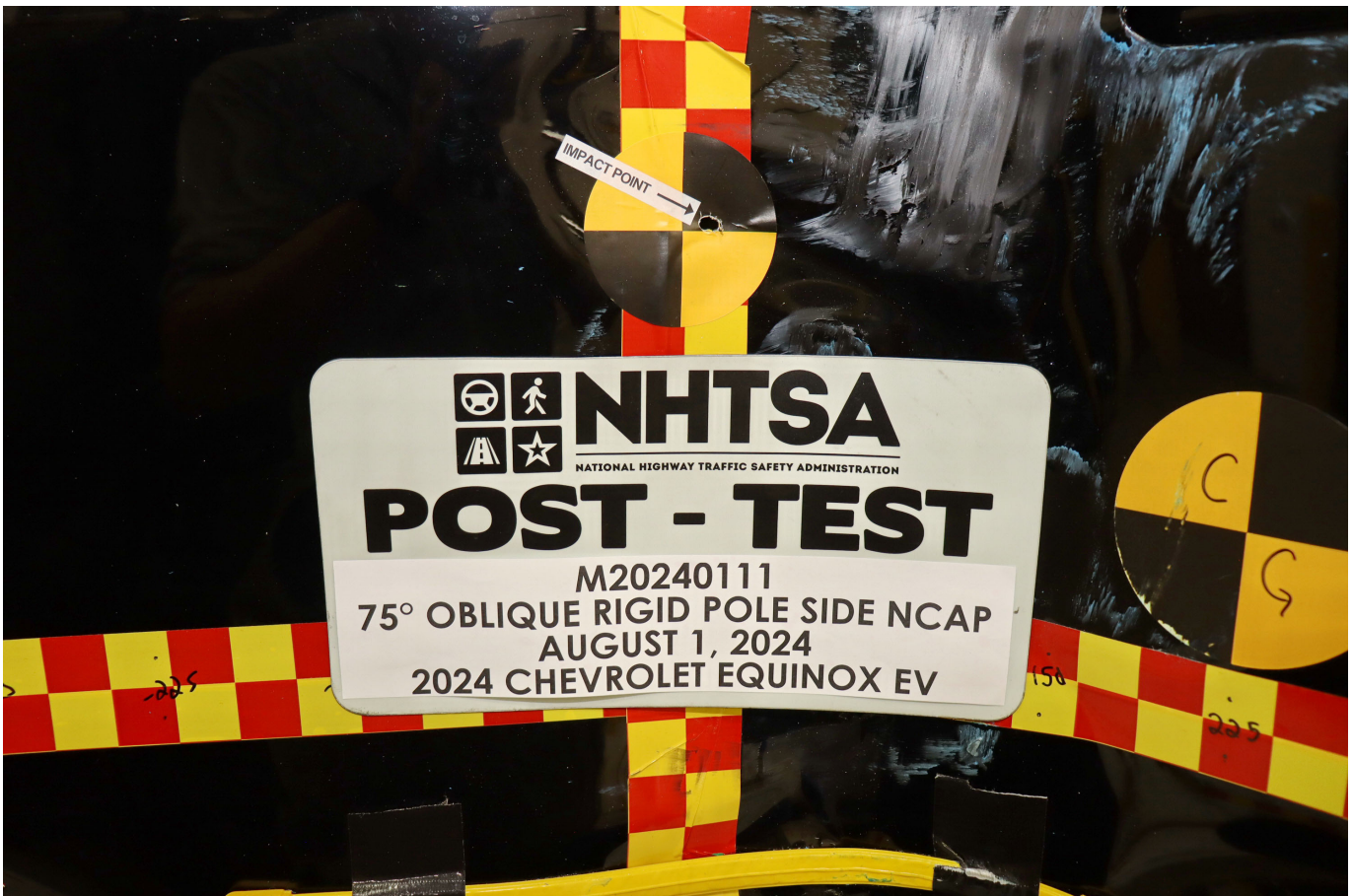
Photo No. 020 - Post-Test Close-Up View of Impact Point Target Showing Impact Location
