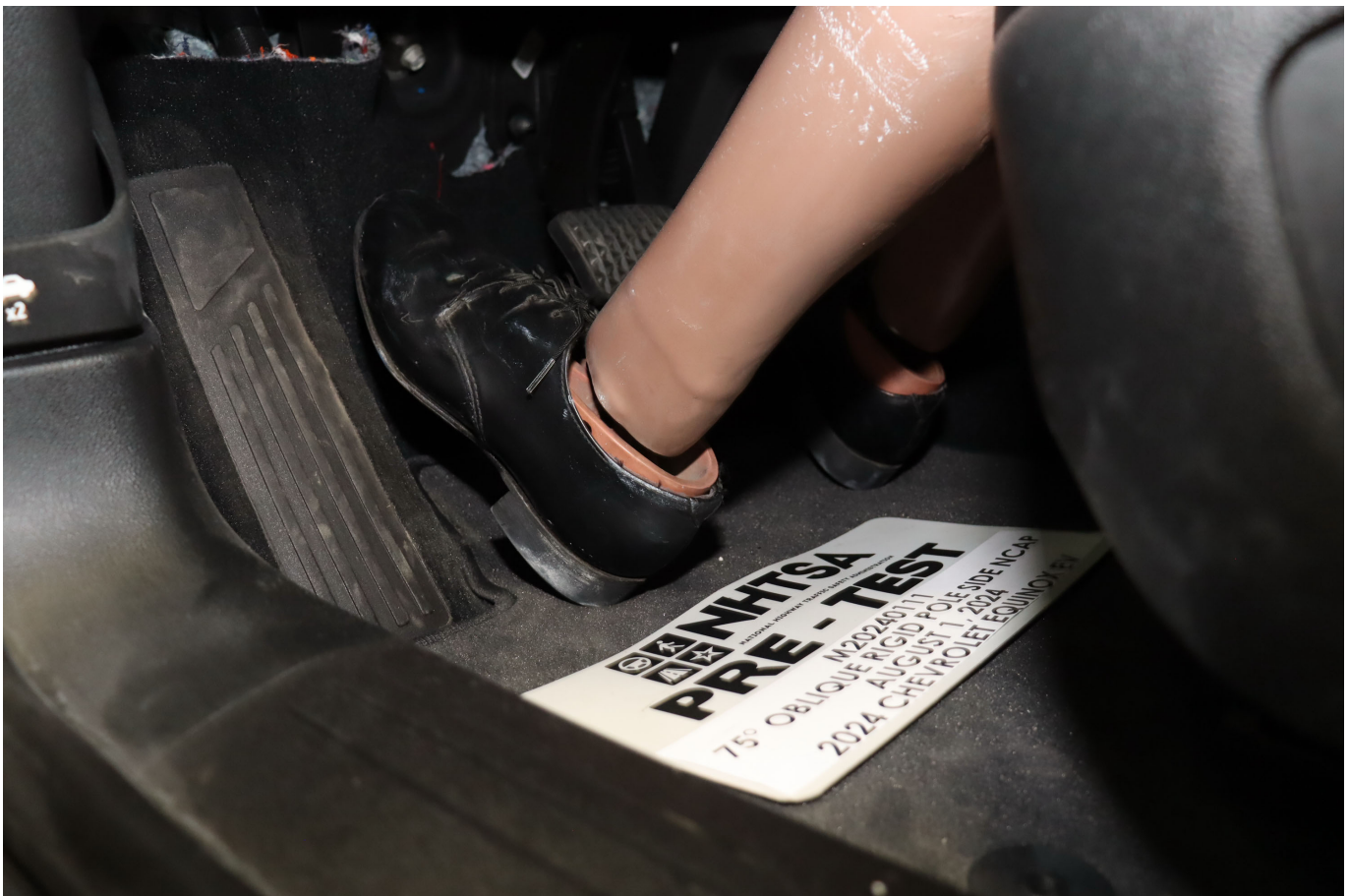
Photo No. 032 - Pre-Test Placement of Dummy's Feet
