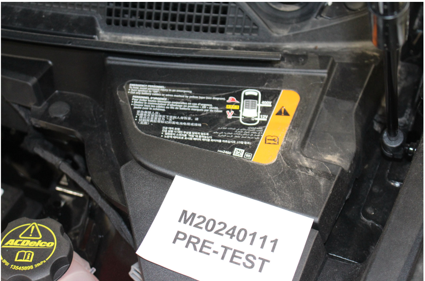
Photo No. 305-03 - First Responder Warning Label
