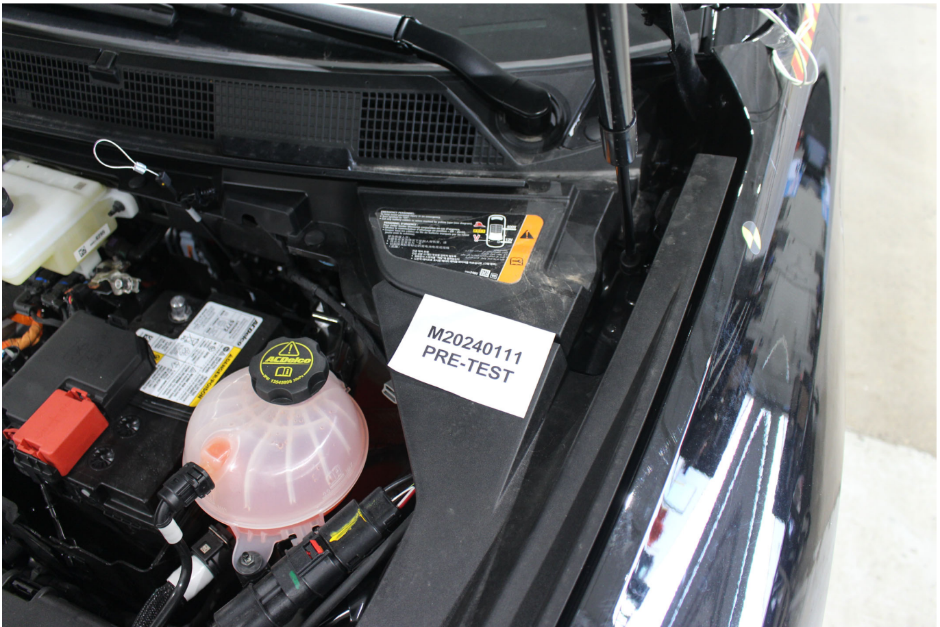
Photo No. 305-04 - First Responder Warning Location
