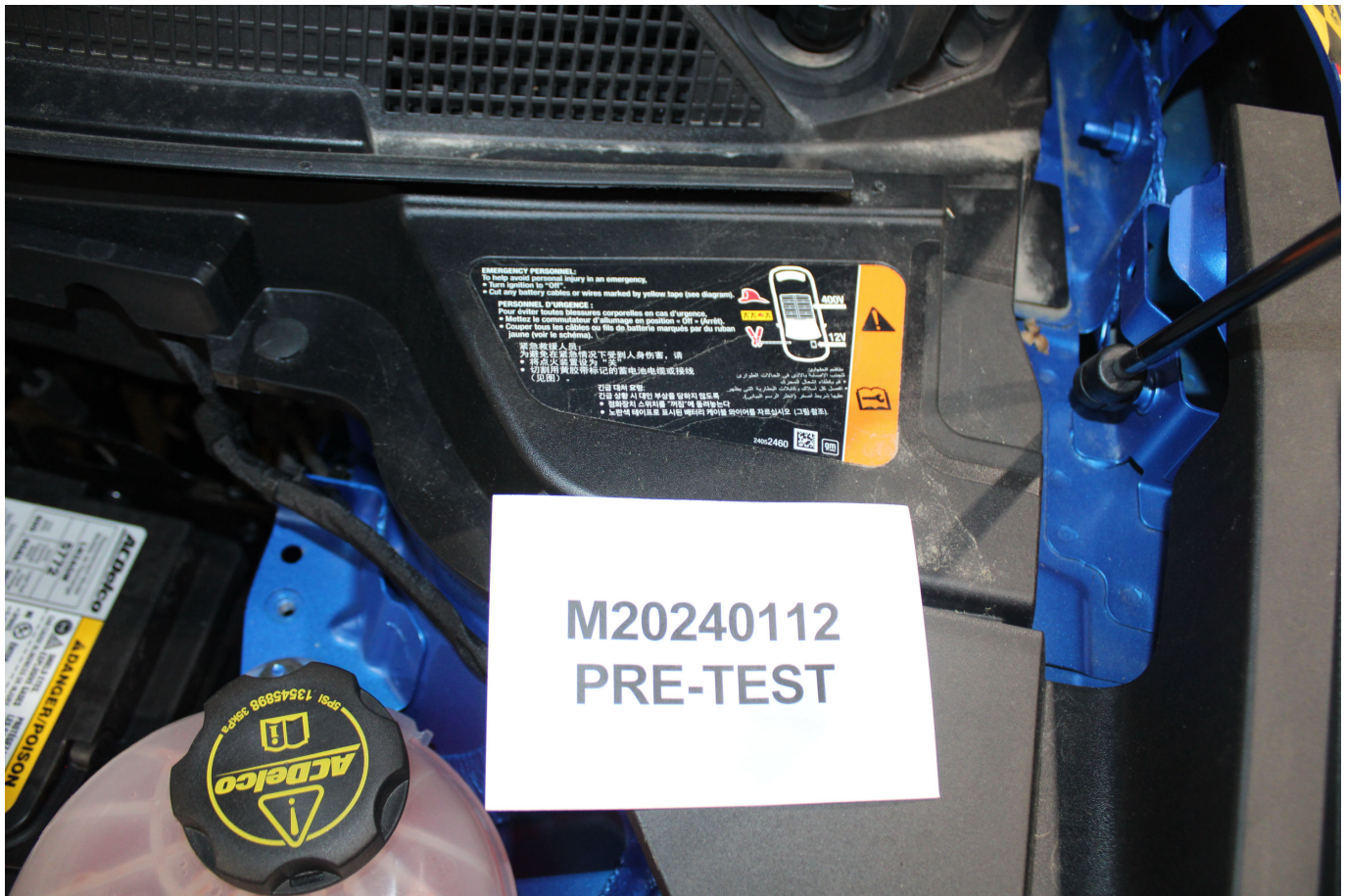
Photo No. 305-03 - First Responder Warning Label
