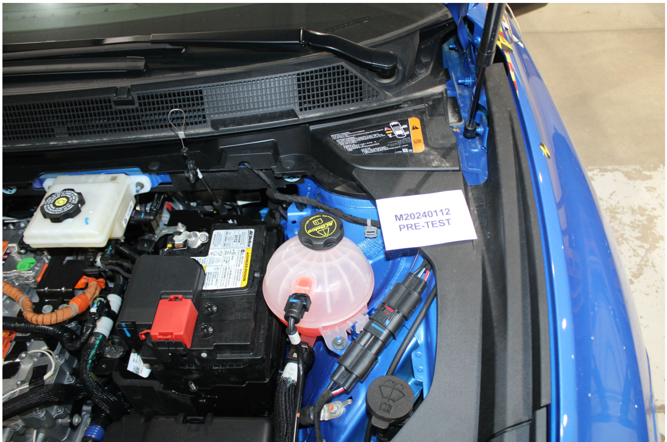
Photo No. 305-04 - First Responder Warning Location
