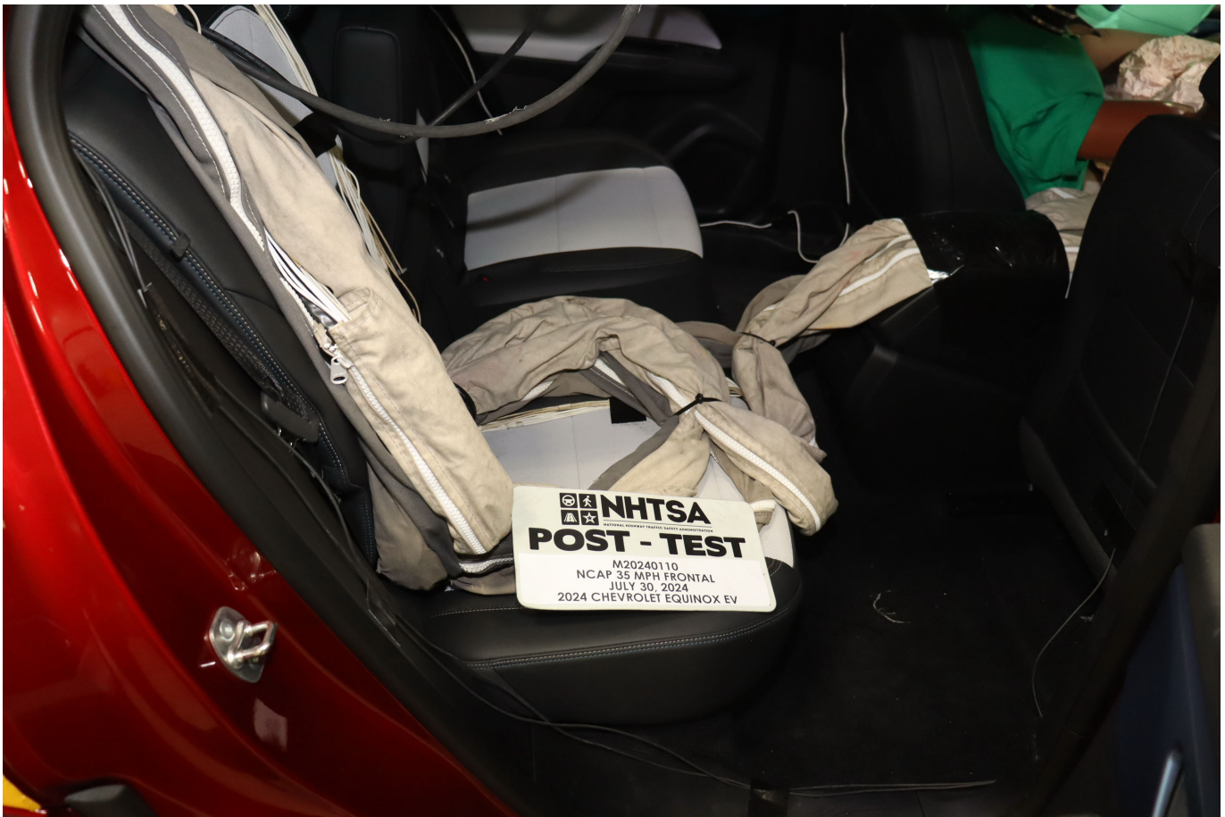
Photo No. 029 - Post-Test Dummy Cable Routing
