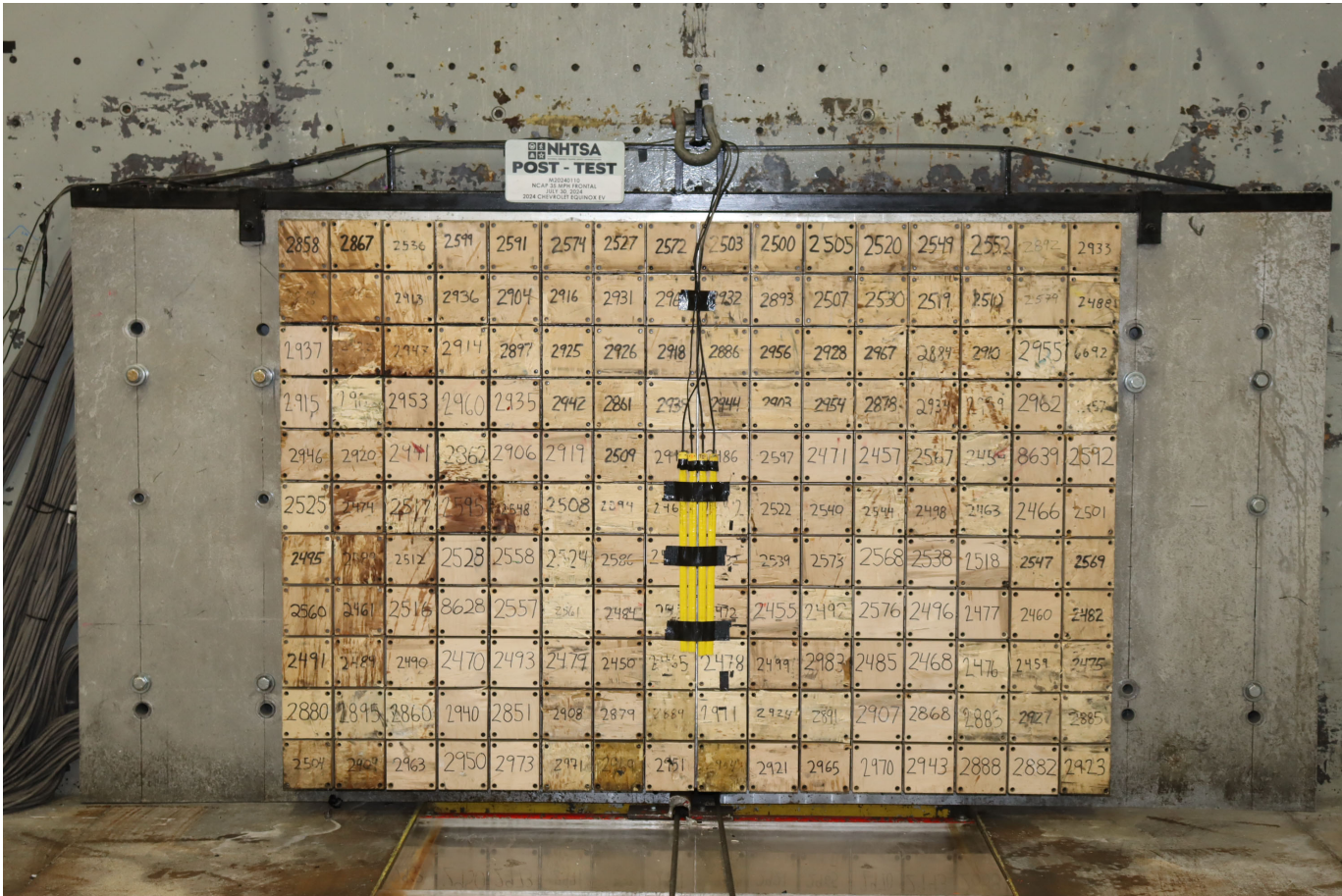
Photo No. 003 - Post-Test Load Cell Wall
