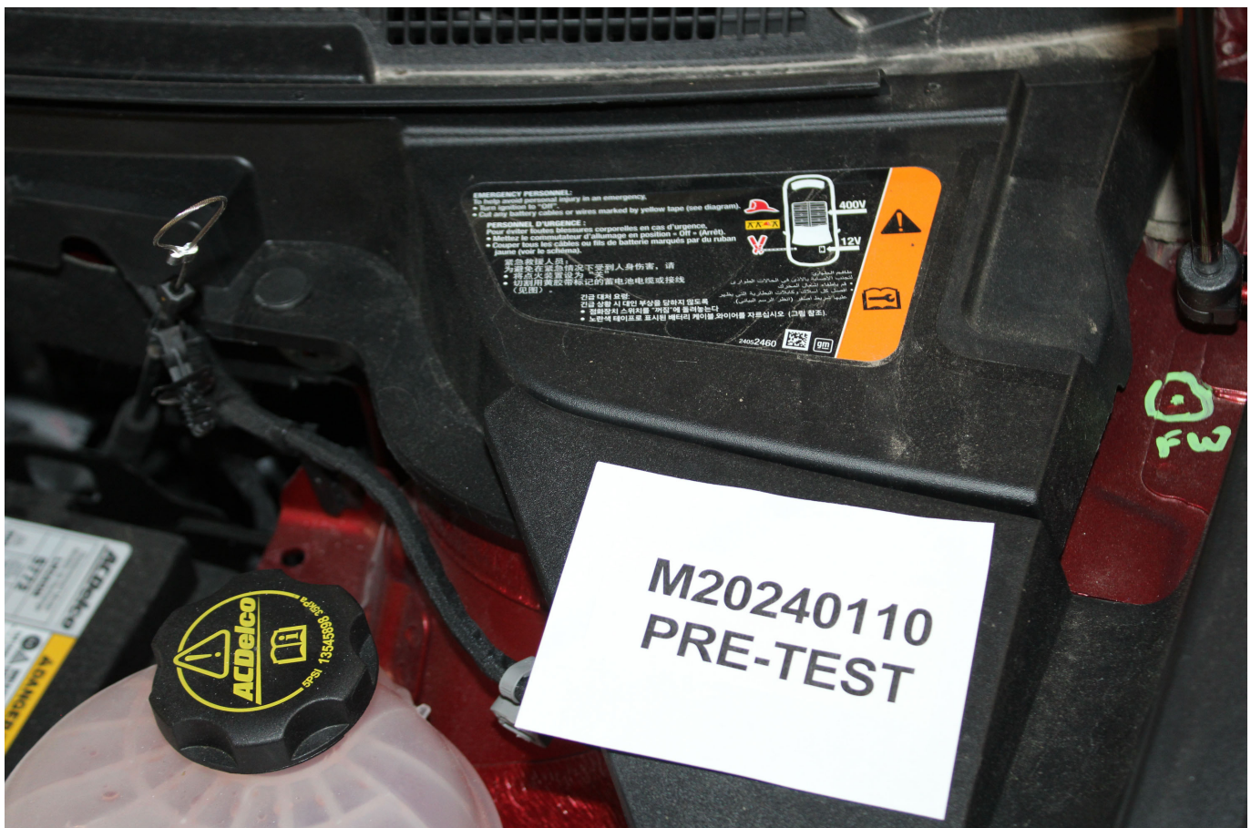
Photo No. 305-03 - First Responder Warning Label
