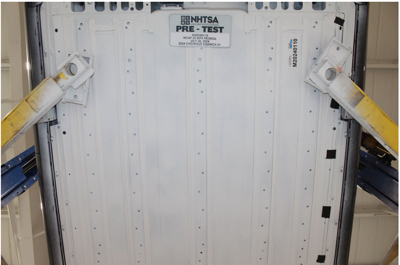
Photo No. 305-09 - Pre-Impact View of Propulsion Battery
