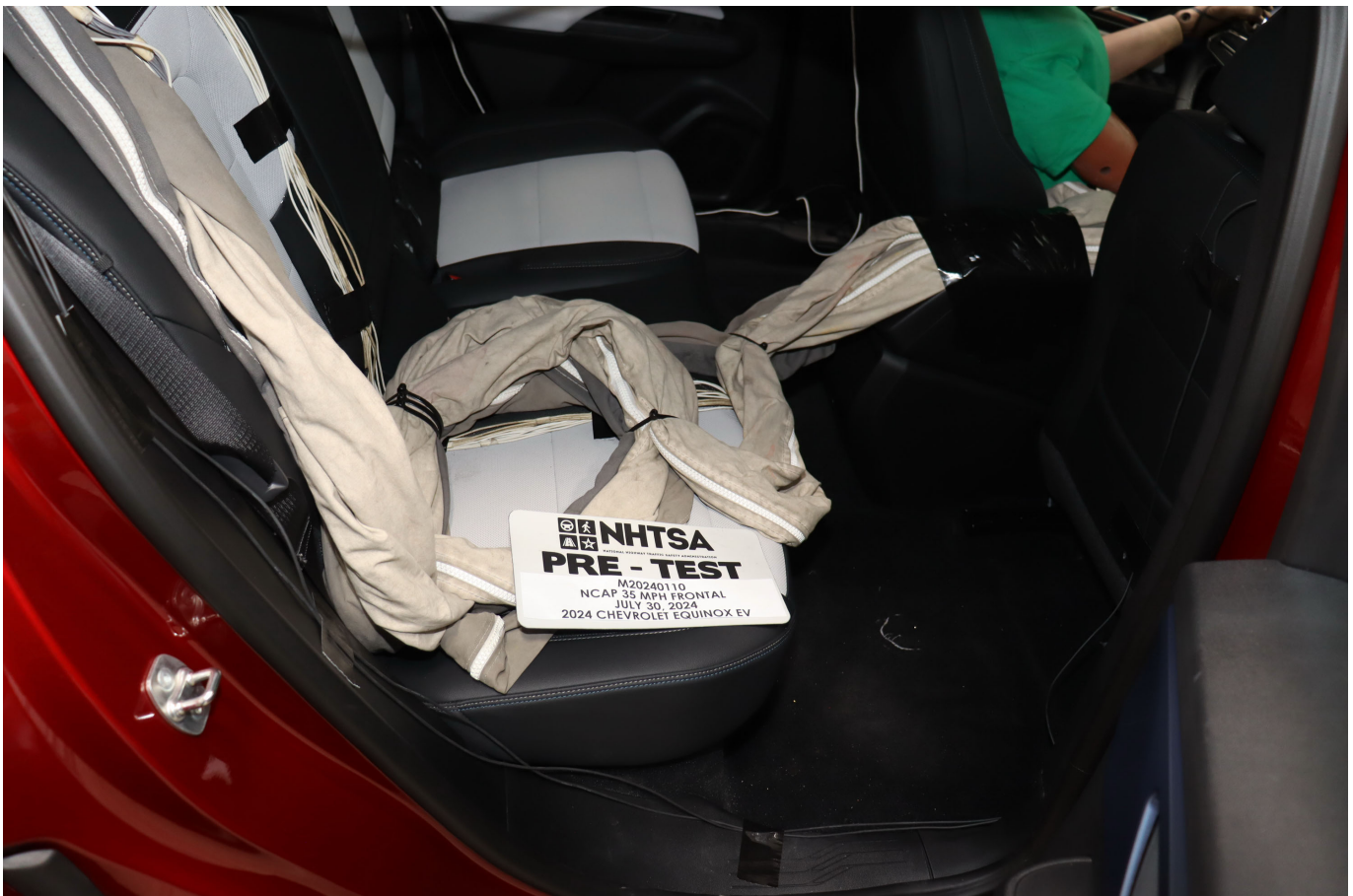
Photo No. 028 - Pre-Test Dummy Cable Routing
