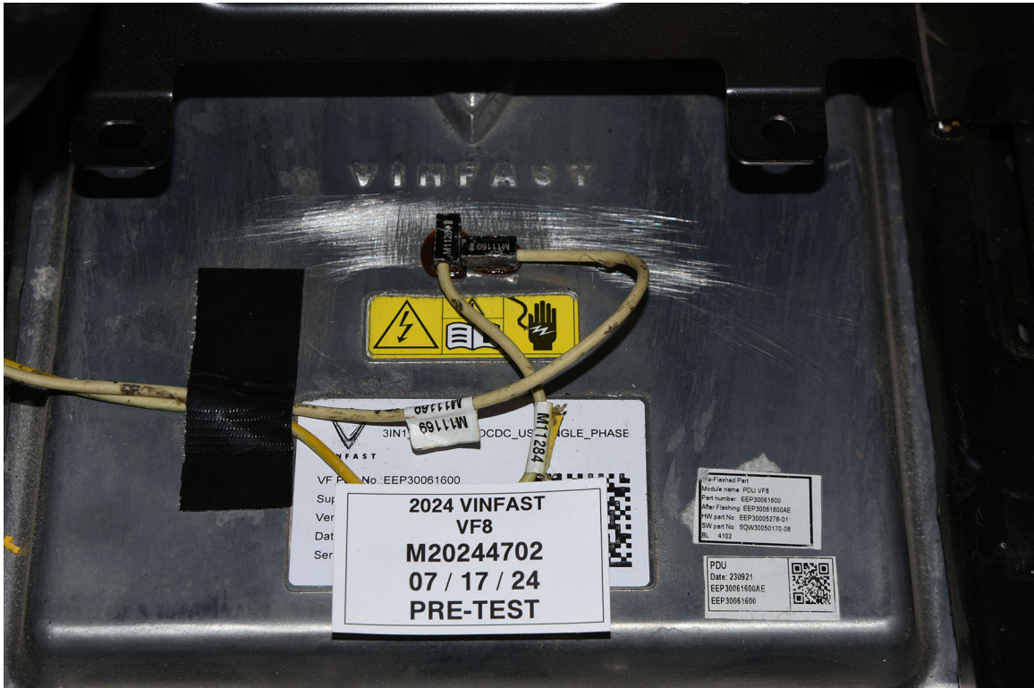
FIGURE 305-01 Auxiliary Power Module Warning Label
