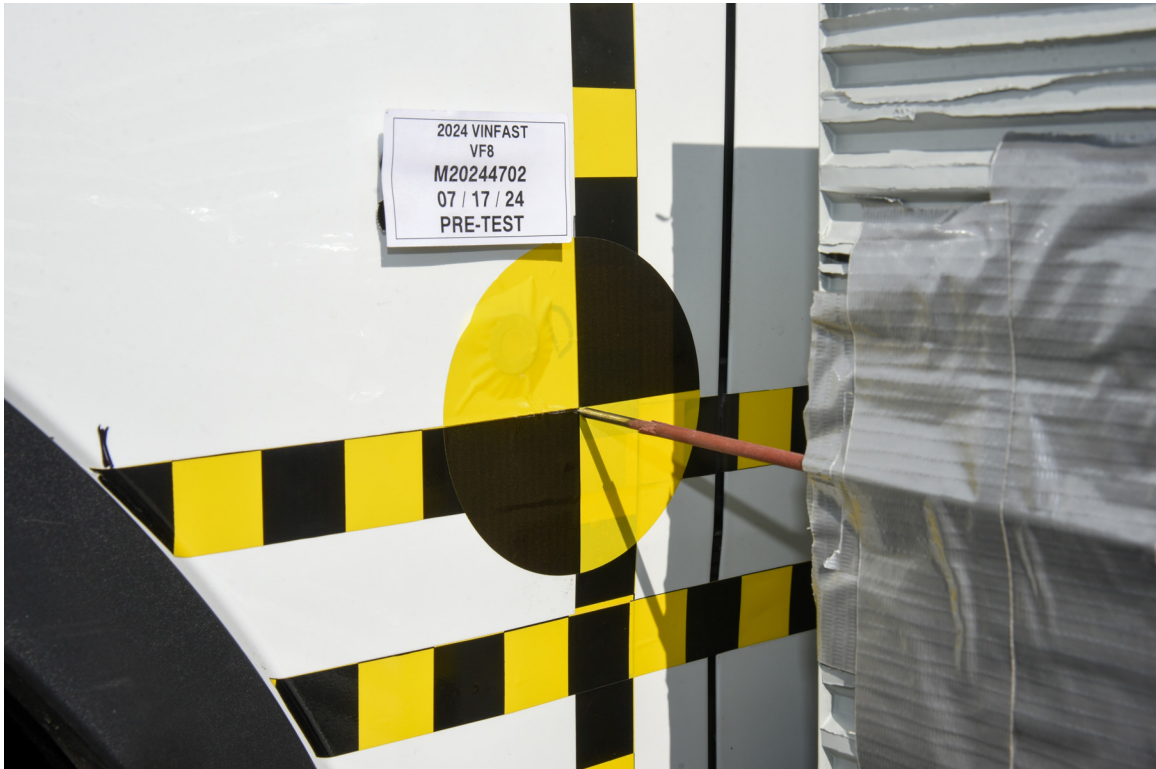
FIGURE 19. Pre-Test Close-Up View of Impact Point Target
