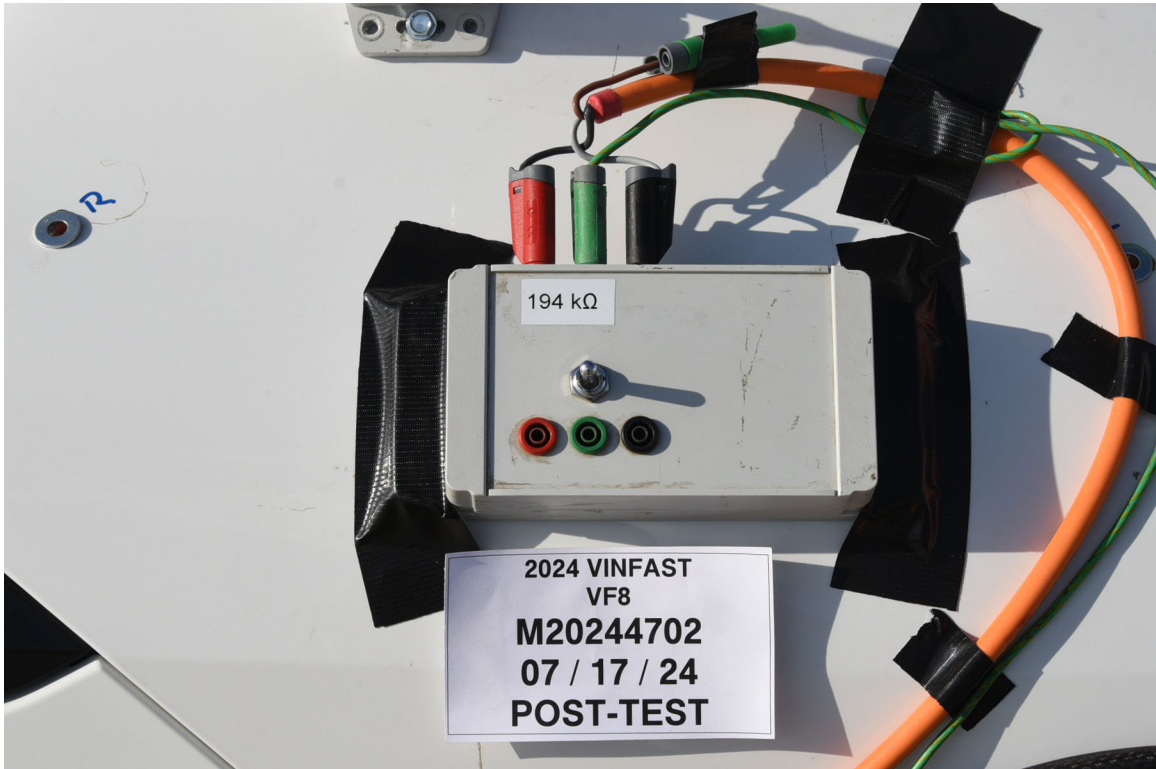
FIGURE 305-025 Post-Impact View of Installed Test Interface Port
