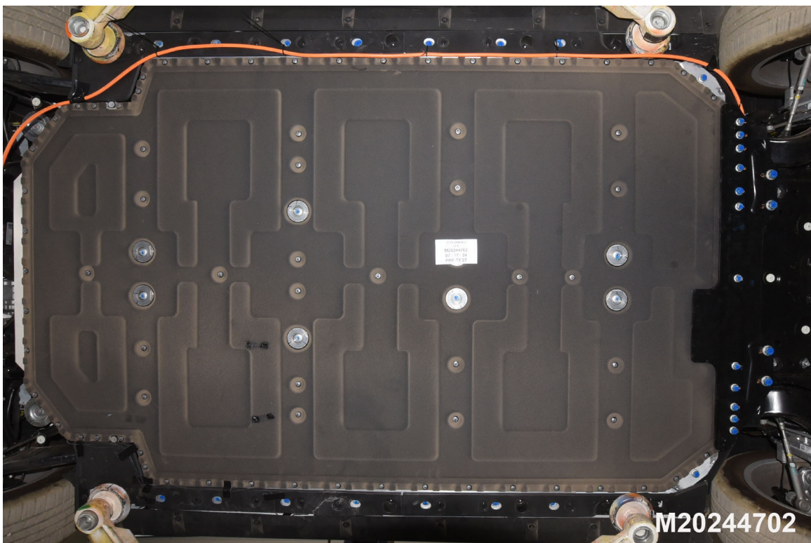
FIGURE 305-012 Pre-Impact View of Battery Box(s) or Container(s) Which Holds Individual Battery Modules
