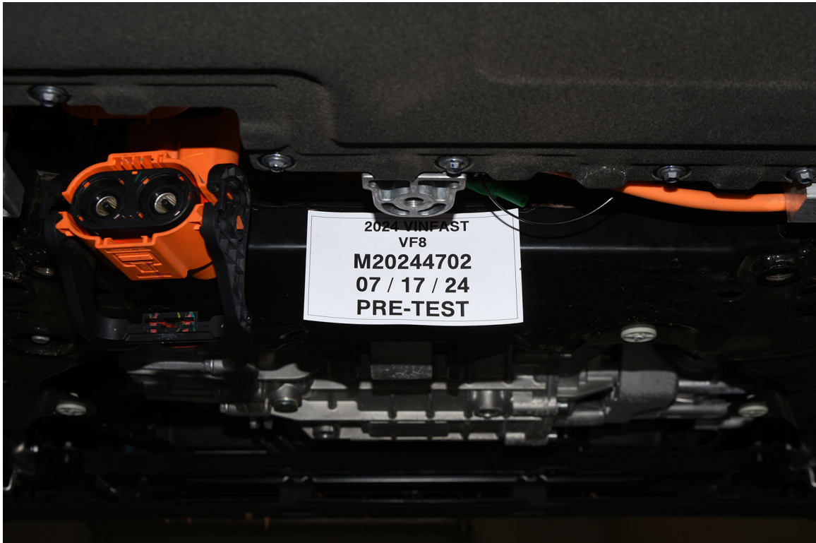
FIGURE 305-07 Manual High Voltage Service Disconnect Removed
