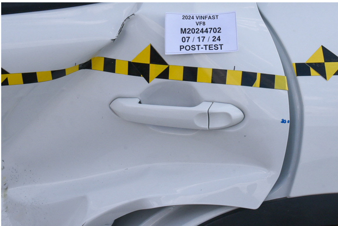
FIGURE 24. Post-Test Left Rear Door Latch Close-Up
