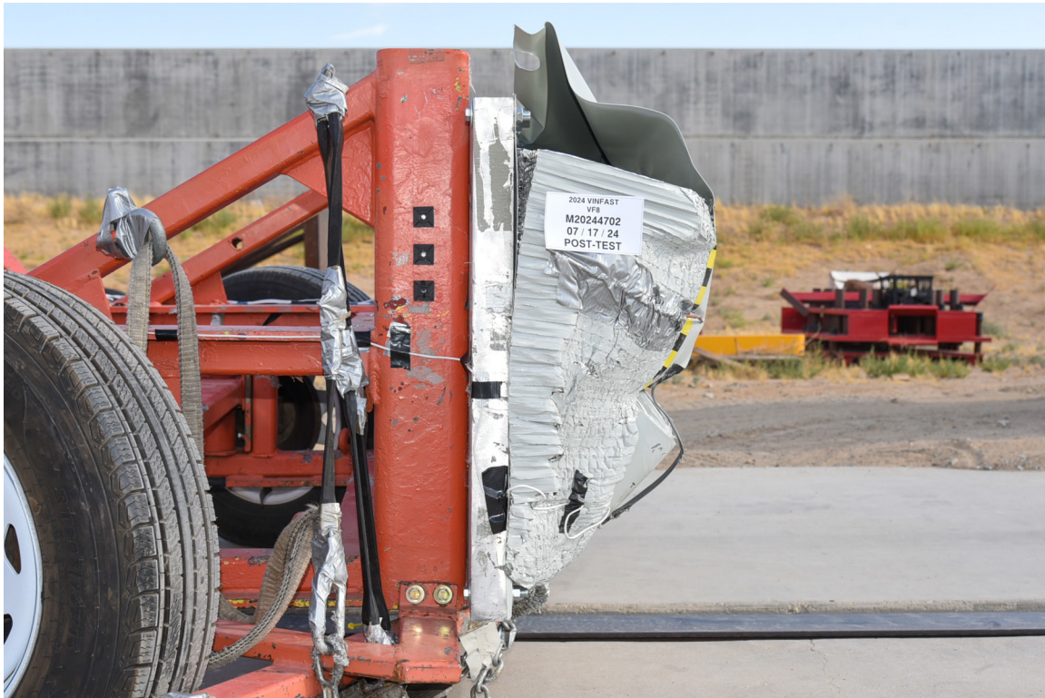
FIGURE 91. Post-Test Right View of MDB Impactor Face
