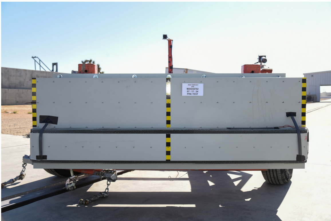
FIGURE 84. Pre-Test Front View of MDB Impactor Face
