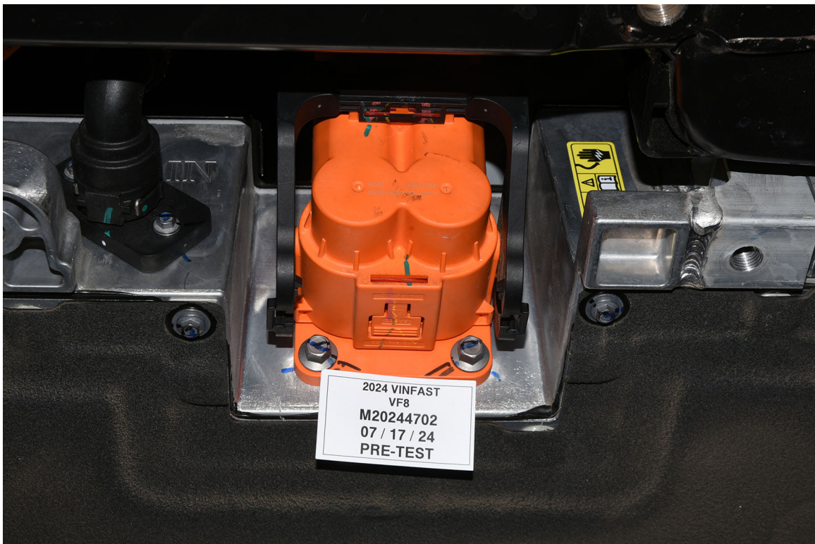
FIGURE 305-06 Manual High Voltage Service Disconnect in Place
