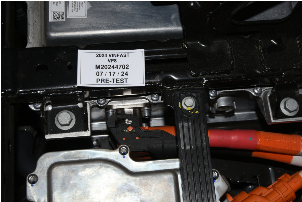
FIGURE 305-019 Pre-Impact View Propulsion Battery Venting System(s)
