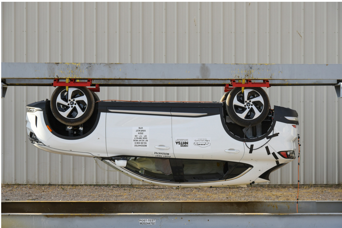
FIGURE 98. FMVSS No. 301 Static Rollover 180 Degrees
