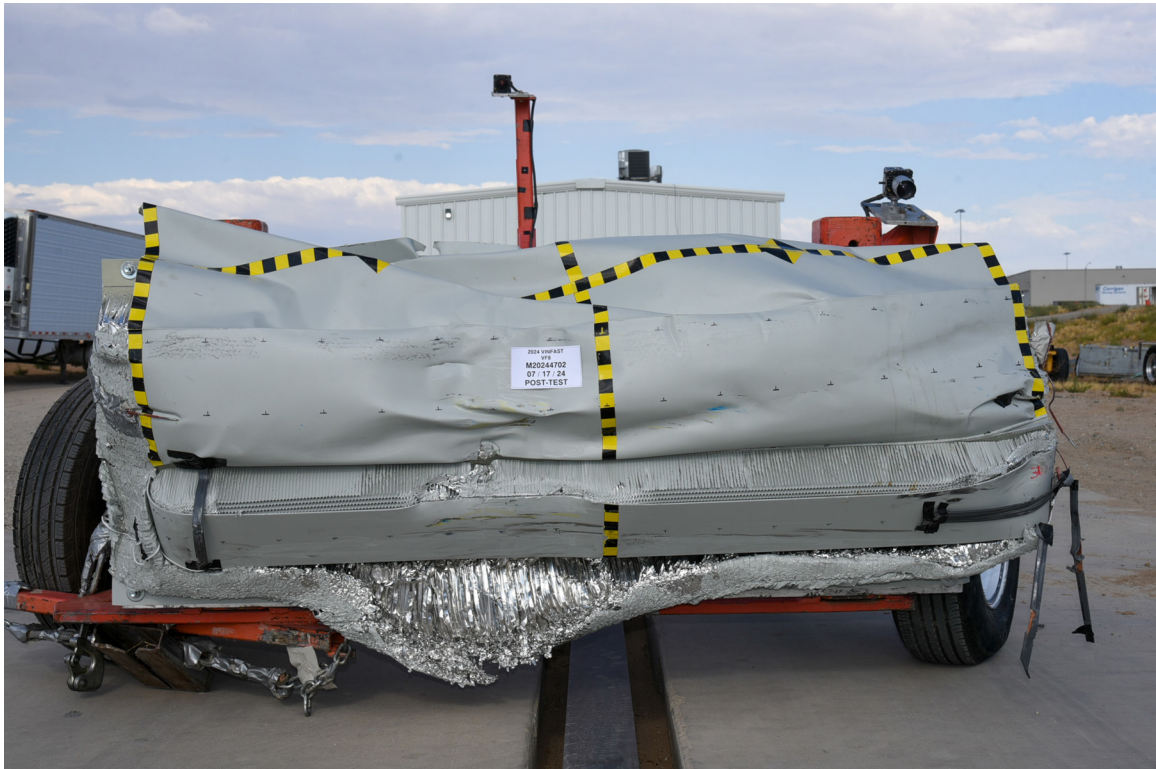
FIGURE 85. Post-Test Front View of MDB Impactor Face
