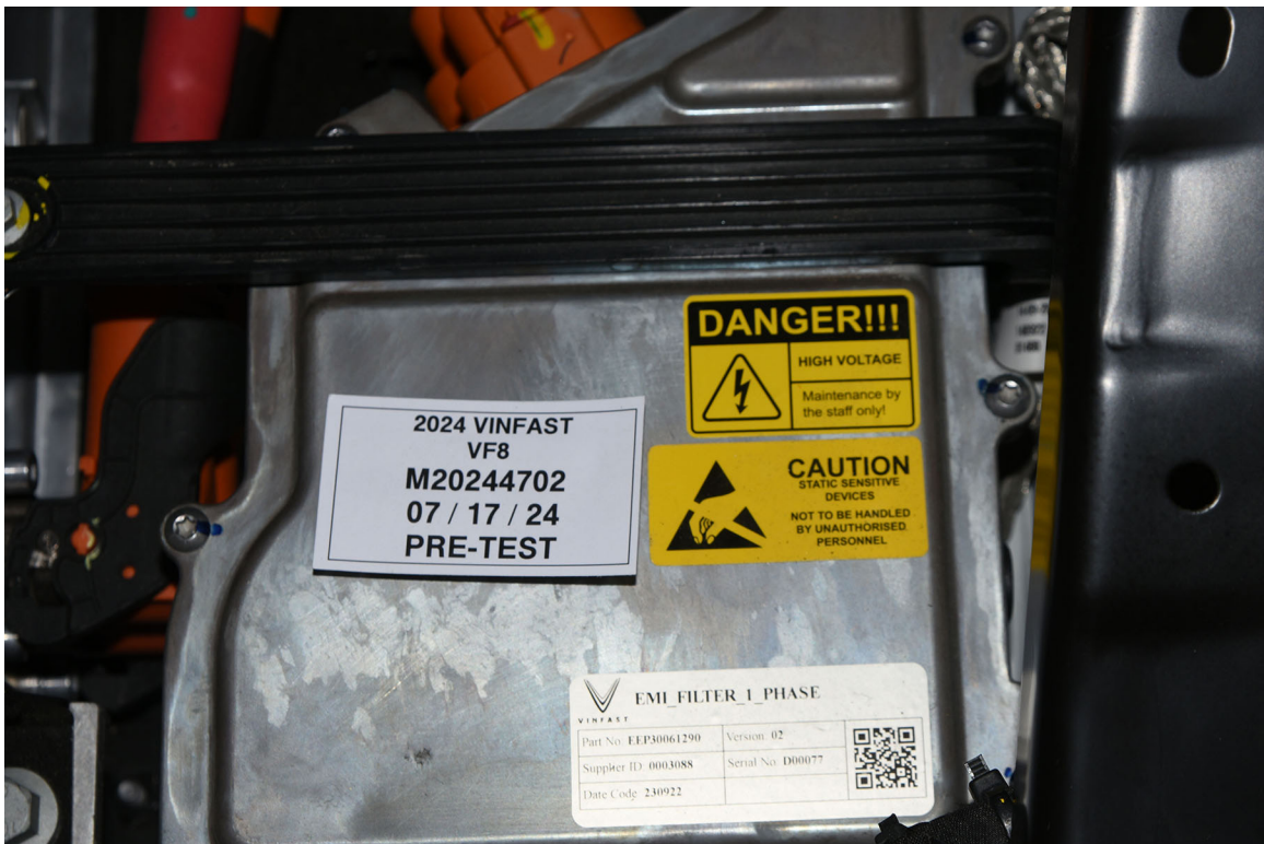
FIGURE 305-02 Power Inverter Warning Label
