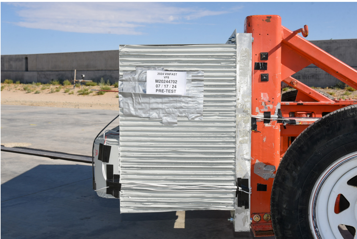
FIGURE 88. Pre-Test Left View of MDB Impactor Face
