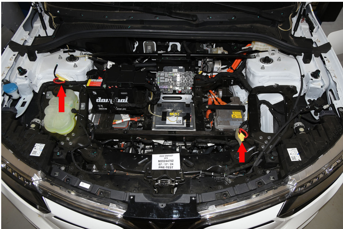
FIGURE 305-04 First Responder Warning Location
