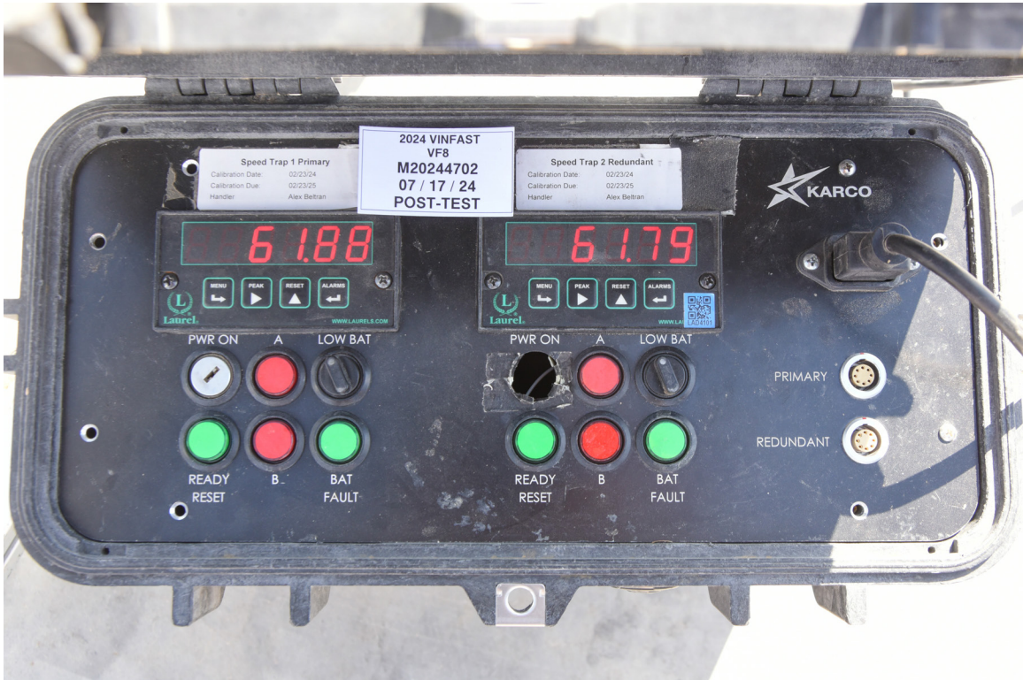
FIGURE 95. Post-Test Primary and Redundant Speed Trap Read-Out
