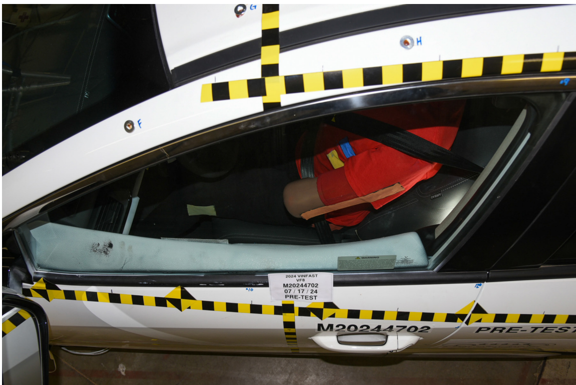
FIGURE 42. Pre-Test Driver Dummy and Door Clearance View
