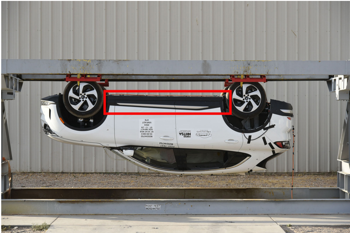
FIGURE 305-029 FMVSS No. 305 Static Rollover at 180°
