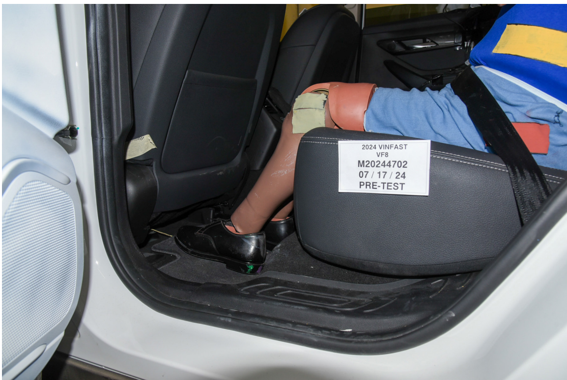
FIGURE 64. Pre-Test Placement of Rear Passenger Dummy's Feet
