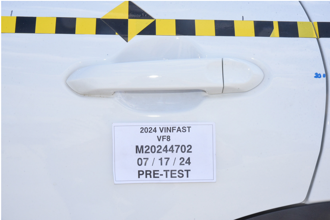
FIGURE 23. Pre-Test Left Rear Door Latch Close-Up
