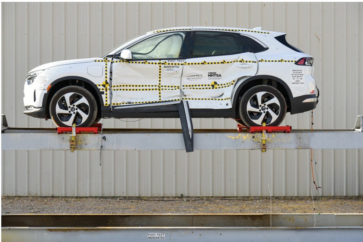
FIGURE 96. FMVSS No. 301 Static Rollover 0 Degrees
