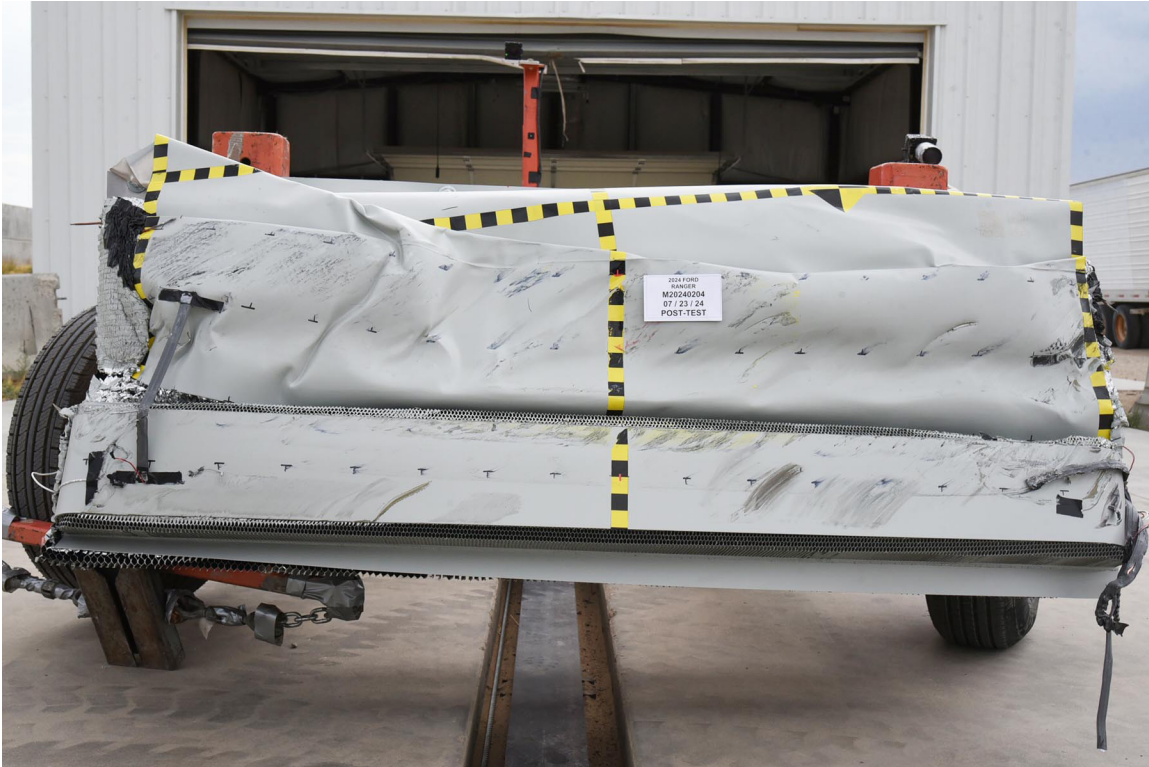
FIGURE 85. Post-Test Front View of MDB Impactor Face
