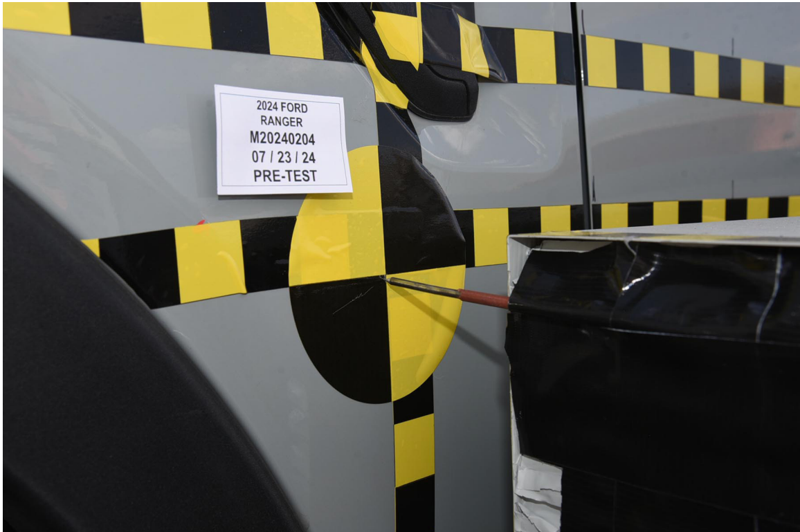
FIGURE 19. Pre-Test Close-Up View of Impact Point Target
