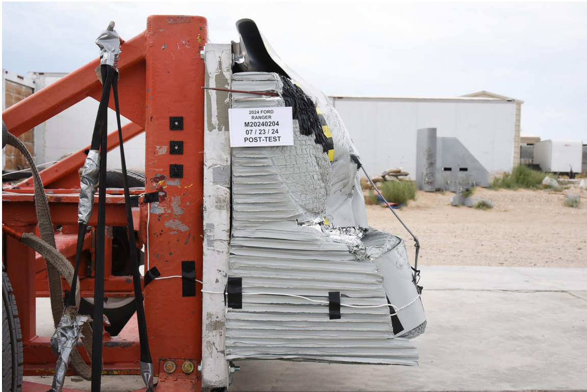
FIGURE 91. Post-Test Right View of MDB Impactor Face
