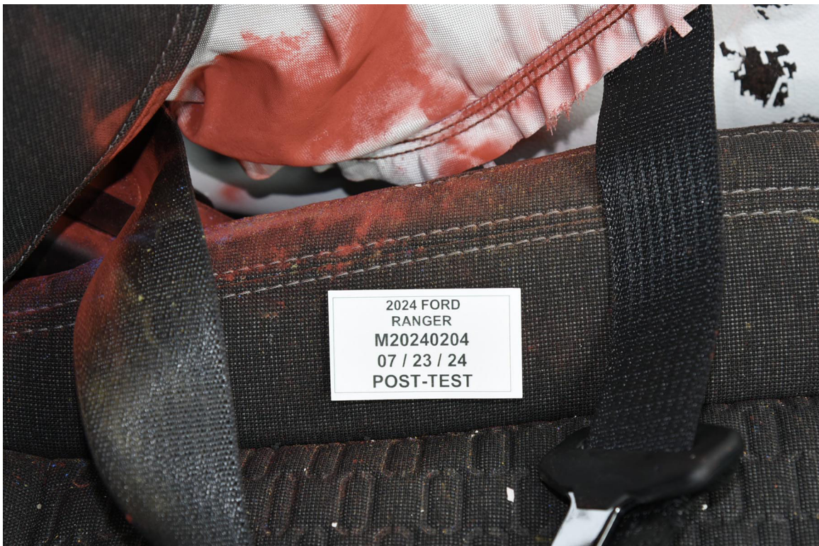
FIGURE 52. Post-Test Driver Dummy Close-Up Pelvis Contact With Vehicle Interior View
