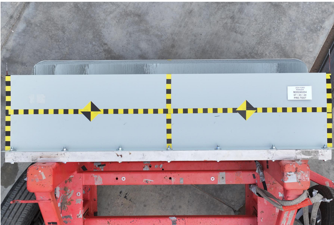
FIGURE 86. Pre-Test Top View of MDB Impactor Face
