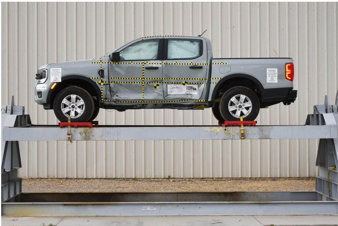
FIGURE 96. FMVSS No. 301 Static Rollover 0 Degrees
