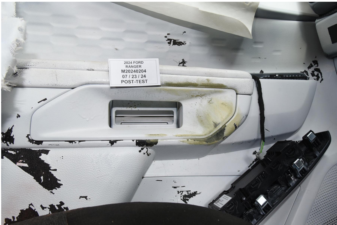
FIGURE 54. Post-Test Driver Dummy Close-Up Knee Contact View
