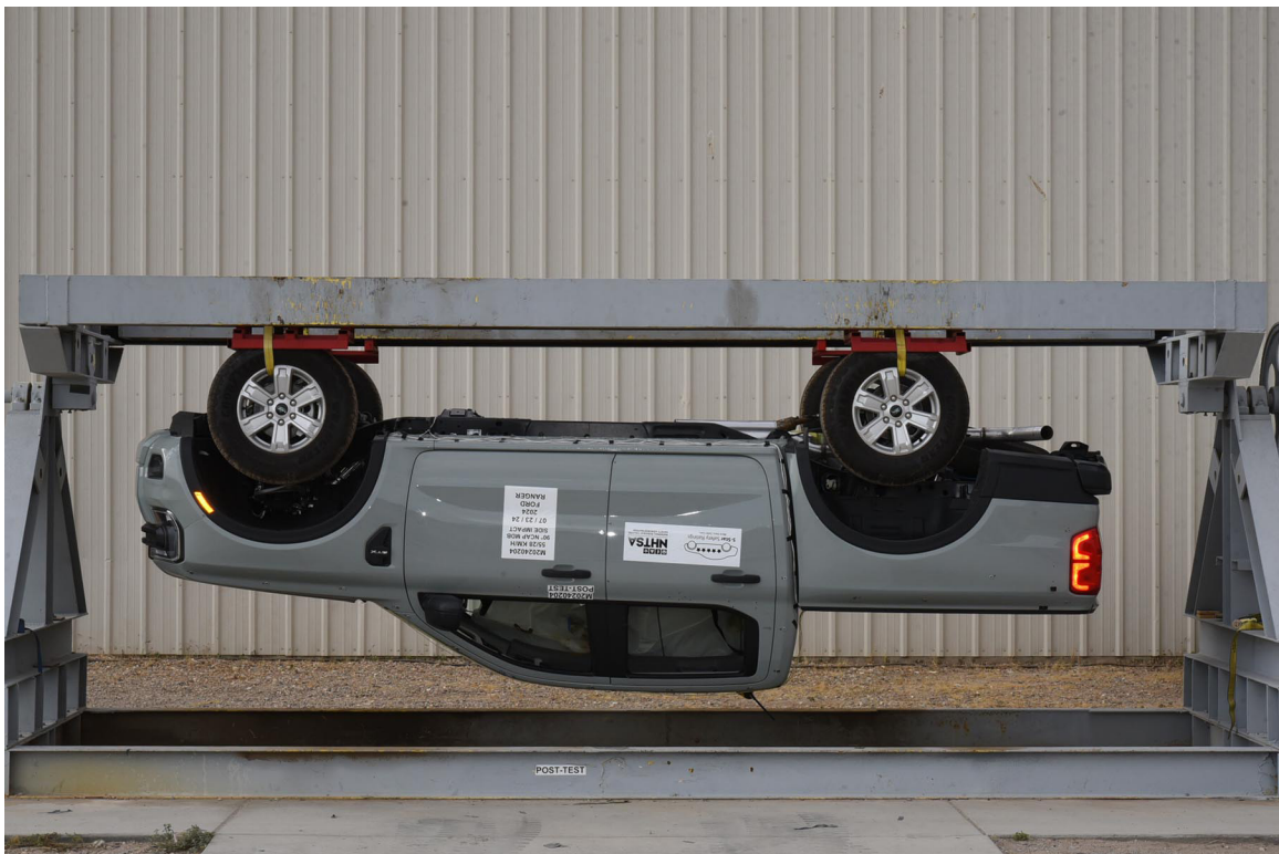
FIGURE 98. FMVSS No. 301 Static Rollover 180 Degrees
