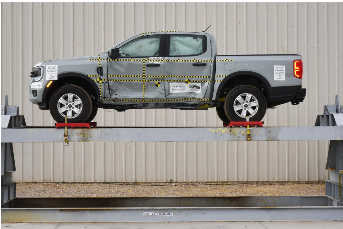
FIGURE 100. FMVSS No. 301 Static Rollover 360 Degrees
