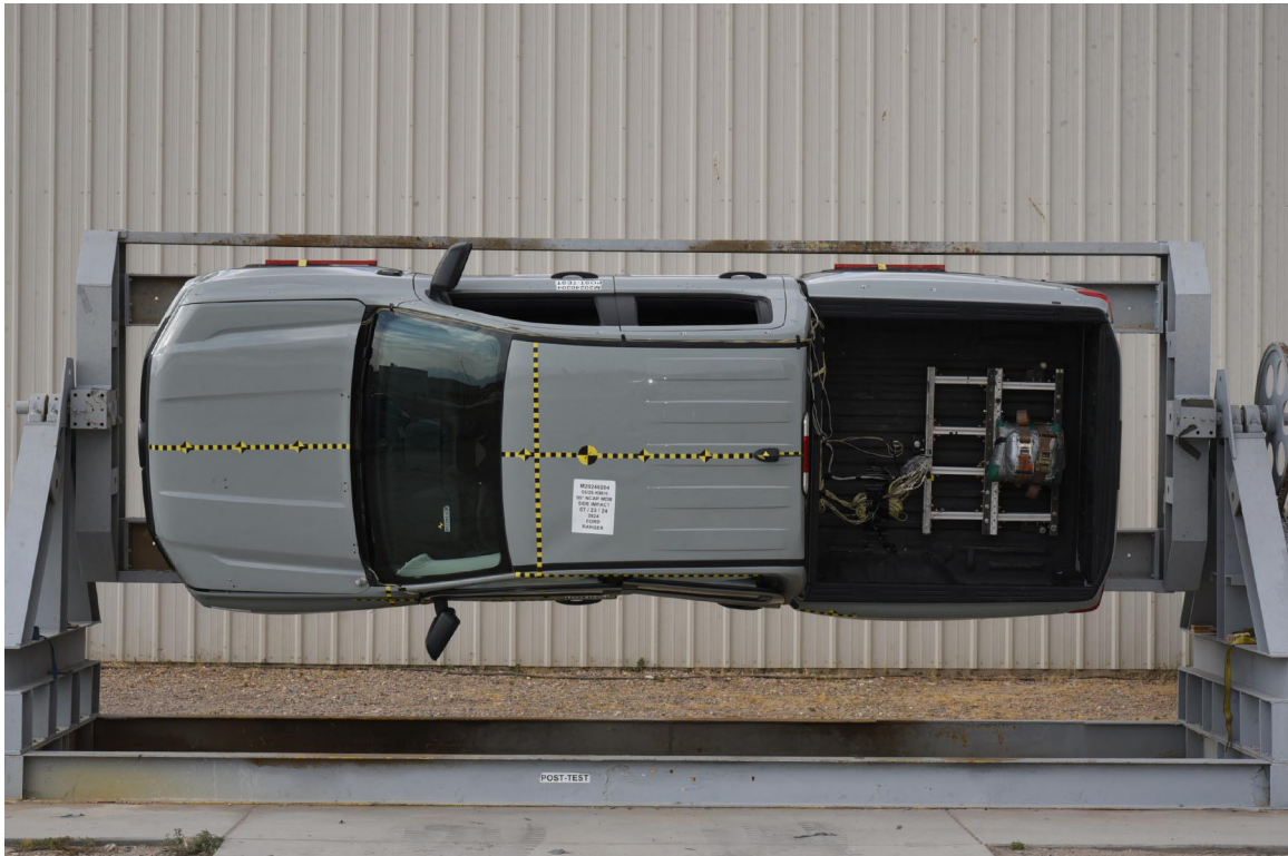
FIGURE 97. FMVSS No. 301 Static Rollover 90 Degrees
