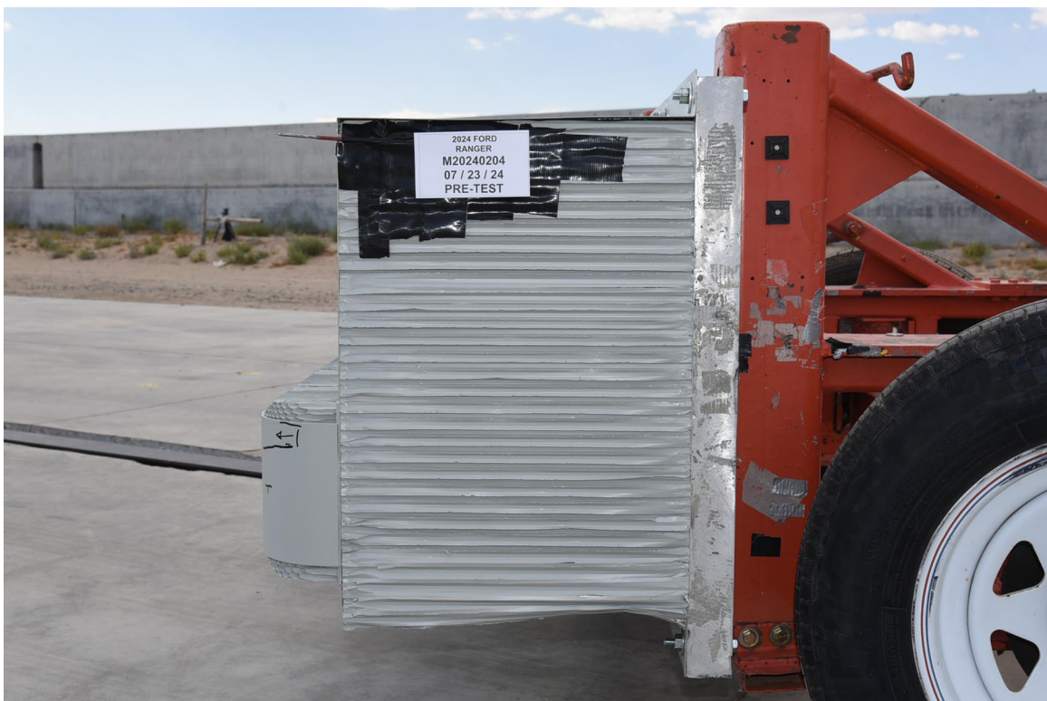
FIGURE 88. Pre-Test Left View of MDB Impactor Face
