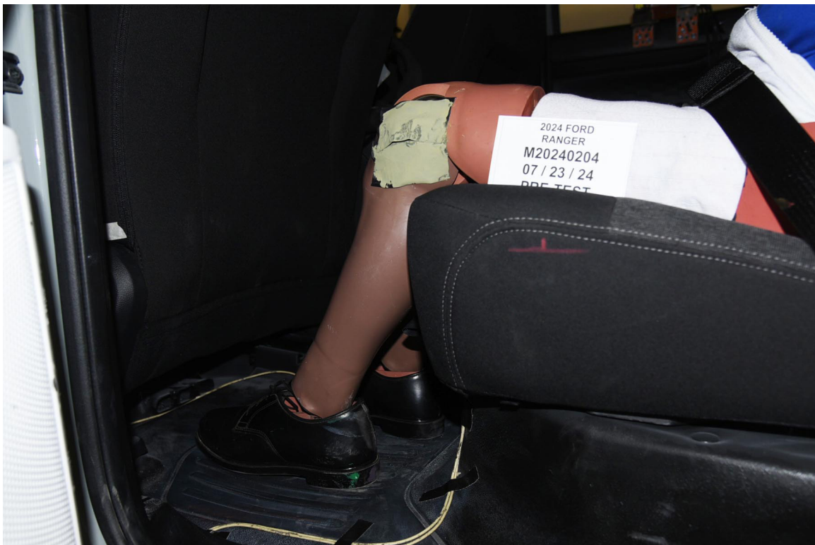
FIGURE 64. Pre-Test Placement of Rear Passenger Dummy's Feet
