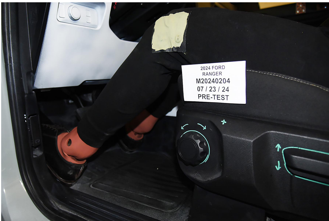
FIGURE 34. Pre-Test Placement of Driver Dummy's Feet
