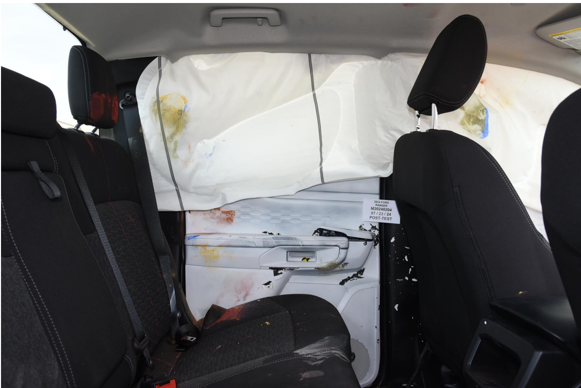
FIGURE 74. Post-Test Rear Passenger Inner Door Panel View
