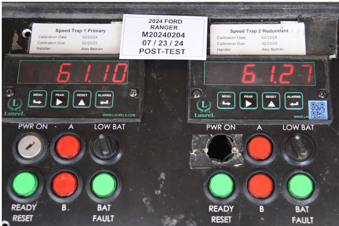
FIGURE 95. Post-Test Primary and Redundant Speed Trap Read-Out
