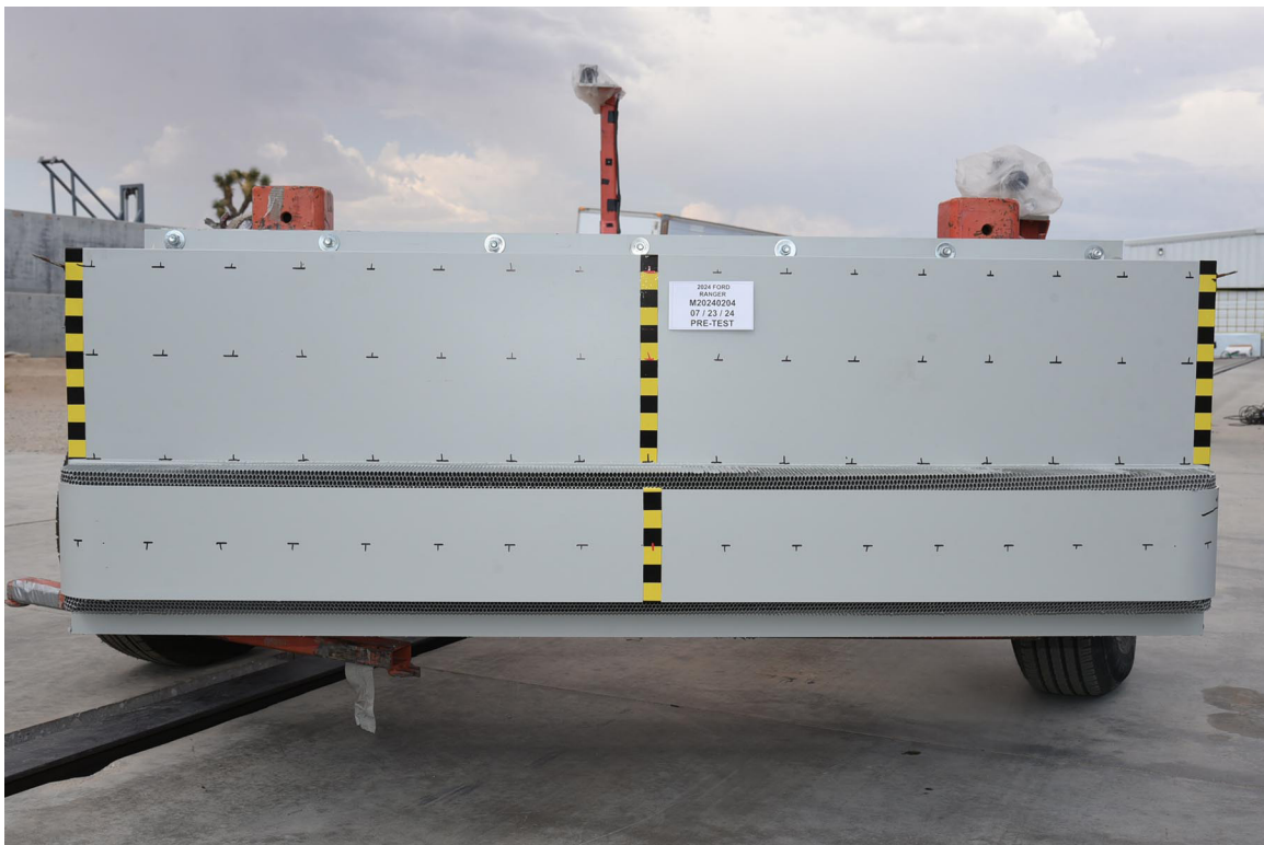
FIGURE 84. Pre-Test Front View of MDB Impactor Face
