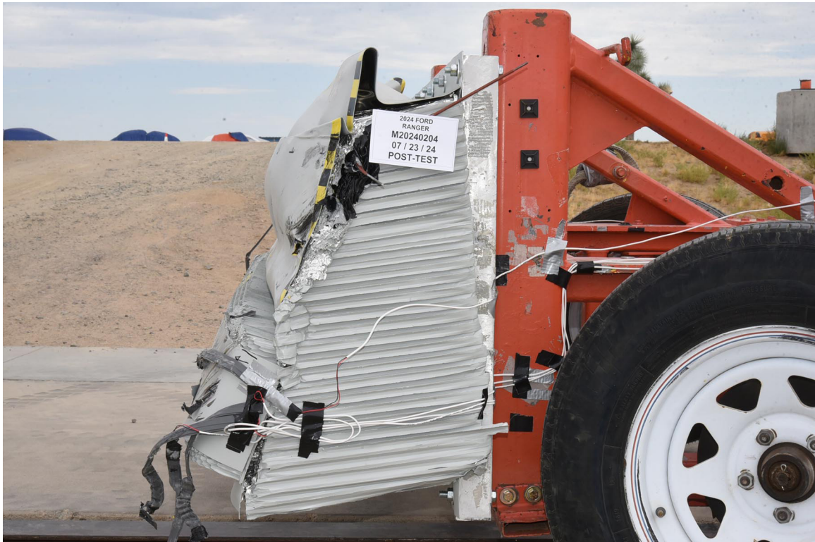
FIGURE 89. Post-Test Left View of MDB Impactor Face
