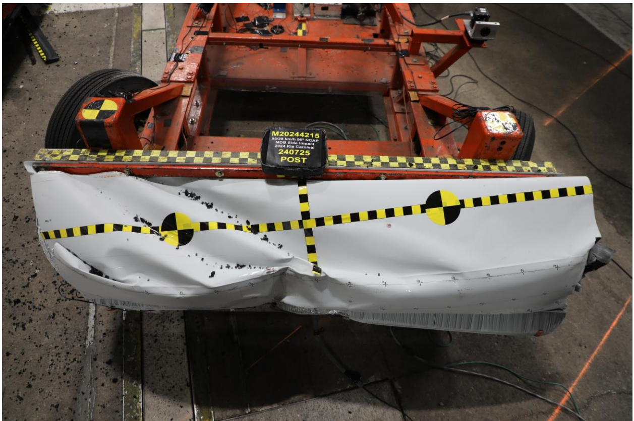
087 Post-Test Top View of MDB Impactor Face
