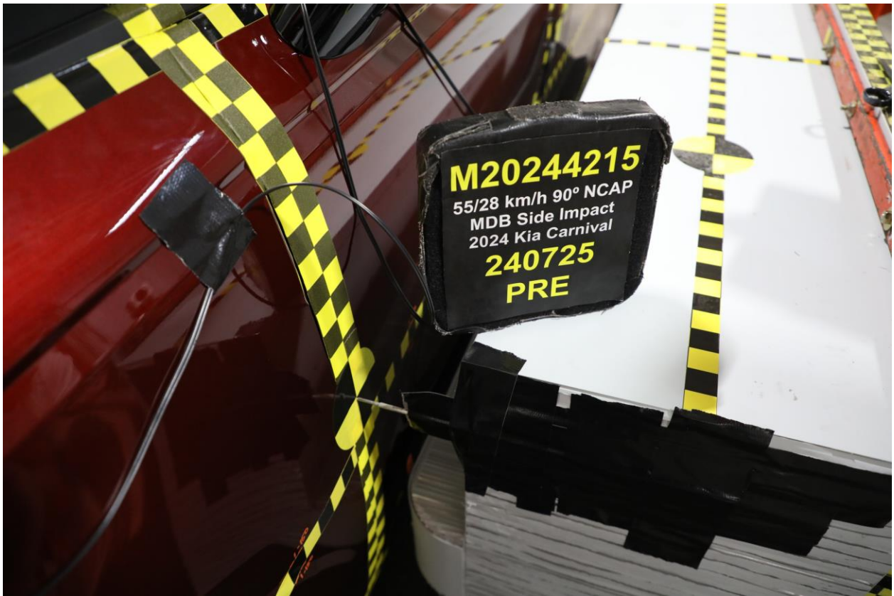
019 Pre-Test Close-Up View of Impact Point Target
