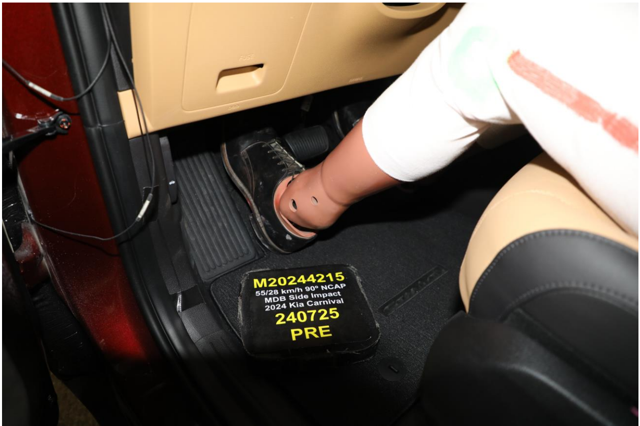
034 Pre-Test Placement of Driver's Dummy Feet
