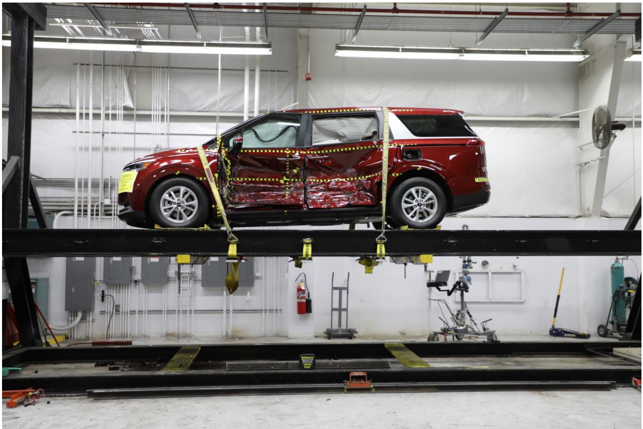
100 FMVSS No. 301 Static Rollover 360 Degrees
