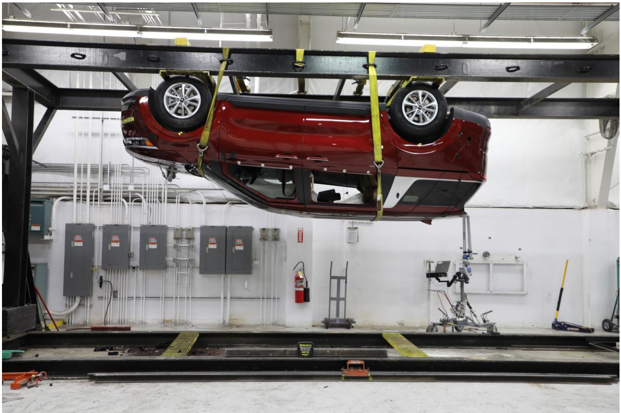
098 FMVSS No. 301 Static Rollover 180 Degrees
