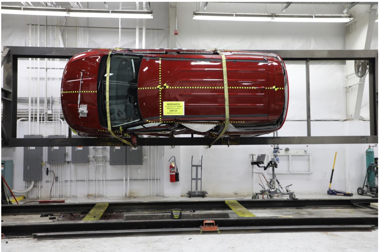
097 FMVSS No. 301 Static Rollover 90 Degrees
