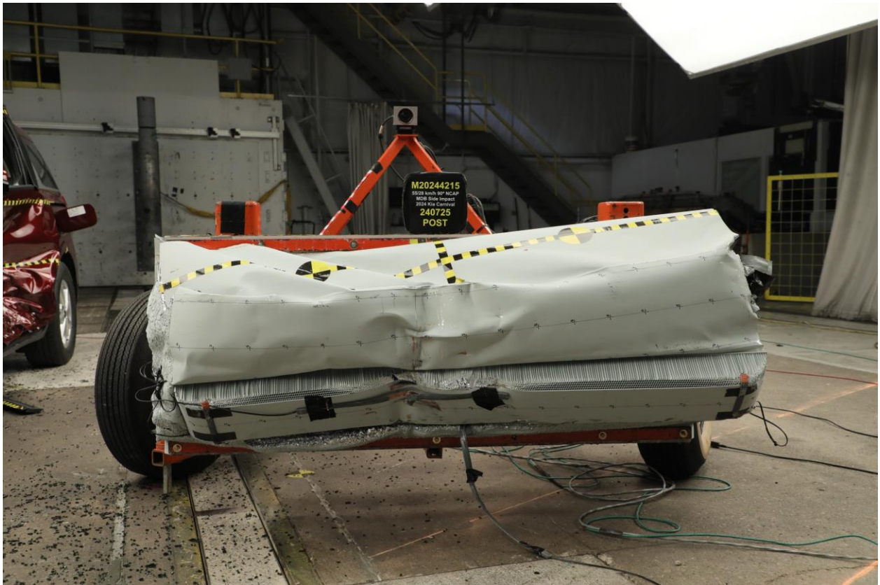
085 Post-Test Front View of MDB Impactor Face
