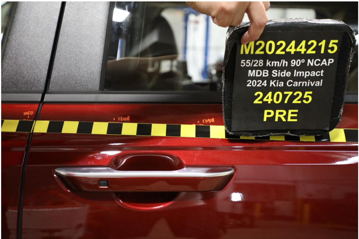
023 Pre-Test Left Rear Door Latch Close-Up
