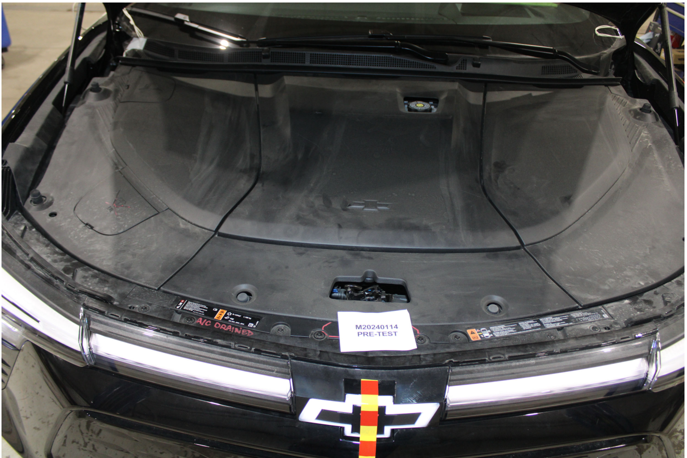
Photo No. 305-04 - First Responder Warning Location
