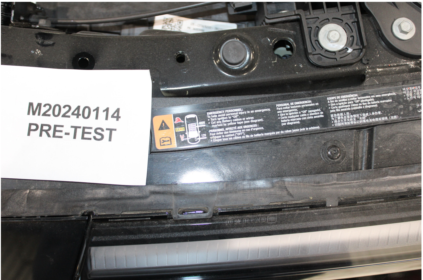
Photo No. 305-03 - First Responder Warning Label
