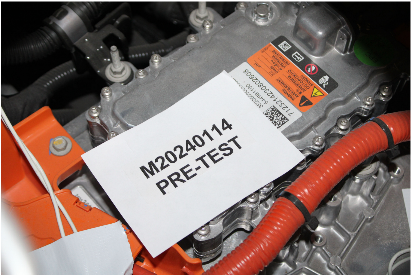
Photo No. 305-02 - Power Inverter Warning Label
