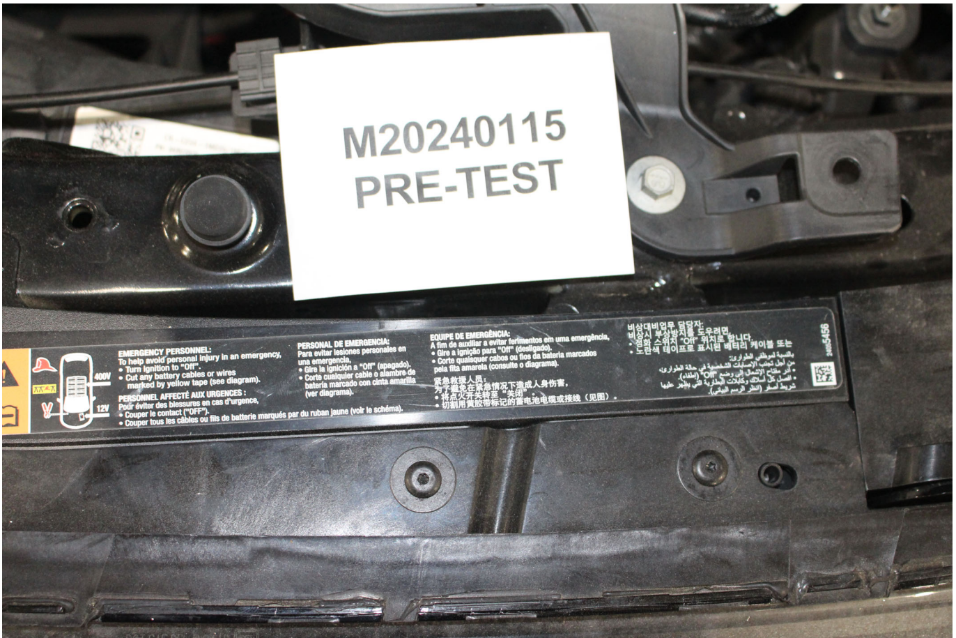
Photo No. 305-03 - First Responder Warning Label
