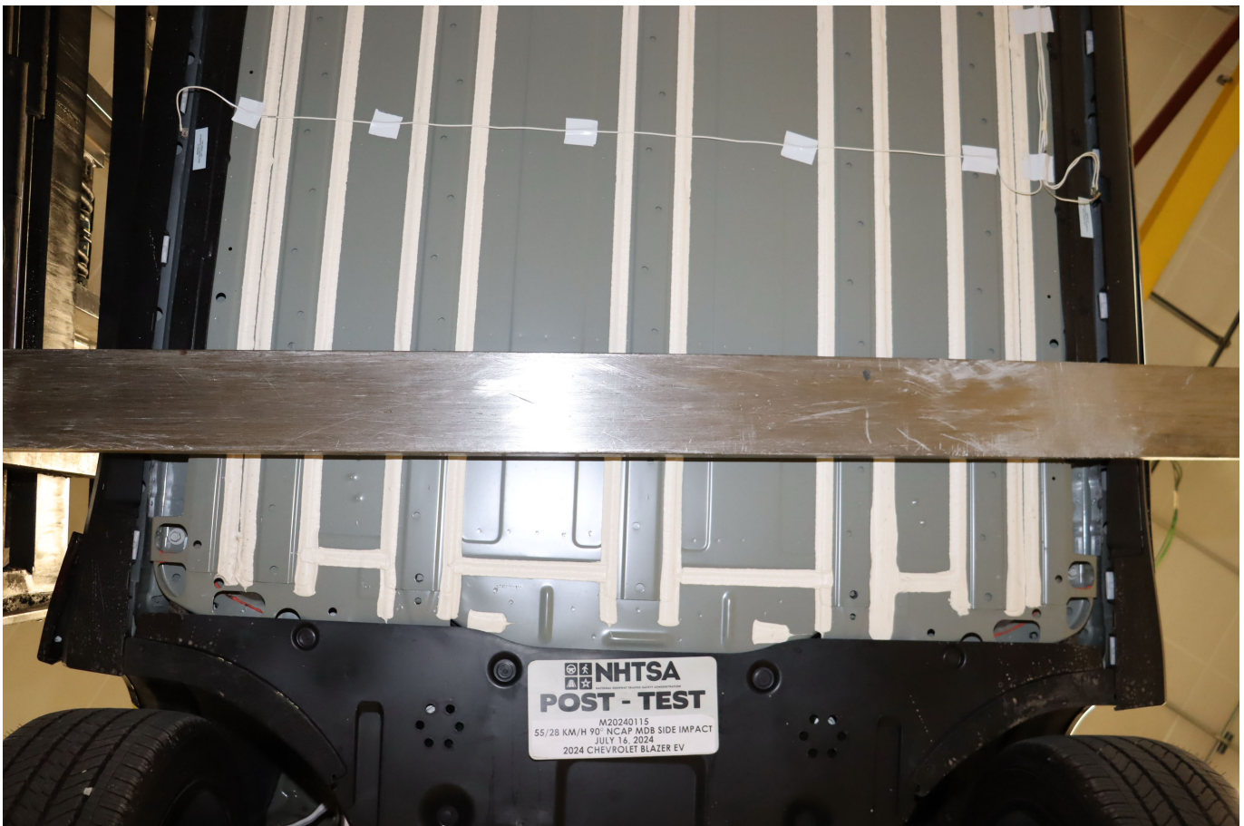
Photo No. 305-10 - Post-Impact Front View of Propulsion Battery
