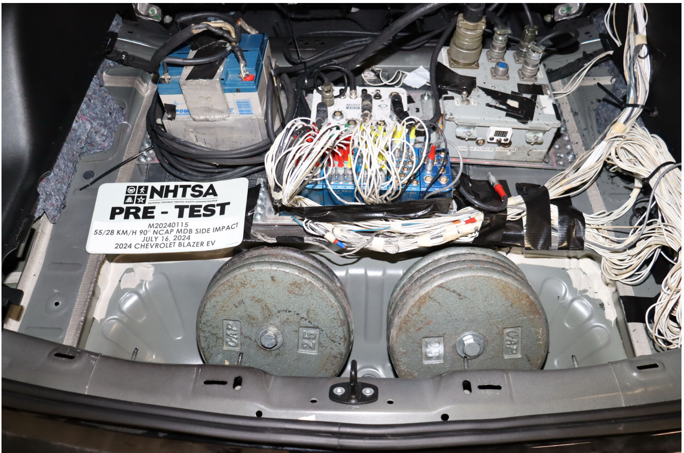
Photo No. 094 - Pre-Test Ballast View
