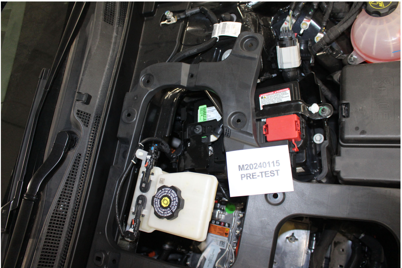
Photo No. 305-01 - Auxiliary Power Module Warning Label
