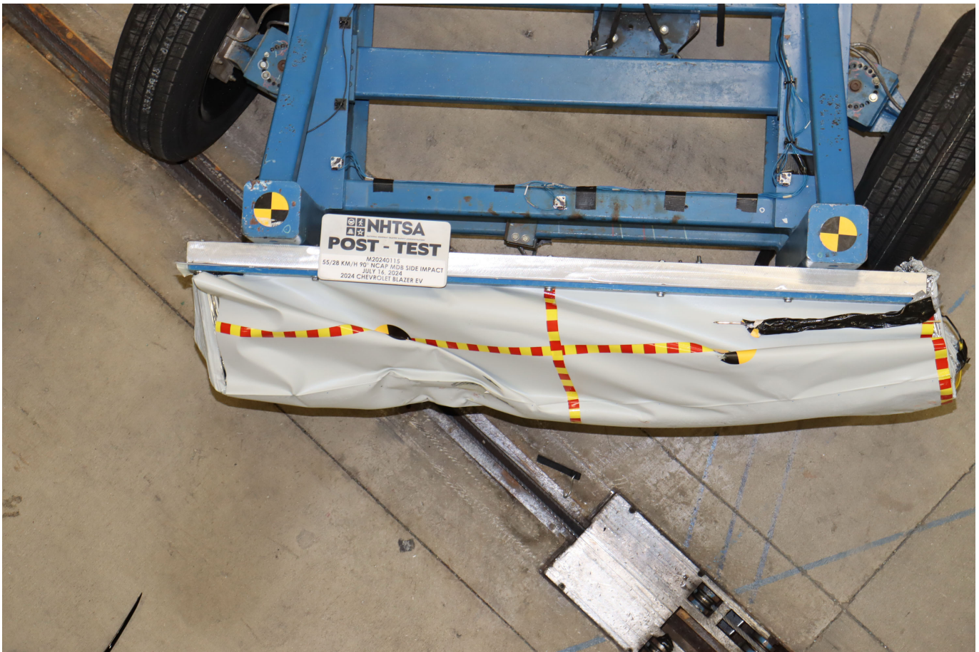
Photo No. 087 - Post-Test Top View of MDB Impactor Face
