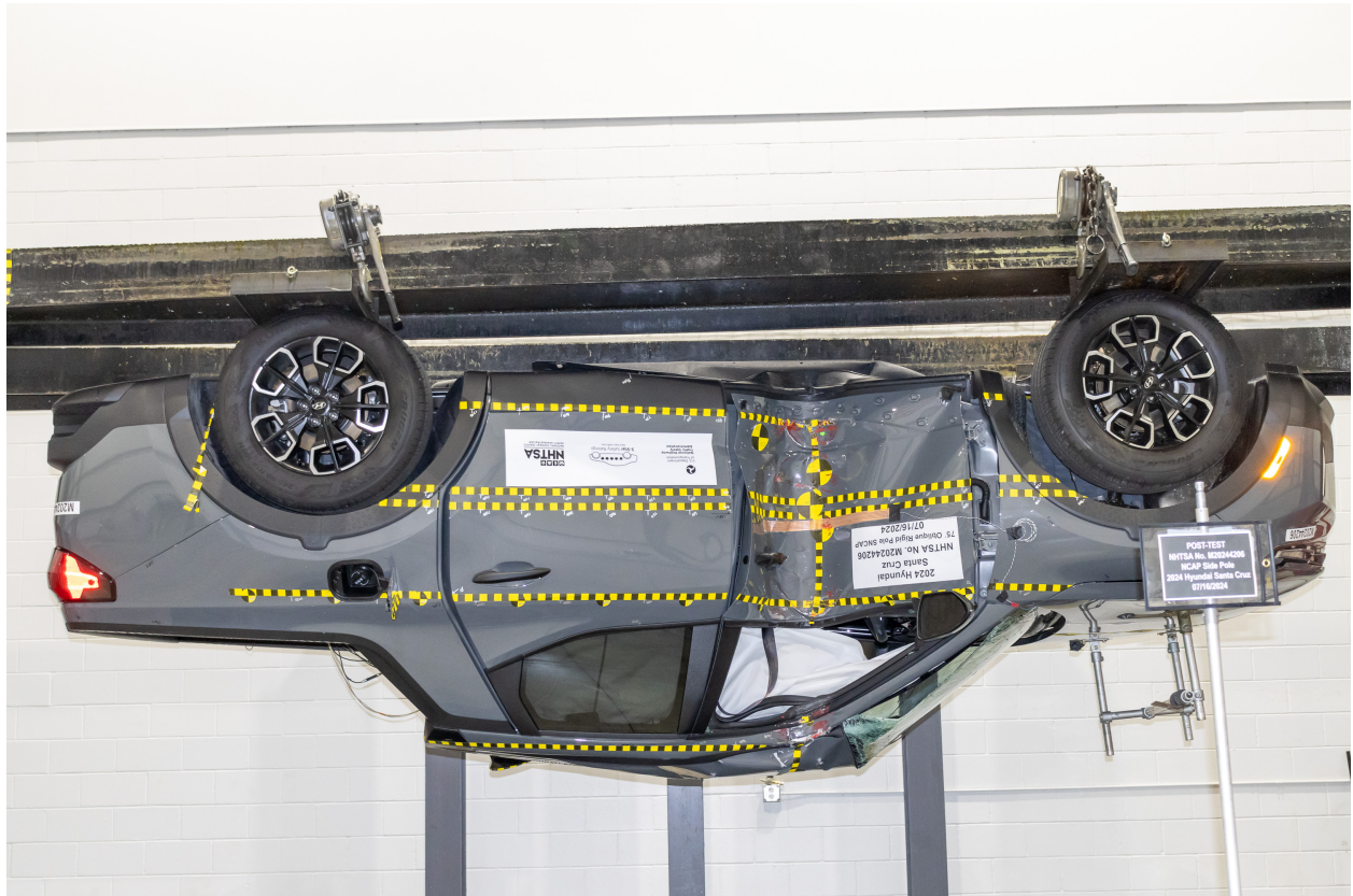
Figure A-67: FMVSS No. 301 Static Rollover 180 Degrees
