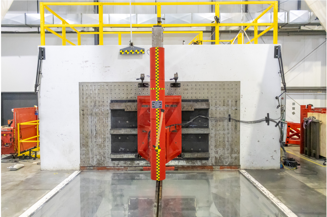
Figure A-59: Pre-Test Pole Barrier Front View
