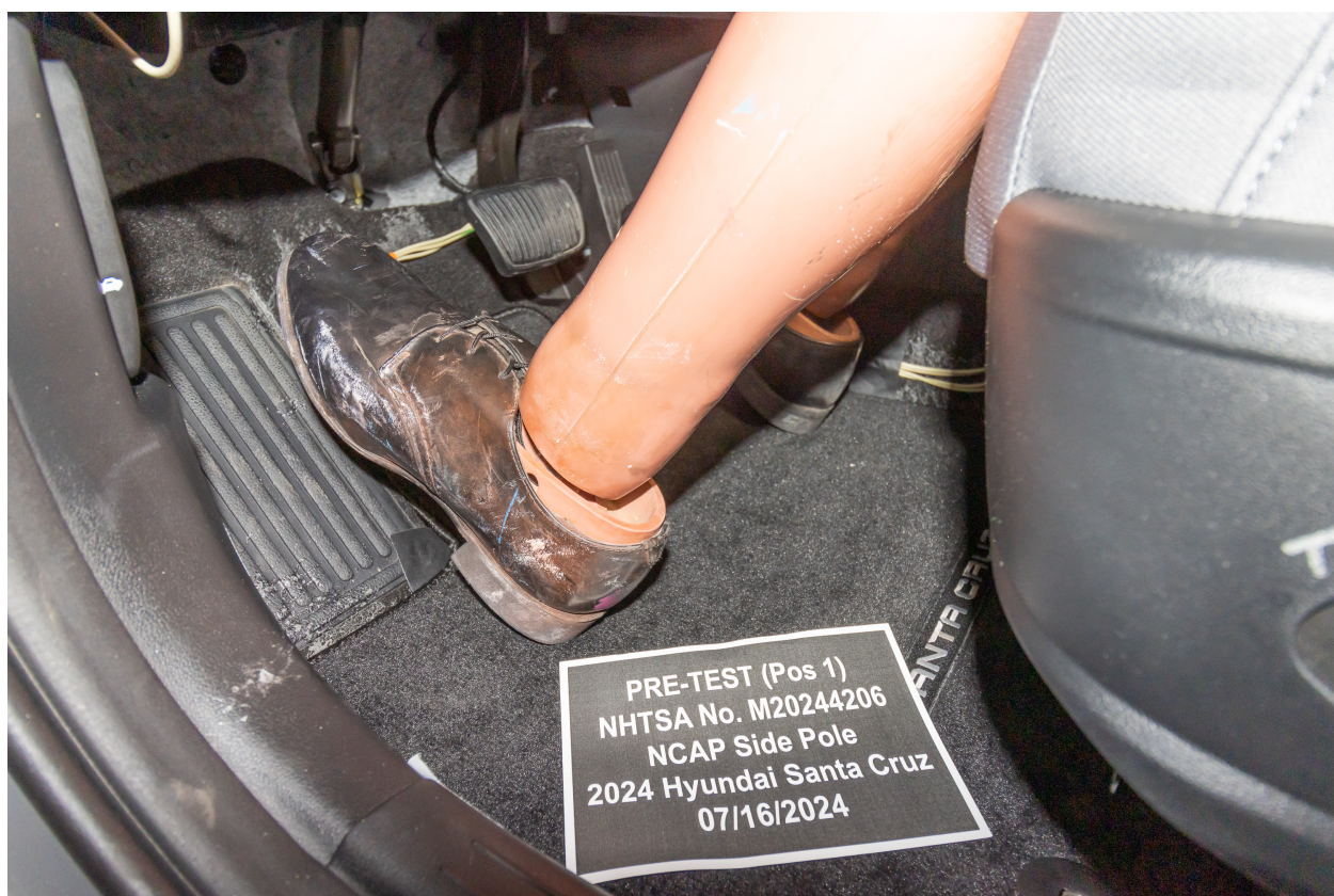
Figure A-32: Pre-Test Placement of Dummy's Feet
