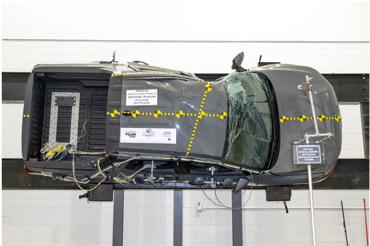
Figure A-68: FMVSS No. 301 Static Rollover 270 Degrees
