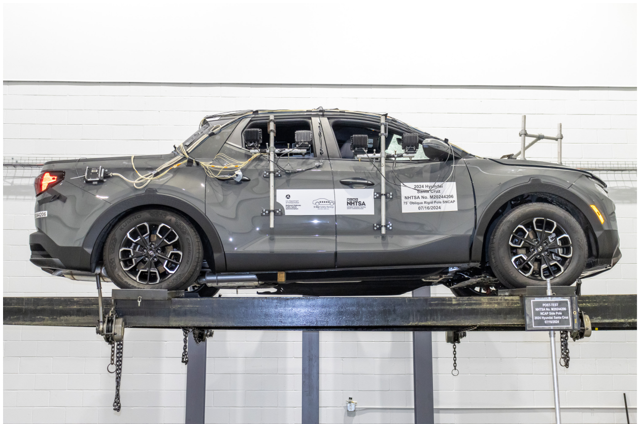
Figure A-69: FMVSS No. 301 Static Rollover 360 Degrees
