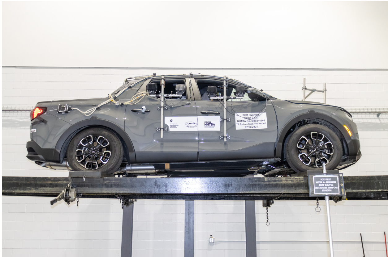
Figure A-65: FMVSS No. 301 Static Rollover 0 Degrees
