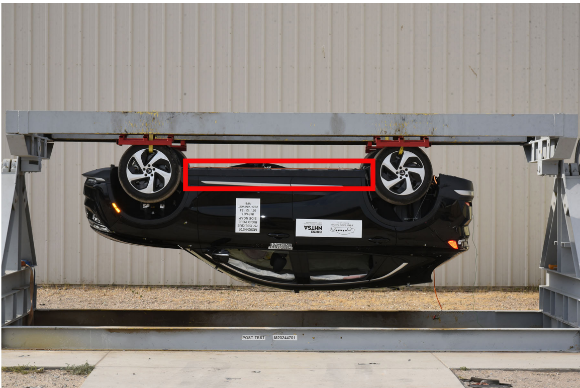
FIGURE 305-029 FMVSS No. 305 Static Rollover at 180°
