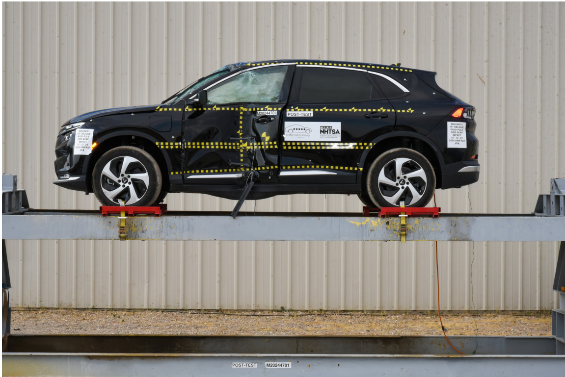
FIGURE 69. FMVSS No. 301 Static Rollover 360 Degrees
