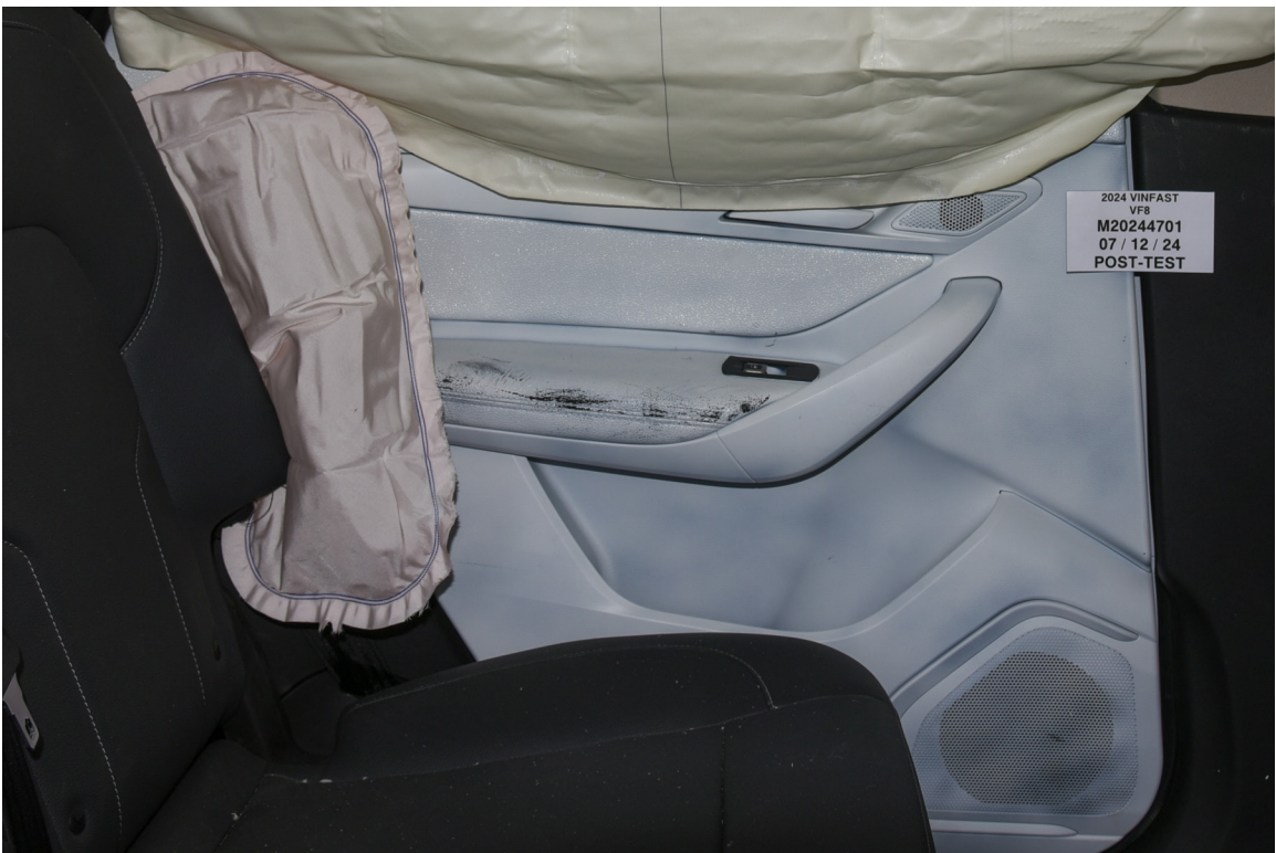
FIGURE 54. Post-Test Inner Rear Passenger Torso Air Bag Deployment View
