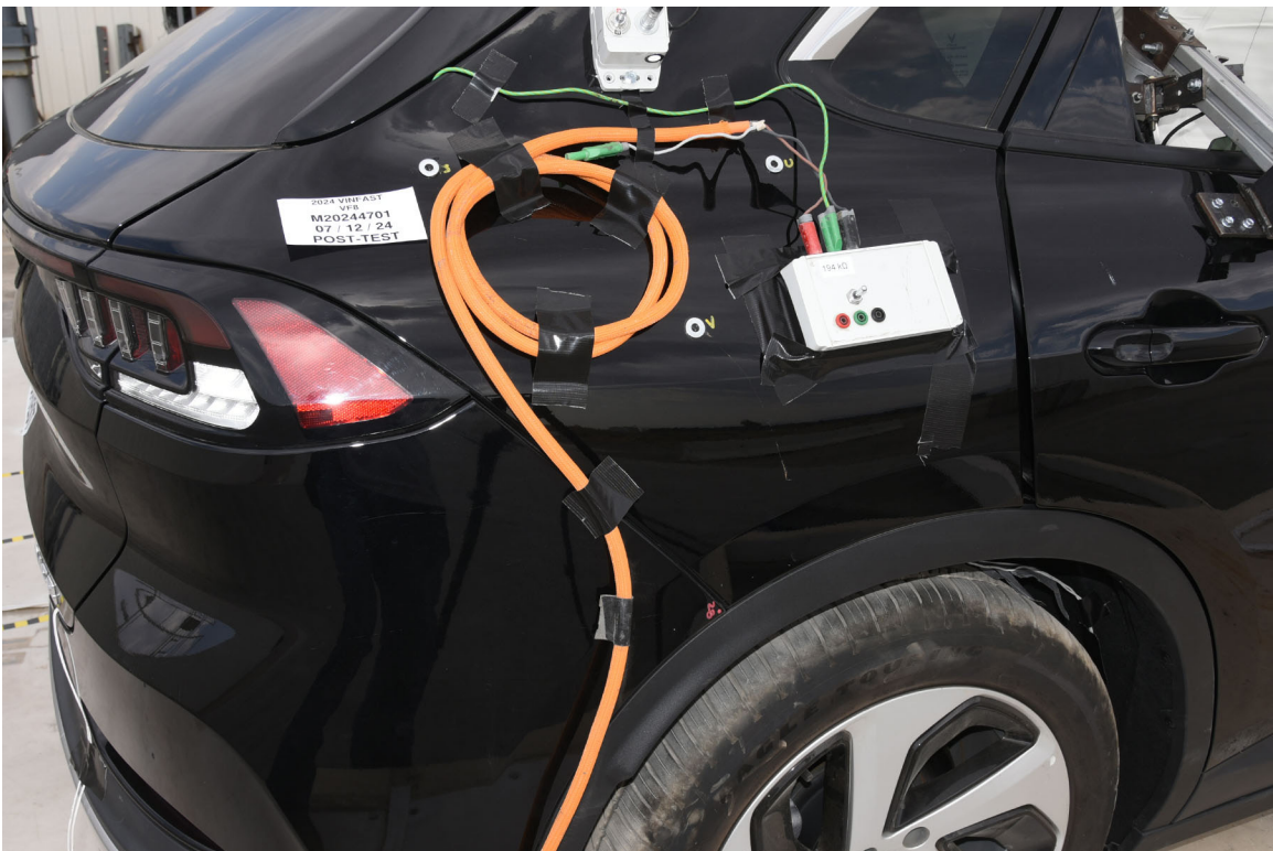
FIGURE 305-027 Post-Impact View of Other Test Devices
