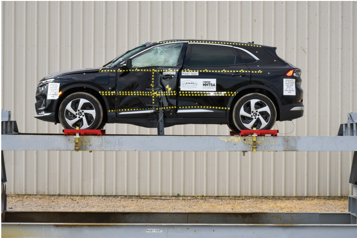
FIGURE 65. FMVSS No. 301 Static Rollover 0 Degrees
