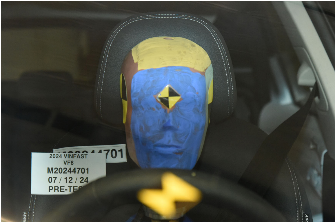
FIGURE 27. Pre-Test Frontal View of Dummy Head and Shoulders in Relation to Head Restraint
