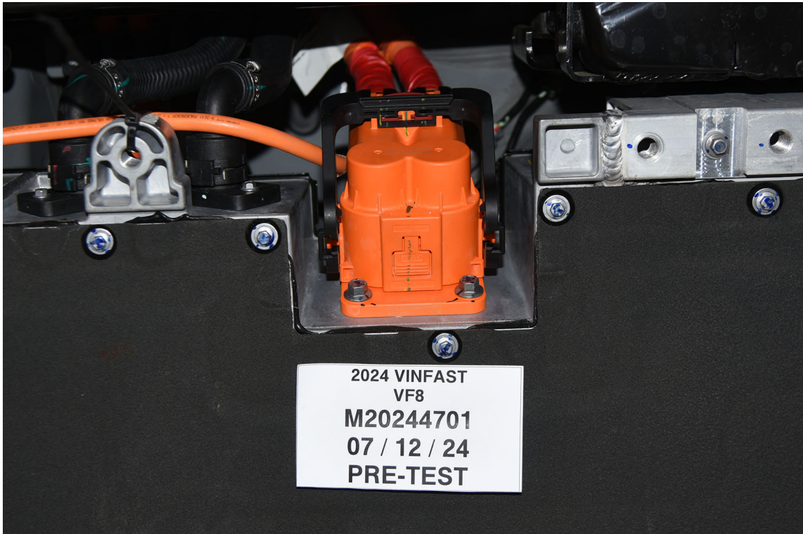
FIGURE 305-06 Manual High Voltage Service Disconnect in Place
