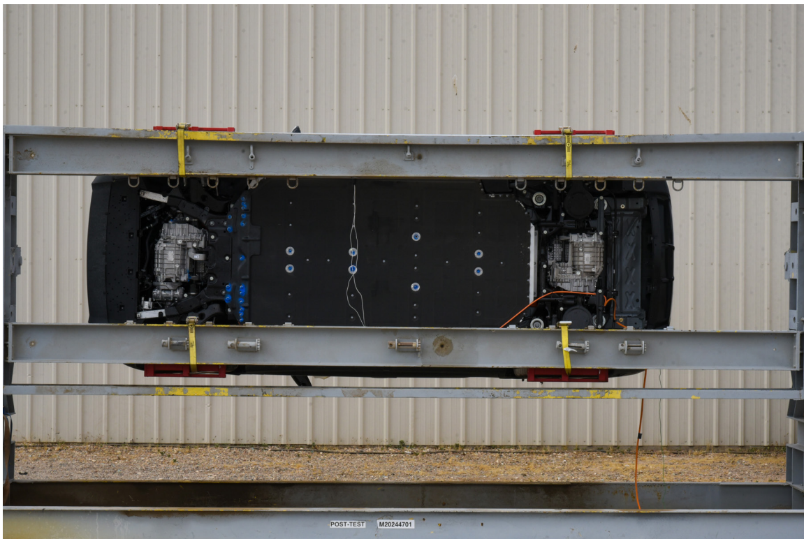
FIGURE 68. FMVSS No. 301 Static Rollover 270 Degrees
