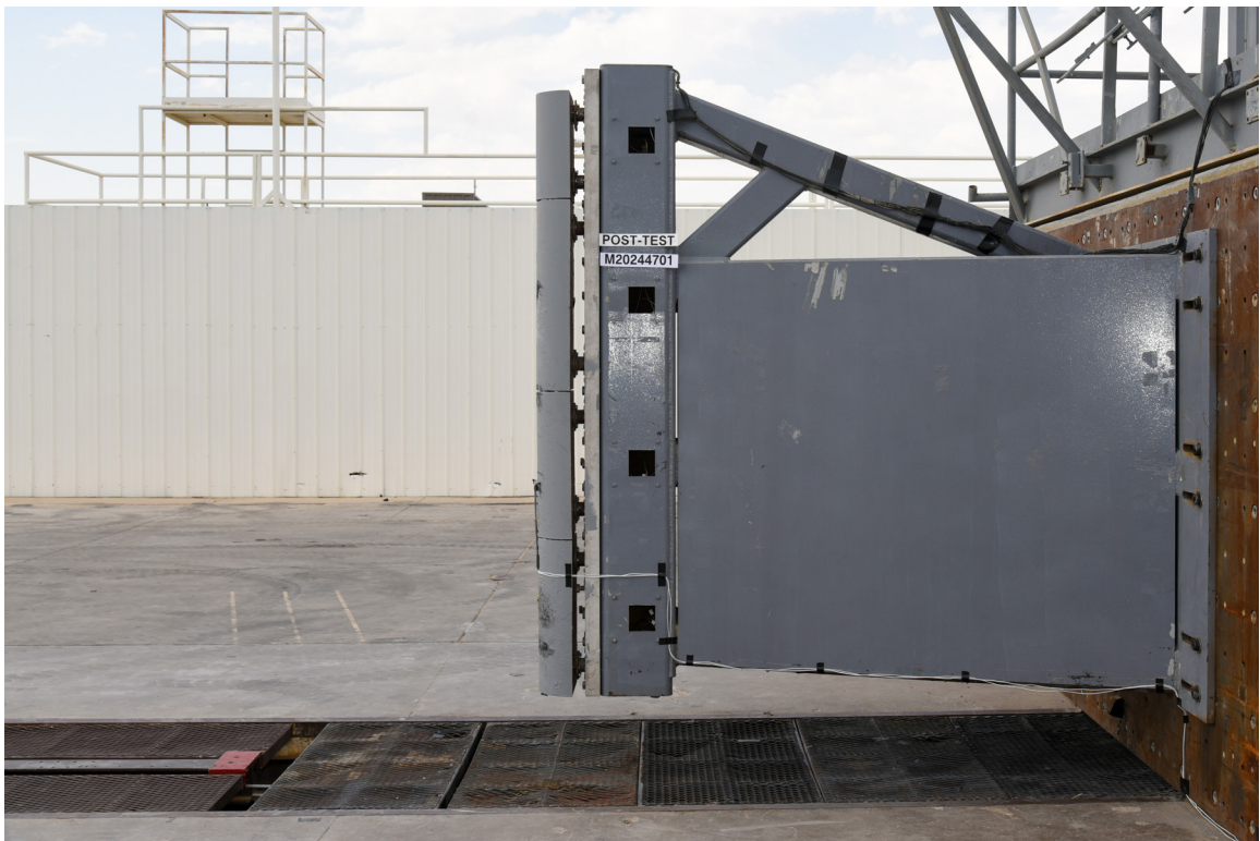
FIGURE 62. Post-Test Pole Barrier Side View
