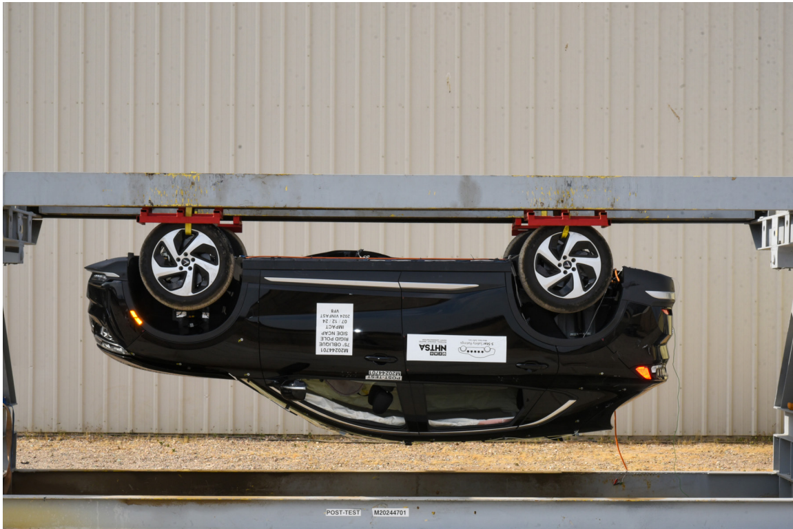
FIGURE 67. FMVSS No. 301 Static Rollover 180 Degrees
