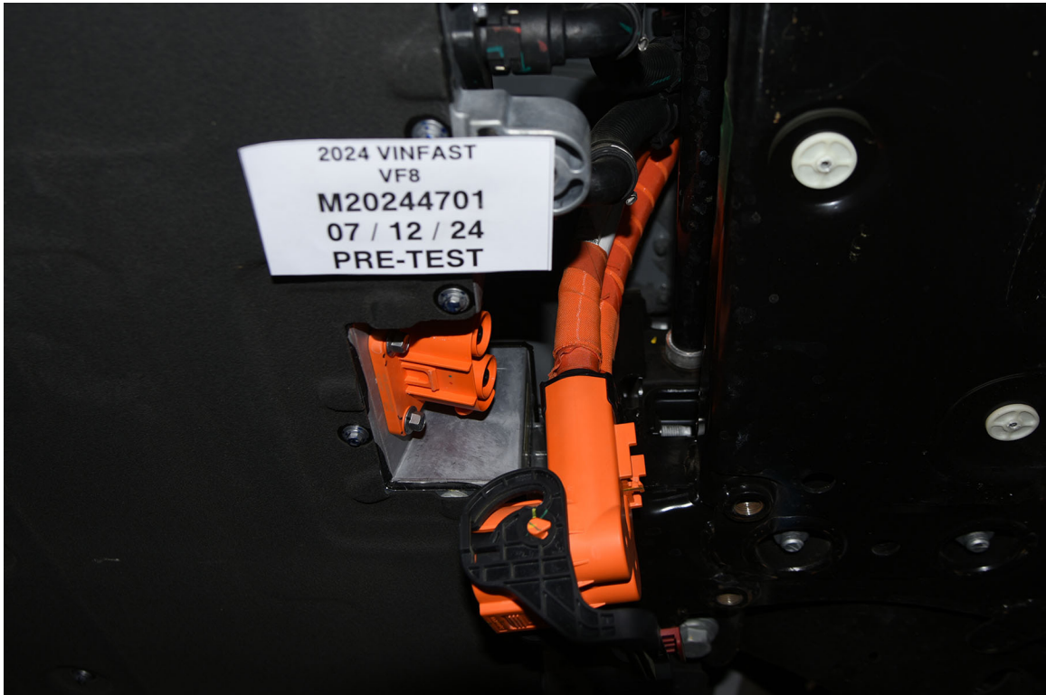
FIGURE 305-08 Manual High Voltage Service Disconnect Removed
