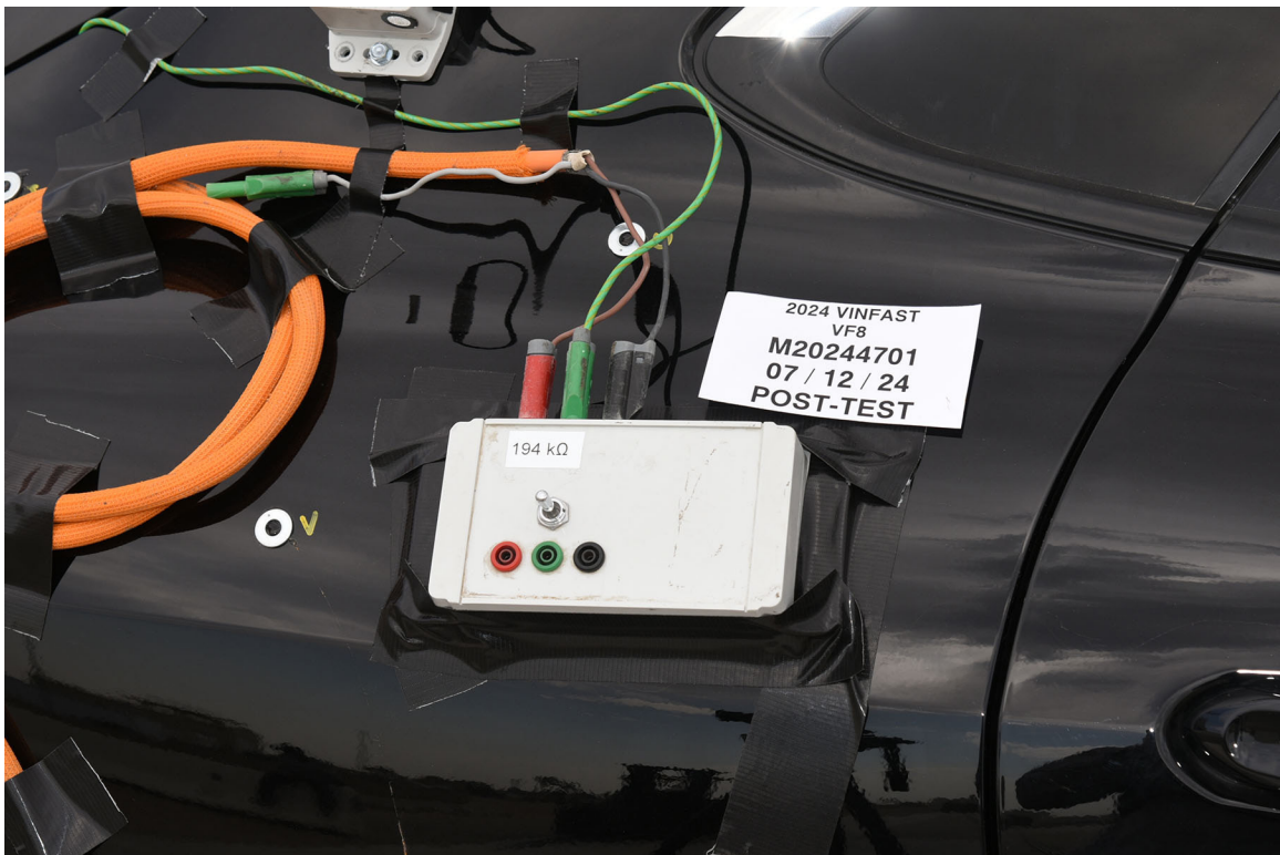
FIGURE 305-025 Post-Impact View of Installed Test Interface Port
