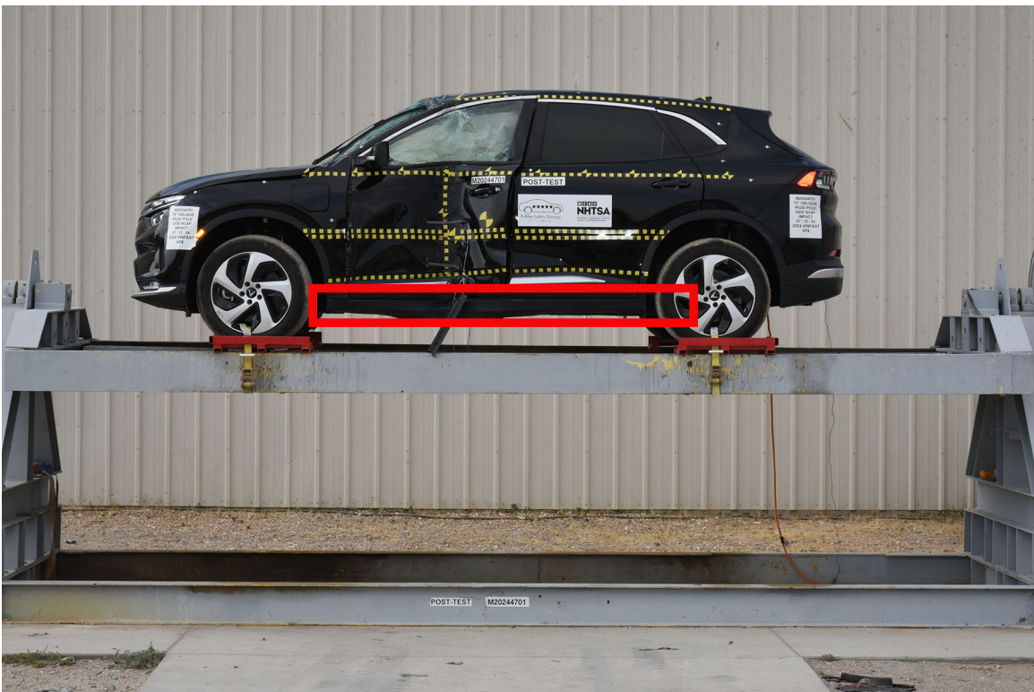
FIGURE 305-031 FMVSS No. 305 Static Rollover at 360°
