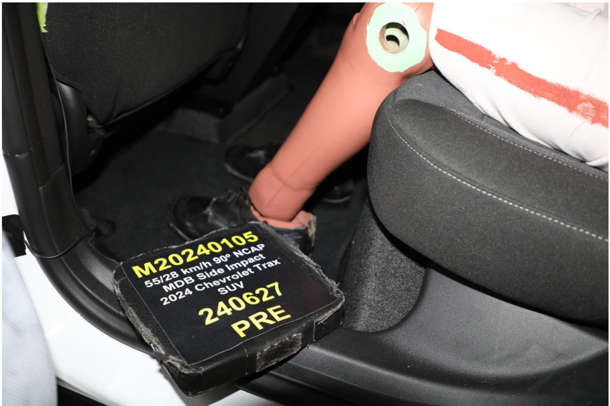
064 Pre-Test Placement of Rear Passenger Dummy's Feet
