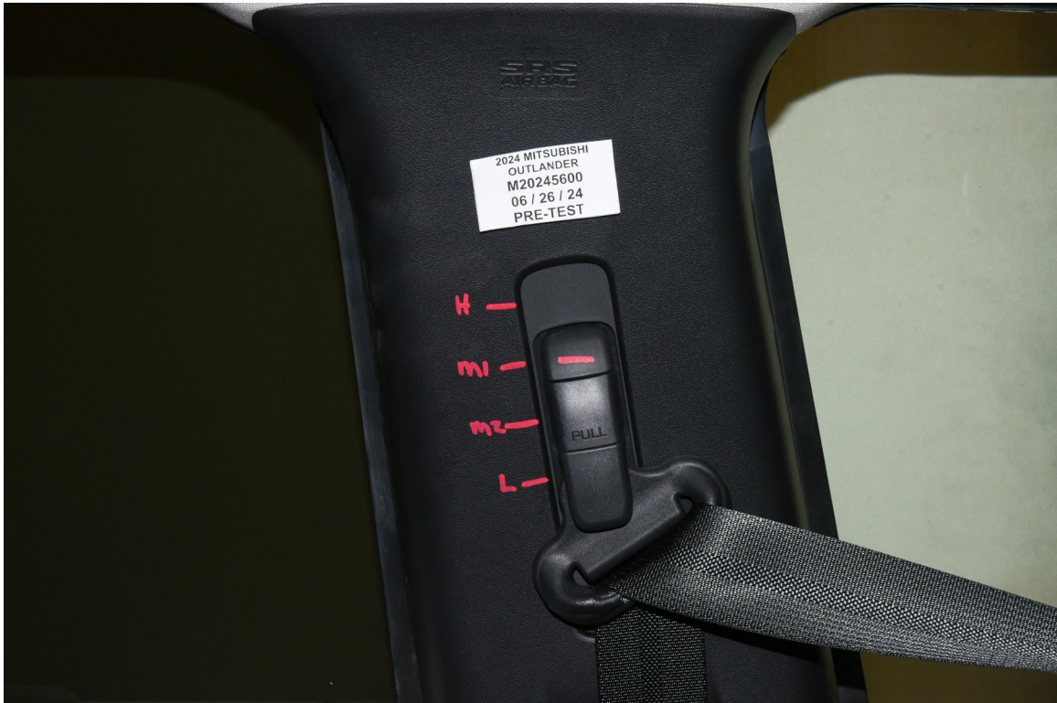
FIGURE 33. Pre-Test View of Belt Anchorage for Dummy
