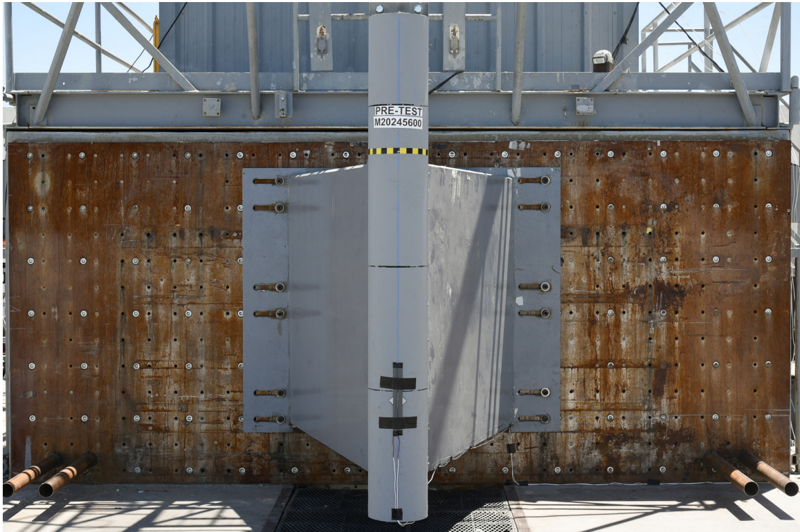
FIGURE 59. Pre-Test Pole Barrier Front View
