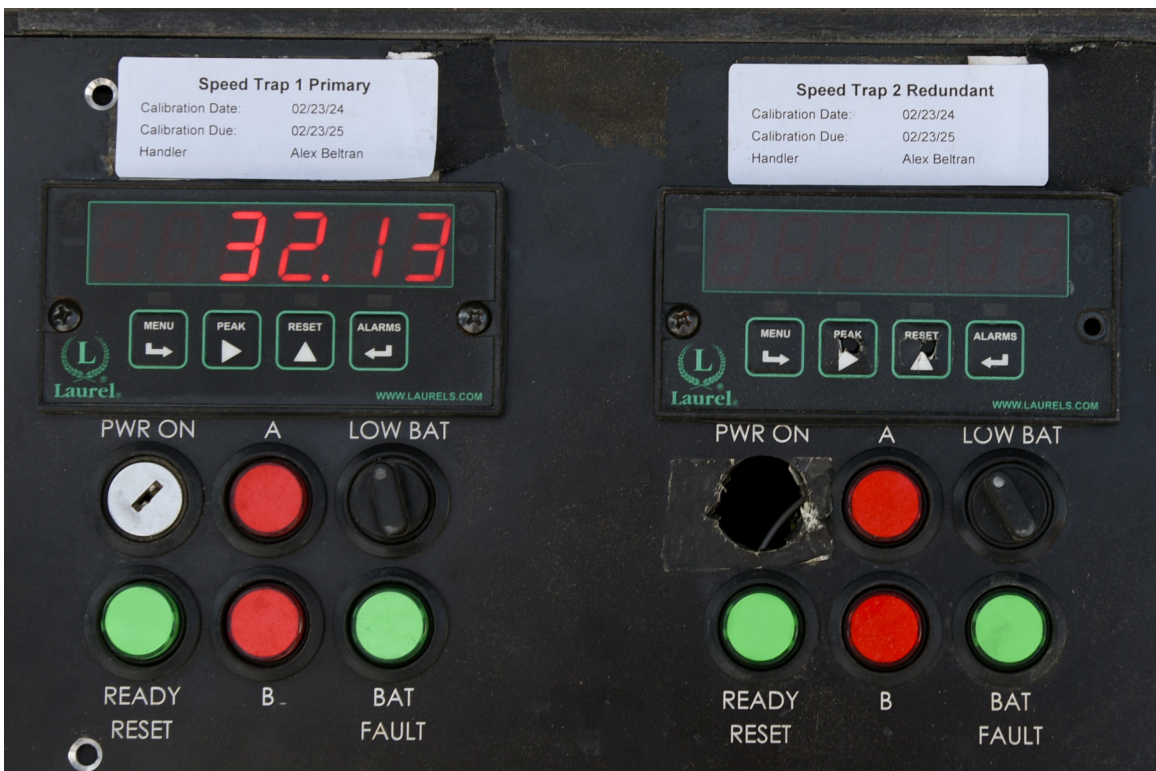
FIGURE 64. Post-Test Primary and Redundant Speed Trap Read-Out
