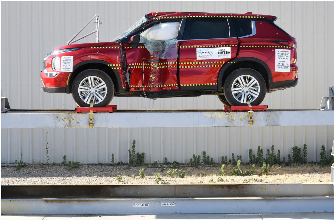
FIGURE 69. FMVSS No. 301 Static Rollover 360 Degrees
