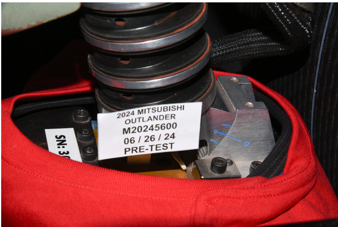
FIGURE 30. Pre-Test Left Side View of Dummy's Neck Showing Position of Adjustable Neck Bracket
