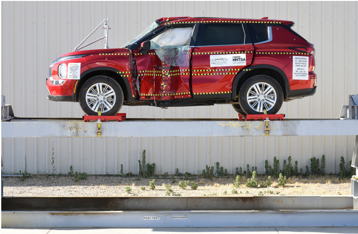
FIGURE 65. FMVSS No. 301 Static Rollover 0 Degrees
