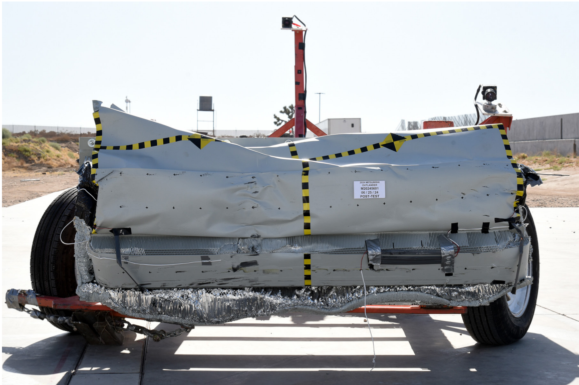
FIGURE 85. Post-Test Front View of MDB Impactor Face
