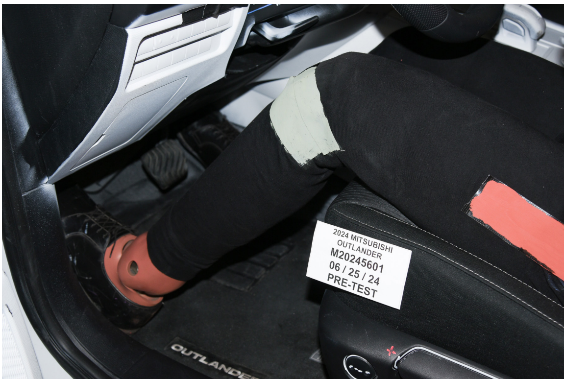
FIGURE 34. Pre-Test Placement of Driver Dummy's Feet
