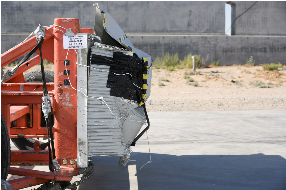
FIGURE 91. Post-Test Right View of MDB Impactor Face
