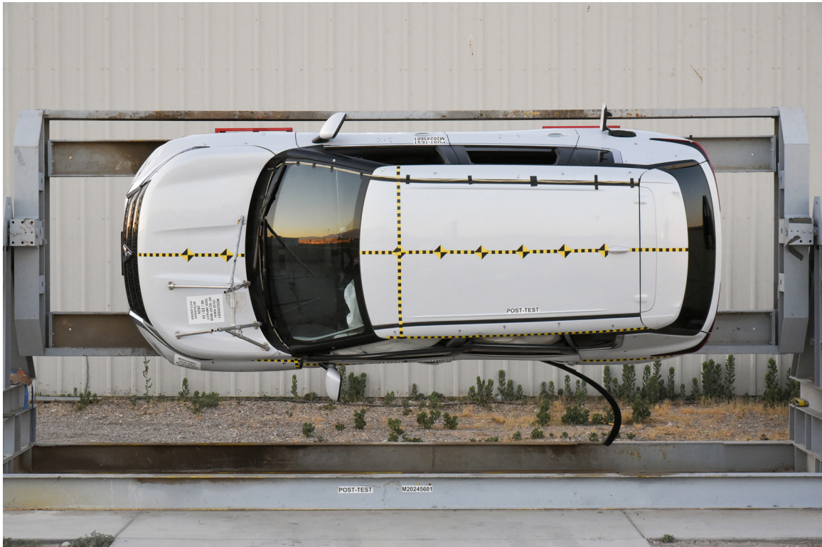
FIGURE 99. FMVSS No. 301 Static Rollover 270 Degrees
