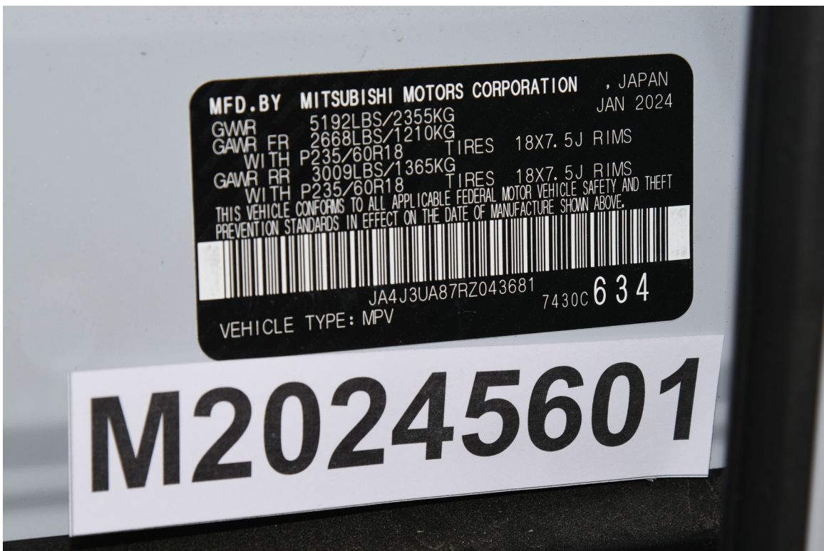
FIGURE 92. Close-Up View of Vehicle's Certification Label
