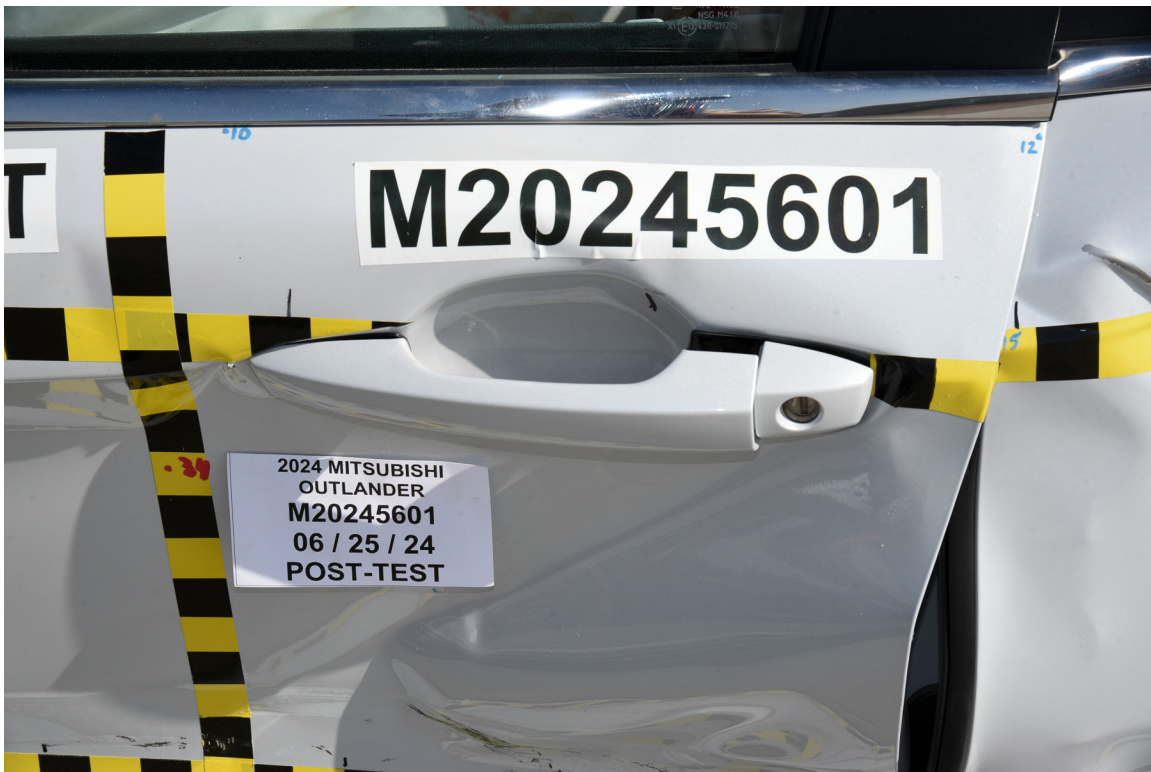
FIGURE 22. Post-Test Left Front Door Latch Close-Up
