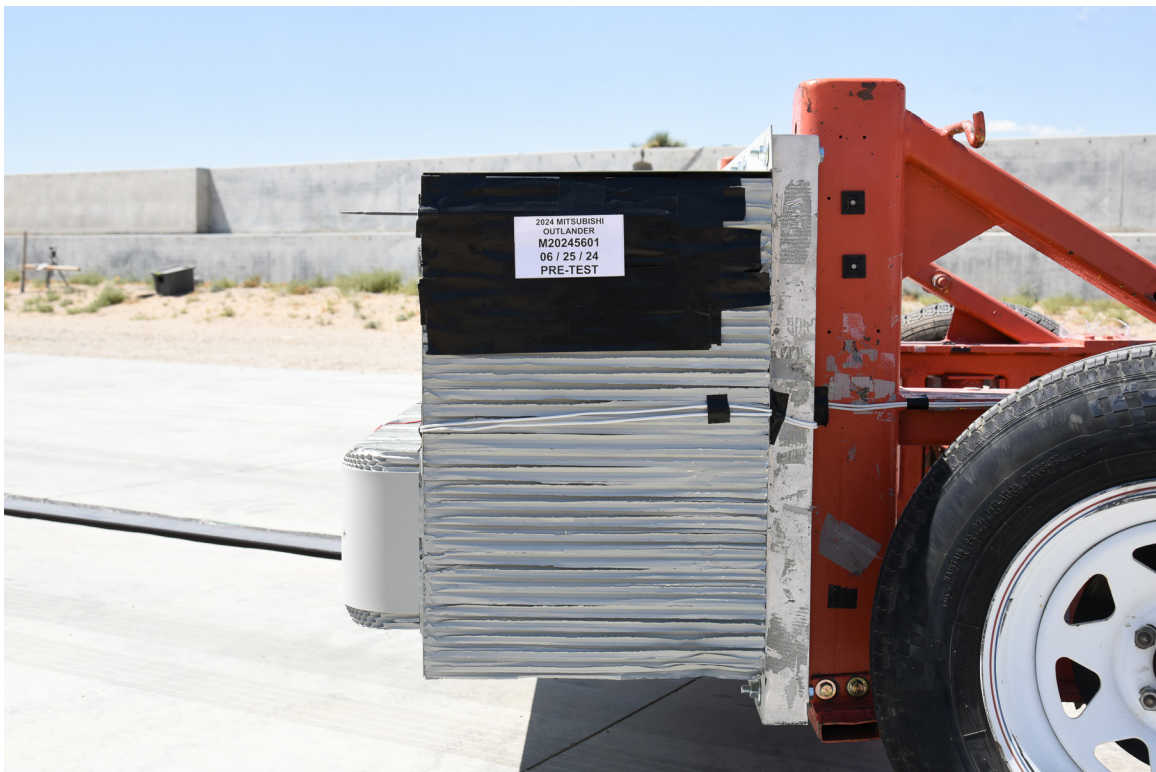
FIGURE 88. Pre-Test Left View of MDB Impactor Face
