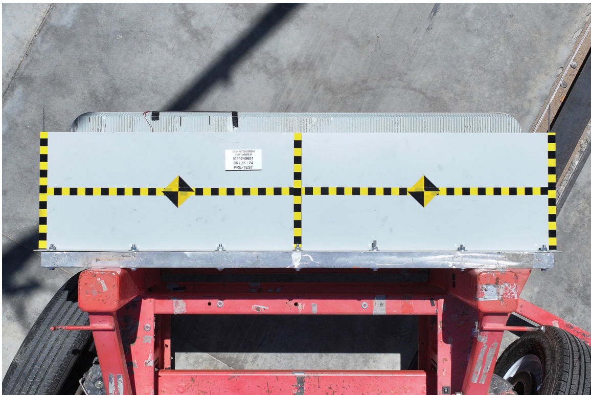
FIGURE 86. Pre-Test Top View of MDB Impactor Face
