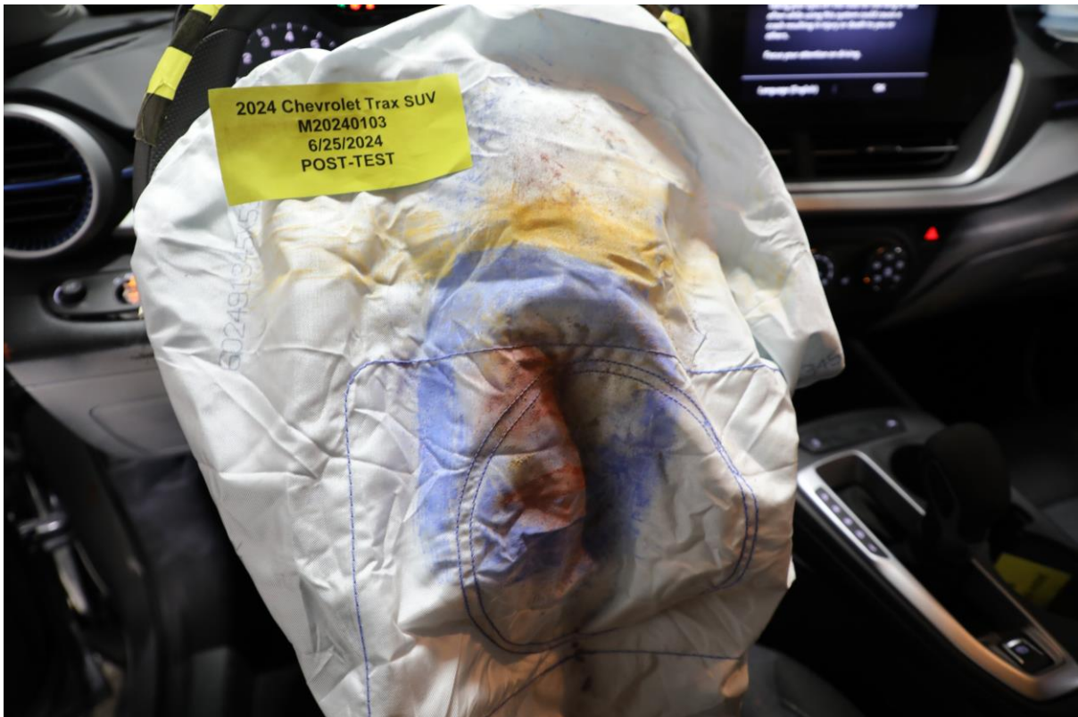
049 Post-Test Driver Dummy Contact with Airbag
