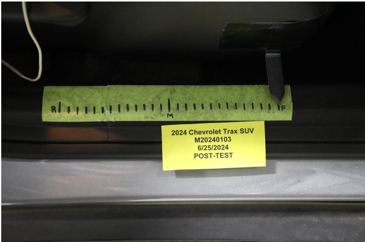
060 Post-Test Passenger's Seat Fore-Aft Markings
