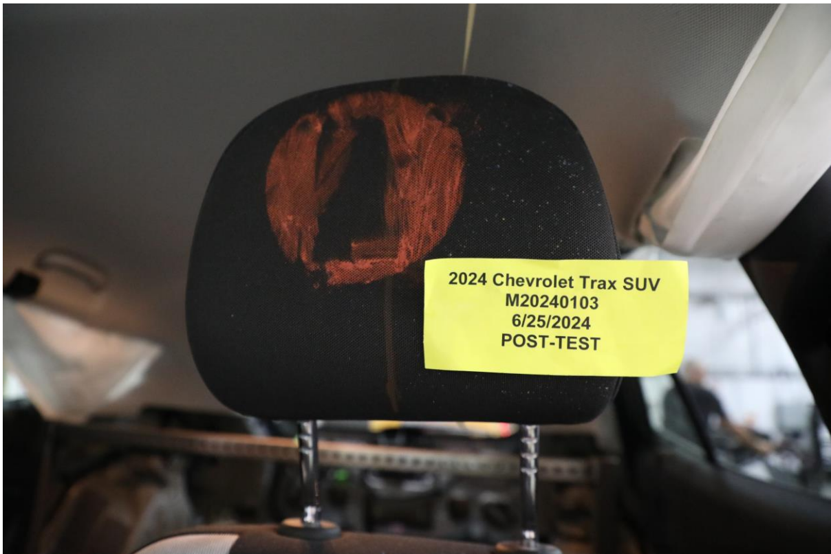
050 Post-Test Driver Dummy Contact with Headrest
