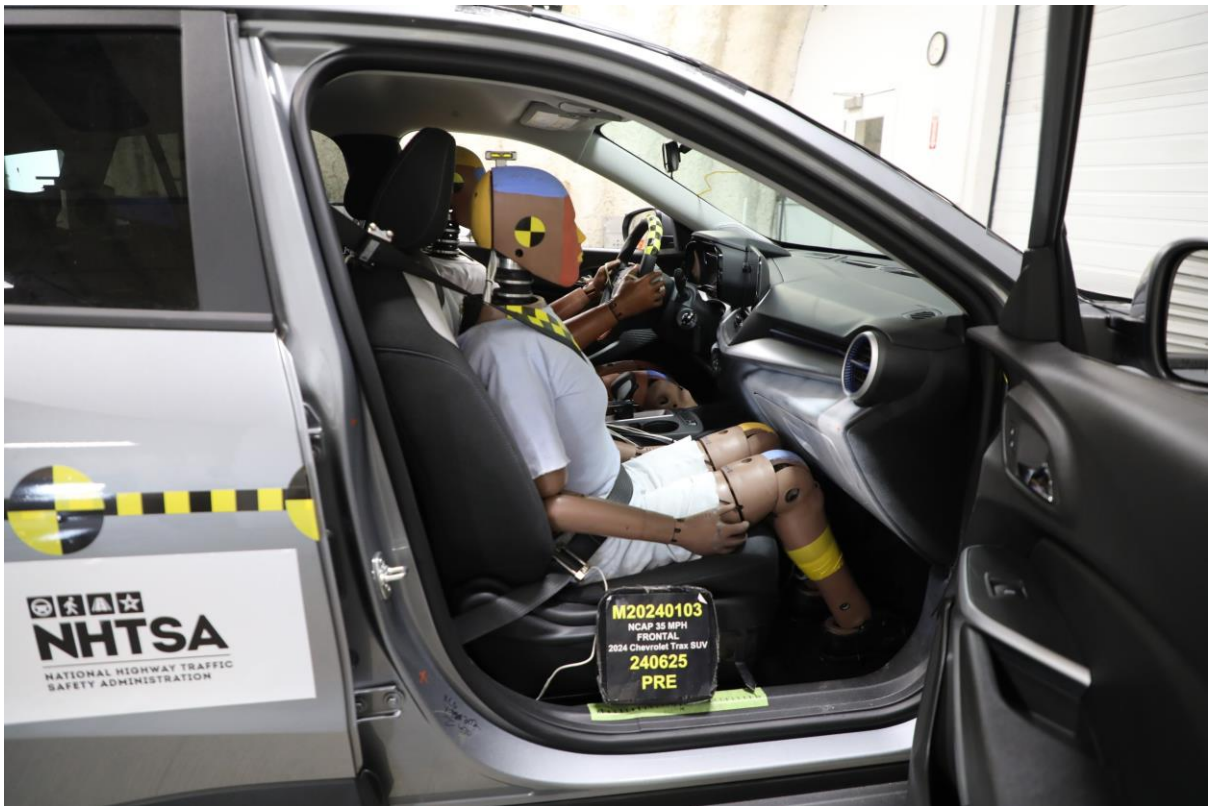
057 Pre-Test Passenger Dummy and Vehicle Interior View
