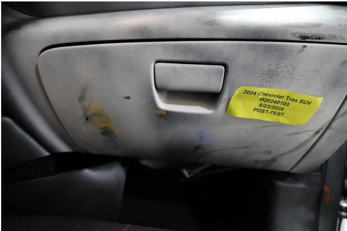
068 Post-Test Passenger's Side Knee Bolster
