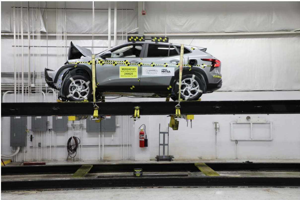
077 Vehicle at 0° on Static Rollover Device
