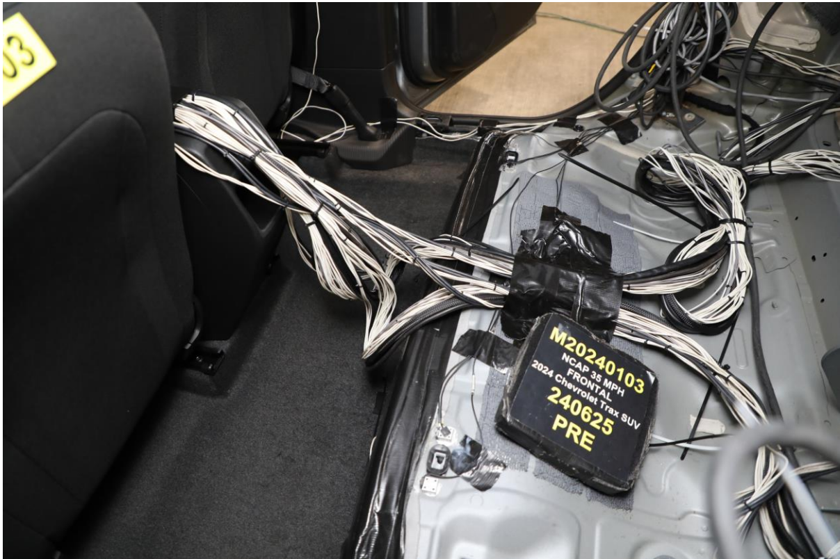
028 Pre-Test Dummy Cable Routing
