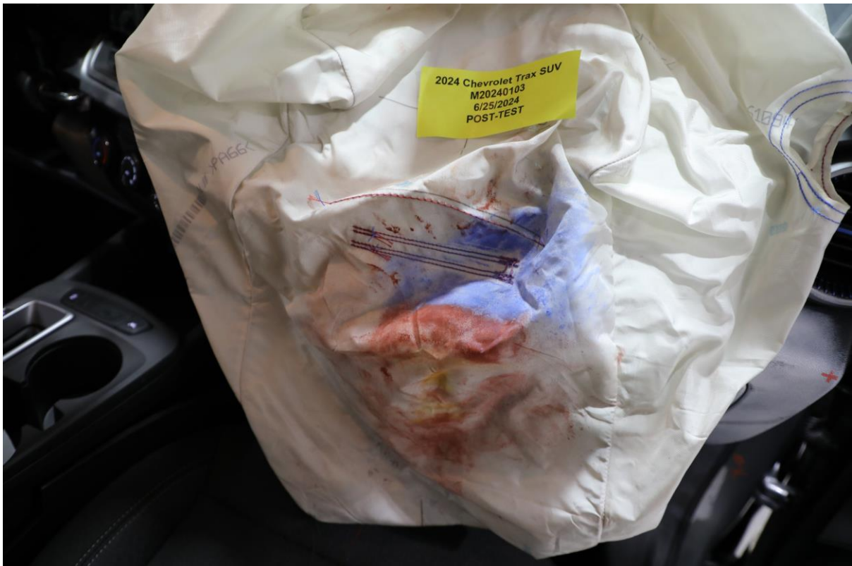
072 Post-Test Passenger Dummy Contact with Airbag
