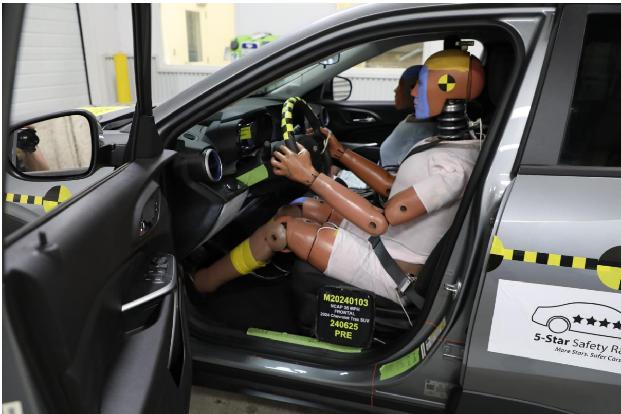
034 Pre-Test Driver Dummy and Vehicle Interior View
