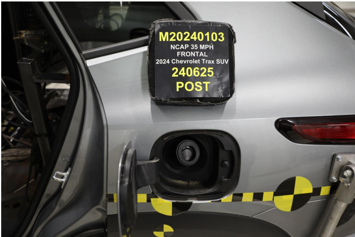
023 Post-Test Fuel Filler Cap View
