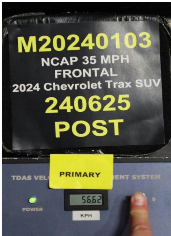
076 Post-Test Speed Trap Read out
