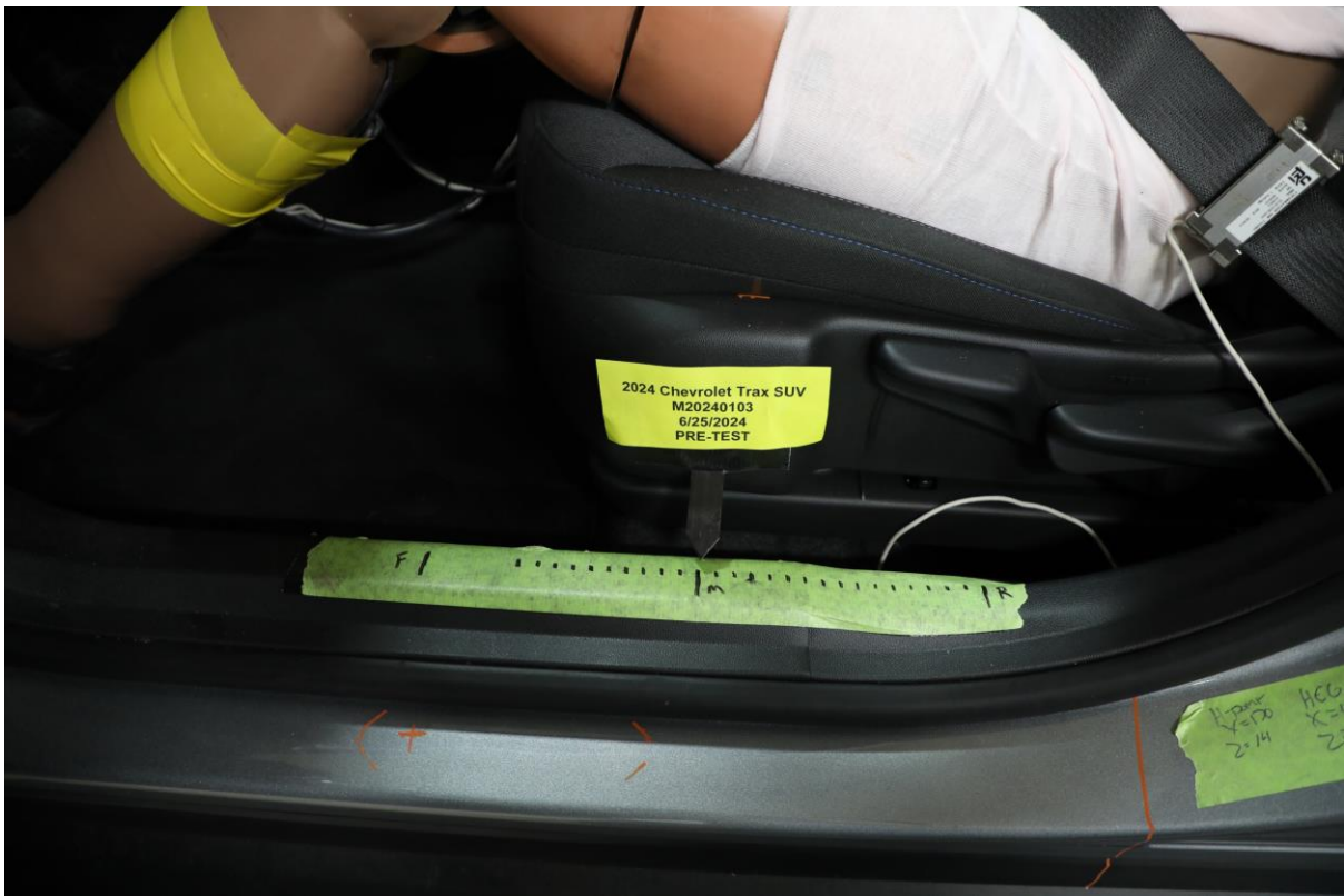
036 Pre-Test Driver's Seat Fore-Aft Markings
