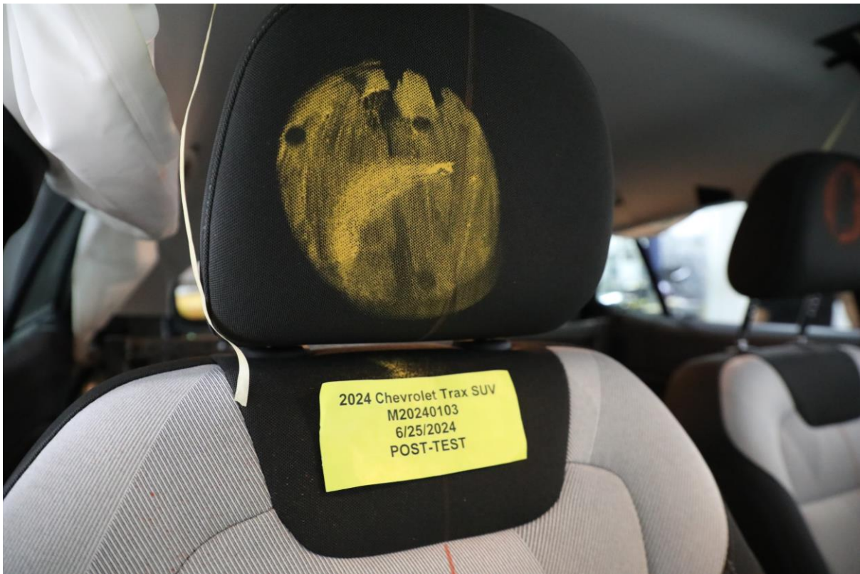
073 Post-Test Passenger Dummy Contact with Headrest
