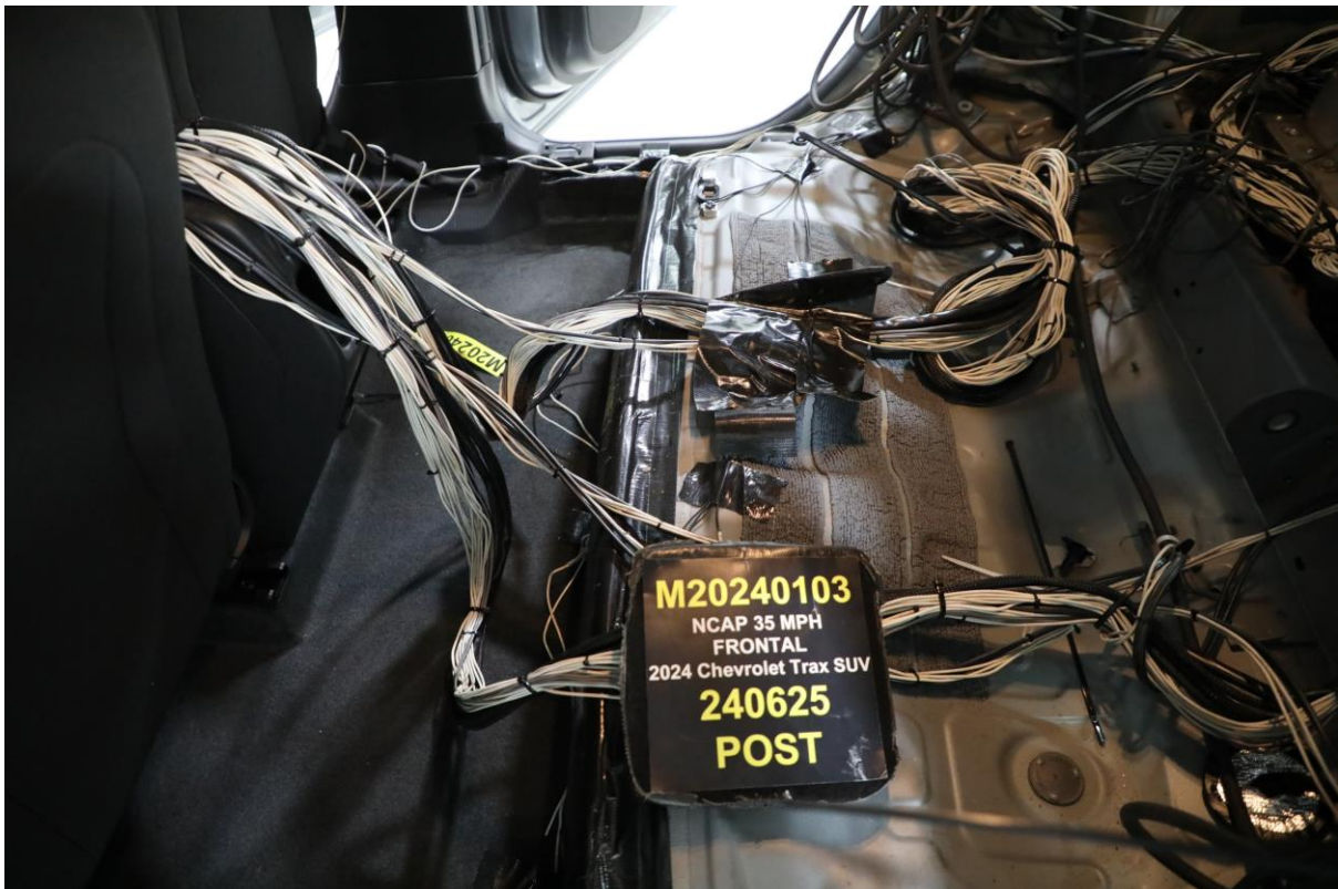
029 Post-Test Dummy Cable Routing
