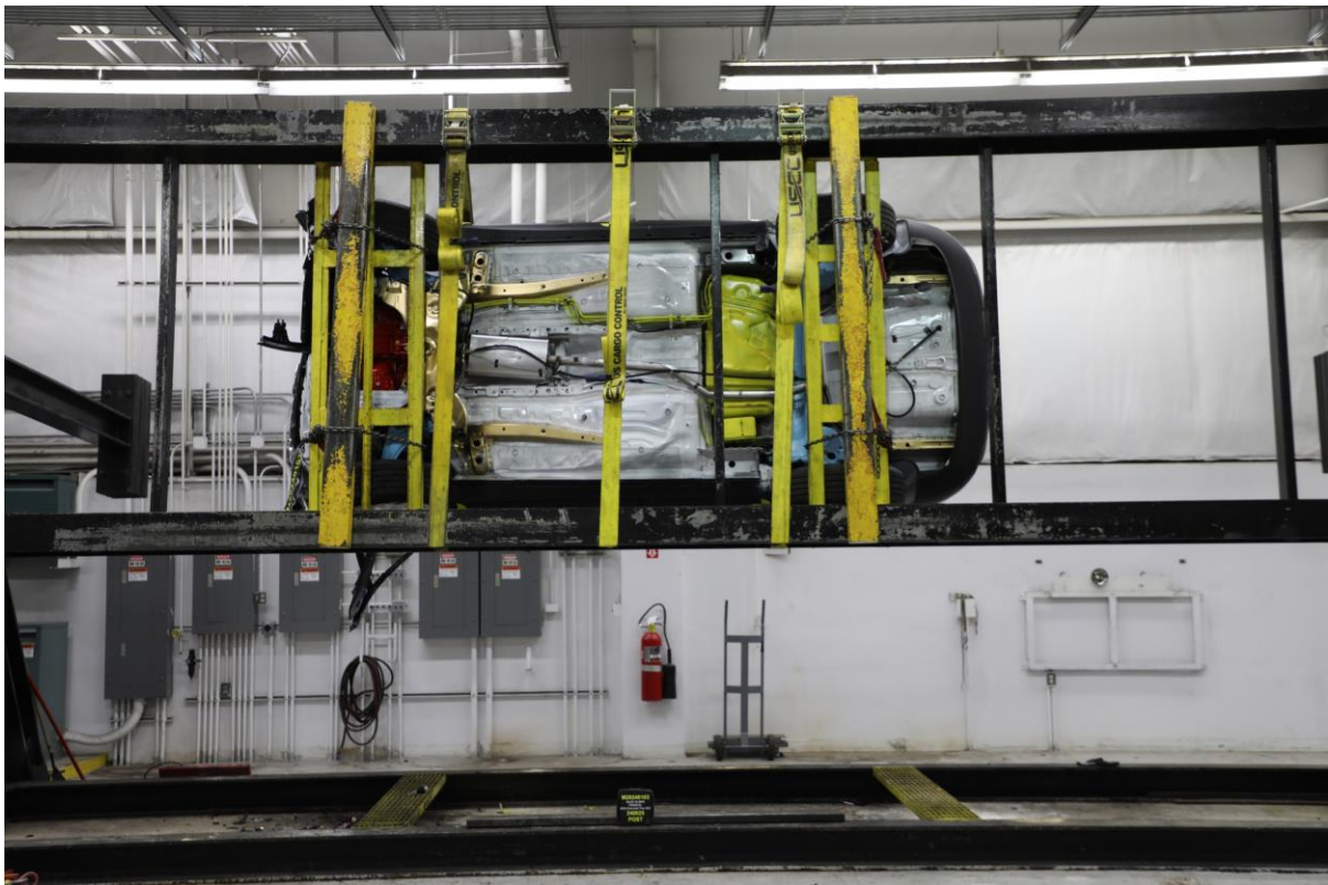
080 Vehicle at 270° on Static Rollover Device
