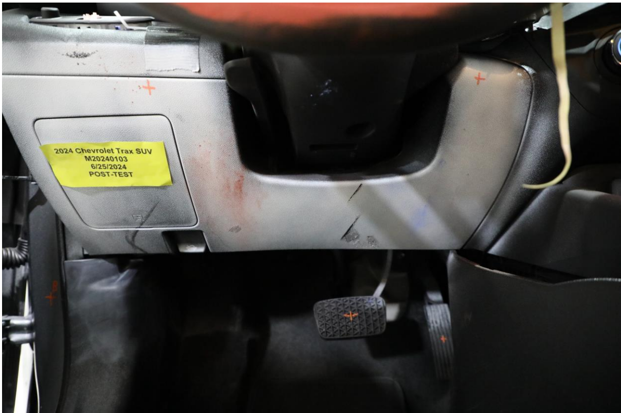
045 Post-Test Driver's Side Knee Bolster
