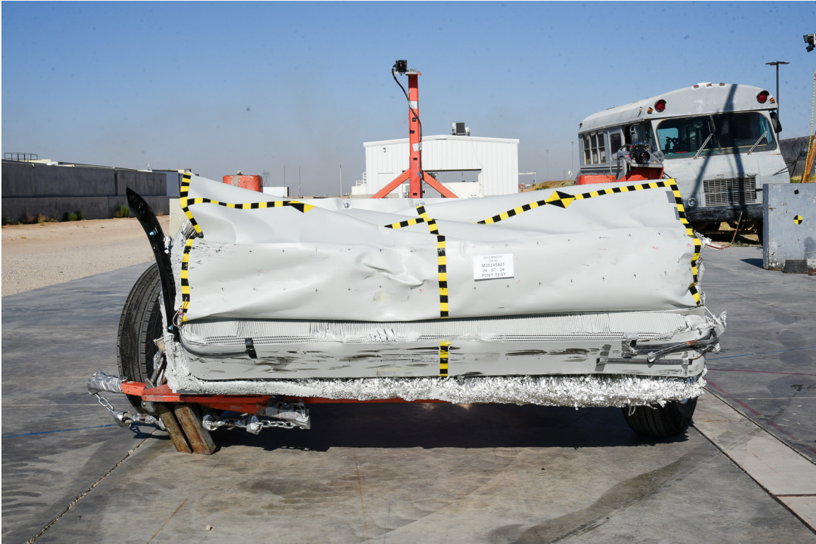
FIGURE 85. Post-Test Front View of MDB Impactor Face
