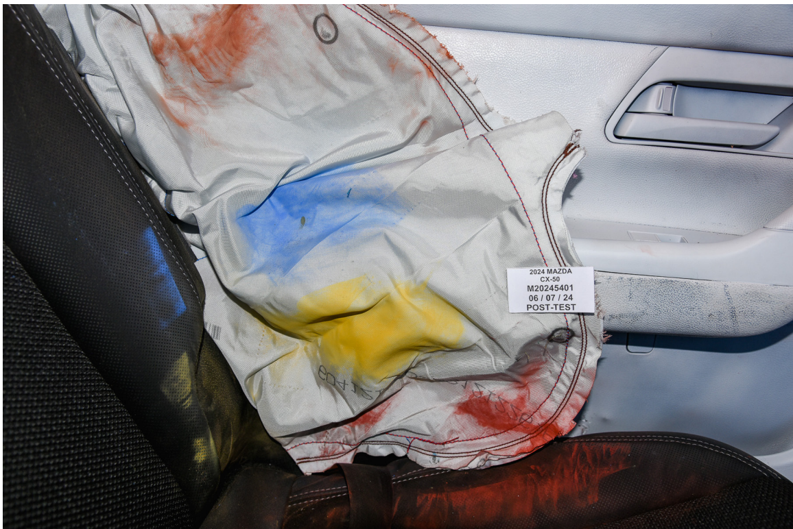
FIGURE 78. Post-Test Rear Passenger Dummy Close-Up Torso Contact with Vehicle Side Airbag View
