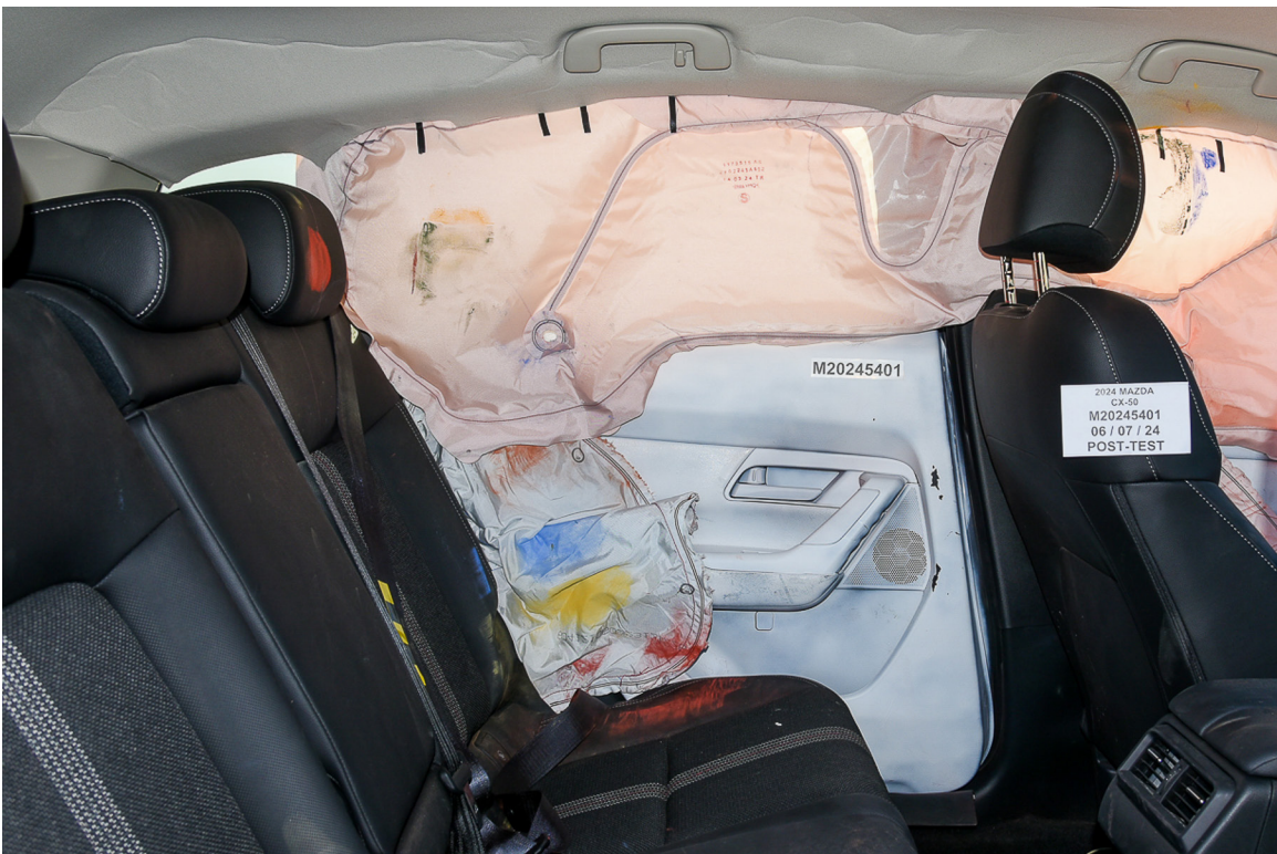
FIGURE 74. Post-Test Rear Passenger Inner Door Panel View
