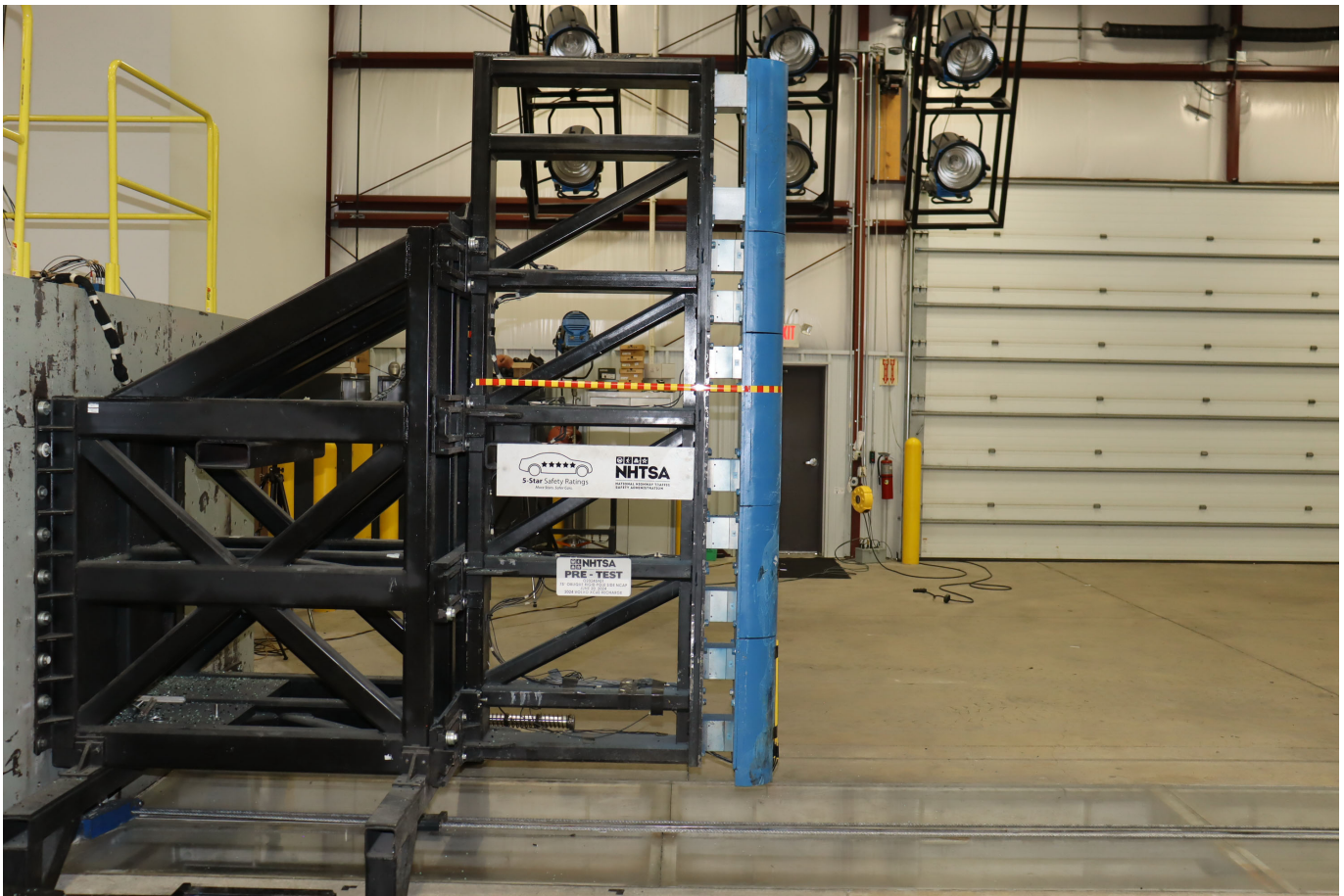
Photo No. 061 - Pre-Test Pole Barrier Side View
