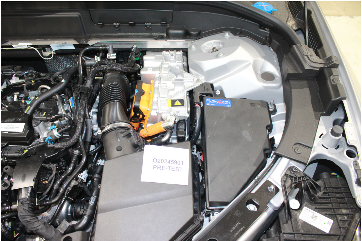
Photo No. 305-02 - Power Inverter Warning Label
