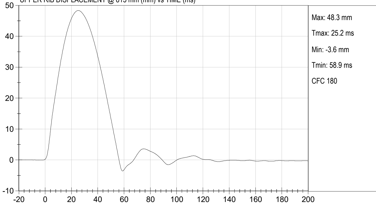
UPPER RIB DISPLACEMENT @ 815 mm (mm) vs TIME (ms)
