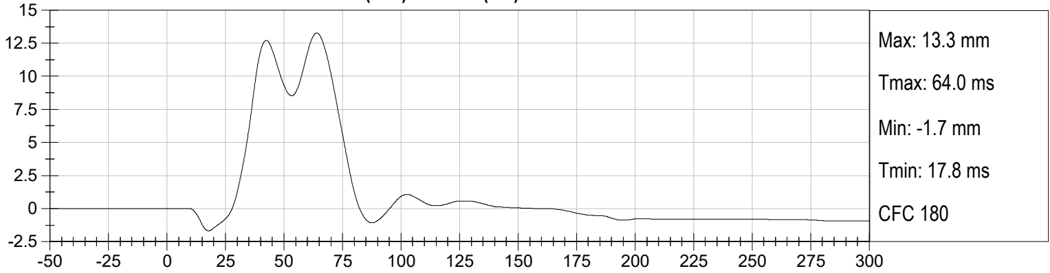
DRIVER MID RIB DISPLACEMENT (mm) vs Time (ms)
